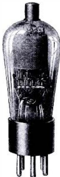
the special cathode construction, the heater voltage may vary during the charge and discharge cycles of the automobile storage battery, without affecting seriously the performance or serviceableness of this tube. No resistor in the heater circuit is required for operation from a six volt battery.
