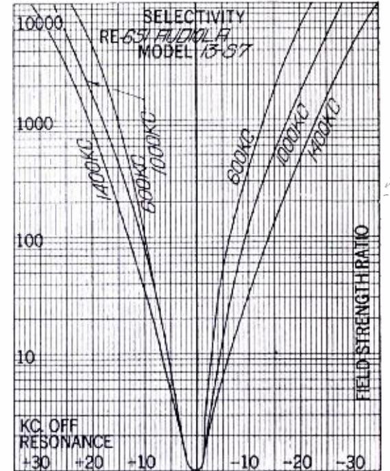
noninductive load resistance of 7000 ohms was connected across the plate circuit of the single 247 pentode output tube, which in turn was capacitatively coupled to the output indicating tube voltmeter, which read the standard audio level of .05 watts, except for power overload measurements. To prevent its impedance reflection on the plate circuit of the output tube, the voice coil circuit was disconnected during measurements.
