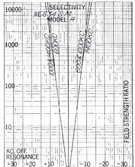
uuf and 25 ohms, connected across the chassis antenna circuit. A load resistance of 7000 ohms was connected across the plate circuit of the output pentode to match its operating load impedance. In order to prevent the loading effect of the voice coil circuit, it was opened for all measurements. The vacuum tube voltmeter was capacitatively coupled to the plate circuit, and indicated a standard output level of .05 watts, except for the power overload measurements.
