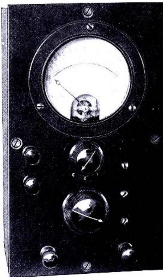
the value specified as 43,000 ohms, for which a 50,000 ohm unit was employed. To adjust this resistor the terminal at one end was loosened and moved along until, with a 45 volt battery, the terminals marked X shorted, and the rheostat set to about its middle position, the meter read just full scale, i. e., zero ohms.
