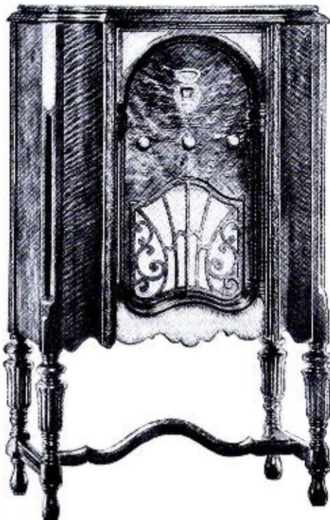
The Sentinel model 118 uses two 224 screen grid, two 235 variable mu, three 227 triode, two 247 pentode, and one 280 rectifier tubes.
