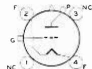
up to 100 Mc. Class C Telegraphy maximum plate dissipation, CCS 125 watts, ICAS 175 watts.
