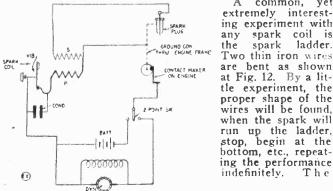
A common, yet extremely interesting experiment with any spark coil is spark ladder. the Two thin iron wires are bent as shown at Fig. 12. By a little experiment, the proper shape of the wires will be found, when the spark will run up the ladder, stop, begin at the bottom, etc., repeatheated air caused by the passage of the spark, is the reason for the spark tending to rise. Heated air is a better con-ductor than ordinary air.
