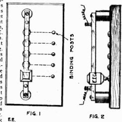
piece of copper wire run to each corresponding binding post as shown. Put a number 2222 Hard rubber slider on the rod and nail down through the pillar on to the base, so that slider will pass over brass tacks nicely. The switch is completed except for a coat of varnish. It is connected up just the same as a multipoint switch only it has a binding post for buzzer test connection.
