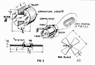
winding terminals are soldered to the segments. The shaft of steel, iron or brass is detailed at Fig. 3, and needs no special description. The armature laminations, forming the special description. The armature laminations, forming the core "H," are locked between two No. 10-32 nuts threaded on the shaft. The commutator core is drilled out to make a driving fit on the shaft.
