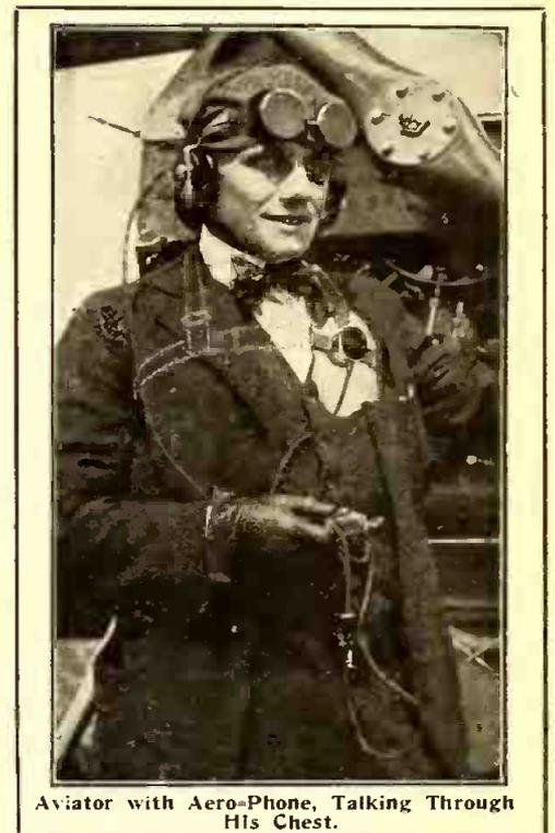
s-tered in a jack mounted on the framework of the aeroplane. The only battery current required is that furnished by three regular dry cells, which will provide continuous service for 100 hours without any appreciable loss of transmission quality.
