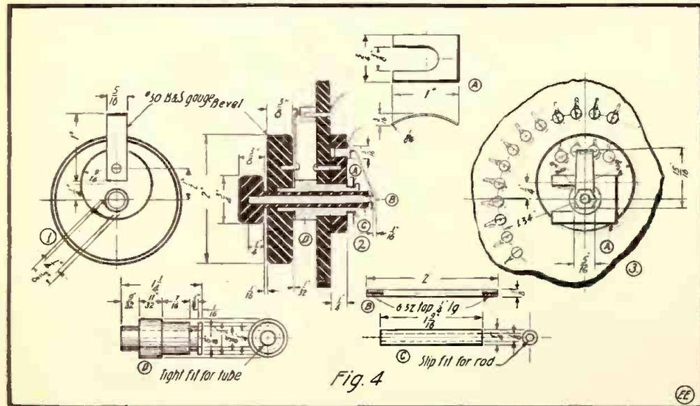
Fig. 4. Parts Making Up "Primary" Switch of Coupler.
