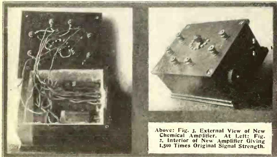
Above: Fig. 3. External View of New Chemical Amplifier. At Left: Fig. 2. Interior of New Amplifier Giving 1,500 Times Original Signal Strength.
