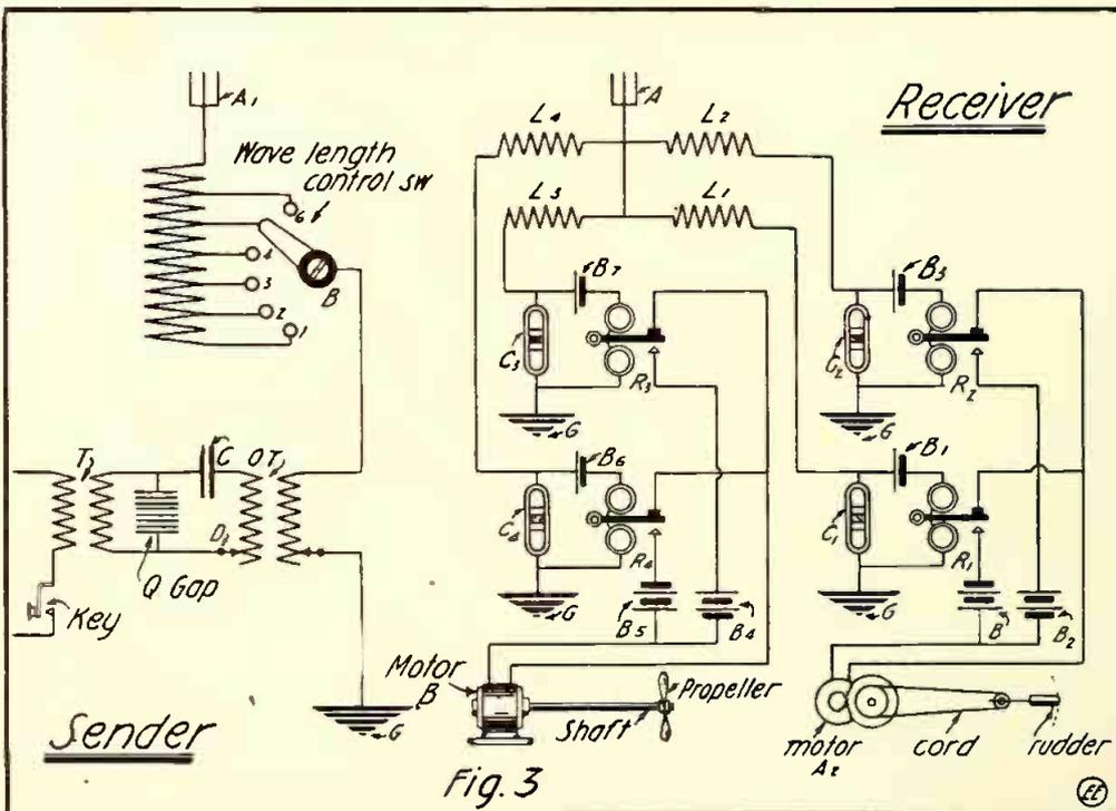
Fig. 3. Control Circuits for Wireless "Telemechanics."
