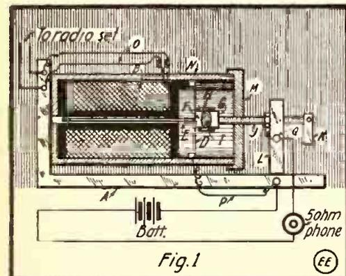
Fig. 1. Diagrammatic View of New Chemical Amplifier.
