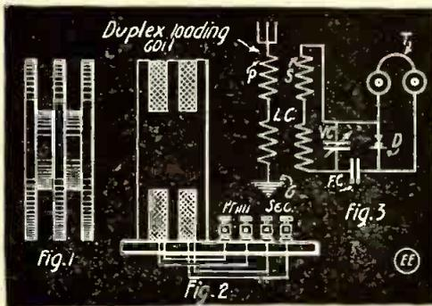
Making a Duplex Loading Coil.
