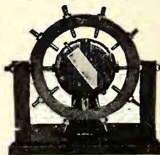
Gives 600 cycle whistling spark like a quenched gap. Attains full speed in 1 second; stops dead inside of 3 seconds. You do not have to wait for this Rotary to start nor do you have to wait for it to stop. It always beats you to it. The light revolving discharger arm allows a quick start and quick stop. Will work on sets up to 1 K. W. Used on 60-cycle current.
