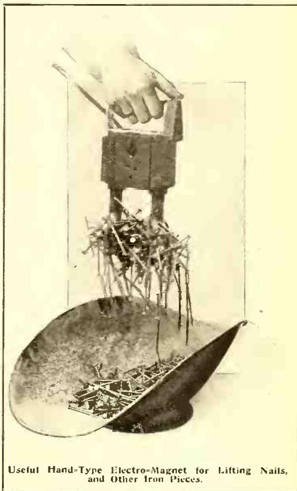
Useful Hand-Type Electro-Magnet for Lifting Nails, and Other Iron Pieces.
