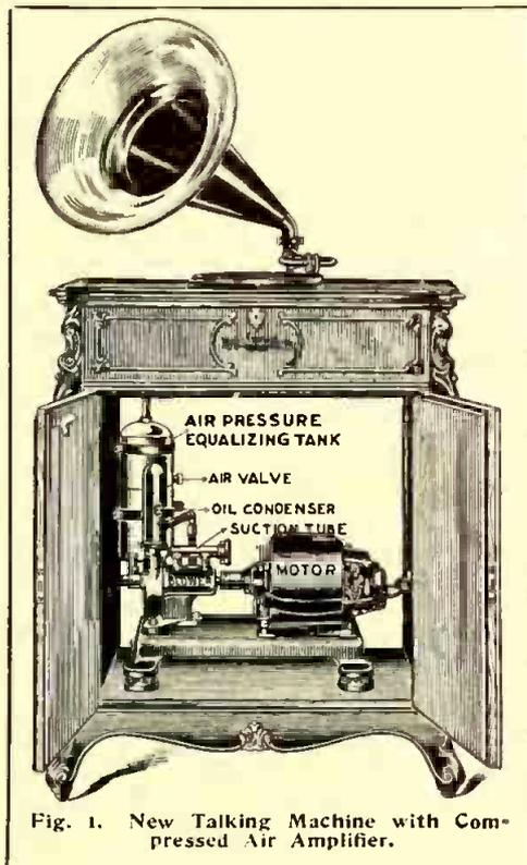
Fig. 1. New Talking Machine with Compressed Air Amplifier.
