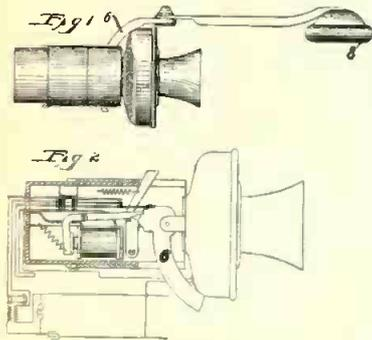
cause the switch springs, as perceived, to automatically control the cutting in and out of circuit of the telephone transmitter and receiver, instead of having to hang up the receiver in the usual way. A very good idea.
