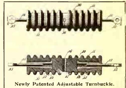
Newly Patented Adjustable Turnbuckle.
