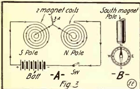
Fig. 3. Hooking Up Magnet Coils for Proper Polarity.
