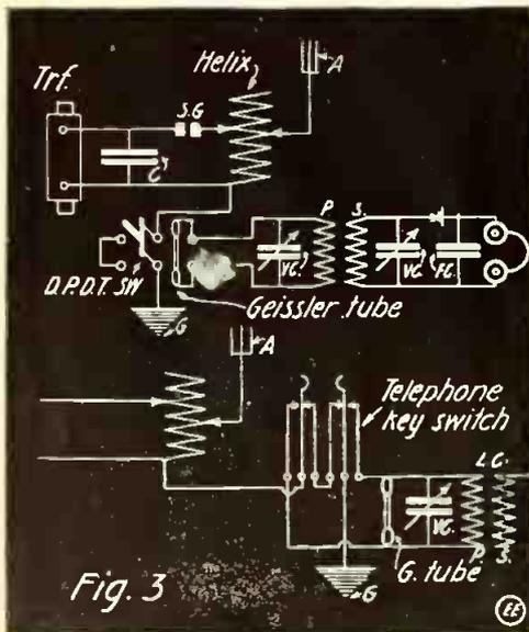
Fig. 3. Simplified Transmitting and Receiving Radio Hook-ups.
