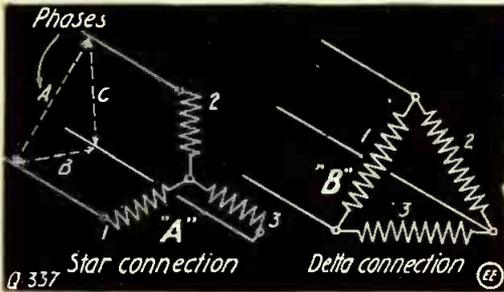
Alternating Current Hook-ups, at "A" the Star Connection; at "B," Delta.
