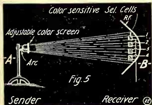
Fig. 5. Using the Selenium Cell for Wireless Control.
