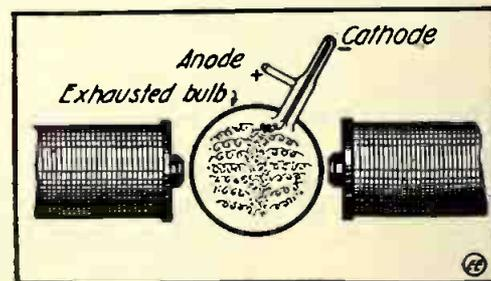
Fig. 3. Producing an Artificial "Aurora Borealis" in the Laboratory.
