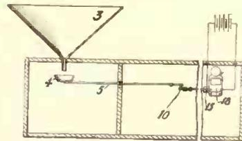
a spring switch 15, which closes the battery circuit for an electric alarm bell 18 or instead, this circuit may control an electric motor for closing windows or skylights.
