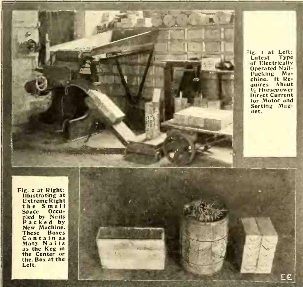
Fig. 1 at Left: Latest Type of Electrically Operated Nail-Packing Machine. It Requires About 1/2 Horsepower Direct Current for Motor and Sorting Magnet.
