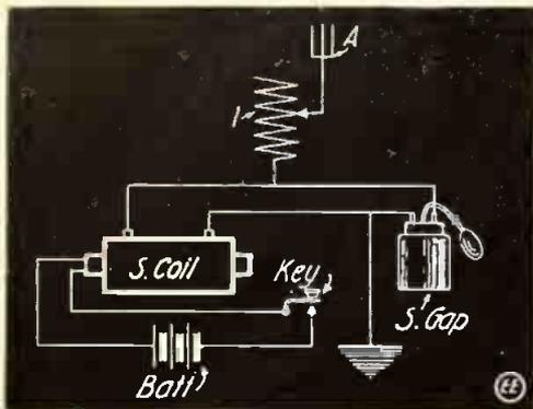
Fig. 1. Connections for Compressed Air Spark Gap.
