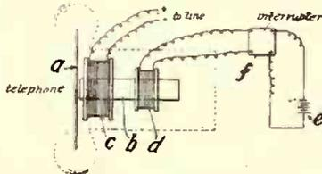
in a constant state of vibration, at a frequency above audibility, that the ordinary sound waves to be reproduced by the diaphragm from the telephone line coil C, in the usual way, will be much clearer and freer from distortion or false tones than in the usual way, where the diaphragm is allowed to vibrate by itself.
