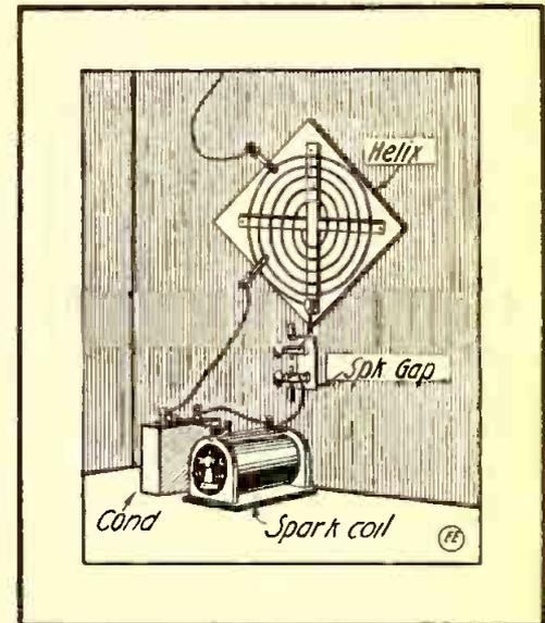
Fig. 2-B. Short Wiring Possible for Radio Set on Table and Wall.
