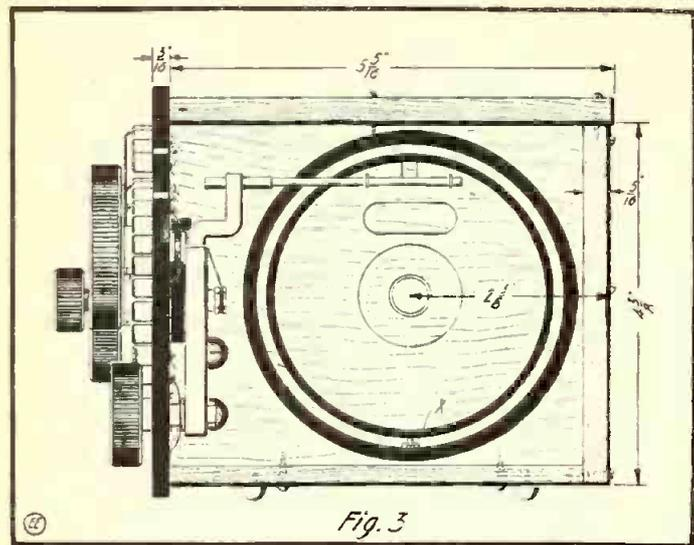
Fig. 3. Assembly of Primary and Secondary Coils in Cabinet.
