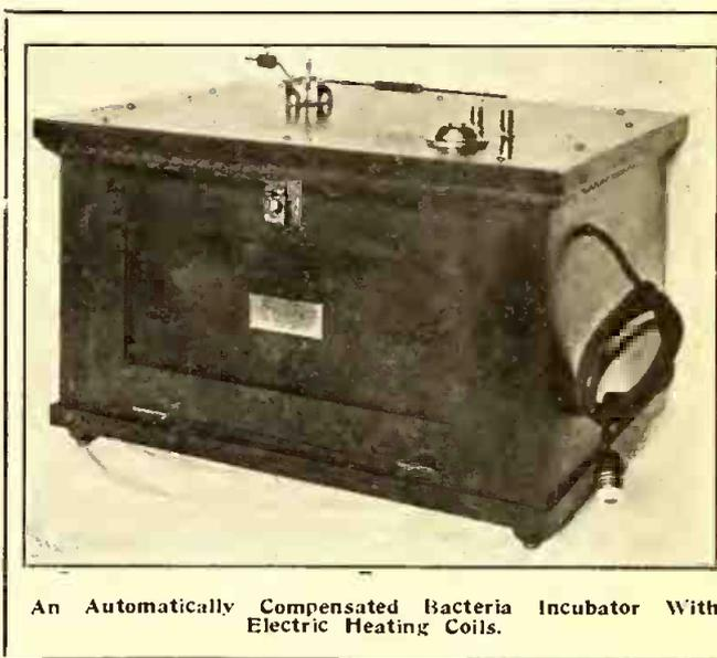
An Automatically Compensated Bacteria Incubator With Electric Heating Coils.
