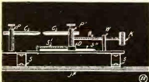
Efficient Hand-feed Arc Lamp.
