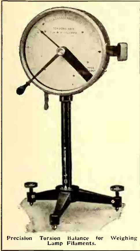
Precision Torsion Balance for Weighing Lamp Filaments.
