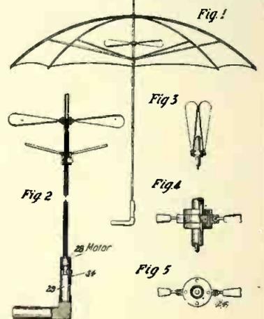
stem, as is evident. This shaft connects with a miniature electric motor 28, which receives current from a small flashlight type battery 29, in the handle of the umbrella. A push button 34 controls the battery current to the motor. The expense in making up this arrangement and also considering the gross efficiency, and especially the small "breeze producing power" in this case, does not seem to warrant at all the expense in making up such an arrangement.
