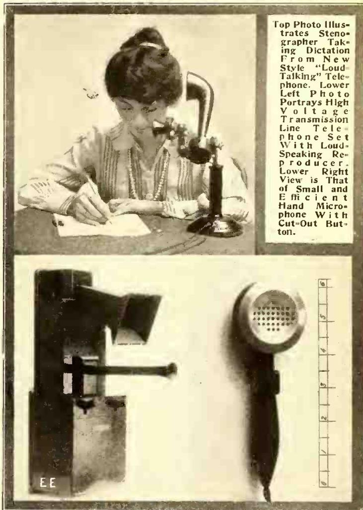
Top Photo Illustrates Stenographer Taking Dictation From New Style "Loud-Talking" Telephone. Lower Left Photo Portrays High Voltage Transmission Line Telephone Set With Loud-Speaking Reproducer. Lower Right View is That of Small and Efficient Hand Microphone With Cut-Out Button.
