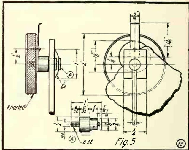
Fig. 5. Details of Secondary Switch.
