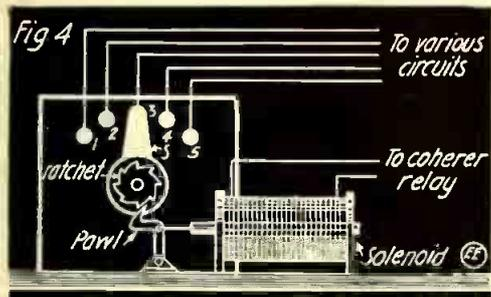
Fig. 4. "Step by Step" Radio Control Relay.
