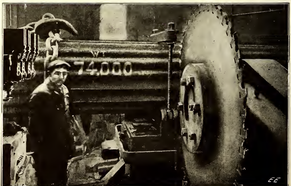
Sawing a 74,000 Pound Steel Ingot in Half with a Cold Saw. The Saw is Motor Driven. The Saw Teeth Never Touch the Steel—the Air Compress in Front of the Teeth Does the Cutting.
