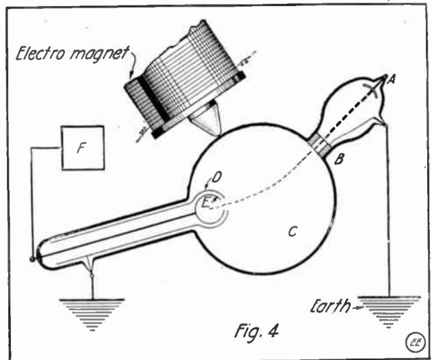
Fig. 4.—Evacuated Glass Bulb and Powerful Magnet Used to Prove Cathode Rays Are Negatively Charged Particles.
