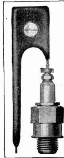
It consists of a crotch containing a spark gap and two legs containing the terminals. One leg is three inches longer than the other, so as to permit of convenient contact.
