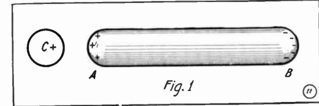
Fig. 1.—Charging a Metal Rod A-B by Induction from Sphere C.
