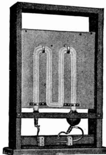
New Mercury Vapor Lamp for Photographers
