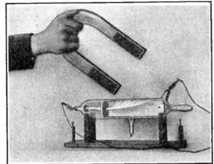
Fig. 5.—Cathode Ray Being Deflected by a Magnet
