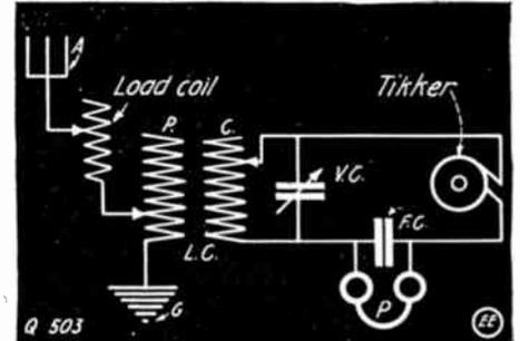
**"Tikker" Hook-up for Undamped Waves**
