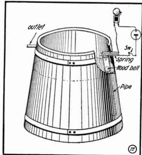
Wooden Ball Floating in Pipe Actuates High-Water Alarm Switch.
