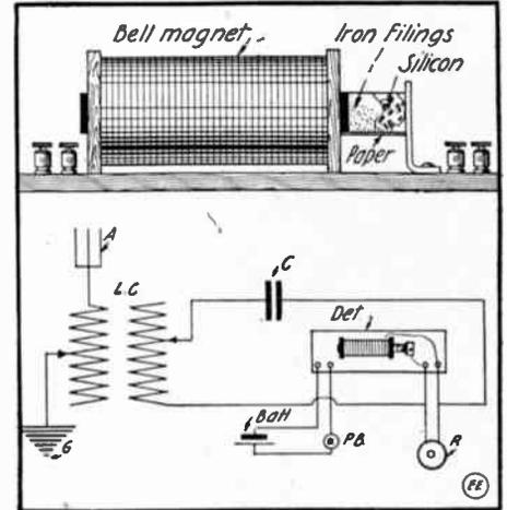
Electro-magnetic Control for Detector.
