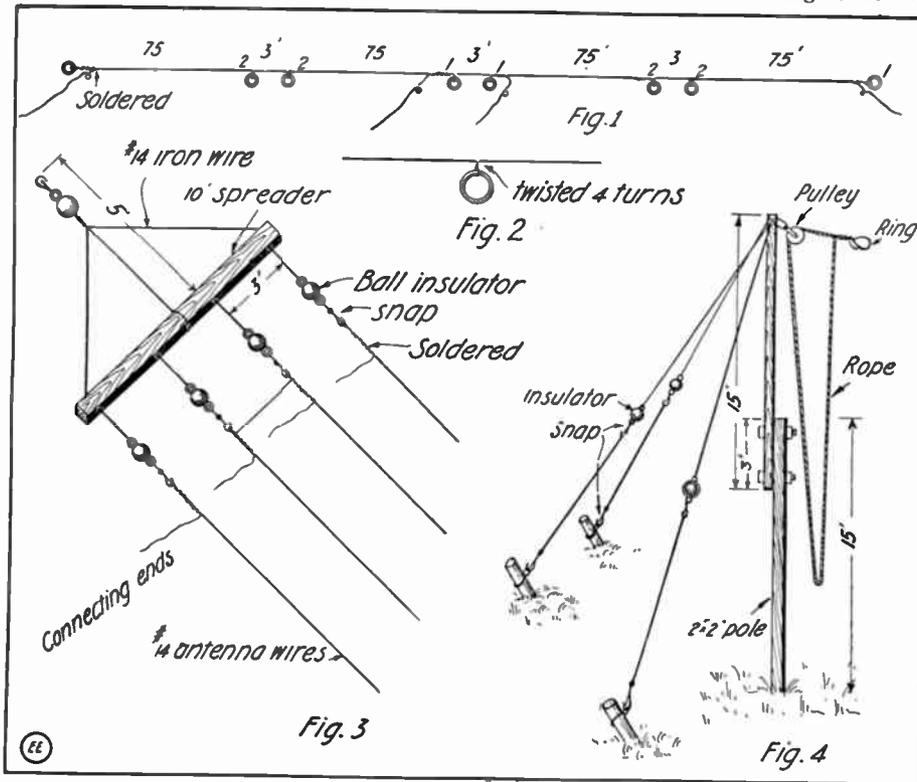
Design for Portable Aerial and Mast Suitable for Boy Scout Maneuvers, Camping, Testing, Etc.
