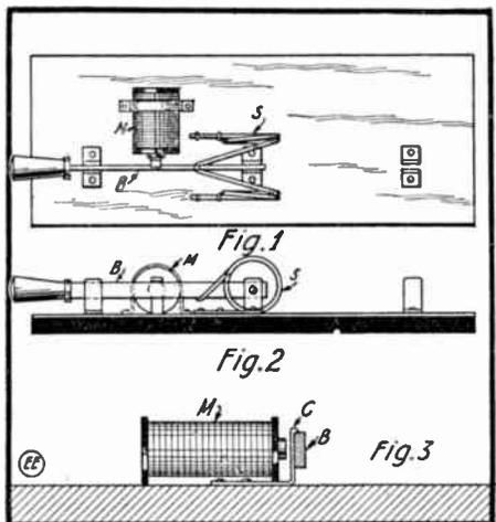
Release Magnet Coil Fitted to Lightning Switch.
