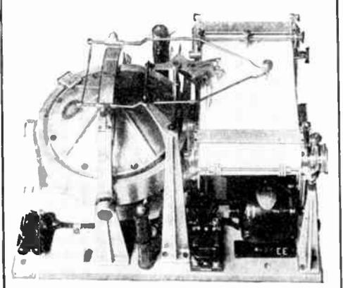
Fig. 3 (Left): Type of Stabilizing Gyroscope Installed on U. S. S. *Worden*. Fig. 4 (Centre): Small Auxiliary Gyro Used to Control Larger One Seen at Left. Fig. 5 (Right): Latest Type of Gyroscopic Pitch Period and Amplitude Recorder. Produces Graphic Chart Accurately Timed.
