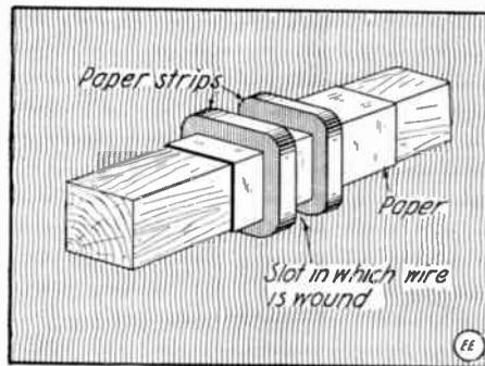
Fig. 3. How Form Is Constructed for Winding Galvanometer Coil.
