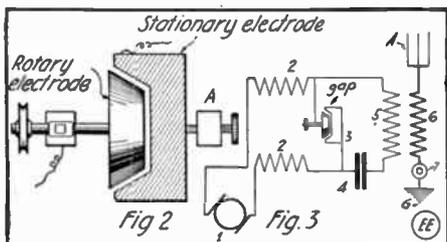
**Details of Dubilier Rotary Quenched Spark Gap.** through a key or microphone 7, as depicted in illustration.
