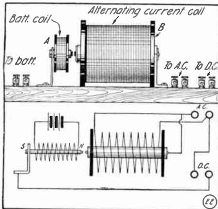
Magnetic Type of Polarized Rectifier.
