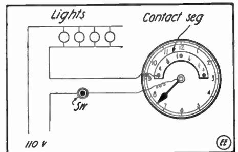
Time Switch Constructed from Any Clock.
