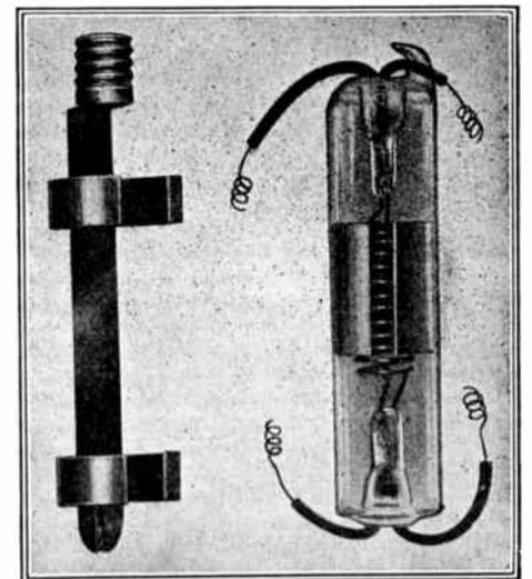
Latest Audion Detector and Holder Adapted to Screw Into Any Standard Socket.
