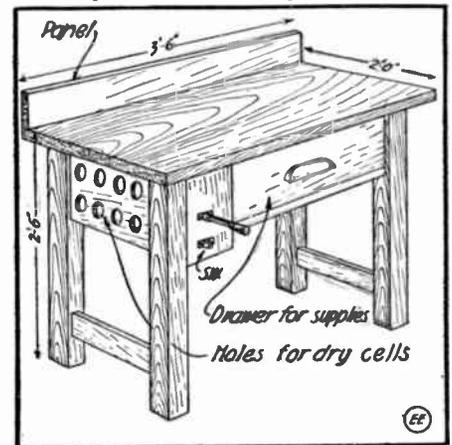
Neat Design of Radio Table with Tool and Apparatus Drawer.
