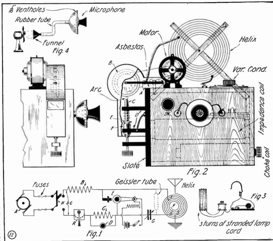
Details and Assembly of Experimental Radiophone Arc and Auxiliary Apparatus.
