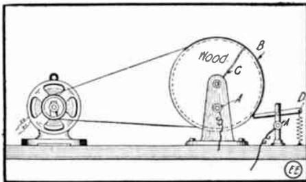
Easily Made Rotary Flasher for Battery Lamps.
