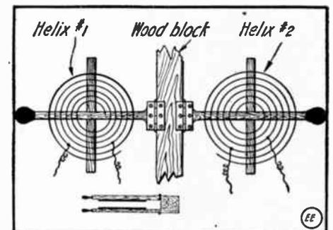
Efficient Mounting for Oscillation Transformer.
