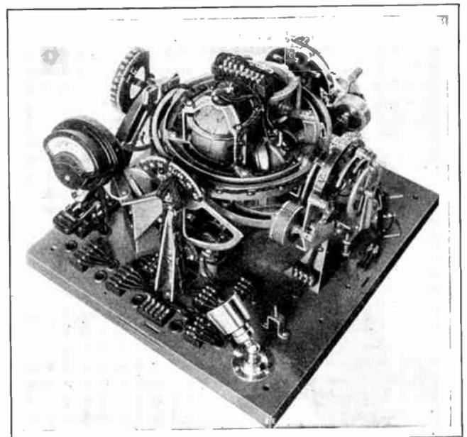
Fig. 6. Automatic Gyroscopic Stabilizing Set for Aeroplanes.
