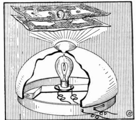
Clever Device for Detecting Counterfeit Money. counterfeit bills, owing to the distinct difference noticeable in the paper pulp and fiber structure of same, as compared with genuine bills.
