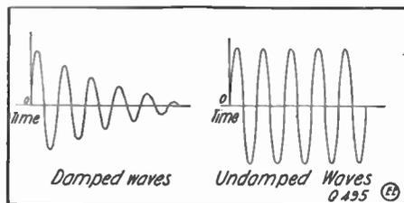
Showing Difference Between Damped and Undamped Waves.
