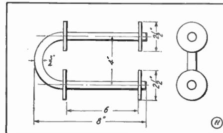
Powerful Electro-magnet Suitable for Use on Batteries.
