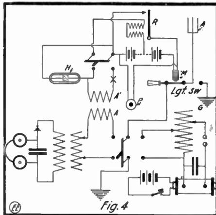
Hook-up of Automatic Lightning Switch in Radio Station Circuits.
