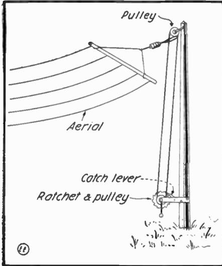
Scheme for Raising Aerial by Means of Ratchet Wheel and Crank.
