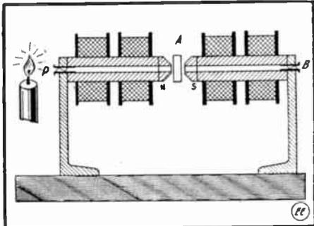
Apparatus for Demonstrating Effect of Magnetism on Light.
