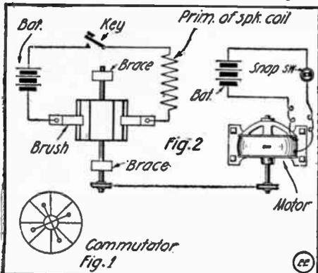
Utilizing Regular Commutator as Spark Coil Interrupter
