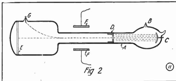
Fig. 2.—Special Cathode Ray Tube for Studying Their Characteristics.
