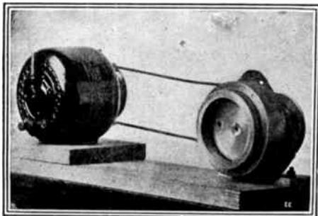
**Fig. 1. New Form of Rotary Quenched Gap of Very Simple Design.**
