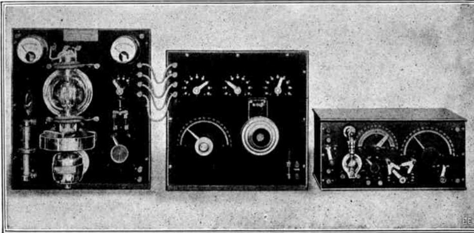
Improved Vacuum Bulb Generator Type of De Forest Radiophone Sending and Receiving Apparatus.
