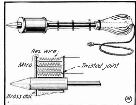
A Useful Electrically Heated Soldering Iron, up well by filing to a good point, then tin it thoroughly. Procure several sheets of thin mica (about .002 inch in thickness) and wrap it around the iron until you have five or six layers on. Obtain 20 feet of No. 26 nichrome resistance wire and two feet of No. 16 asbestos-insulated copper wire.
