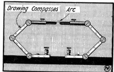
Battery Arc Lamp Made from Pair of Drawing Compasses.
