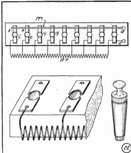
Efficient Form of Rheostat Using Plug Type Switch.
