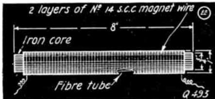
Details of Choke Coil for 1/2 K. W. Transformer Circuits.
