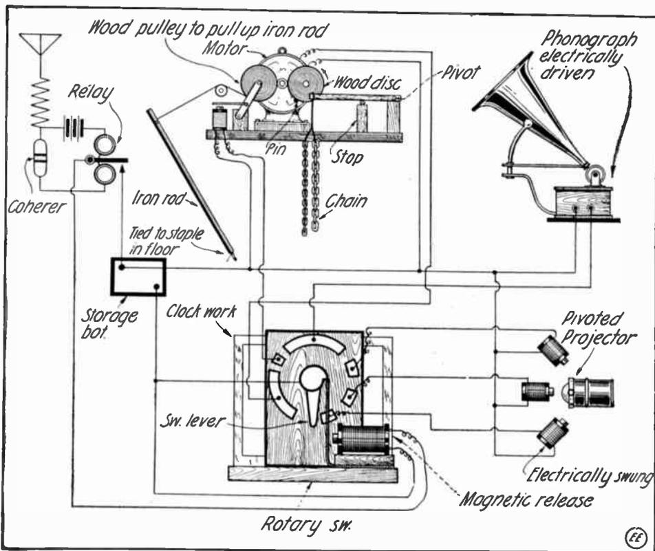
Simple Apparatus Used by the "Wireless Wiz" to Create the Haunted House Effect
