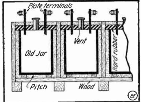
Scheme for Repairing Cracked Storage Battery Jars.
