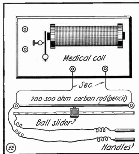
Potentiometer Method of Regulating Shock Coil Secondary Current.
