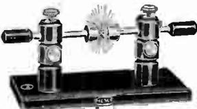
Adapted for stations up to 1/2 K.W. capacity. Base is of polished hard rubber. Standards are of hard rubber composition of the highest insulating properties. Hard rubber ends on the brass rods permit the length of the gap to be varied, while sending. Spark terminals are of zinc, and are renewable.
