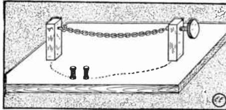
Battery Rheostat Made From Piece of Chain.
