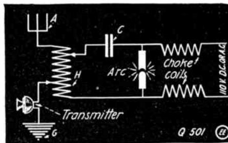
**Wireless Telephone Hook-up for Arc Generator**
