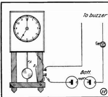
Clock Pendulum Makes and Breaks Test Buzzer Circuit.
