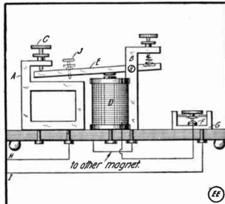
Scheme for Hooking up Telegraph Sounder to Act as Buzzer.
