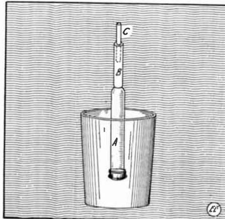
Simple Method of Filtering Quicksilver.
