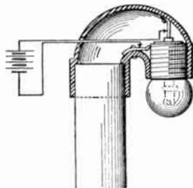
indicated and adapted to fit a pencil and also to contain an electric lamp receptacle. Two wires from the receptacle lead out to an external battery. This device would seem adaptable to use with a fountain light battery, which is already on the market.
