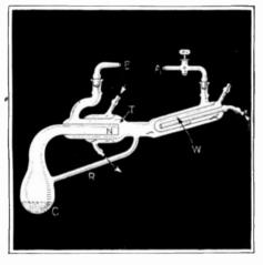
Fig. 1 Shows All-Glass Mercury Vapor Vacuum Pump. The Boiler C, Containing Mercury, is Placed in the Flame of a Bunsen burner. The Vessel to be Exhausted is Connected to B. A Mechanical Vacuum Pump is Connected at A, While the Inner Condenser W, is Cooled by Water Circulating Through It.
