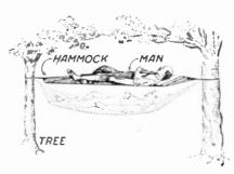
Is There a Greater Strain on the Ropes Sup-porting the Hammock Rigidly Between the Two Trees, as Compared to the Lower Sagging Position Shown in Dotted Lines?
