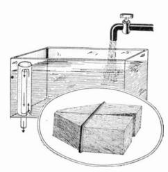
The Correct Method for Allowing the Water to Flow Out of a Washing Tank, is Shown Above, While the Insert Shows the Construction of the Cork Clip Which Holds the Prints and Floats Upon the Surface of the Water.
