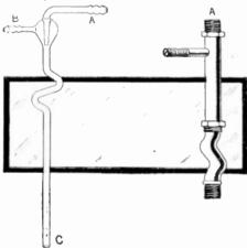
Fig. 2. A Water Jet Pump Will Produce a Pair Degree of Vacuum. This Type of Pump is Fre-quently Used to Back Up a Mercury Vapor Pump,
