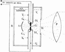
Fig. 2. Sectional View of the Cleverly Designed Short Wave Transmitter. The Short Tungsten Electrodes H1 and H2. Are Charged Through Spark Gaps G1 and G2. The Waves Are Reflected by M, and Focused by the Paraffine Lens P.
