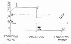
Through What Changes Would the Pitch of a Fire Engine Bell Appear to Pass to the Observer Listening to the Bell from a Point Midway Between the Starting and Stopping Points, Along a Straight Course Followed by the Engine.
