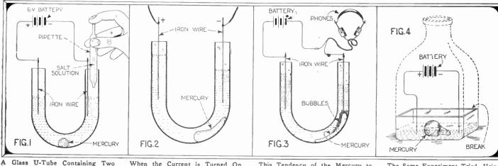
A Glass U-Tube Containing Two Iron Terminals Connected to a Suitable Source of Current and a Drop of Mercury, is Filled with Salt Solution from a Pipette.
