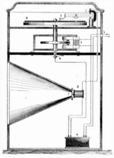
Here is an Idea Worth Developing. This Phonograph is Entirely Electrical From the Driving Motor to the Reproducer and Loud Speaker.
