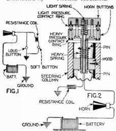
A Two-Tone Push Button Which Can Be Mounted on the Steering Column So as to Give a Low Note for City Driving, and by Pushing Real Hard on the Button a Stronger Note for Country Driving
