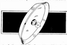
An Ordinary Flat Tin Pan with a High Candle-Power Lamp and Socket, Mounted in the Center of It. This Whole Contraption Fastened Underneath the Car Provides a Very Good "Ground Light," as an Aid in Marking Out the Car When You Have the Headlights Dim, and Also for Shooting Trouble at Night Underneath the Car.
