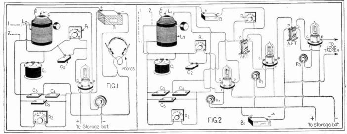
The Flewelling Circuit Which Has Created Such a Sensation Among Amateurs is Shown Above. At the Left the Standard One-Tube Circuit is Shown, and Each Instrument Clearly Drawn so that the Novice Will Have no Trouble in Hooking Them Up. To the Right is Shown the Same Circuit with the Addition of Two Stages of Audio-Frequency Amplification. When a Loop is Used, It Should be Connected to Points Marked 1 and 2.
