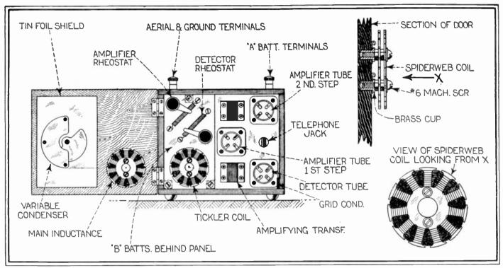
The Constructional Details of a Tuner, Detector, and Two-Stage Amplifier, Contained in a Cabinet Only 5" High by 6" Wide, by 5\%" Deep, Are Plainly Shown Above. The Spider Web Coils Are Wound on Fibre Armature Disks, as Shown in the Lower Right Hand Corner, and They Are Mounted as Shown in the Upper Right Hand Corner.
