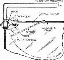
A Motor-Driven Windshield Cleaner, the Motor Being of the Six-Volt Type and Operated from the Storage Battery.
