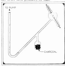
A Vacuum Can Be Produced by Absorb-Gas in the Vessel by Charcoal Cooled to the Temperature of Liquid Air.
