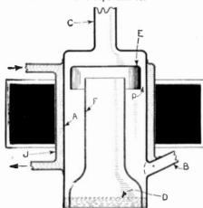
Fig. 3. A Condensation Pump Constructed of Metal is Shown in This Figure. The Air from the Vessel Under Exhaustion Connected at C, Passes Out C, Through Passage P, and is Removed via B, by Means of the Backing Pump.
