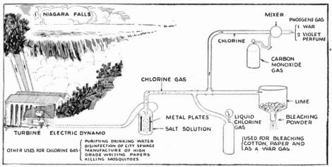
There Are a Great Many Uses For Poisonous Gases in Industry For Both War and Peace-time Uses. The Cheapest Way of Making the Products From the Gas is to Use Current Generated at Large Hydro-Electric Plants for Producing the Gas, and Develop the By-Products in the Same Plant.
