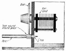
Fig. 6. Handy Vernier for Condenser Dials Made from a Lead Pencil, and a Piece of Friction Tape.
