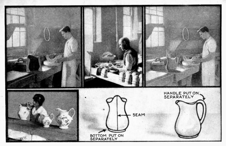
Do You Know the Various Stages Through Which Your Clay Water Pitcher Went in Its Manufacture? The Photographs from Left to Right, Beginning with the Top Row, Show the Two-Part Mold and How the Wet Clay is Molded Therein; Also How the Handles of Such Pitchers, Tea Cups, etc., Are Put on Separately, and the Ware Then Glazed and Decorated with Stencils or Otherwise, by Painting.
