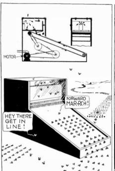
A Fly-Trap Designed by an Ambitious Inventor is Illustrated Above. The Sectional Elevation at the Top of This Illustration is Taken From the Patent and the Comic Version Shown Below. Notice the Endless Belt Used to Convey the Flies
