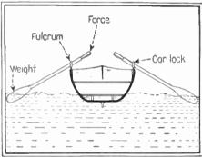
A Diagrammatical View of a Rowboat and Its Oars Are Shown Above. This Illustrates the Lever Action Which is Explained in the Text.
