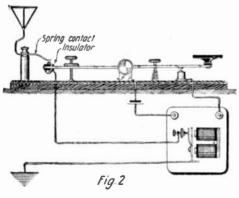
At the Left, is a Side View of the Key Used For Transmitting Music by Means of a Buzzer. Note That the Antenna Circuit is Closed at the Same Time That the Battery Circuit is Completed.
