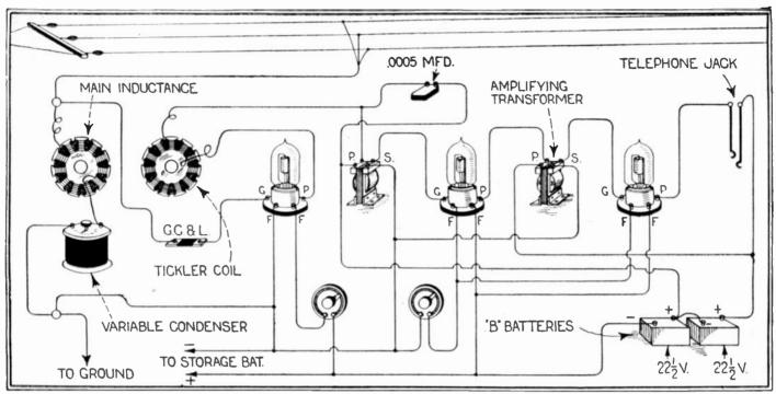
The Circuit Diagram for Connecting the Compact Radiophone Receiving Set Described by Mr. Fitch, is Given Above. This Circuit is Regenerative, and is of the Feed-Back Type. Note that the Filaments of the Amplifying Tubes Are Both Controlled With One Rheostat.
