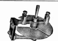
The Air Gap in the Vernier Condenser Above Shown, May Be Adjusted So That a Very High Capacity Can be Obtained.
