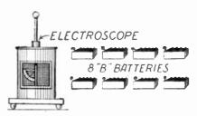
A Man Wishes to Charge an Electroscope to a Potential of 1,000 Volts, and He Possesses Eight Radio "B" Batteries, Each One of Which Supplies a Potential of 22½ Volts. Could You Tell Him How to Obtain the Necessary 1,000 Volts D. C, From These Eight Batteries?
