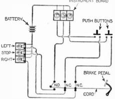
The Inventor of this Rinktum Provides Tell-tale Signal Lamps on the Dash for His Stop Signals, and Has Also Ingeniously Provided an Interlocking Switch Arrangement Tied Fast to the Brake Pedal, so That if He Should Use the Brake, the Stop Light Will Flash on at the Rear, but the Right and Left Switchea Will Be Opened Simultaneously, so as to Prevent Confusion of Signals.
