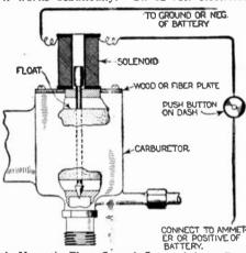
A Magnetic Float Control Operated by a Push Button from Driver's Seat, So as to be Able to Flood the Carburetor at Any Time Desired; Par-ticularly Useful in Starting Engine.
