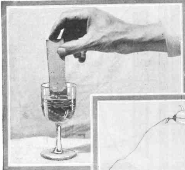
Hot water is lighter and floats upon cold water. A bit of paper coated with luminous paint will show this because the heat will cause the top part to glow. Below: A common medicine, salophen, will glow if rubbed between glass surfaces.
