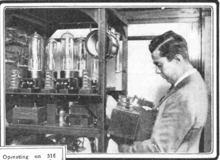
Operating on 316 meters, the law demands that no deviation from the allotted wave-length be allowed. The engineer checks up the wave-length daily.
