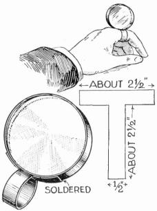
When reading fine type or doing other work which requires the constant use of a small magnifying glass, the usual handle with which these glasses are equipped is rather awkward and tires the hand. If a strip of metal is cut to a T shape with the dimensions shown above and soldered to the metal rim surrounding the glass, the combination may be used as shown.
