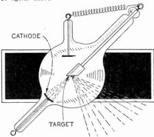
The above shows a common form of X-ray The target may be of platinum, and the cathode of aluminum.
