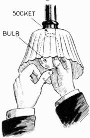
A simple and safe method of taking out and putting electric light bulbs into sockets is illustrated above. Rest the glass tip of the bulb on the thumb and screw the bulb in with the other hand. The thumb prevents the bulb from falling.
