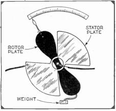
An electrostatic voltmeter may easily be made using thin variable condenser plates. must be calibrated from a standard meter.
