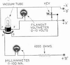
When buying tubes be sure that they come up to the highest possible standard. In order to ascertain this, construct a vacuum tube tester as shown above.
