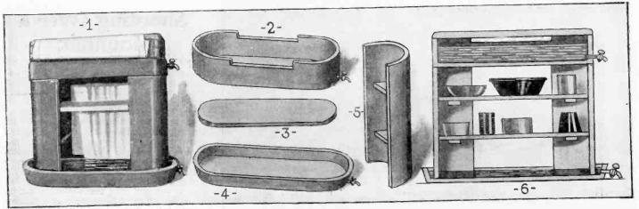
For use in warm climates and during the summer months in temperate zones, the iceless refrigerator illustrated above is handy and economical. 1 shows the completed assembly with the strip of cloth rolled up. 2, 3, 4 and 5 show the concrete castings to be made. Two ends such as illustrated at 5 are necessary. These parts are assembled as shown
