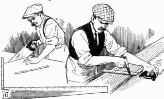
No. 1,514,180, issued to William A. Spitler protects the design of a saw, the back of which is scaled off as shown and carries a lug to which an arm may be attached at right-angles as a square.
