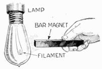
If a bar magnet is held near the filament of a carbon lamp, and D.C. is flowing through that filament, it will bend toward the magnet as shown. If the current is alternating, filament will vibrate.
