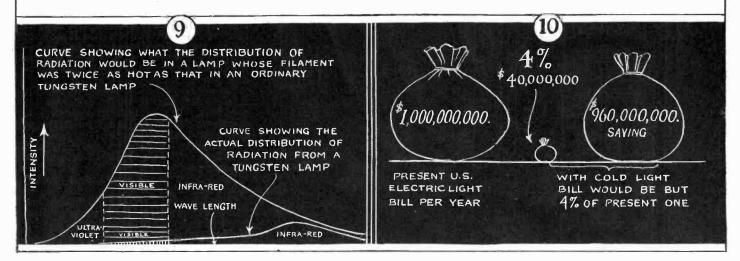
The maximum possible efficiency of any light depending on the heating of a filament is about 50%. The hotter the filament of a lamp, the greater its efficiency up to about 6,000° C., but no present substance will stand this temperature. The above chart shows how the efficiency of a lamp would be increased if the filament could be made twice as hot without burning out.
