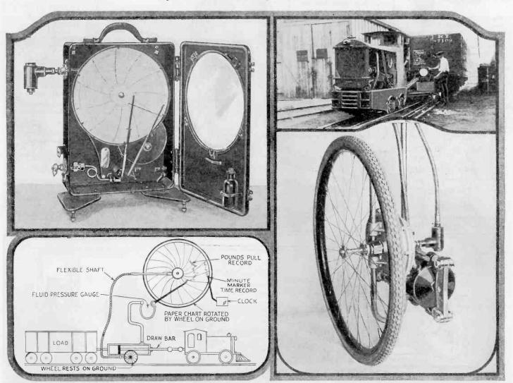
Our illustrations above deliniate the construction and use of a novel type of hydrostatic dynamcmeter. In use, the draw bar extending from the piston in the oil cylinder is attached to the device under test such as is shown in the illustration of the locomotive directly above. Any strain placed upon this draw bar registers on the fluid pressure gauge which in
