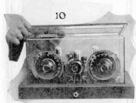
After assembling the receiver and putting the tubes in, place the cover on and the receiver is ready for operation. Dial indicators may be made by scratching the glass with a sharp file.
