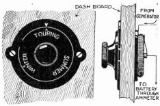
A regulator for automobile storage batteries, to prevent overcharging.
