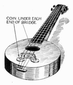
If two coins are placed under the bridge of a banjo ukelele in the positions shown in the illustration above, the tone given out by the instrument when played will be found to be of a far better quality than before the addition. Not only will the tone be richer, but if large coins such as half dollars are used, the chords will be much softer.—F. Cariveau.
