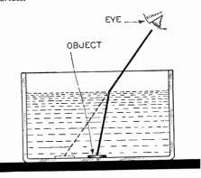
The above shows the effect of refraction of light through water.
