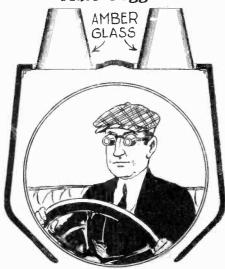
No. 1,511,357, issued to Eldridge Nairne covers the design of automobile goggles shown. By tilting the head, sun or approaching headlight glare can be eliminated.
