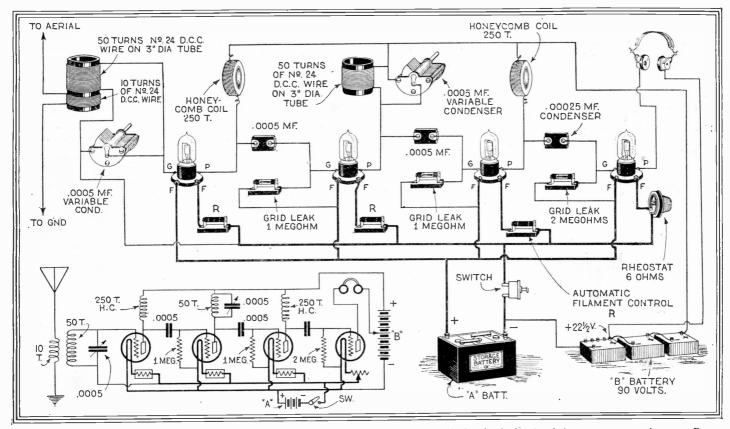
The above diagram shows what is called the T.A.T. system. It is used very much in England because it does not oscillate. The reason for this
