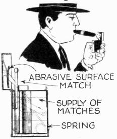
No. 1,513,091, issued to A. Y. S. Album protects match box design illustrated above. When the cover is released and opened by the spring, a match is forced up into the position shown and at the same time is lighted.
