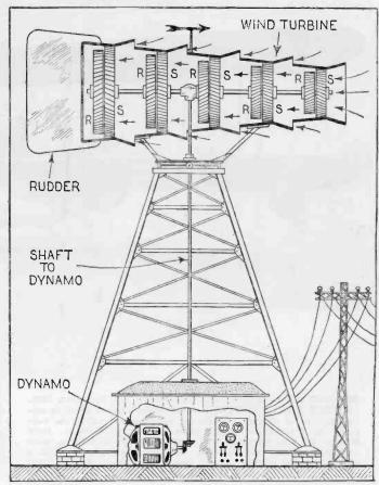
entrance and a stationary series of vanes against the first rotor. This it turns and then proceeds to the second rotor. Here it is reinforced by wind entering the second opening and is again concentrated on a rotor. The procedure is followed throughout. The rudder keeps the entire device facing the wind.
