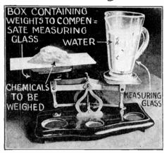
The experimental chemist whose supply of graduated weights is limited may use water instead. Place a graduate on one pan and a weighted box on the other to balance. Then each cubic centimeter of water in the graduate will balance one gram in the opposite pan.
