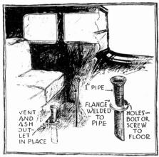
A combination ventilator and ash receptacle for the closed car may be quickly made from pipe fittings as shown above. A 1 inch or larger pipe is flared out at one end and a flange welded to it as shown. The lower end of the pipe is cut off at an angle. Mounted in the floor board as shown, this accessory is very handy as an ash tray and also serves as a ventilator.
