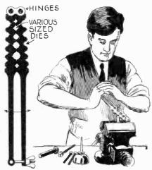
No. 1,521,647, issued to Edwin M. Perry describes the device illustrated above with which damaged threads on bolts and nuts may be quickly re-formed.
