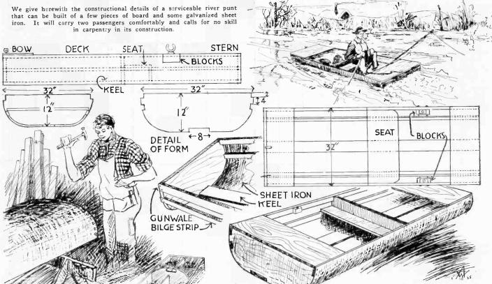
In the construction of this boat, first cut three forms from one inch cypress for the end and center blocks. Place two about ten feet apart with the third in the center, and fasten the keel in place with wood screws. Then fasten the gunwhale and bilge strips as shown, taking care that the surfaces of all the strips come flush with the edges of the forms. The outside covering of this boat consists of a single sheet of light gauge galvanized iron ten feet long and somewhat over four
