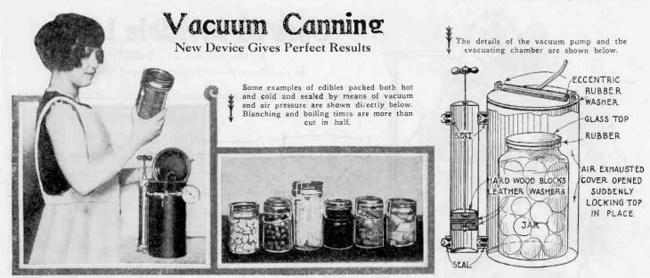
A new device of great assistance to the housewife has recently been invented by A. C. Whitefield and is illustrated in detail above. In use, the foods to be preserved are placed in a standard glass jar, the rubber ring and the glass cover put into position and the cover of the vacuum tank clamped on. A few strokes of the pump serves to create a vacuum of
