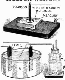
Place a block of moistened sodium hydroxide, in which a small cavity has been made, upon a carbon slab. Fill the cavity with mercury and insert a carbon rod in the position shown. Connect to an electric potential of about ten volts and a sodium amalgam will be formed in the cavity. By evaporating the mercury in a vacuum pure sodium will remain. The apparatus shown in the lower part of the pressilients of
