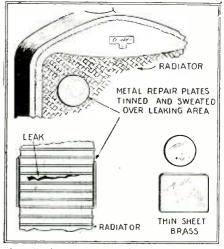
An effective way to repair a radiator leak. Monogram may be soldered over the patch.
