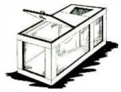
No. 1,578,061 issued to Jacques Abadie. This trap utilizes the knowledge that a roach prefers an opening only slightly larger than his body to one much larger. The bait is placed in a screened, covered box which is entered through a wedgeshaped passageway containing slots of various widths. The roach attracted by the bait, chooses the slot most suitable to its size, enters the box and is unable to find the way out.
