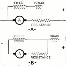
Q. 2109. Circuit diagram for dynamic braking system for electric motors.
