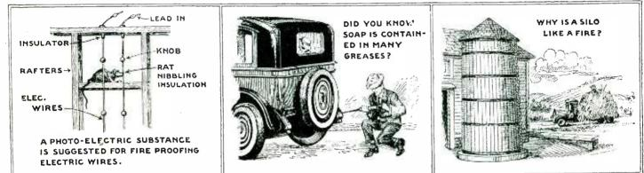
Selenium, used for coloring red glass and photo-electric cells, may be incorporated with wire insulation to make them fireproof.
