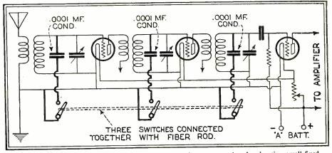
A method of increasing tuning range of radio frequency receiver by shunting small fixed Q. 503. condensers across secondary variable condensers of radio frequency stages.
