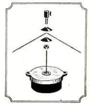
An exploded view of the most essential parts of the cone type loud speaker is shown in the above diagram.
