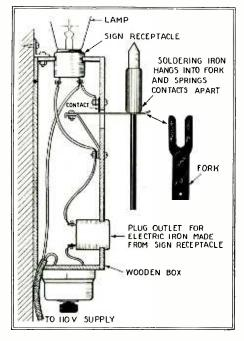
light will light up. If the iron is wanted in a hurry it is removed from the hook, cutting off the light, and laid on some noncombustible object on the bench. As the work progresses the iron is hung on the hook when not actually in use which automatically connects the lamp in series with it. Thus while not in actual use the current through the iron is reduced to such a value as to just keep it hot without overheating
