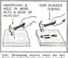
Left: Hammering mercury which has been frozen by carbon dioxide snow into a wooden board. Right: Rubber tubing is made so hard by the snow that it can be broken like glass.
