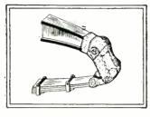
No. 1,574,898 issued to Jason A. H. Johnson. This invention relates to a cover for spring shackles on automobiles. It consists of a boot of leather or similar material, which is laced about the spring ends and shackle bolts and protects the moving parts of the spring assembly from the intrusion of injurious dust and grit. A cover applied in this fashion also functions to prevent the leakage of grease from the spring leaves.
