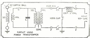
Here the Tesla coil is supposed to be supplied from the standard lighting circuit, using the power transformer described above. Again the grounded horn gap is used to protect the system. from one to two meters long will be found best with this particular coil. The wire should be thoroughly insulated at each end. In this manner the proper radiating system can be determined for radio use or for the coil only.
