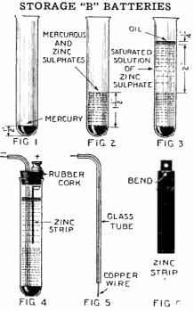
A storage "B" battery made according to the specifications shown will prove very serviceable, since frequent charging will not be necessary. The cells deliver  $1\frac{1}{2}$  volts each. When completed, the battery should be charged and discharged three times before being put into service. —Edward Geroux.
