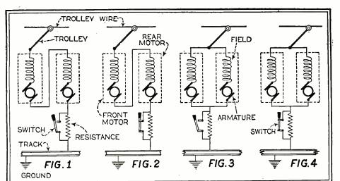
Q. 2112. The four drawings above show the connections made by trolley car controller to vary the current supplied to the motors
