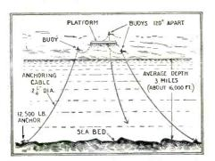
Method of anchoring seadrome, utilizing stranded steel cables 2<sup>1</sup>/<sub>4</sub> inches in diameter.
