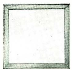
Fig. 8 .- Now glue the parts together with the square of plain veneer on the bottom, the piece of 3-ply panel in the middle, and the squared veneer on top, exerting all possible pressure with the Be sure not to try glueclamps. ing the taped side to the panel. Allow ample time for glue to thoroughly set, then scrape paper off and sandpaper.
