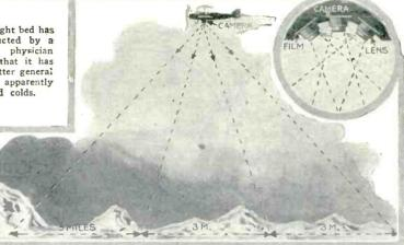
Three cameras of a new type have been assigned to the Alaskan Mapping Expedition for an extended aerial survey. From a height of 15,000 feet an area of 9 miles of territory may be mapped at one exposure.
