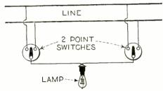
This method of connection permits Q. 2104. a light to be operated from two points
