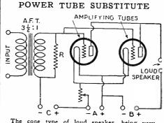
The cone type of loud speaker, being very sensitive to noises of all kinds, is operated most successfully in conjunction with nondistorting power tube amplifiers. Power tubes being more expensive than the ordinary ampli-fying tubes, two tubes of the latter variety may be connected in parallel, and thus deliver an undistorted output. —Frank d'Annunzio,
