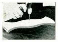
Three small holes are then drilled in the upper end piece to pass screws fastening it to the dowel sticks.
