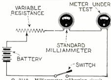
Q. 2110. Milliammeter calibrating circuit.
