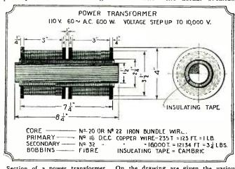
Section of a power transformer. On the drawing are given the various dimensions required, so that the reader will have no trouble in building the apparatus, which is designed for the standard A.C. circuit.
