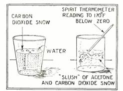
Left: Carbon dioxide snow floating on water. Right: Mixing acetone and carbon dioxide snow. This is so cold that you must use a spirit thermometer.
