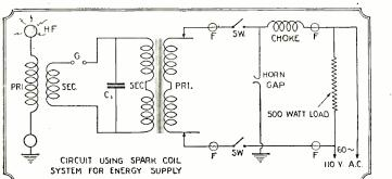
This is the layout of the circuit, using the spark coil system for the energy supplied. Note the protection afforded by the grounded horn gap.
