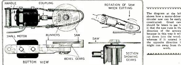
The diagram at the left shows how a motor-driven circular saw can be easily constructed. Great care should be taken to see to it that the saw runs in the direction of the arrows, because in this way it will cut down into the wood; whereas if it rotated in the opposite direction it might run away from the work.
