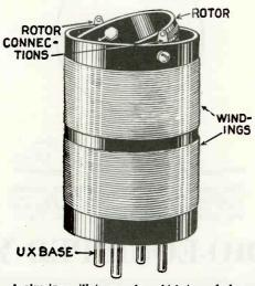
A plug-in oscillator coupler which is made by the same manufacturer is shown above. This also is equipped with a standard UX base.
