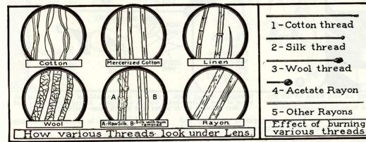
The above illustration shows how the various threads look when placed under the microscope. The effect of burning various threads and a litmus paper test of cloth are also illustrated.
