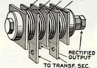
Above is a view of the dry rectifying element of the full-wave type.
