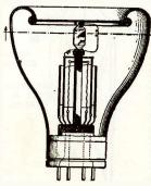
No. 1,636,921, issued to Alexander McLean Nicolson. The audion shown above, comprises an evacu-ated envelope in which are placed a grid, filament, plate and a plezo-electric crystal element.
