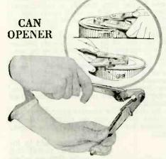
The device illustrated above and diagrammed in use is a can opener which will accommodate round or square cans. A pair of jaws on one side grip the ledge of the can. The cutter is inserted into the can and by merely opening and closing the apparatus, the cutter can be made to slice off the entire top and turn down any sharp edge which may be formed.
