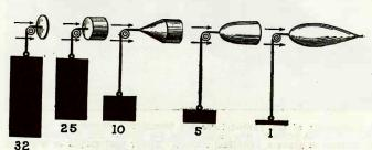
Fig. 3—Influence of the form of the body on the air resistance, which here for comparison is indicated by black weights. As we see, the resistance on the simple disc to the left, is about 32 times as great as that on the stream line Zeppelin model of the same cross-section.
