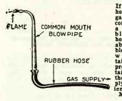
If a rubber hose from the gas supply is connected to a common blowpipe, a hot flame suithot flame suitable for all blowpipe work will be obtained. The pressure obtained from the gas supply is sufficient.—Donald Manwaring.
