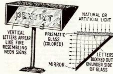
Here is an illuminated sign which announces the products it advertises both in the day-time and at night. The top is open so as to admit daylight which is reflected by the mirror through the sign. The prismatic glass enhances the brilliancy. At night electrical illumination is substituted for natural light.
