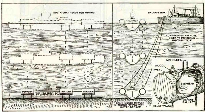
The above illustration shows how sunken submarines are now raised with pontoons by the U. S. Navy. This method was employed on the S-51 and was again used on the S-4. "Sub" hull was blown out by compressed air.
