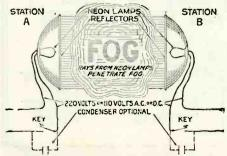
A night "blinker" set using neon lamps for signaling by dot and dash code.
