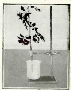
The rise of sap in plants can be clearly demonstrated by slipping a short piece of rubber tubing over the end of a young shoot and inserting a soda straw as shown above.
