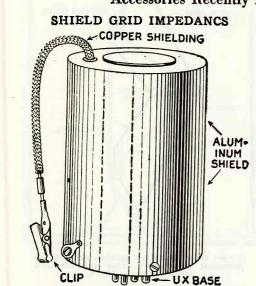
Above is a view of a new shield grid radio frequency impedance. Each unit is entirely enclosed in a metal shield and is fitted with a UX base.
