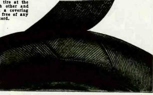
is further a great saving in the cost of construction which can, in turn, be put into the quality of the tire, by using machinery instead of manual labor for placing the cords. Between the two cord layers there is a layer of rubber which prevents the friction action here. When vulcanized, the whole becomes a homogeneous one-piece cord and rubber structure.
