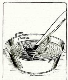
A loose hammer head, besides being an annoyance, is decidedly dangerous and should be repaired before it is used again. Such tools are generally repaired temporarily by hammering nails into the end of the handle; this method seems to be unsatisfactory in many cases. A very efficient, but little known method of tightening loose tool heads, is to soak the loose part in a pail of water overnight.—R. Wailes.
