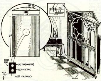
Above is a novel suggestion for making a cone speaker of exceptionally artistic and pleasing design. It measures 3 feet by 5 feet and is built with balsa wood or ply wood. The front is covered with a grill work and the cone is supported at each end, as shown. The cone is depicted at 1 and the unit at 2.
