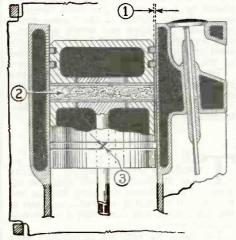
Above 1 shows .002-inch piston clearance; 2, wrist pin hole filled with graphite and oil; and 3, a clearance of .01 inch at joints of piston rings.
