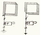
No. 1,639,913, issued to Roy A. Weagant. This aerial comprises two collecting portions which form a single antenna, one is an open loop, and the other a vertical antenna connected to the mid tap of the loop. The radio circuits are coupled to the vertical antenna. Two forms are shown above.
