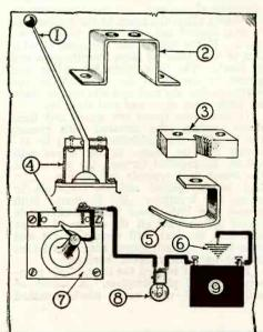
Above, 1, shift lever; 2, bracket; 3, insulation; 4, switch; 5, contact finger; 6, ground; 7, indicates a plan view; 8, the rear light; and 9, battery.
