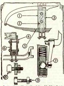
In the above illustration 1 is a blocking for a broken spring, 2, 3, 4 and 6 are boards, 5 is the broken spring, 7, broken drag link ball, and 8 a substitute for the broken ball made from 9.
