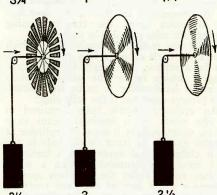
Fig. 5—The amount of wind pressure exerted on motionless (above) and moving (below) wind-wheels are indicated by black weights; left: wind-turbine; center: wind-mill; right: Venti-motor.
