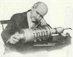
An airplane motor which weighs but fifty pounds is shown above. With the exception of the ball bearings and adjusting screws, the motor has but four major parts and has no valves or springs. The single cylinder acts as a cam to separate the intake and exhaust. The inventor, Edwin L. Rice, claims that the motor is equivalent in horse power to a 450 pound motor. The motor is capable of making 200 miles per hour.
