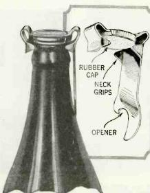
This spring steel bottle closer produces a perfect seal for crown cap bottles. There are two grips on either half which settle in the groove beneath the mouth of the bottle. A rubber disk serves as the stopper. To release, merely lift up on the depending blade, which also serves as a bottle opener.
