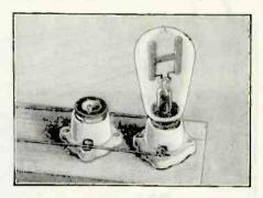
When the fuse shown here blows, the neon lamp lights, indicating the fact.
