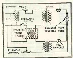
The above diagram shows a method of con-trolling X-ray tube-filament voltage by using a booster transformer having a 1:1 ratio. This transformer has a low resistance winding in both circuits.
