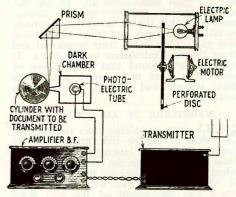
above illustration snows clearly the ar-ement of the apparatus and how it is coupled to the radio transmitter.
