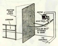
The automatic closing of a door can be accomplished easily by employing the method shown above. A circular rack attached to the door is moved by means of a gear train, actuated by an electric motor.—Je Sais Tout.
