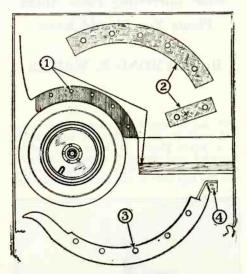
Above, 1 indicates holes to be marked on tem-plate, 2 indicates template, and 3 and 4 show holes drilled in new fender.
