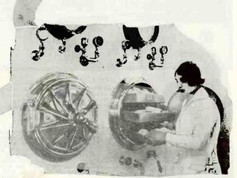
New cabinets for the sterilization of dental and surgical instruments employ super-heated steam. The above is installed at the New York University College of Dentistry, and is demonstrated by Miss Kathryn Blond.
