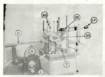
In the above photo B is the paper band for recording, R is a water reservoir, L the lamp which deposits lamp black on the paper strip, T is a drum over which the paper passes, RD is a regulator for the unrolling of the paper, SE is a stylus for registering the movements of the tuning fork, CP is the stylus counter-balance, and SS is the stylus for registering the seconds.
