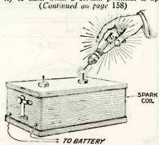
The characteristic glow of neon gas can be shown by touching one terminal of a neon lamp to a spark coil high voltage terminal.
