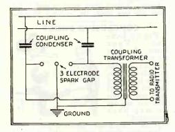
Above is the hook-up of a wired wireless system, showing how the transmitter is coupled to the line.
