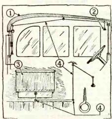
Above, 1 indicates sectional view of car, 2, knob; 3, curtain; 4, screw eyes, and linen or silk fishline.
