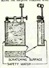
Photograph on the right Photograph on the right shows the phoney invention cigarette lighter and at the left are the details of its construction. Note that the wick has been removed and a safety match substituted therefor. A scratching surface is shellacked to the bottom of the box. This can be obtained from an ordinary match box.
