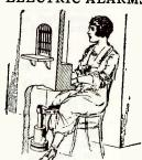
No. 1, 657,459, issued to Frank Davis. This alarm system has an alarm circuit which is closed by a specially designed circuit closer. The circuit closer is worn on the leg and is operated by the other leg. A floor cord connecting the circuit closer with the alarm circuit, permits a limited amount of
