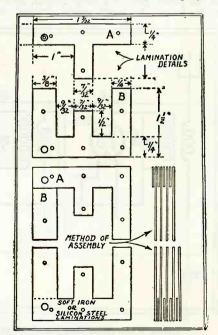
Lamination details and the method of assembly are given above. Either soft iron or silicon steel may be used. Fig. 3.
