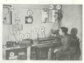
The above photograph shows the installation. PS is a synchronized pendulum, MA is a milliammeter, V a voltmeter indicating the voltage passing through the photo-electric cell, R is a relay, A shows a bank of three amplifying tubes, P shows the potentiometers, PL the free pendulum, and EP the photo-electric equipment.
