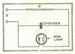
The above diagram shows how a neon lamp may be employed for measuring the capacity of condensers.
