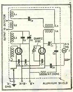
An audio frequency oscillator with quartz crystal control is shown above. A straight frequency line condenser is used for changing the frequency within the audible range.
