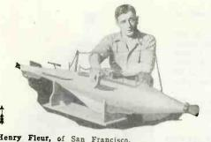
Henry Fleur, of San Francisco, recently demonstrated his model submarine which works entirely without propellers. The model which is shown above sucks in water through the bow and expels it under terrific pressure from the stern. The release of this water carries the craft forward and it makes 35 knots an hour below the surface and 55 knots an hour on the surface. According to the inventor, the model marks a new trend in marine navigation. The stabilizing fins on the propellerless
