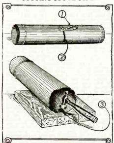
The stove pipe may be cut with an ordinary can opener, as shown in the upper illustration. The resulting ragged edge can be smoothed out with a hammer and a block of wood, as shown. Tin snips are awkward to use in contrast to this use of the can opener. G. H. Luers.
