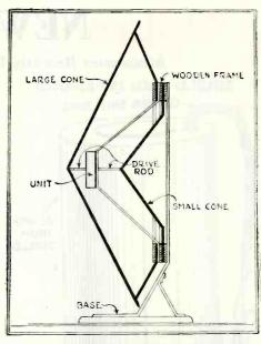
A view of the completed speaker, showing the placement of the two cones and the unit appears above. Fig. 6.
