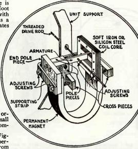
view of the unit showing the method of sembly appears above. Note the position of e drive rod which is used to actuate both the large and small cones. Fig. 1.
