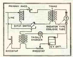
twelve-volt storage battery with an auto-atic switch and relay and trickle charger, n also be used with the tube, as shown love. In this way the filament voltage is kept constant at all times. A two
