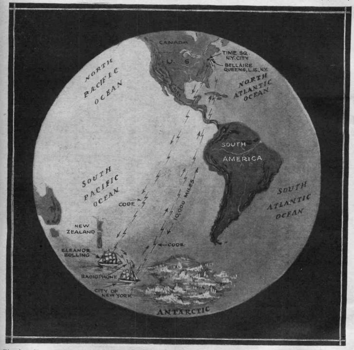
The above illustration shows how the operator at Times Square called Bellaire, Queens, by way of the Antarctic. The Byrd expedition, now about 10,000 miles away, acted the part of central. The message from Times Square was sent in code to the "Eleanor Bolling" and was relayed by radiophone to the "City of New York."
