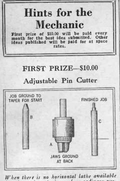
When there is no horizontal lathe available for pin cutting, the jaws of an ordinary ver-tical or press drill can be ground to a rake which converts it into an adjustable cutter. It is advisable to grind a taper on the end to cut B for the purpose of a good start. A shows the jaws ground at the back and C the finished job. The job can be held in a drill vise or disused lathe chuck. —R. Brown.
