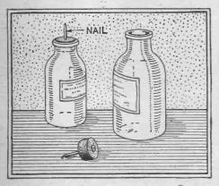
By pushing a nail through a bottle cork, so that the head is at the bottom, as shown, a good handle is provided and the cork never need be pushed into the bottle, which often happens, particularly when the bottle has a wide mouth or a flat cork is used.— B. Hoopes.
