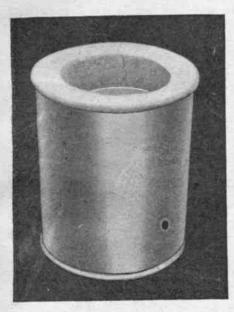
The furnace itself is shown above. The edge of the crucible may be seen just below the rim of the shell.
