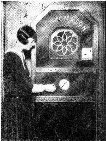
At the left is a photograph of the front view of the Radiomaton receiver, which is the main receiver of the coin-in-the-slot system. The receiving set is capable of operating 300 pairs of headphones simultaneously.
