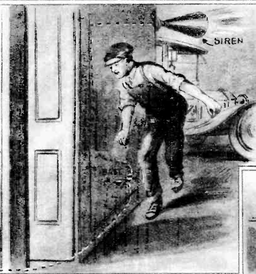
A device which will stop an automobile almost instantly has been perfected by a New Jersey inventor. It stops the vehicle by dropping under the rear wheels a shoe fitted with a cork pad to prevent skidding. The shoes are fastened on rocker arms and fit under the wheels.
