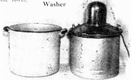
A small portable pneumatic washing machine is shown in the above photograph. The illustration at the left shows the operating principle. An electric motor at the top drives a fan, which produces a partial vacuum, pulling the air in from the sides to the bottom and up through the water. The arrows show the pathway of the air.
