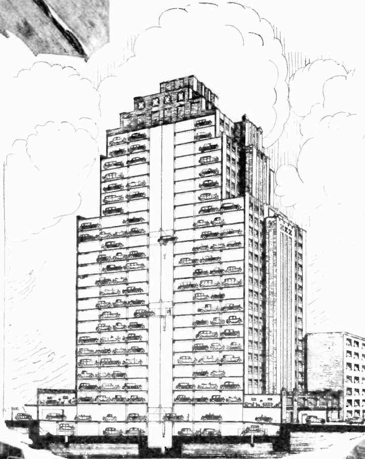
Above: The layout of the thousand-car garage. Below: How the system operates. The motorist stops his car at the elevator. The elevator man sends out the parker, which tows the car on the elevator and pulls it out on the floor allotted to it. See story for further details.
