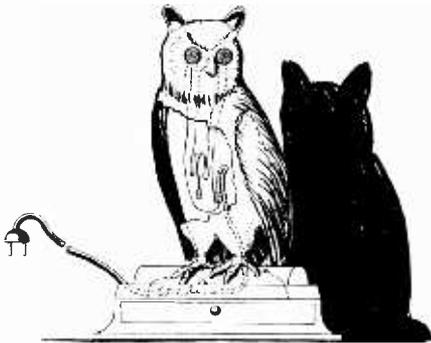
No. 1,727,002, issued to William B. Weaver. This lighter is a novelty using the form of an owl to contain coils which are heated to incandescence. The eyes of the owl contain the coils which are heated to incandescence; the base of the figure is equipped with an off-and-on switch. When the eyes light up they give the impression of an owl blinking.
