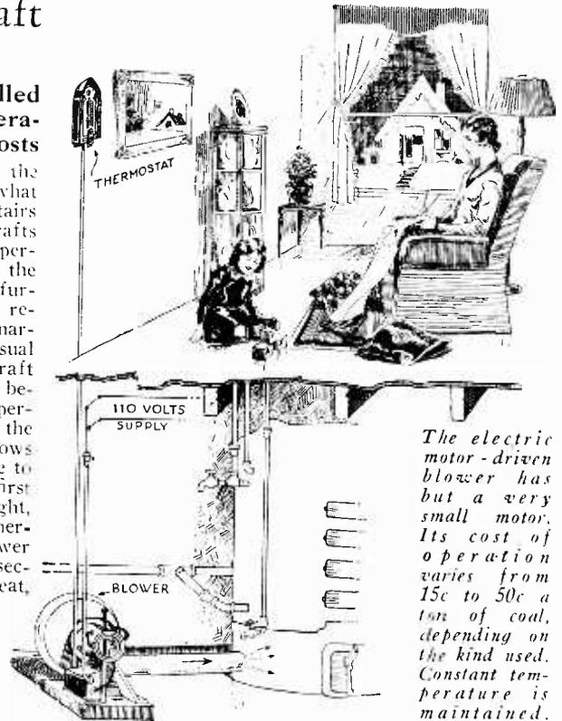
The electric motor-driven blower has but a very small motor. Its cost of operation varies from 15c to 50c a ton of coal, depending on the kind used. Constant temperature is maintained.
