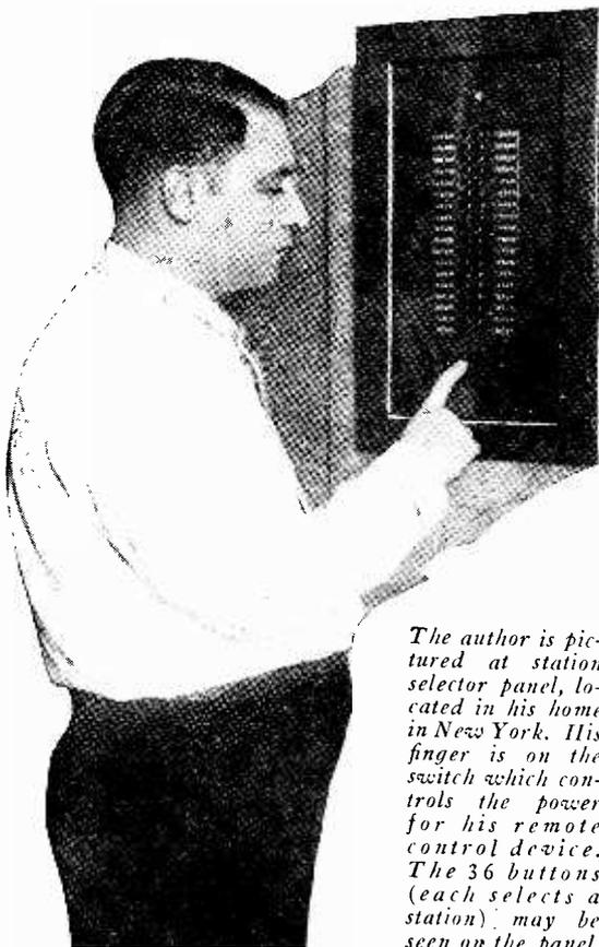
The author is pictured at station selector panel, located in his home in New York. His finger is on the switch which controls the power for his remote control device. The 36 buttons (each selects a station) may be seen on the panel.
