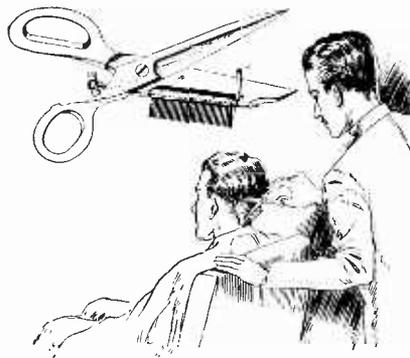
No. 1,726,390, issued to John W. Erhard and Antoinette Erhard. This patent relates to a device for combing and cutting the hair and also a means of gauging the length of the hair cut off. It consists of a pair of scissors, two shear members pivotally connected, a rod with a comb on it and a rack and pinion for rotating the comb upon opening and closing the scissors.
