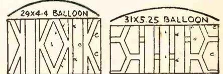
The movements of the tread are different for the center, intermediate and outer portions, thus causing the curves on the straight part of the pattern.
