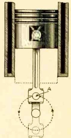
Section of a typical cylinder is shown. The dotted lines indicate the position which the piston assumes at the bottom of its stroke.
