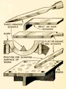
Fig. 4—After you have milled or shaped flat and curved surfaces, true them with a scraper.
