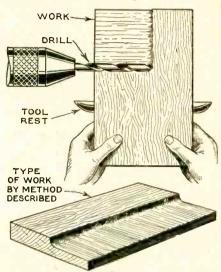
PERHAPS you do not use a planer or gouge often, so have not purchased them. Or perhaps they break in the middle of an operation. You may not realize it, but your drill is a good sub-stitute for these tools. Merely support the work upon the tool rest of a woodturning lathe, and allow the portion to be shaped or gouged to come in contact with the point of the drill. While the work will not be as perfect as with the correct tool, it will serve the purpose .---R. Wailes.
