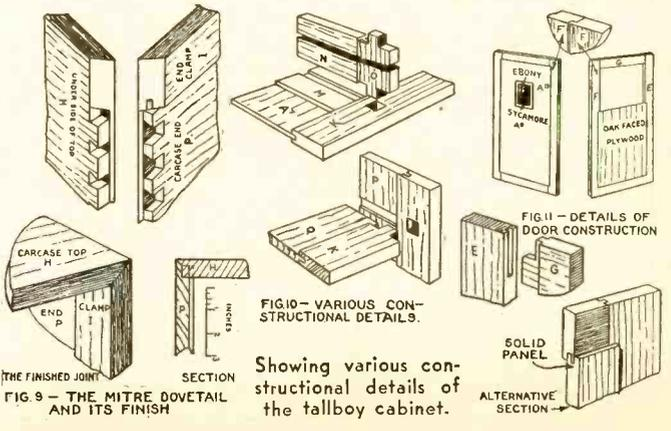
FIG. 9 - THE MITRE DOVETAIL AND ITS FINISH FIG. 10 - VARIOUS CONSTRUCTIONAL DETAILS. FIG. 11 - DETAILS OF DOOR CONSTRUCTION. Showing various constructional details of the tallboy cabinet.
