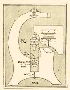
Fig. 2:-Details of bearings and method of oiling.
