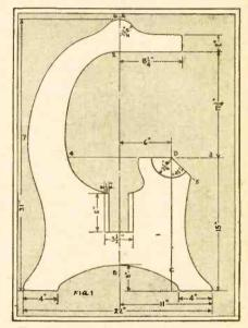
Fig. I:-Outline of the frame, showing measurements
