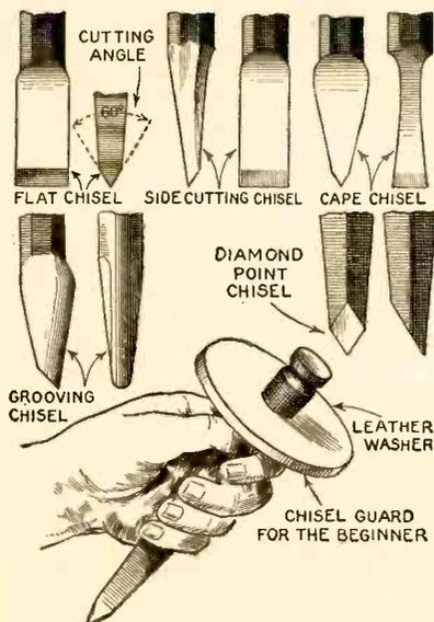
Fig. 3—The five general types of chisels. All should be adjusted to a 60° cutting angle for work.
