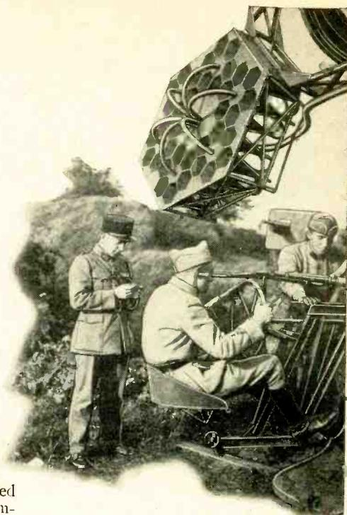
A French officer supervising the observations being made with the aircraft detector unit shown at the bottom of this page.
