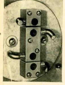
A close-up of the carbon holder unit. Note how the thumb screws are staggered. The round head bolt fitted with the washer is the three-inch bolt that holds the various units together.
