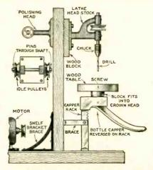
pins thrust through holes drilled through the shaft. Stock pulleys are used. The drill head is a lathe headstock, or, if desired, a polishing head, with one end of its shaft threaded to take the chuck.
