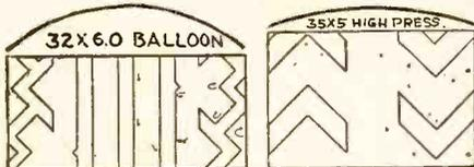
Drawings taken from wax records showing tread movements. A V-shaped mark on a wax plate is a common record from this part of the tread.
