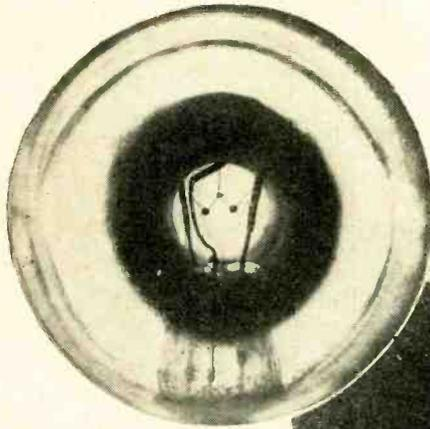
Looking at a thermocouple (much enlarged). Note the two metal discs and the thin wires upon which heat rays are focused.
