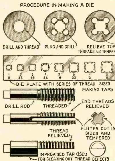
Fig. 2—As the usual taps and dies can not be used for special sizes of screws, these directions will help to make whatever additional ones you need.
