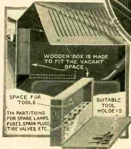
Installing a modified parking light over the front left-hand window. To the left—a wooden tool box can be put in the unused space under the hood.
