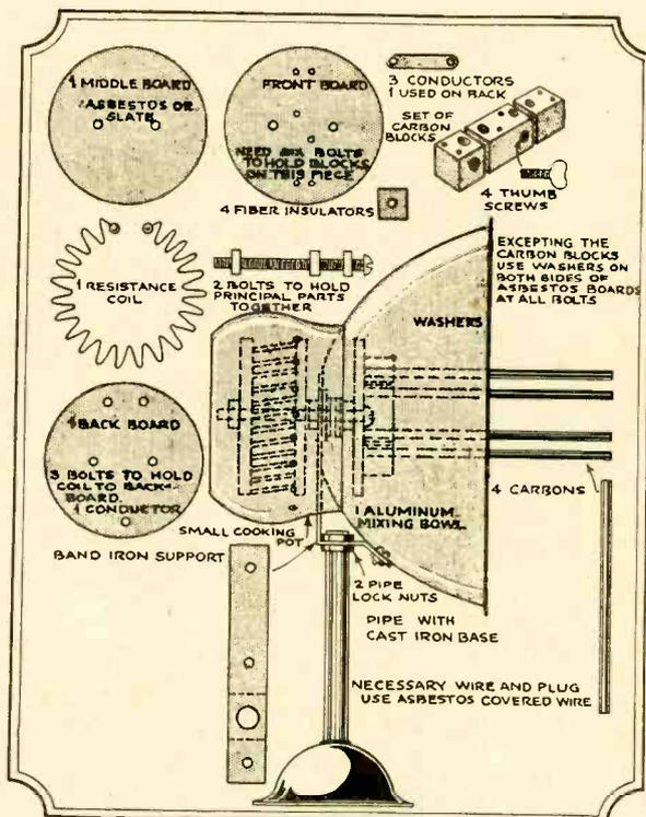
Working plan of the assembled lamp; details of the resistance coil, a set of carbon blocks, and the front, middle, and back boards are also shown.
