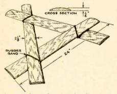
A correctly made triangular boomerang. Note the placement of the three arms.
