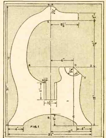
Fig. 1:—Outline of the frame, showing measurements.
