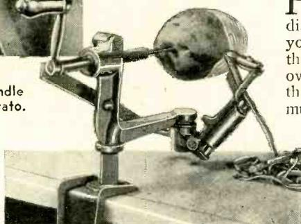
chine is so adjusted that it will cut the same fine wafer-like strip from the entire surface, regardless of how irregularly shaped it may be. The device can also be used for making finely cut garnishes for salads, to cut carrot, beet and apple strings for decorations, and to peel turnips and other vegetables that are not very soft.
