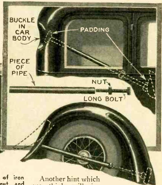
A piece of iron pipe, a nut, and a long bolt, are the requisites for making this efficient buckle eliminating tool.
