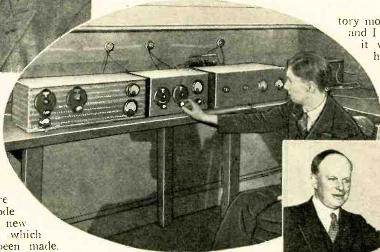
A laboratory model of the Stenode at the London Headquarters of the British Radiostat Corporation.
