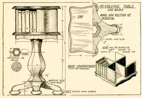
These detailed drawings give all the necessary constructional data. The exact measurements will have to be altered to suit different piano stools which individual readers may have around the place and decide to convert.
