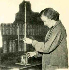
An excess of alkali added to an acid which contains a drop of methyl orange changes the color of the solution from pink to yellow. Left—In the preparation of fluorescein, anhydrous zinc chloride is added to resorcinol and phthalic anhydride, after fusion over an oil bath.
