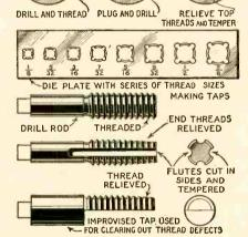
Fig. 2—As the usual taps and dies can not be used for special sizes of screws, these directions will help to make whatever additional ones you need.
