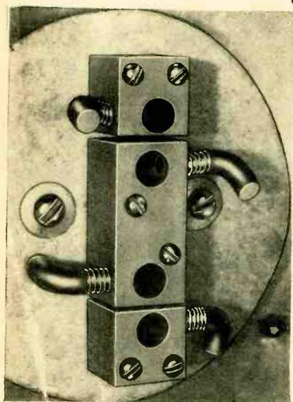
A close-up of the carbon holder unit. Note how the thumb screws are staggered. The round head bolt fitted with the washer is the three-inch bolt that holds the various units together.
