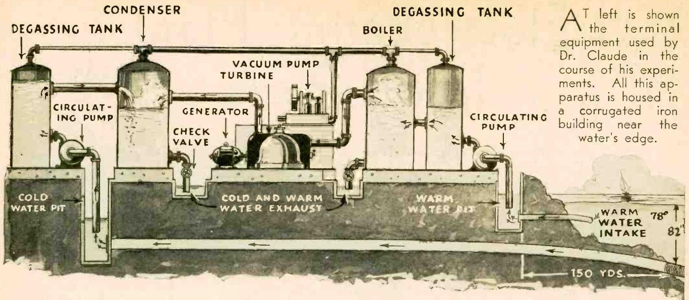
At left is shown the terminal equipment used by Dr. Claude in the course of his experiments. All this apparatus is housed in a corrugated iron building near the water's edge.
