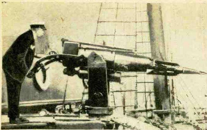
A harpoon gun, loaded with a modern harpoon with fluke-expanding bomb in the tip. The range is 40 to 60 yards.
