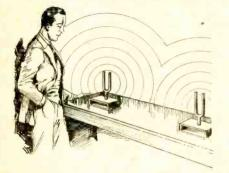
MOUNT two similar tuning forks on suitable resonance boxes and place them a few feet apart. If one of the tuning forks is set vibrating for a moment and then stopped it will be noticed that the other fork is vibrating. Does the second fork receive its energy principally from the sound waves that strike the prongs of the fork or from the waves which enter the resonance box?
