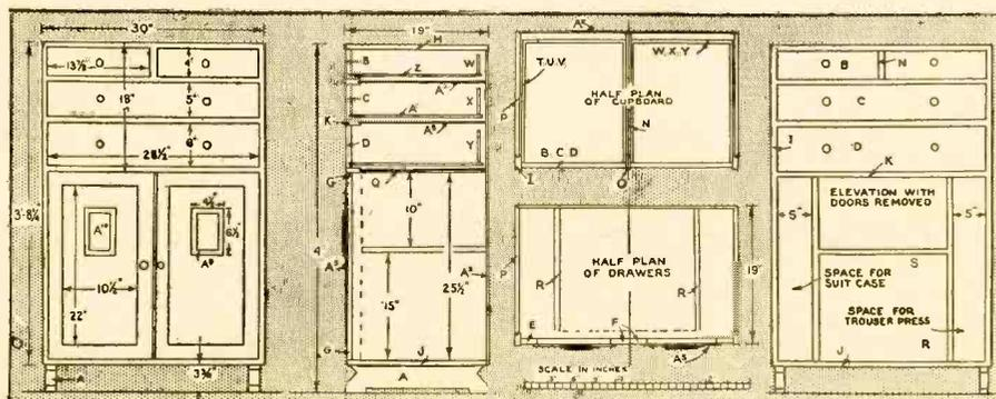
Fig. 7—Elevations of tallboy cabinet with doors closed (left) and open (right), sections and plans in centre.
