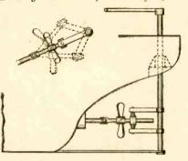
propeller of a ship, but also as a de-pendable, efficient and easily controlled steering device which completely eliminates the rudder. The propeller is not mounted directly upon the propeller shaft. A universal joint is provided at the end of the main shaft. The other end of the universal joint is fitted to the auxiliary shaft to which the propeller is secured.
