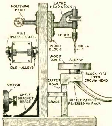
pins thrust through holes drilled through the shaft. Stock pulleys are used. The drill head is a lathe headstock, or, if desired, a polishing head, with one end
