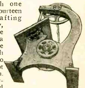
View showing underside of saw table.
