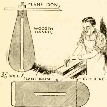
take the blade and cut the top portion off straight (or you can leave it as it is). Then get an old handle, drill or burn a hole through it at least large enough to hold a 3/16" bolt. Put the blade on, the bolt through the handle, and tighten the nut.—*F. M. Edwards.*
