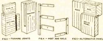
Various constructional details of the bedstead, showing how joints are made.
