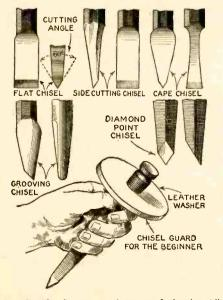
Fig. 3—The five general types of chisels. All should be adjusted to a 60° cutting angle for work.
