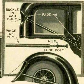
piece of iron pipe, a nut, and a long bolt, are the requisites for making this efficient buckle eliminating tool.
