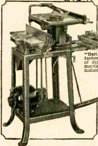
"Delta" Boring and Routing Attachment, makes child's play out of difficult boring, routing, and mortising. Easy to operate. Furnished separately if desired.
