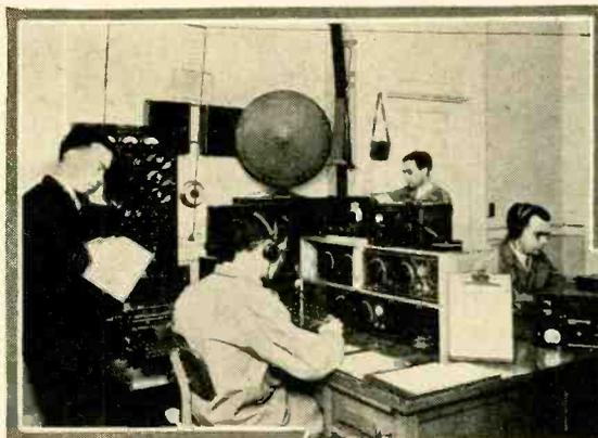
The main operating desk at Station WIXV controls six receiving sets for waves ranging from ten to 7,000 meters and four transmitters operating on ten, twenty, forty and eighty meters. . . .
