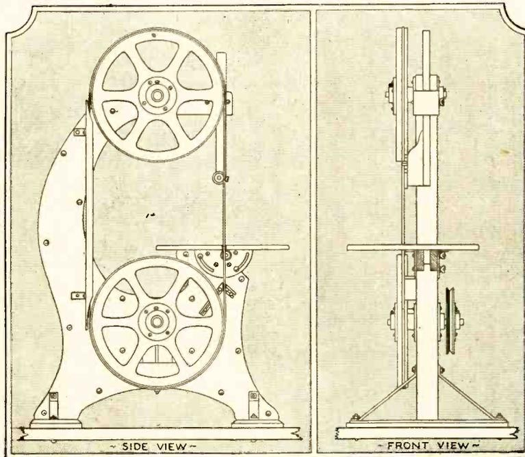
Fig. 3.—Side and front elevations of the completed saw, showing how the various parts are fitted together.
