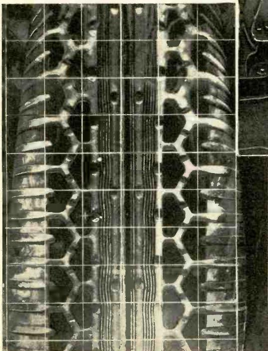
Photograph taken through the plate glass, showing contact area of a tire under load. The depressions in the tread are painted to show contrast.
