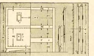
Fig. 2—Scale elevations and sections of head and foot ends of bedstead. Plan given at right.
