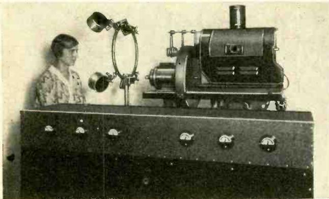
Light-spot transmitter built by Fernseh, A.G., for the German Post Office. Note the extensive photoelectric cell amplifier in the foreground.
