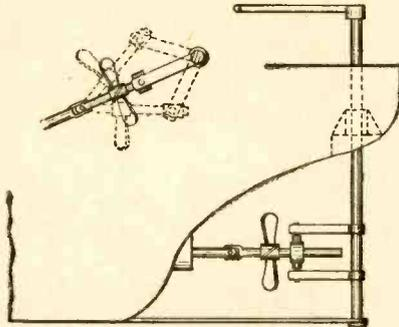
propeller of a ship, but also as a dependable, efficient and easily controlled steering device which completely eliminates the rudder. The propeller is not mounted directly upon the propeller shaft. A universal joint is provided at the end of the main shaft. The other end of the universal joint is fitted to the auxiliary shaft to which the propeller is secured.
