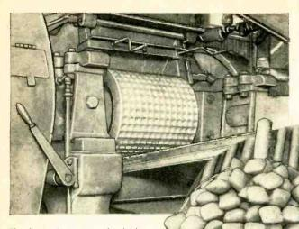
The first pile contains finished anthracite briquettes; other, raw bituminous coal.
