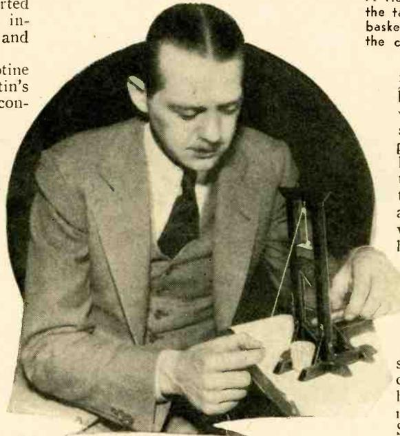
The guillotine in operation as a cigar cutter. The cigar is held on the table, the knife pulled up to the top, and released. In falling, it snicks off the end of the cigar.
