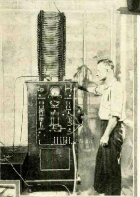
To generate electricity, this three kilowatt 250,000 volt outfit is used. From it, two feeders carry the current along the sides of the orchard; it is distributed over the trees from a network of wires.
