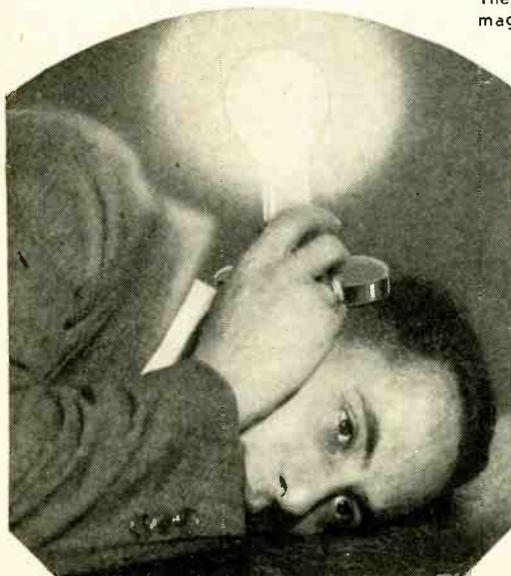
The coil to which the lamp is connected forms the secondary winding of a transformer. The primary coil is the magnet located in the table.
