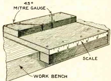
bench top. In addition, it can function as a mitre box. If it has no scale in front, paste or engrave one there. Then equip it with a left and a right 45-degree slot on the back cross member.—*R. Wailes.*
