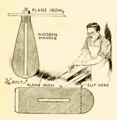
take the blade and cut the top portion off straight (or you can leave it as it is). Then get an old handle, drill or burn a hole through it at least large enough to hold a 3/16'' bolt. Put the blade on, the bolt through the handle, and tighten the nut.-F. M. Edwards.
