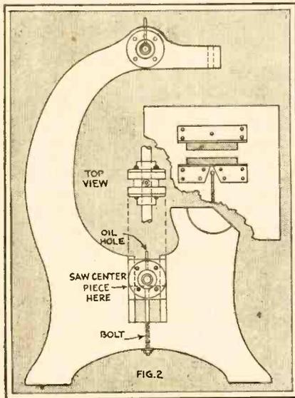
Fig. 2.—Details of bearings and method of oiling.
