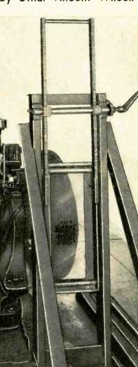
Above — Apparatus designed by the Government scientists for the study of tire tread wear. Below — Another wax record drawing. The arc above each section shows the profile of the raised portion of the tread.
