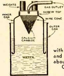
The handy worker can make this efficient automatic acetylene generator by fitting two discarded milk cans with some of the odds and ends usually found about the workshop. Cost is negligible.
