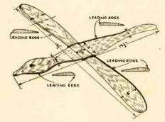
The cross boomerang, shaped like a bird. forefinger, with the curved side inwards. Always move the arm straight from the shoulder, but you can toss in any direction between the hours of twelve and six o'clock through three o'clock.
