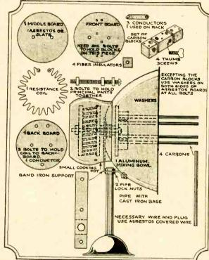
Working plan of the assembled lamp; details of the resistance coil, a set of carbon blocks, and the front, middle, and back boards are also shown.
