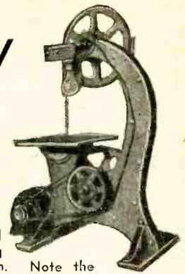
The finished band saw, with driving motor in position. Note the lamp to illuminate the table.
