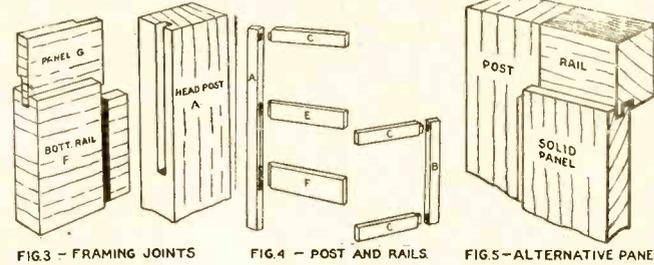
FIG. 3 - FRAMING JOINTS FIG. 4 - POST AND RAILS FIG. 5 - ALTERNATIVE PANEL
