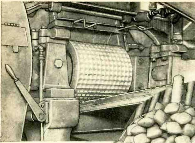
Briquetting press. The revolving drums mould the finished product after it has been mixed with asphalt.
