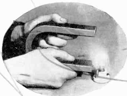
If a magnet is held near a lighted filament and vibrations of the filament can be observed, alternating current is flowing through the circuit.
