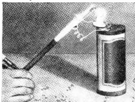
Heating a wire increases its resistance.
