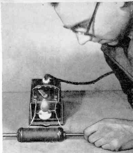
The alternating current flow to a device such as a lamp can be cut down if an iron rod is inserted into a hollow core coil included in the circuit.
