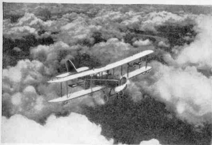
Above the clouds on an insect hunt. Only the light, small bodied, wind-borne insects are found in this region. A streamlined trap is mounted on each wing of the airplane to equalize head resistance.
