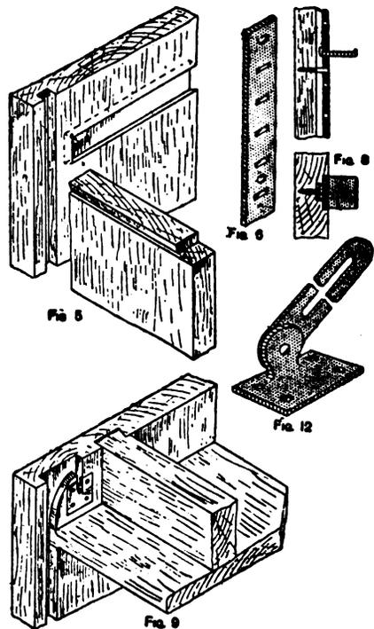
parts of cast brass,  $\frac{1}{8}$  in. thick. The stop and guide (Fig. 13) is a brass plate with a packing or shoulder piece soldered to it, and a hole bored through the centre to take a strong round-headed brass screw, which secures and forms a guide for the slotted suspender (Fig. 12).
