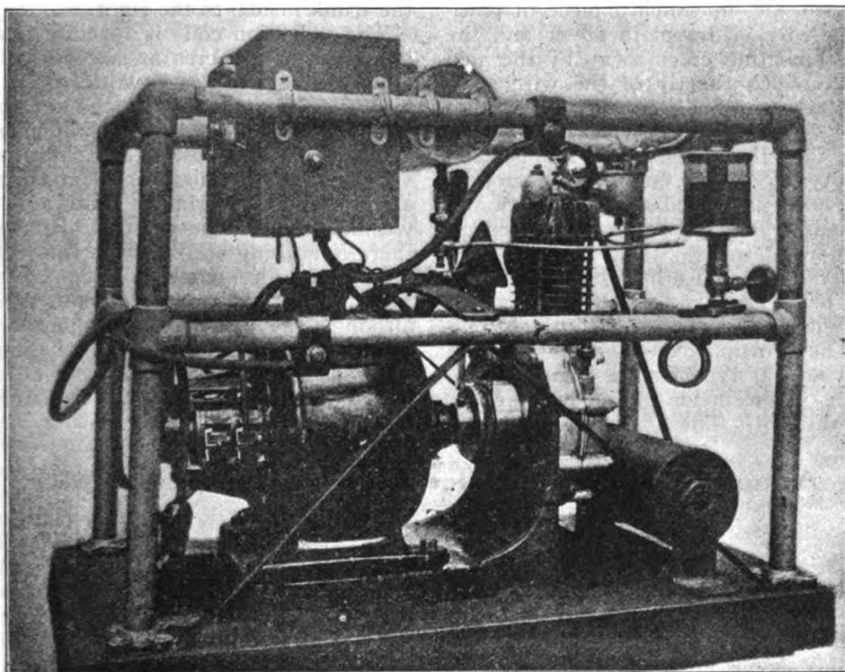
Portable Gasoline Engine and Generator for Field Wireless Telegraph
