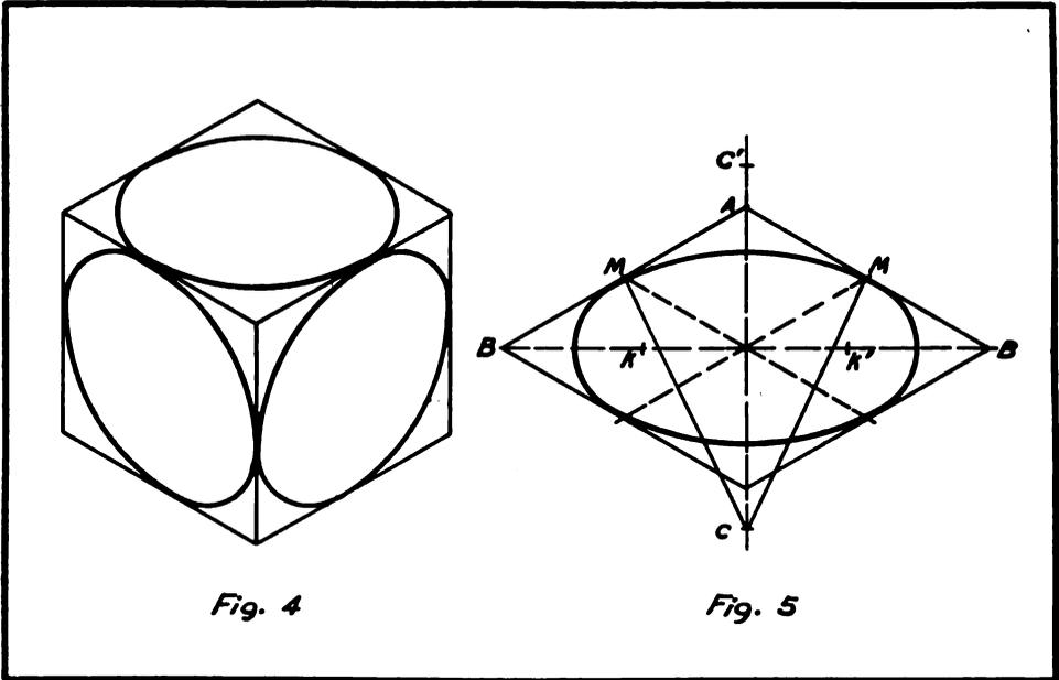
Right angles in the object are usually either 60 degrees or 120 degrees in the drawing. See Fig. 2.
