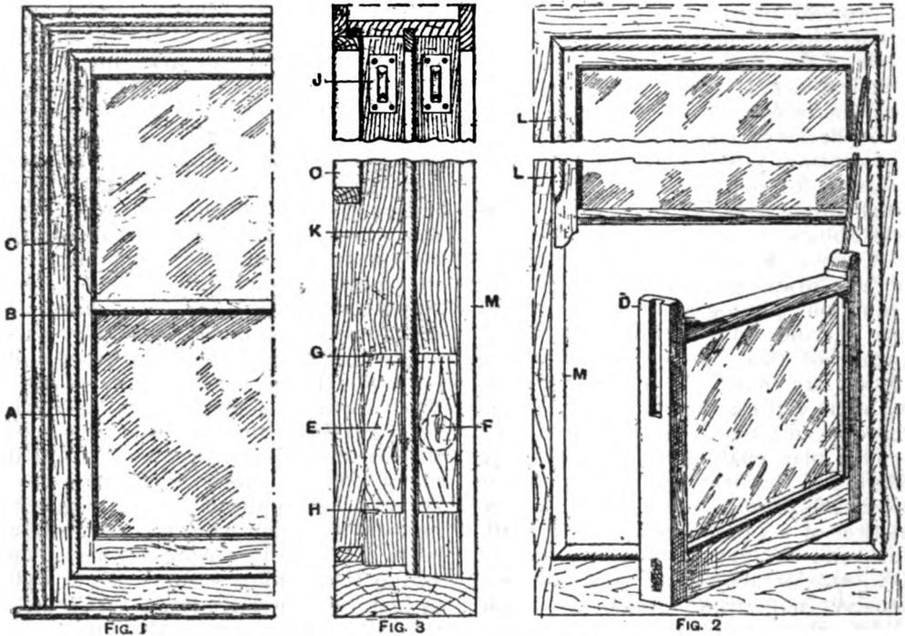
Replacing a Broken Window Cord
