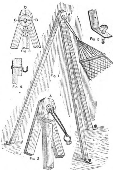
Support for Fixing Hammock in Room. Fig. 1.—View of Tripod Supporting One End of Net. Fig. 2.—Head of Tripod. Fig. 3.—Back of Head of Tripod. Fig. 4.—Vertical Section at C (Fig. 3) showing Shank of Hook Riveted to Back Plate. Fig. 5.—Bracket Iron and Thumbscrew.
