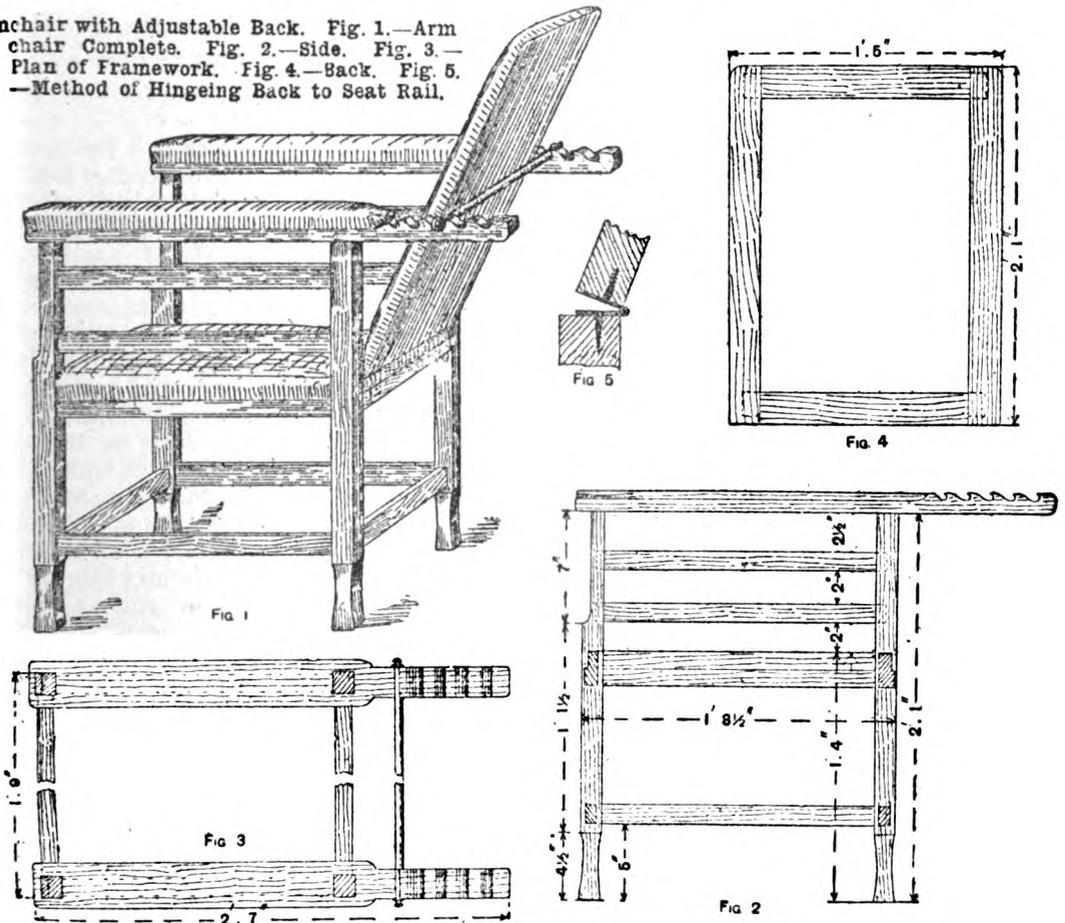
should have a shallow rebate to take the edge of the stuffing, showing  $\frac{3}{4}$  in. on the bottom edge. The legs are mortised through the arms and wedged.
