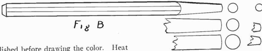
be polished before drawing the color. Heat the end of the punch, for about 1 inch from the end, to a nice cherry red, then plunge quickly into the oil. Be sure to carry it deep enough to cover the whole punch. When cool, the oil may be removed with a
