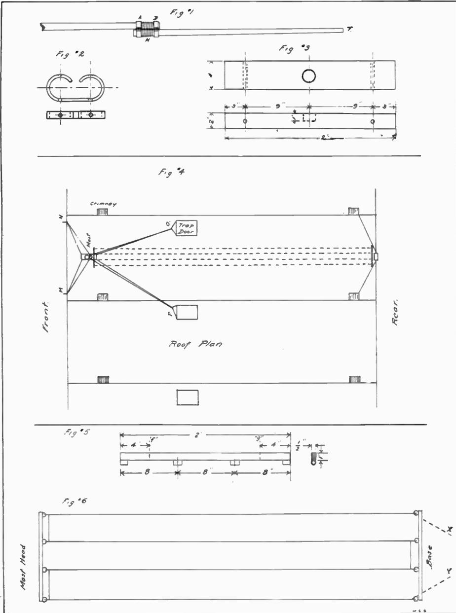
The mast having been erected, we will now turn our attention to the antenna. Get two pieces of well seasoned wood about 1 x 1/2 inch, and each 2 feet long. Fasten porcelain insulators to them, as shown in Fig. 5. These knobs can be tied to the wood with short pieces of wire running around groove on surface. The wood should then be given several coats of good paint.
