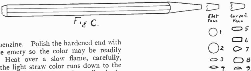
little benzine. Polish the hardened end with a little emery so the color may be readily seen. Heat over a slow flame, carefully, until the light straw color runs down to the end, then plunge again into the cooling bath. Care must be taken not to draw the temper too far, because if too soft the working end will soon batter out of shape. If too hard, it will break off.
