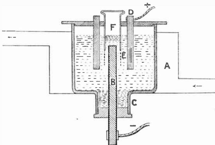
Fig. 132. Castner's Electrolytic Method of Producing Metallic Sodium
