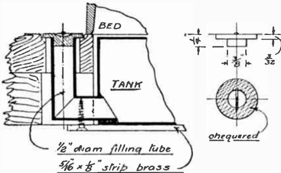
FIG. 57.—FILLING TUBE AND STOPPER FOR WATER-TANK. (Half full size.)
