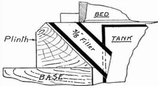
FIG. 58.—ALTERNATIVE DESIGN FOR FILLER, WHERE PLINTH BOARD IS USED. (Half full size.)
