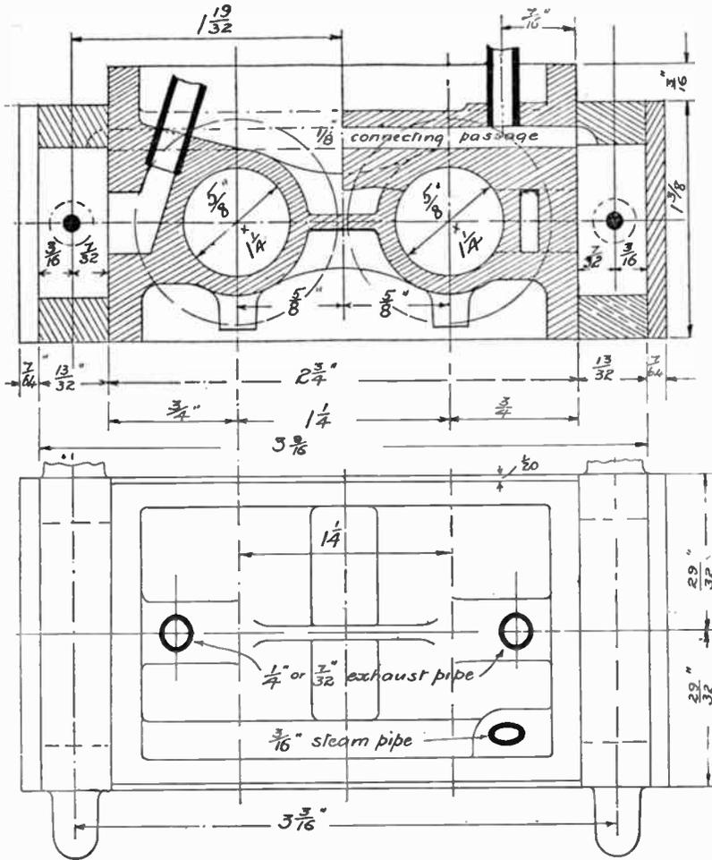
FIG 53.—CROSS-SECTION AND PLAN OF ALTERNATIVE TWIN HIGH-PRESSURE CYLINDERS FOR SMALL MODEL UNDERTYPE ENGINE.
