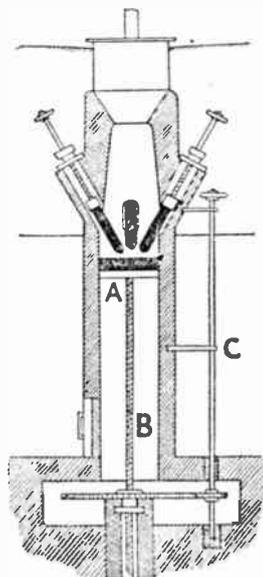
Fig. 130. Calcium Carbide Furnace for Operating with Three-phase Alternating Currents
