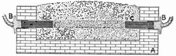
Fig. 131. Furnace for Producing Carborundum
