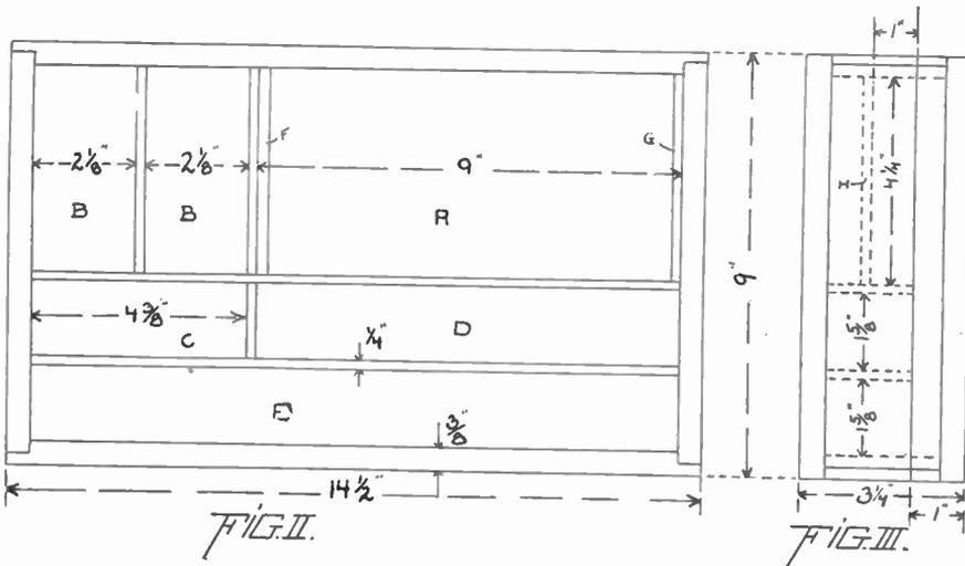
any special instruments outside of the case may be kept. As to the remaining spaces: B, B are for the reception of bottles of ink; C is for erasers, thumb tacks, etc.; D is for pencils, penholders, and brushes; and E is for scales. On the underside of the cover triangles may be fastened by means of small blocks of wood, screw-hooks, or screw-eyes.
