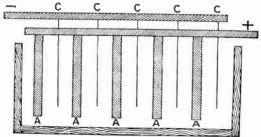
Fig. 126. Arrangement of Plates for Electrolytically Refining Copper
