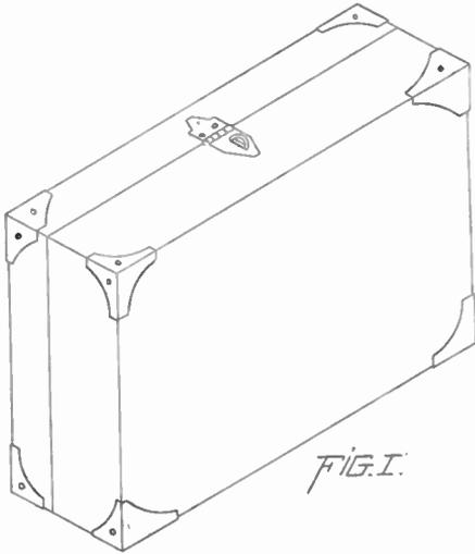
box is to be lined. Figure 1 gives a perspective view of the outside of the box as it should appear when finished, with the exception of the brass handle and padlock, these being left out for the sake of clearness.
