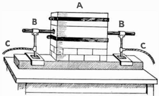
Fig. 129. Laboratory Pattern of Moissan's Electric Furnace
