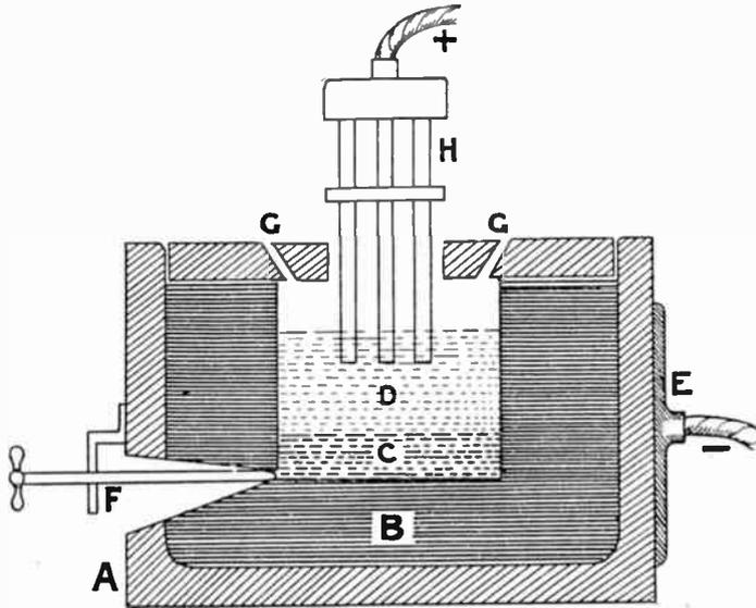
Fig. 128. Héroult's Furnace for Producing Aluminum
