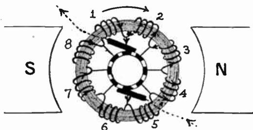
Fig. 1. Simple Ring Armature with Bipolar Field-magnet
