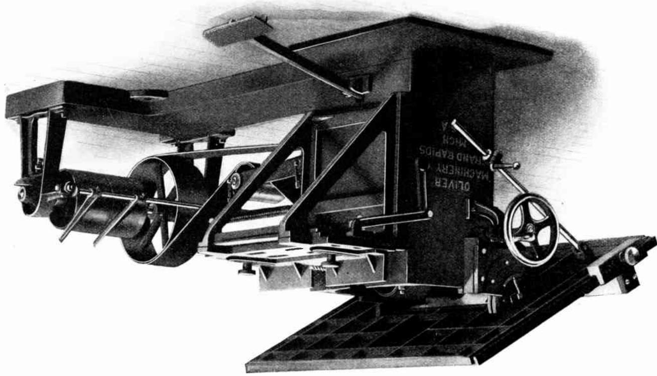
Fig. 1. A Variety Saw Table, showing Boring Attachment
