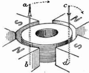
Fig. 2. Scheme of Conductors in Four-pole Field-magnet
