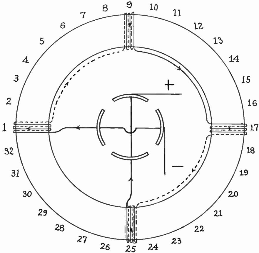
Fig. 6. Scheme of Winding a Ring Armature with Coils in Series for Use with Four-pole Field-magnet
