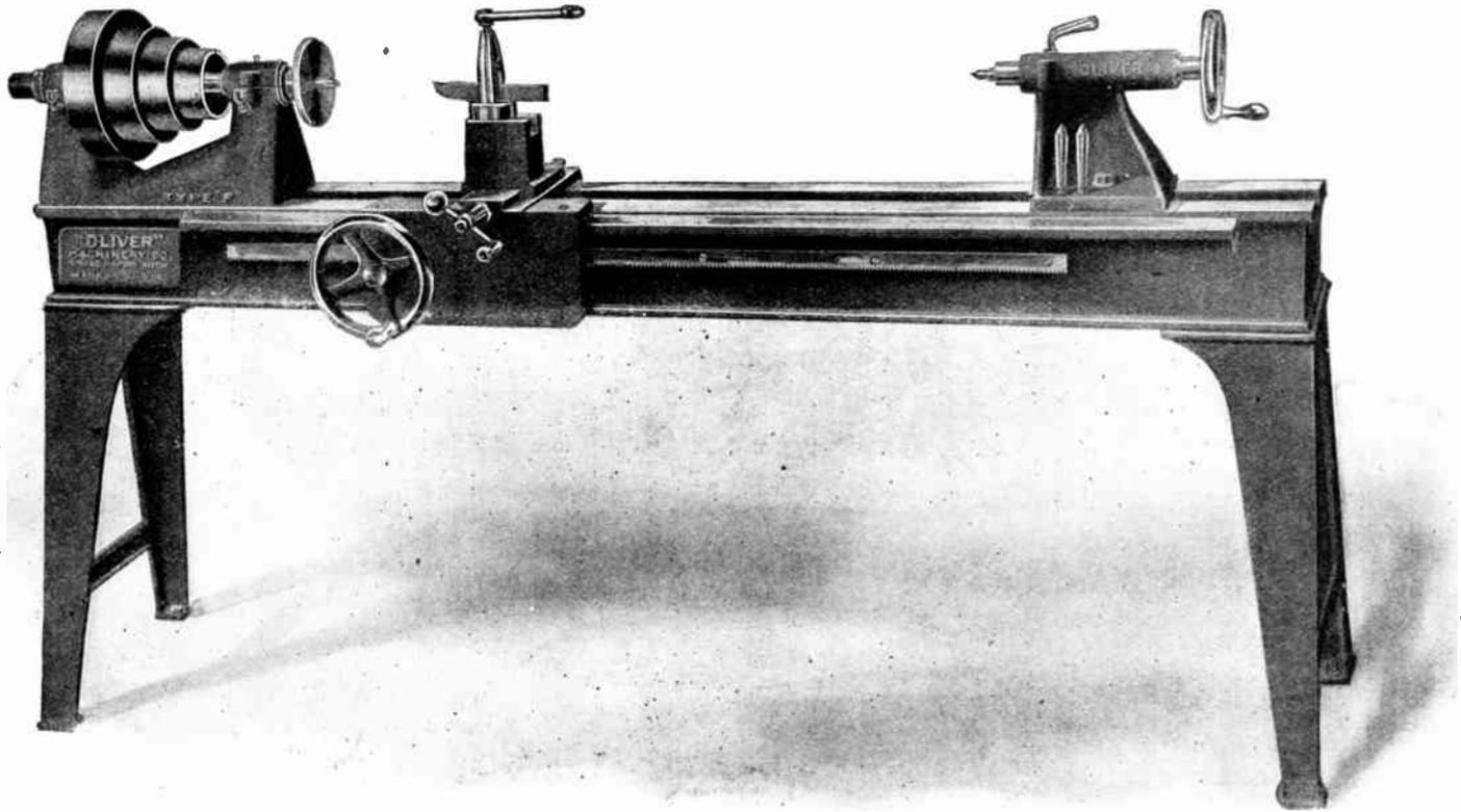
Fig. 3. Metal Bed Wood Lathe with Hand Feed Carriage
