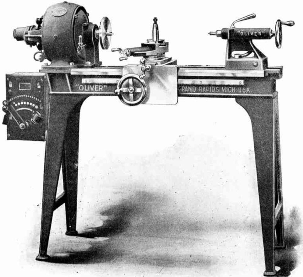
Fig. 2. Motor-head Speed Lathe
