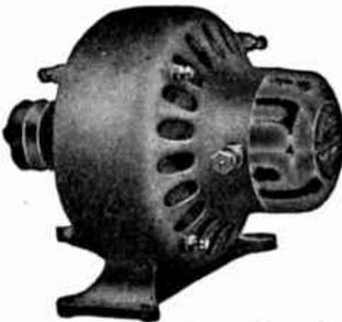
1-12 and 1-8 H. P. The only high speed, single phase, alternating motor that absolutely will not heat. Armature and field pieces are laminated. Brushes are self-adjusting.
