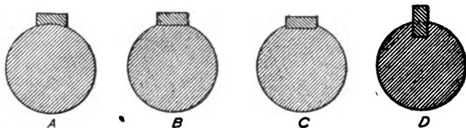
Fig. 4. Forms of Keys used for Pulleys
