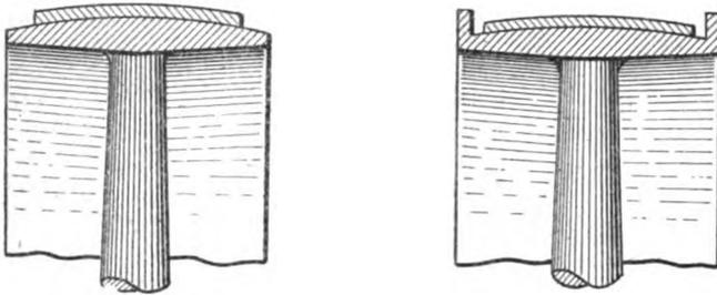
Fig. 2. Rims of Crowned and Planged Pulleys
