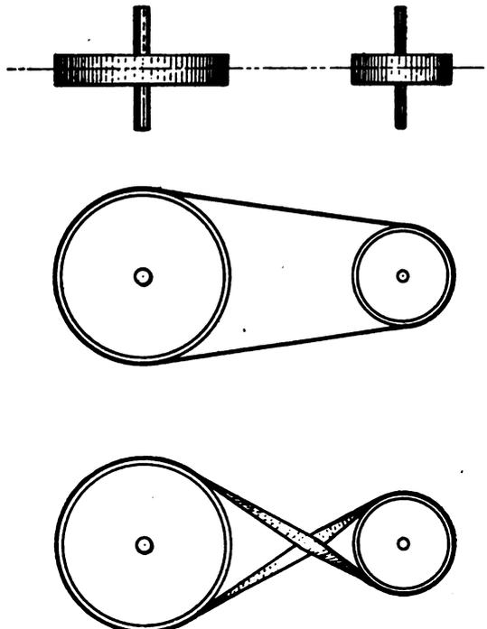
Fig. 9. Open and Crossed Belt Arrangement
