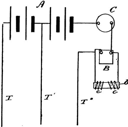
The wires *TT''* lead to the gas jet. A buzzer *B* is placed in series with the coil as indicated. This buzzer alone, however, is not sufficient to produce the result desired, for it will be found that on attempting to light the gas, that the buzzer only will ring and the spark for lighting will be at the buzzer rather than at the jet.
