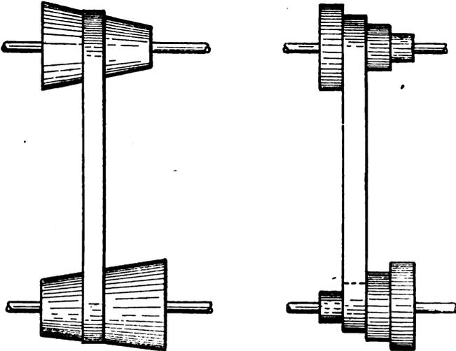
Fig. 3. Cone and Step Pulleys
