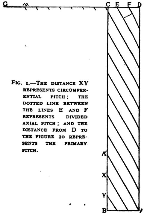
FIG. 1.—THE DISTANCE  $XY$  REPRESENTS CIRCUMFERENTIAL PITCH; THE DOTTED LINE BETWEEN THE LINES  $E$  AND  $F$  REPRESENTS DIVIDED AXIAL PITCH; AND THE DISTANCE FROM  $D$  TO THE FIGURE 10 REPRESENTS THE PRIMARY PITCH.
