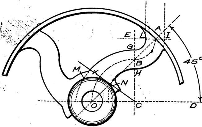
Fig. 7. Laying out a Double Curved Arm
