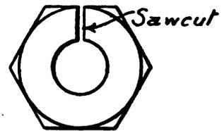
to cut another thread on the stud, but the job was done as follows: The nut was taken and a saw-cut made in one face as shown, the nut was then pinched up in the vise till the saw-cut was closed. On threading the nut on the bolt it was found to grip the remaining scraps of thread quite tightly and made a satisfactory temporary repair.
