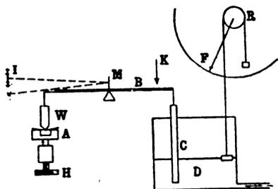
FIG. 1 — FILAMENT TESTING MACHINE.
