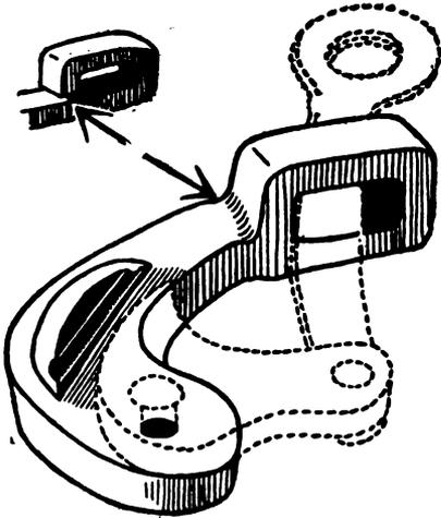
In the illustration the dotted lines show the solid steel forgings, and the makers broach a hole and pass the slip-neck through the forging, thereby making it practically an impossibility to break it. During the life of the patent on the old-style tool, it was never made in this way, and the Smith & Hemenway Co. announce that they have met with wonderful success with this new
