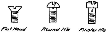
Fig. 5—Machine Screws
