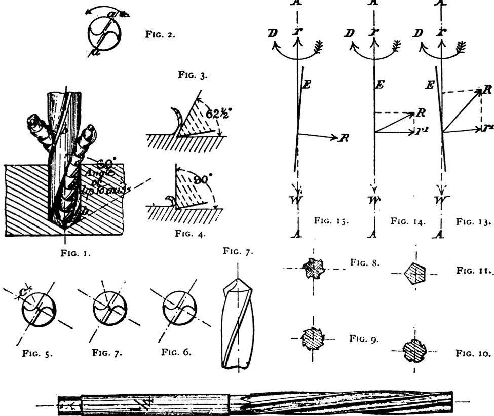
conditions in such as a lathe or planer tool. This is shown on Figs. 1 and 2, and it should be noted that the extremes of these edges *aa*, Fig. 2, must not be allowed to become worn away, otherwise the edges of the flutes will take some of the work, and the drill, sooner or later, seize and break. If it does not break, the flute edges, not being adapted for cutting, as in a reamer, will rapidly wear, thus throwing the drill out of caliber,
