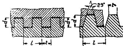
Fig. 16—Square and Acme Standard Threads
