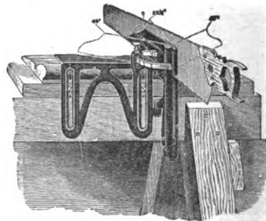
The "RED DEVIL" Mitre Box is all metal. It is light (2 lbs.) and is self-contained, that is, it is all complete, and has no extra parts to become misplaced or lost. It is so constructed that any width, depth or length of mitre can be cut, and any saw can be used. No special mitering saw is required. The mitering gauge is so simple that a child can use it. All that is required is to set the gauge at any angle.
