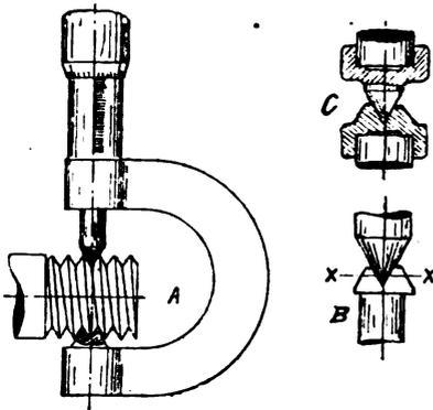
Fig. 13—Measuring Angular Diameter of Screw
