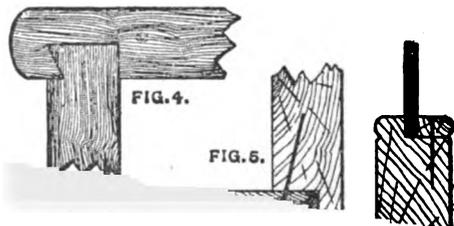
spond with the slit in the street door. If the slit is made in the horizontal door rail it should be cut in a horizontal position, but if it is in the middle vertical rail it should be in a vertical position, and a convenient size would be about 5 in. long by  $1\frac{1}{2}$  in. wide.
