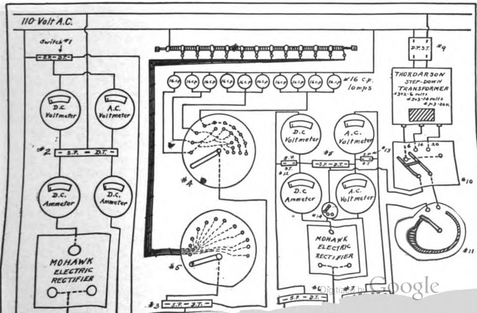
tion for 6 to 14 volts; third position for 14 to 20 volts; No. 8 to right for A.C.; left for D.C.; No. 11 as rheostat; *A.C. Voltmeter reading*, No. 7 to right; *D.C. Voltmeter reading*, No. 6 to right.
