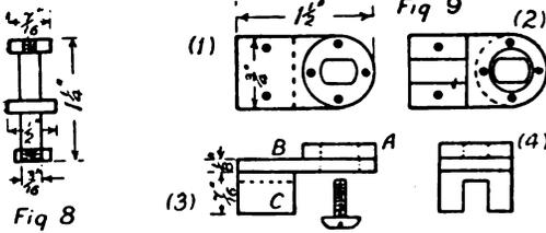
arm turns is shown in Fig. 8. It is fitted with a nut top and bottom—the latter to clamp it to the vulcanite base; and the former to act as a fixed point for a small coiled spring, shown in Fig. 1, which keeps the boss of the arm firmly pressed upon the flange of the spindle. To prevent this spring's cutting into the brass, two thin washers, not shown, are placed for it to bear upon. They can be made from softened clock spring.
