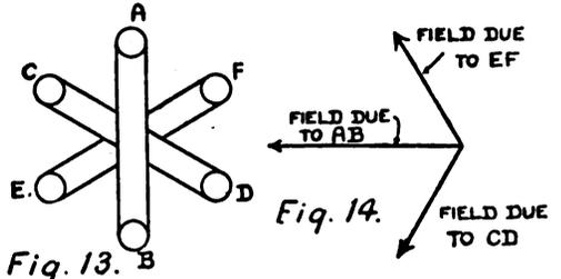
1,500 revolutions per minute. We could by increasing the number of poles still further reduce the field speed; therefore, the rotor speed. For instance, a six-pole field would give 1,000 revolutions per minute, and an eight-pole field 750 revolutions per minute, and so on; this is, of course, reckoning on a supply of 50 periods per second.
