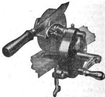
viates any danger of the knife's being jammed between the guide and the wheel, as the wheel continually lifts the knife. Sharpening it on the side face of the wheel gives a finer, smoother edge than could be otherwise attained. It leaves it also with no graining, especially if the knife is moved forward and back while being sharpened.
