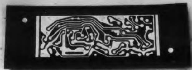
Two steps in making printed circuits are shown. Copper is first punched into the molding board and then excess copper is stripped away. Later the board is cured in a compression mold.
