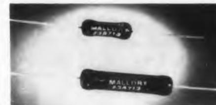
Of axial-lead construction, these types offer small physical size for their dissipation ratings. Designated types 3-AE, 5-AE, and 10-AE, they are of 3, 5, and 10 w ratings respectively. Thermally matched materials provide high resistance to thermal shock. All three types are made in accordance with the MIL-R-26C specifications.
