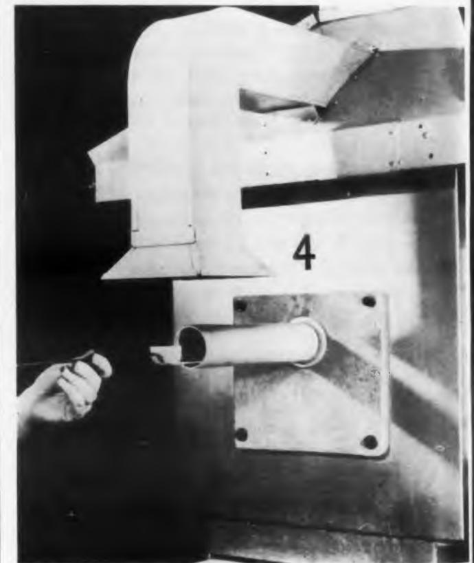
A block of ferrite material resting in an alumina tray is being inserted in a furnace for firing. The material has been improved by adding copper and manganese in proper quantities to the basic ferrite. Copper increases the reactivity of the mixture and thus decreases the firing temperature by at least 100 C. The manganese addition lowers the conductivity, making possible smaller dielectric loss.
