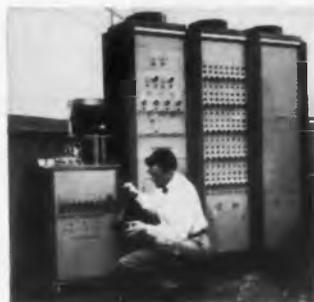
The PSI Auto-Sorter tests for as many as 8 different diode types simultaneously at a rate as high as 8,000 diodes per hour.
