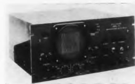
This oscilloscope has built-in quadrant switching identical vertical and horizontal dc to 50 kc amplifiers, and low noise and drift. It can be used as an output indicator with analog computers, characteristic curve generating devices, etc. Unit will operate from 105-125/210-250 v, 50/60 cy lines.
