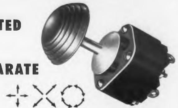
A familiar sight to helicopter pilots is this versatile Hetherington Type F441 Four-Way Switch. Here it is housed, along with other Hetherington Switches, in a hand-grip which fastens to the flight control stick. Moving the Switch's thumb-type knob up or down, right or left, operates control motors for hoists or lateral trim.
