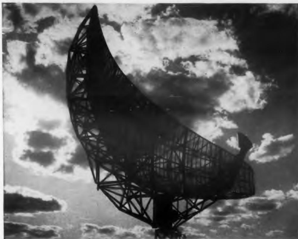
**EXTENDING THE RANGE** of radar is a constant challenge to Raytheon engineers. This 40-foot high-gain L-band antenna was designed to increase the range of existing radar and for use with new radar under development.
