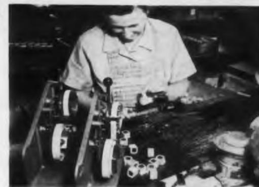
Finish wrap on Woodward-Schumacher transformer coils is made with "SCOTCH" Brand No. 28 acetate cloth tape. Thermosetting adhesive holds tight, giving good conformance and neat appearance. Completed coil is then varnished.
