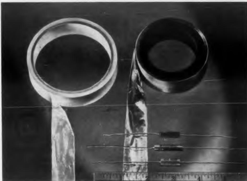
High-temperature capacitors using thin dielectric films of TEFLON are rated for a temperature range of  $-70^{\circ}\text{C}$ . to  $+200^{\circ}\text{C}$ . Shown are films of metallized TEFLON  $\frac{1}{4}$  mil thick,
