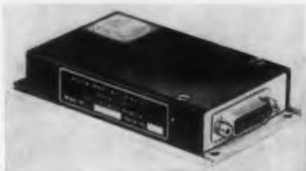
The REL-102 instrumentation amplifier covers the subsonic, sonic and ultrasonic regions. The design accomplishes the function of amplifying and impedance transforming low level signals from transducers, to a level and an impedance suitable to drive a transmission line, subcarrier oscillator, direct writing recorder or an oscillograph recorder at a considerable distance from the pick-up.
