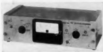
Model 412, features a single six-inch meter scale covering six decades from 10<sup>-13</sup> to 10<sup>-7</sup> amp. Response time is less than 2 sec to 90 per cent of currents larger than 10<sup>-12</sup> amp with 500 μf across the input. Zero drift is within 0.5 decade in eight hrs; accuracy, within 0.2 decade. A 216 v tap for polarizing ion chambers is provided and a 6 v output (proportional to input) can drive either 50 mv or 5 ma recorders.
