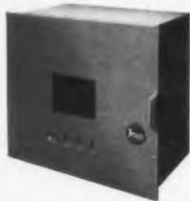
**LIBRASCOPE PUNCHED TAPE CONVERTER** operates from punched tape reader. Can be modified to operate with any digital computers furnishing a punched tape output. If printed listing desired, unit may be operated from tape-actuated typewriter, such as the Flexowriter. Programming need not be specified on tape. Sequence operation. A particular tape may be programmed to accommodate various tape formats. Accuracy, 0.1%.
