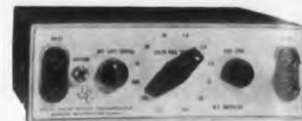
**M**ODULATED entirely by electronic means, this all-transistor dc amplifier has no mechanical chopper to introduce problems of noise, maintenance and wear. The eleven transistor unit provides sufficient gain to drive most galvanometric recorders from millivolt signals. Since no vacuum tubes are used, the unit is reliable, requires no warm-up time, and quickly stabilizes itself. A floating input allows the amplifier to operate from any source resistance.
