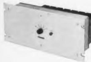
**LIBRASCOPE BINARY CONVERTER, MODEL 252** consists of two banks of relays and precision resistors simulating a precision potentiometer. The resistors weight the relays in straight binary so that each bank serves as an input to one axis of the XY plotter. Total resistance is 10,000 ohms per bank. Relays within the converter control the plot cycle. Mounting: Standard RCA, RMA rack mounts.
