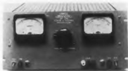
This magnetic amplifier controlled dc power supply, Model C169, has a voltage range of 0 to 150 v, at currents from 0 to 1-1/2 amp. The unit is regulated to  $\pm 1$  per cent for line or load, with a compensating adjustment control to secure positive or negative impedance, thus giving 0 per cent load regulation. Ripple is 0.1 per cent for all line or load conditions. Transient response is better than 0.2 sec. Line input range is from 105 to 125 v ac at 60 cy.
