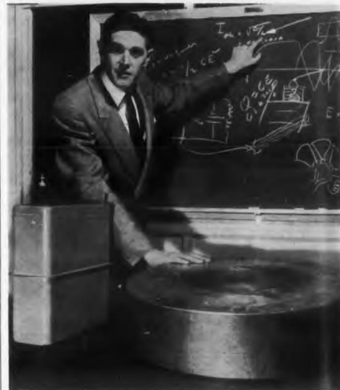
**Electron Storage Vault:** A low inductance capacitor for energy storage, built by General Electric Co., is shown at right. The unit is rated at 100 kv, 0.25  $\mu\text{f}$ , and has a ringing frequency of 2.5 mc. The existing standard type of energy storage capacitor, shown at left, is rated 20 kv, 7.5  $\mu\text{f}$ , and has a ringing frequency of 200 Kc.
