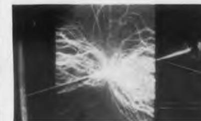
**HIGH DIELECTRIC STRENGTH.** Average of 4,000 volts per mil . . . average power factor of 0.003 at 60 cycles . . . dielectric constant above 3.0 at 72°F., 1,000 cycles.
