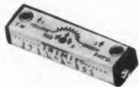
TRIMIT®—an important new development for manufacturers of computers, industrial controls, communications equipment and high-quality test and measuring equipment. Provides 33 times the adjustment accuracy of single-turn rotaries, occupies only a fraction of the space, and has far greater stability of setting—at no additional cost. Wirewound Models 271 (L), 273 (S), 275 (P). Carbon Models 272 (L), 274 (S), 276 (P).
