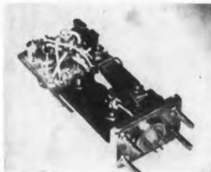
Requiring 115 v 60 cps power, this amplifier is capable of supplying up to 15 w controlled power for the operation of standard 60 cps servo motors. The amplifier has a nominal 30 k input impedance, voltage gain of 400, 90 deg phase shift and as a plug-in unit, it sits on a miniaturized 28 v dc regulated power supply as required.
