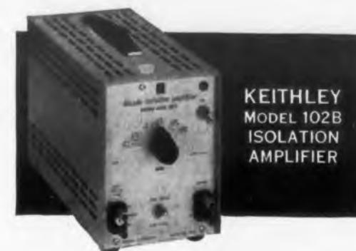
**TYPICAL** applications are: vibration and noise studies, work with accelerometers and hearing aids, and pulse amplification. A 5-volt 50-ohm output is provided for driving oscilloscopes, sound level meters, and pen recorder power amplifiers.
