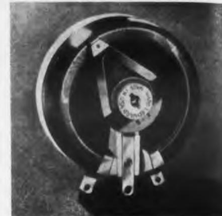
These 100 and 150 w ring rheostats have twin-shoe self-lubricating contacts; molded ceramic base and core featuring high density, low porosity, and high dielectric strength. Ratings of 100 and 150 w rings are based on a 300 C rise in 40 C ambient. Both sizes are available in resistance values to 10,000 ohms. Tapered windings, tandem mountings, dial plates, and other accessories are available.
