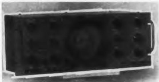
The model 85-A oscilloscope is designed particularly for the teletype communications field and allied operational systems. Emphasis has been placed on providing superior low frequency sweep linearization and balanced input dc amplifiers of high gain. The oscilloscope generally fulfills the technical specifications outlined in MIL-O-15525D, with greatly improved capabilities in the low frequency spectrum.
