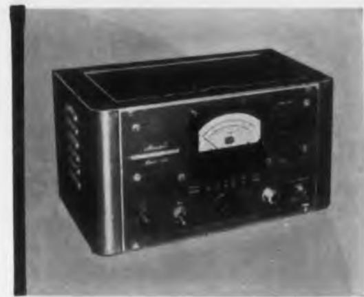
**Microline® 123B Wattmeter Bridge.** Measures average power to accuracy of 3%. Self-balancing and direct-reading, bridge operates with Microline barretter or thermistor mounts. Frequency coverage depends on mount used.
