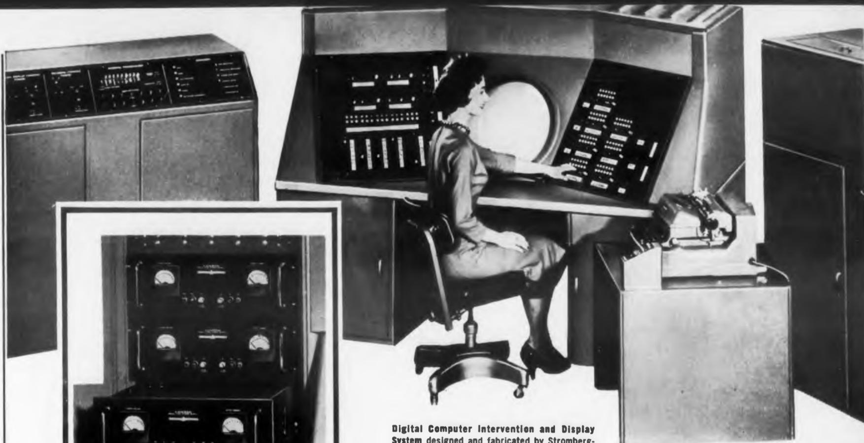
Digital Computer Intervention and Display System designed and fabricated by Stromberg-Carlson Company, a Division of General Dynamics Corporation, for the Air Proving Ground Center (ARDC) Armament Division, Eglin Air Force Base. The system is built around the CHARACTERON\* Shaped Beam Tube, designed by Stromberg-Carlson for high-speed information display and micro-film recording.
