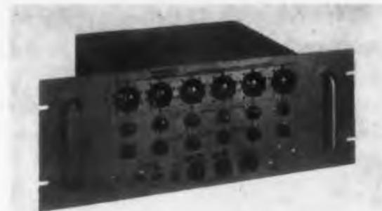
Since cold cathode glow counters and transistors are the only critical components, this counter provides substantial reliability. Available with single and dual presets, 2 to 6 digits, and optional Nixie-in-line readout, tentative specifications include a count rate above 5000 cps, sensitivity of 50 mv at 20,000 ohms, and a pulse output of 30 v. Output relay is mercury wetted, hermetically sealed, spdt.
