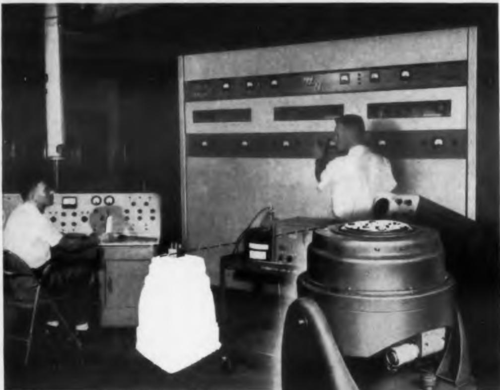
With new 6000 cps rating, the MB Model C10VB electrodynamic exciter further extends the complex motion testing range . . . yet delivers 1750 pounds force for sinusoidal testing with an MB Model T666 15 KVA amplifier (36,000 watt plate dissipation).
