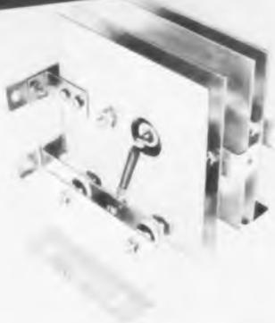
This is a 4-1-1 single-phase full-wave bridge using 303 cells on 5" x 5" copper plates. At an ambient temperature of 30° C, it will deliver up to 27 amperes d.c. with convection cooling, or 53 amperes d.c. with forced air cooling at 1000 l.f.m. The primary applications are d.c. power supplies, vibrator and magnet coil supplies, motor control, etc.
