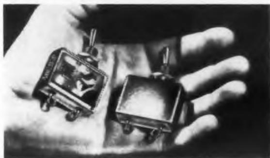
The model SM3 circuit breaker is a series-overload type designed for operation at 110 v at either 60 or 400 cps, or for 50 v dc. It is available in ratings from 50 ma to 10 amp. A choice of two time delay curves is offered, for fast or slow overload response. The breaker is also available for instantaneous-trip response.
