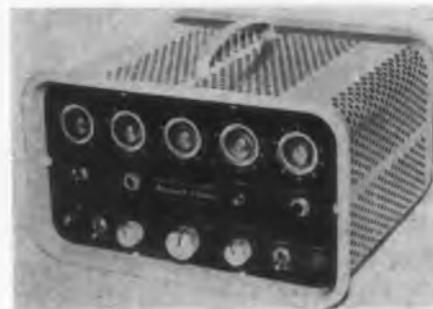
Model WE-120 five-decade frequency or events per unit of time meter and counter uses decade glow transfer tubes for both digital presentation and digital division of the time base frequency. Frequency range is 10 to 100,000 cps, and stability is 0.001 per cent  $\pm 1$  count. Sensitivity is 75 mw to 120 v rms, with 105-125 v, 75 w power input.
