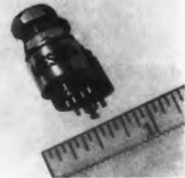
Offering high stability under temperature cycling in a small size, these Aceset potentiometers will dissipate 2 w at 60 C. They are available in nine resistance ranges between 100 and 25,000 ohms. Temperature cycling stability is made possible through the use of 20 ppm temperature co-efficient wire.
