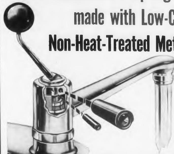
Nickel stainless steel SPIROL pins are used as corrosion-proof fastenings on "Moen" one-handle mixing faucets. SPIROL pins can be made with lower-cost, non-heat-treated metals — stainless steel, brass, and ordinary copper — because stress is evenly distributed throughout the spiral coils, giving full radial spring action, with no flexing concentrated along a "hinge" line.
