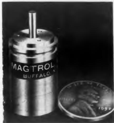
These units are available in a number of configurations, consisting of clutches, brakes, clutch-brakes, and a special dual clutch-brake. Other models are available for fail-safe or reverse energization applications. The method of mounting is with a standard 1/2 in. diameter servo mount, on either or both ends, with concentric output and input members. Shown is the model FB-59 Microbrake.
