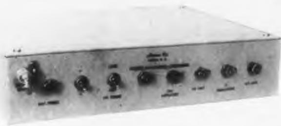
This is the compact control box for the programmed microwave attenuator.
