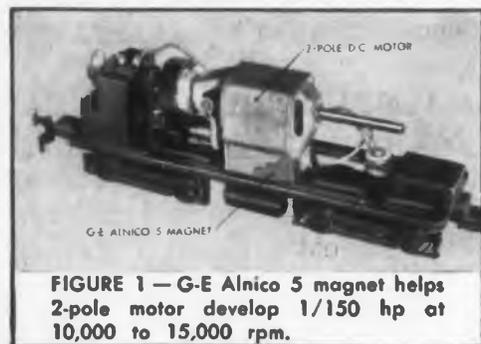
FIGURE 1 — G-E Alnico 5 magnet helps 2-pole motor develop 1/150 hp at 10,000 to 15,000 rpm.
