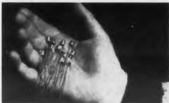
Part of the component line available from the manufacturer are 13 germanium and fusion alloy transistors in a case measuring 0.002 cu. in. There are four computer, four general purpose rf and 5 general purpose audio types. Four types of glass silicon rectifiers all rated at 400 ma forward current, having piv ratings from 225 to 500 v, and the CK1053 low power, subminiature time indicator for determining electronic component and equipment life are also included in the line.
