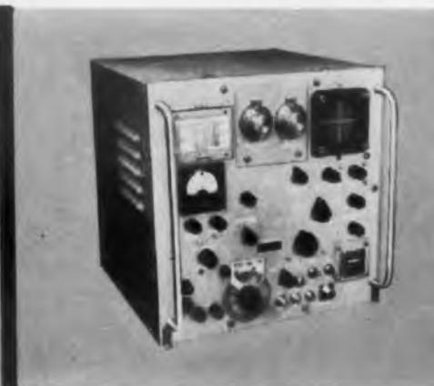
**Microline Combination Test Sets.** All are capable of measuring both peak and average power in radar systems. Also do the job of three or more standard test sets in measuring many other important system parameters. Special gating feature selects and identifies any pulse of a multi-pulse group for peak power measurement and spectrum observation. Available for Lp, S, C, X, K, and V band systems.
