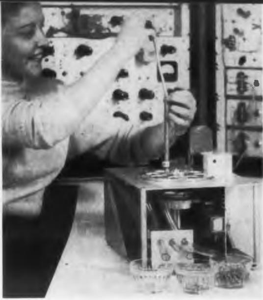
**Mechanical sorter** in operation. Cores are fed into the tube at the top and delivered to the three cups in front—the acceptable cores in the right cup, the intermediate cores in center cup, and reject cores in the left cup.
