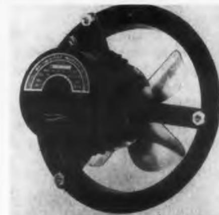
The E2123-200 is a high-speed, 3-phase, 400 cps motor. It automatically changes speed with varying altitudes and air densities to provide constant cooling efficiency from sea level (high density) to 70,000 ft. Used in conjunction with a 4-in. impeller the motor delivers 145 cfm at 0" SP at sea level and
