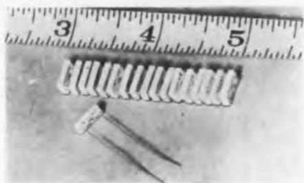
This radial series of capacitors has ratings of 300 v up to 100  $\mu$ f. An extension of the company's axial radial series, the units feature a thin design of 5/64 to 7/64 in.
