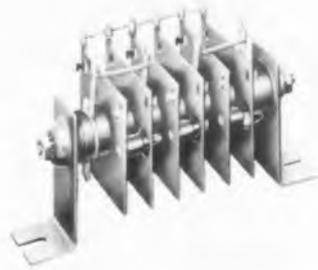
**4JA411 Stacks:** Combine high temperature operation (up to 150° C) with increased ratings (up to 18 amps d-c). Hundreds of stack combinations to meet a variety of circuit conditions. High efficiency plus excellent regulation.
