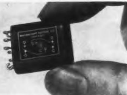
Frame and header assembly or bridge-type construction affords high resistance to shock, vibration, and temperature in this relay. Over-size instrument type bearings at both ends minimize hinge friction. The unit is hermetically sealed and filled with inert gas.
