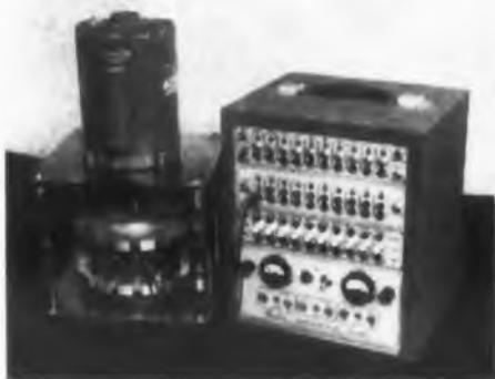
This read-write system for magnetic tape or drum memories measures 11 in. high x 11 in. wide x 9 in. deep. Individual units are entirely transistorized and printed
