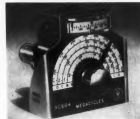
The 90680 series consists of self-indicating, absorption frequency meters covering the range of 170 kc to 700 mc. This frequency range is covered by five basic heads. Each head has three or four plug-in inductor probes and the same number of individual frequency calibrations. A single 500 μamp, end-indicating, plug-in circuit is used with each of the heads. The indicating circuit is partially self-limiting so that a high power signal will not damage it.
