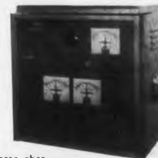
Measures all h parameters . . . provisions for measuring transistor reverse characteristics and external measurement of  $I_{co}$ . Wide range of test conditions —  $I_c$  and  $I_e$ , variable from 0.5 to 300 ma;  $V_c$ , 0 to 100 volts; frequency 200 cps to 200 KC.
