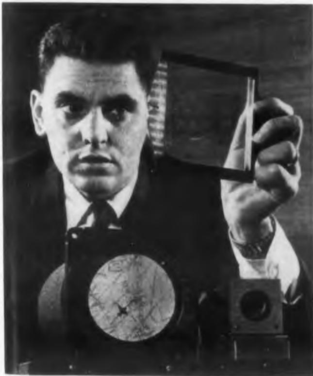
The **Horizontal Situation Display** is a TV device which permits the pilot to see his exact location in relation to the ground. The 45-pound system automatically correlates navigational computer information and presents a TV picture in the form of a map corresponding to the pilot's exact location over the terrain.
