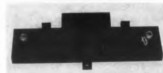
These S-band ferrite isolators are equipped with female type N connectors to meet particular coaxial requirements. Frequency range is 2670 to 2930 mc. The unit's characteristics are as follows: frequency range, 2670 to 2930 mc; isolation, 20 db min; insertion loss, 0.8 db max; input vswr, 1.2 max, and power handling capacity of 10 w average with a 2:1 load vswr.
