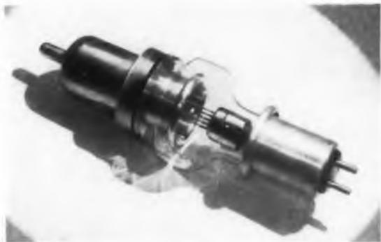
Machlett Laboratories, Inc., offers the designer a new high power rectifier tube, ML-6908. An oil-immersed high-vacuum rectifier tube capable of passing 10 amperes peak anode current, the ML-6908 is particularly suitable for high power radar installations. The tube is adaptable to certain pulsing circuits as a hold-off diode and to power
