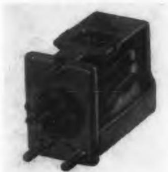
Type BHSM-HT relay is rated at 500 cps at 10 g vibration. The unit uses cross-bar palladium contacts, silicone-glass pile up insulators, a welded bracket assembly and frame, Teflon magnet wire, and a Kel-F-Coil bobbin. The relay is designed to operate at a temperature range of  $-65$  to  $+125$  C and will withstand 30 g operating shock or 70 g non-destructive shock.
