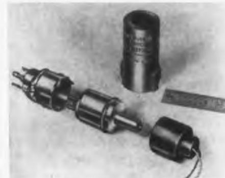
Having low thermal construction, this chopper is useful in dc amplifiers requiring thermal stability and low noise. Contact ratings and reliability are identical with the company's standard external coil units. As in the standard
