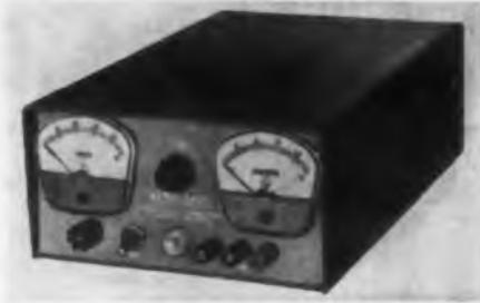
The transistorized Model SC-18-0.5 delivers 0 to 18 v, 0 to 0.5 amp. Regulation for line or load is less than 0.1 per cent or 0.003 v, whichever is greater. Ripple is less than 1 mv rms. Recovery time is less than 50  $\mu$ sec. Stability for 8 hr is less than 0.1 per cent of 0.003 v, whichever is greater.
