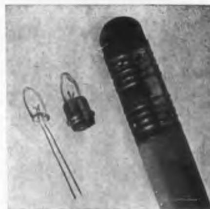
Burning continuously at 5 v, this lamp can be expected to last 60,000 hours or 7 years. It measures 1/8 to 1/4 in. in length. The lamp withstands voltage surges up to 30 v.
