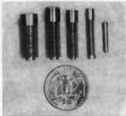
These flexible metal bellows range from 1 to 0.125 in. O.D. and come in any wall thinness down to 0.0008 in. The metal is a nickel alloy of high tensile strength and low hysteresis with resistance to corrosion and temperature.
