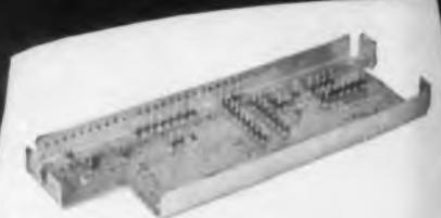
Turret terminals of various types and configurations may be hopper fed into the boards from the underside, thus allowing the operator a clear view of the riveting operation. The utilization of the spin rivet feature coupled with adjustable impact and timer control give consistent results. Cracking and splitting of terminals, particularly the stand-off and feed-thru types, has been virtually eliminated.
