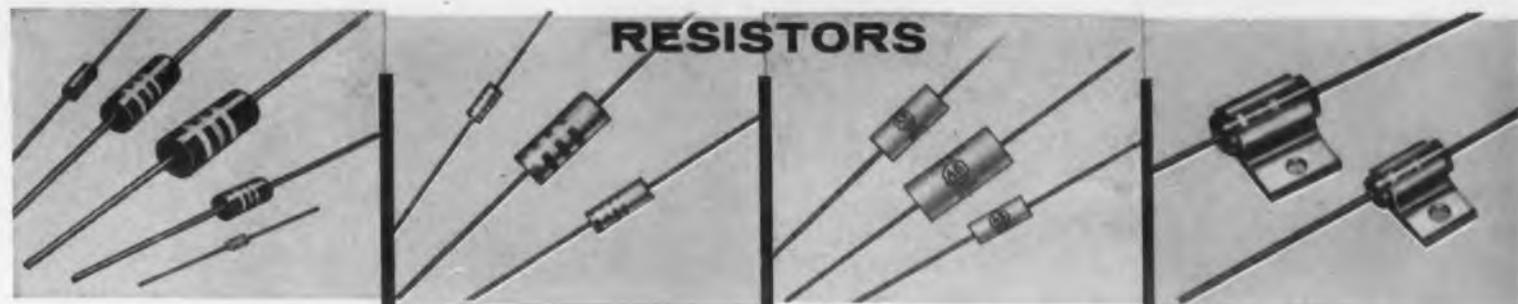
**HOT MOLDED COMPOSITION RESISTORS**—Quality standard of the industry. Rated at 70°C, in 2, 1, 1/2, 1/4, and 1/10 watts. Res. to 22 meg. Tol: 5, 10, and 20%.
