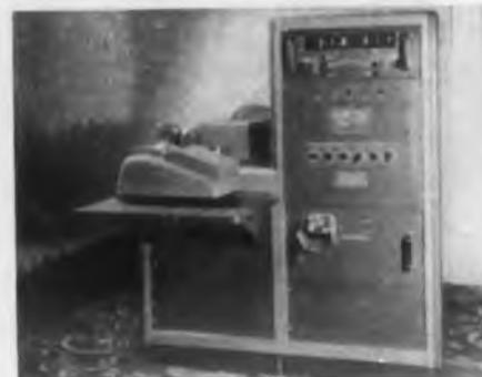
The SPACE self-programming automatic cable evaluator checks for leakage and continuity between wire ends of a cable harness. Using a computer type memory, it performs up to 10 tests per second and can generate its own tape program.
