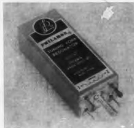
For operation with transistors or tubes, MJ series tuning fork resonators take 15 g 11 msec shock. In frequencies from 400 to 2200 cps, and in 0.01, 0.02, or 0.05 per cent accuracy ratings in -55 to +85 C range. Accuracies unaffected under 5 g vibration to 40 cps.
