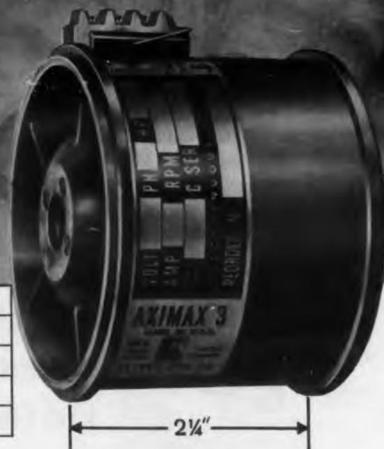
For airborne and missile cooling applications, the AXIMAX-3 when turning at 20,000 rpm will deliver 165 cfm at free delivery. This performance is possible although the fan is only 2.8" in diameter, 2.3" in length and weighs a mere 14 ounces.
