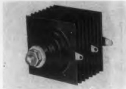
The selenium in these rectifiers has parallel grains. This structure allows higher current ratings for a given cell size. The rectifier is available in cell ratings of 18 to 36 v.
