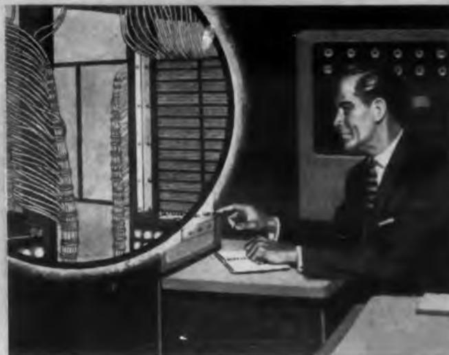
**ELECTRONIC BUSINESS MACHINES**—Non-flammability, safe emergency overloading, and solder resistance are three important reasons why TFE resins are used in machines such as this data-processing equipment. Servicing of wiring panels can be done quickly, with a minimum of downtime, because TFE resins are unaffected by soldering temperatures.
