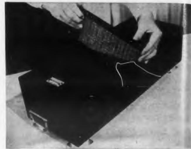
**Gevic computer**, for a typical fighter bomber application, will weigh only 45 pounds and occupy 0.8 cu ft. Arithmetic module is being inserted in package.
