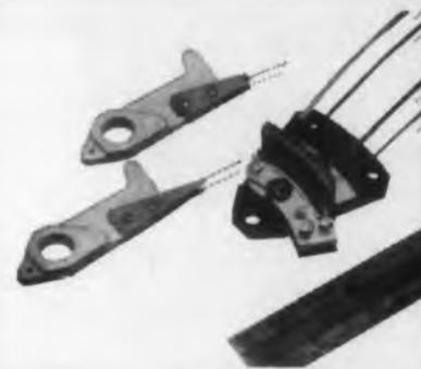
DUAL COIL SECTOR UNIT in which elements are independently phasable with slider positions.
