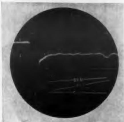
Germanium diode S570G has a 0.9  $\mu$ sec switching time. It has a stored charge, after a 10 ma forward current, smaller than that of a 3  $\mu$ f capacitor at 6 v. The S555G diode is specified at 6  $\mu$ sec and offers better dc characteristics.
