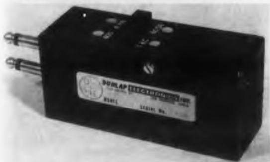
PO-2 and CO-2 oscillators furnish audio signals of 1 kc and 400 cps at output levels of 0 and -60 db at an output impedance of 600 ohms. In the PO-2 output is available at two phone plugs; in the CO-2, at two clip leads.
