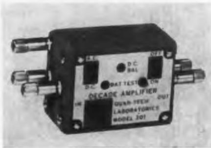
The frequency response of the Model 201 decade amplifier is flat within  $\pm 2$  per cent dc to 100 kc, and 1 db to 500 kc. Its input impedance dc-coupled is 400 K shunted by 30  $\mu$ f; output impedance is nominally less than 100 ohms. It is a gain of 10, and its equivalent noise level is less than 20  $\mu$ v.
