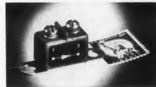
This single silicon diode package offers protection against extremes and is qualified per MIL-T-5422C. It has forward current ratings up to 400 ma, and inverse voltage ratings up to 600 v.
