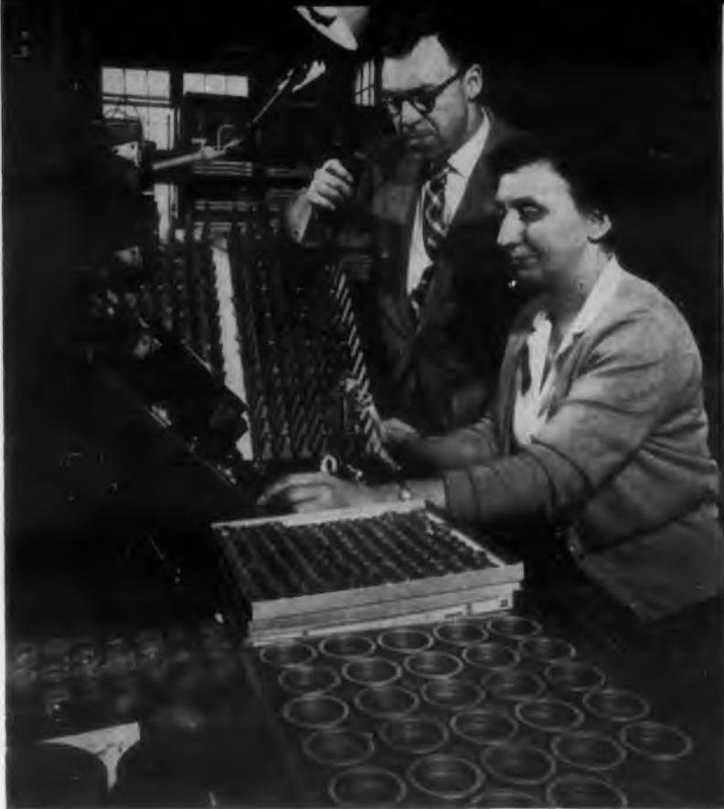
Mr. Cliff Horstman checks performance readings for Hipermag cores using the Roberts Dynamic Tester. This production-line test eliminates costly and complicated testing at your plant. After the Roberts test, Hipermag cores are "pegged" here according to their performance characteristics. This practice assures perfect performance-matching every time.
