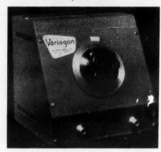
The V-71 phasemeter provides a simple compact and inexpensive measuring and phase calibrating instrument over a very wide frequency spectrum of approximately 100 cps to 5 mc. The instrument offers a 360 deg continuous phase-shifting system utilizing a Variogon phase-shifting transducer.
