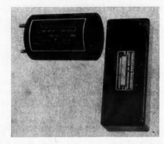
Designated the PA5A and the PA5C, these magnetic amplifiers are capable of proportional control of up to 90 w output power with input power of a few milli-microwatts. The PA5A has a cylindrical case, the PA5C a rectangular case to meet different mounting requirements.
