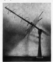
Model MAM-1000 telemetry antenna is for use where the antenna can be manually oriented. It also comes with a remote controlled motordriven mount. Unit pictured is a 4-turn helical beam antenna with a 50 deg acceptance angle and a 10 db gain over an isotropic source.
