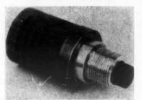
Trapped pools of mercury slide in and out of contact to operate this push button switch. The spdt break before type unit has no contact bounce or chatter. It mounts in any position and stands 15 g shock and vibration.
