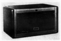
Providing a static nulling error of 0.02 per cent, the DLI-101 servo multiplier has two channels, each of which multiply three variables by a fourth. Its automatic gain control feature maintains constant loop gain for reference voltage variation in the 2 to 100 v range. The unit is composed of Digitrol plug-in building blocks.
