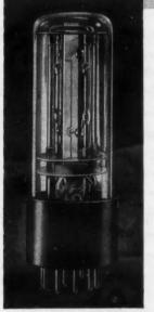
Precision components of the new RHG-DP crystals are enclosed and hermetically sealed in glass holders to assure maximum internal cleanliness and most reliable evacuation. The result is a series of sturdy, miniature, low frequency units having excellent long-term stability and higher Q.
