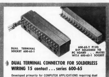
Developed primarily for COMPUTER APPLICATIONS requiring dual solderless wiring leads for each single contact. The right angle plug is dip soldered to the printed circuit board and mated with the dual terminal socket. Socket terminals are precision machine tapered for AMP "53" solderless wiring. Contact rating 20 millivolt drop maximum at 7.5 amps. Connector rating 500 volts RMS.
