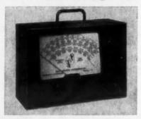
Frequency meter T-2 has 14 ranges from 25 cps to 80 kc and 7 ranges from 1250 to 80,000 rpm, all in direct reading scales. Accuracy is 1 per cent. The unit accepts voltages from 10 my to several hundred volts at high impedance.
