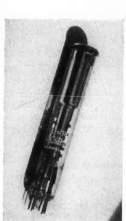
Machlett Laboratories, Inc. makes available to the designer the ML-6198, a small television camera tube intended primarily for industrial use. Tube design includes a photoconductive layer as a light sensitive element characterized by a spectral response approaching that of the eye.
