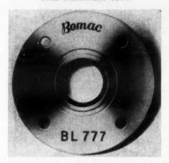
The BL 777  $K_u$ -band pressurizing window has a maximum vswr of 1.12 over a frequency range of 12.4 to 18.0 kmc. The BL 777 can be pressurized to a maximum pressure differential of 30 psi and will operate up to 100 kw maximum.
