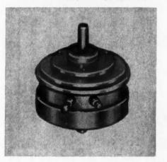
Half as long as its mounting diameter, the model PC-8 precision clutch has encapsulated coils, fixed terminals, 1.000 servo mounting diameter, and guaranteed torque of 16 oz in.
