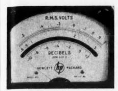
Model 400L vtvm has a logarithmic meter designed to eliminate optical confusion and provide an accuracy which is a constant percentage of the reading. This was accomplished by expanding the lower portions of the voltage scale and by providing a linear decibel scale which spreads 12 db over the full scale length. The unit has two voltage scales ranging from 0.8 to 3.2 and from 2.5 to 1. It measures any voltage from 0.3 my to 300 v in the 10 cps to 4 mc range.
