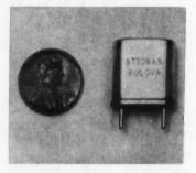
Series ST-70NXS low frequency crystals cover a frequency range of 100 to 250 kc with a frequency tolarance of  $\pm 0.015$  per cent from -55 to +90 C. They stand 100 g initial shocks and 20 g vibration up to 2000 eps.
