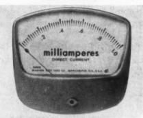
Panel meter MM-5 occupies panel space of conventional 4-5/8 in. meters and mounting space of ASA/MIL 3-1/2 in. units, yet provides greater scale length and readability. Tracking can be held to 0.5 per cent of full scale, when plotted linearly or with a protractor reference for deflection angles up to 100 deg.
