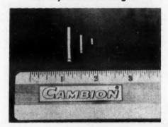
For mounting to terminal boards or panels, the X1246 rivet standoff comes in shank lengths to accommodate panel thickness from 1/32 to 1/4 in., and in eight mounted heights above the board, from 1/8 to 1 in. Internally threaded, the rivet standoffs are finished with 0.003 in. cadmium plate.
