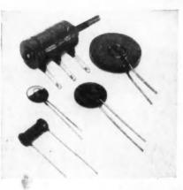
GLOBAR Type BNR varistors are nonlinear (voltage-sensitive) resistors for voltage control and stabilization applications. They are made from the highest electrical grade silicon carbide, ceramically bonded into disc, rod and cylindrical shapes. Flexible production facilities make possible a wide range of physical sizes, watt ratings and changes of resistance with applied voltage. For details, write for Bulletin GR-2.
