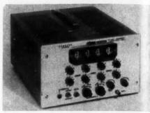
Preset range of this transistorized counter is 0 to 180,000 counts per minute with instantaneous reset. Totalizing speed is 0 to 300,000 counts per minute. The unit features direct reading and long service life
