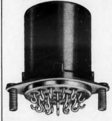
TYPE MHJ ACTUAL SIZE Includes materials and processing necessary to minimize contact resistance variations and dielectric deterioration during life due to contact contamination, mechanical wear and shift of adjustments with
