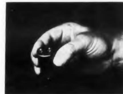
Miniature RM-73 gas density switch detects gas leakage and critical arc-over gas density. It actuates along a temperature line of 0.025 psia per deg Rankin. Rated 28 v dc, 110 v ac, 100 ma, spst or spdt, the unit stands  $\pm 20$  g shock, 10 g vibration from 5 to 1000 cps, and  $-85$  to  $+200$  F. It meets MIL-E-5272 specifications.
