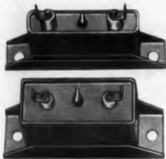
The E-315 capacitor operates from  $-55$  to  $+315$  C. Capacitance is  $0.05$  to  $4 \mu\text{f}$  at  $600$  v dc, with higher voltages available. The unit has been tested for 1000 hours at maximum temperature and rated voltage.
