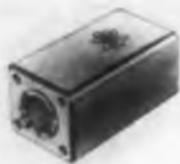
These dc amplifiers have adjustable voltage gains of 100 to 500. Linearity is  $\pm 0.5\%$  based on a 5 v dc output value. The units are 2.5 x 1.19 x 1.19 in. and weigh 7 oz.
