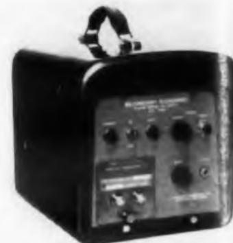
Portable type Q3401 secondary standard has plug-in units for gage differential, and absolute pressures and is suited for calibration or direct parameter measurement. Accuracy is 0.05% for ranges up to 2500 psig, psid, or psia.
