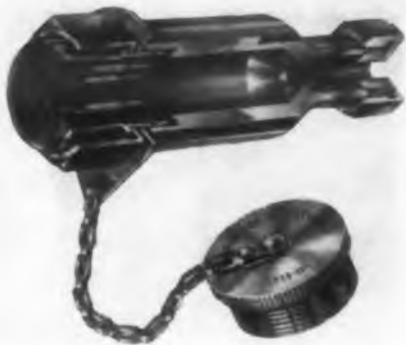
Weatherproof LR and MR connectors have clear and black anodic coating to resist corrosion and rubber glands and gland nuts to seal out moisture. Chain-attached caps seal unmated units. Coupling threads and sizes are standard to MIL-C-5015.
