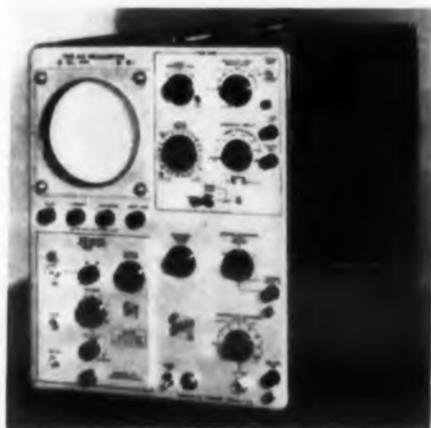
A fast-rise, cathode ray oscilloscope, type 543 handles dc to 30 mc. For versatility, nine plug-in preamplifiers are available. Sweep range is 0.02  $\mu$ sec per cm to 15 sec per cm; accelerating potential is 10 kv. The built-in voltage calibrator has 18 outputs from 0.2 mv to 100 v peak-to-peak. The unit has sweep magnifications of 2, 5, 10, 20, 50, and 100 times. A single knob controls 24 direct-reading calibrated sweep rates.
