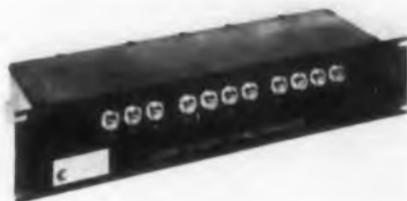
By simple switching, this converter translates pure binary code to binary decimal code. No error is introduced in the translation process.
