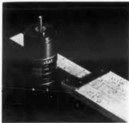
Having a terminal linearity of 0.05%, the series 4 Vernistat's diameter measures 1.062 in. Units are available with maximum output impedances of 200, 100, and 40 ohms. Resolution is 0.01%. Weighing in at 2 oz, the unit can be produced in nonlinear versions.
