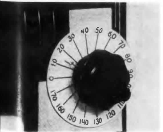
illary scale, drawn on polar paper, extends the frequency usefulness of an RX meter.
