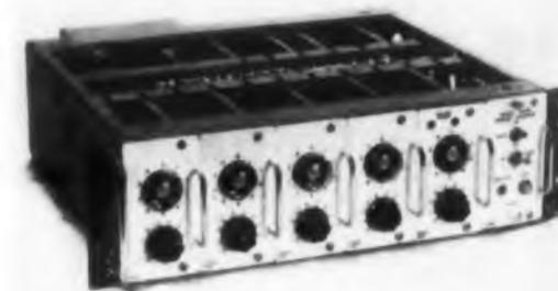
Made of printed circuit plug-in modules, the 7250C five decade preset counter operates to 100 kc. It will recycle at rates to 5 kc without missed counts. The unit features pulse and variable duration or locking relay contact output and gated input.
