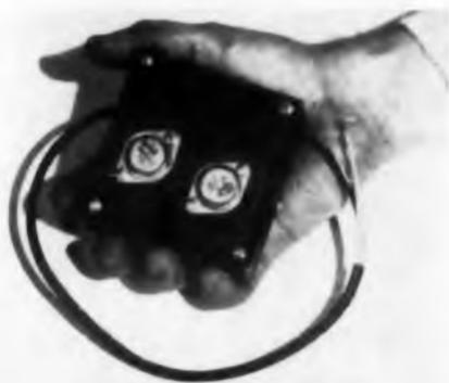
There are no moving parts or vibrators in this rugged power supply. Converting battery to B voltages with 80% efficiency, the unit has 0.05% output ripple and 0.3 v rms input ripple. It is 3.5 in. sq and 1.7 in. high. Models TPS-1 and TPS-2 have outputs of 100 ma, 150 v and 200 ma, 250 v, respectively. Inputs are 12 and 24 v.
