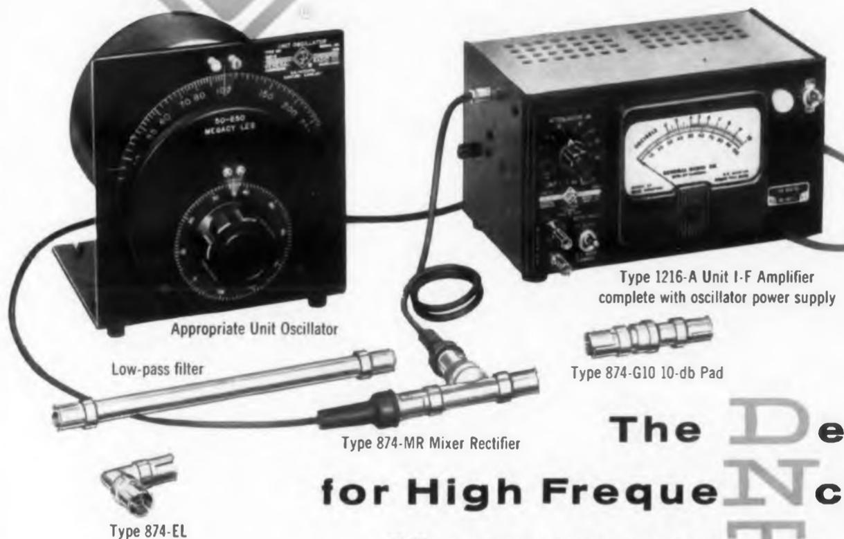
The DNT Detector Assembly operates on the heterodyne principle. Its local oscillator is set 30 Mc above or below the incoming signal to produce a difference frequency at the output of the mixer. Since the mixer operates linearly over an 80-db range, the level of the detected signal can be amplified and accurately measured with the calibrated step attenuator and meter built into the I-F Amplifier.
