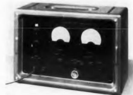
Type B-731A meter may be used for JAN MIL vibration tests on electronic components. It permits remote measurement of vibration distances from 50  $\mu$ in. to 0.5 in. and vibration rates from 1 cps to 10 kc. Accurate to 2%, the unit has a noncontacting probe and can measure the dilation and eccentricity of rotating parts.
