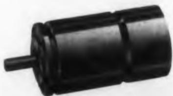
No-load speed of the 8 IM 420 size 8 servomotor is 6000 rpm. Flywheel inertia is 2 gm cm<sup>2</sup> and flywheel damping factor is 40 dyne-cm-sec/rad. The unit has a 26 v fixed and a 40 v center-tapped control phase. It stands 30 g vibration and 100 g shock to 2000 cps and operates in ambient from -55 to +130 C. It also meets MIL-E-5272A requirements. Power input is 2.6 per phase.
