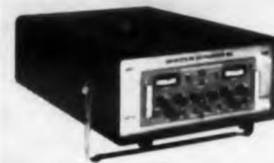
Model 940 dual channel amplifiers are designed to drive the company's 102 and 120 galvanometers. Frequency response is dc to 10 kc  $\pm 1$  db; input impedance, 1 meg constant; input sensitivity,  $\pm 1$  to  $\pm 100$  v for full scale output. The unit can provide  $\pm 10$  v at 200 ma.
