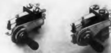
Small, lever action switches, series 12000 have silver contacts rated at 3 amp, noninductive load. In 2 and 3 position types, they are locking and nonlocking. A 3 position model locks on one side only.
