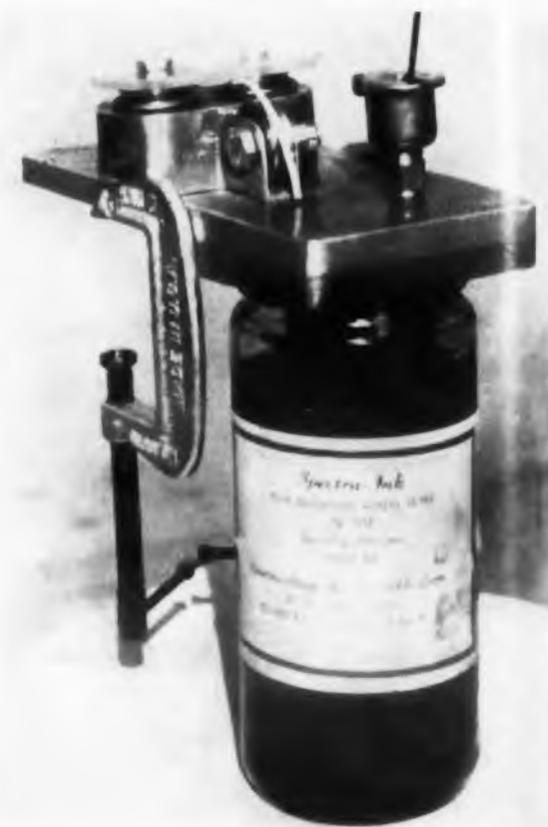
Spectra-Coder model 701 dyes 500 ft of wire a minute. It handles any vinyl insulated wire, and can be used with Spectra-Ink or other instant drying ink.
