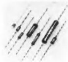
These Blue Jacket resistors are vitreous-enamel, wirewound power units with axial leads. The 2 w size is 3/8 in. long; the 2-1/2 w, 17-32 in. long. Diameters are 3/16 in. Tolerances are  $\pm 1$ ,  $\pm 2$ ,  $\pm 5$ , and  $\pm 10$ %. The series also includes 5, 7, and 11 w units.
