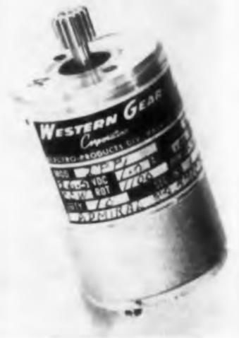
Rated 1/100 hp at 11,000 rpm, model 2PPI miniature motor is qualified according to MIL-M-8609 specifications. A 26.5 v dc unit, it is 1.18 in. in diameter and 1.9 in. long and weighs 3.5 oz. It will run 500 hours without change of brushes.
