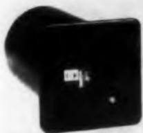
Vernier potentiometer 81-A is a three decade voltage divider with a Kelvin-Varley circuit and a parallax-free dial that registers to four places. Standard resistance is 10 K; accuracy,  $\pm 0.05\%$ ; linearity,  $\pm 0.01\%$ ; resolution, 0.002%; power rating, 5 w; frequency range, dc to 10 kc.
