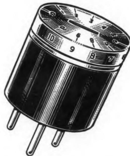
Fig. 1. End cap of potentiometer is dual-calibrated. Unit is enlarged over three times.
