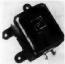
Preset for 20 to 180 sec delays and voltage compensated from 22 to 32 v dc, these time delay relays operate from -65 to +125 C. Series IR units are spno or spnc; series TR are dpdt; and series STR are spdt. All are rated 2 amp at 28 v dc, resistive.
