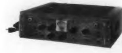
Model 703 microwave leveler flattens rf power to  $\pm 1$  db from 2 to 4 kmc. It may be used with backward wave oscillators, klystrons, signal generators, and twt amplifiers. The unit also provides variable attenuation over the dynamic range of an associated control device.
