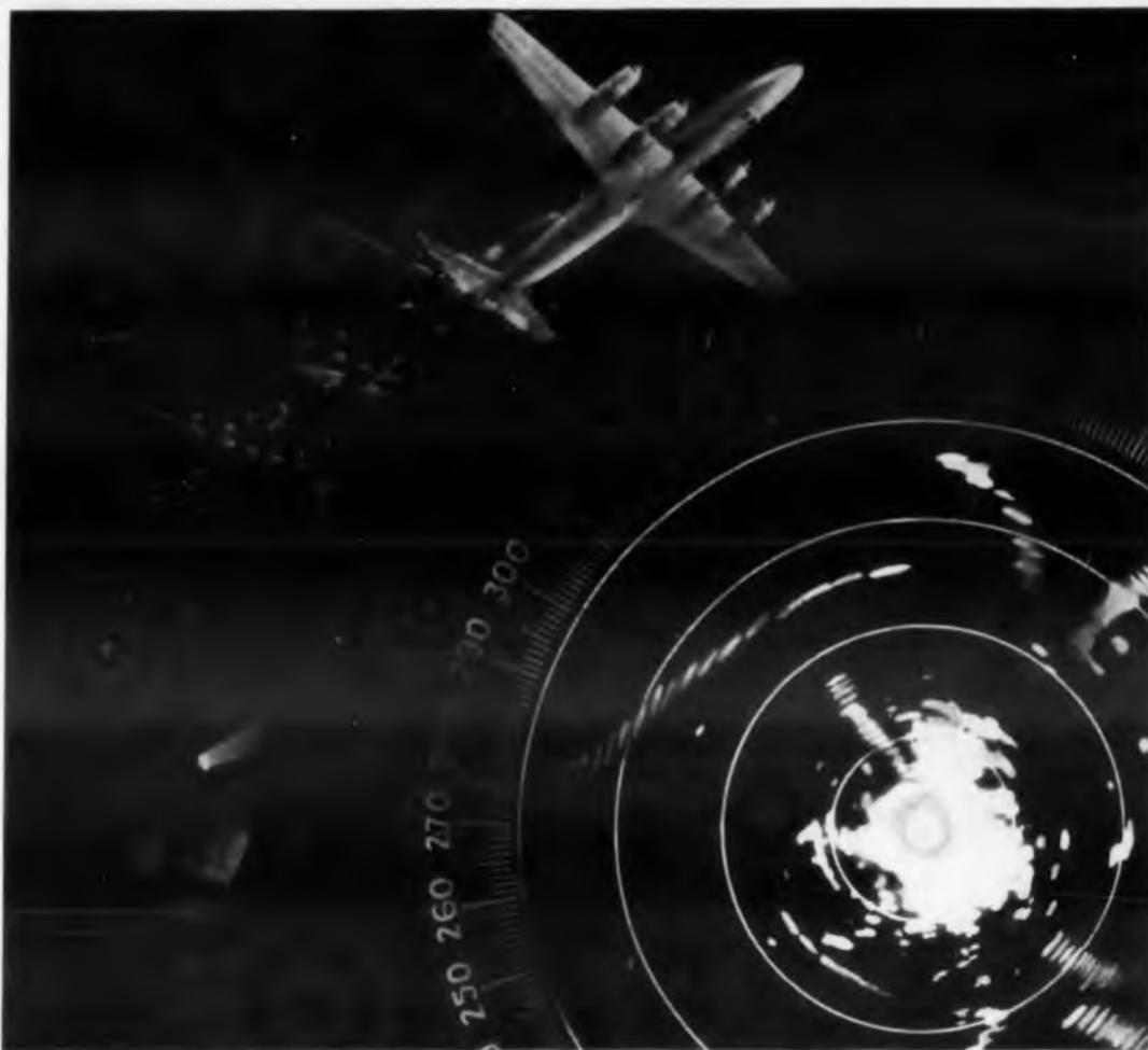
**MOVING-TARGET INDICATOR** is just one of the many dramatic achievements Raytheon engineers are making in radar every day. This development applies the electronic memory of a recording storage tube to a standard plan-position indicator (PPI).
