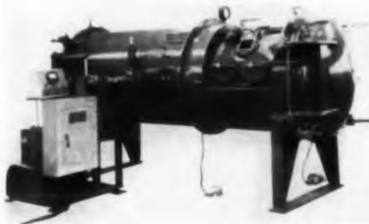
Type 742 inert gas welding machine is a production unit for reactive materials such as zirconium, tantalum, and columbium. For manual or semiautomatic operation, it has dual welding positions with glove ports, sight glasses, automatic welding shields, and lights. It has a high speed, high vacuum pumping system and an inert gas backfill system. In lengths from 6 ft, the units are 42 in. in diameter.
