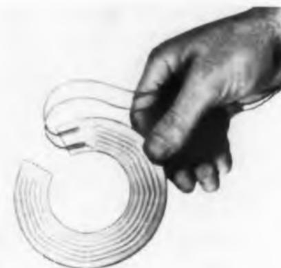
Flexible and rugged, Thermal-Heaters are designed for airborne and other electronic equipment. These 43 w circular heaters weigh less than 1/4 oz, including the 12 in. leads. They are under 0.03 in. thick over the element and less than 0.065 in. thick over the leads. They may be clamped or cemented to flat or curved surfaces. Insulation resistance is 1000 v rms. Heaters in various sizes and shapes are made to customer specifications.
