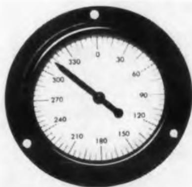
Using a dc synchro and a potentiometer transmitter, this remote readout system reads valve flapper and shaft angles through 360 deg. Accurate to 0.5%, it operates from 28 v dc and requires less than 0.1 w.
