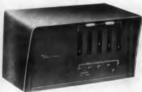
With a single zero, this decimal electronic counter indicates true positive and negative numbers. Counting to ±99999, it operates at rates up to 50 kc. Available with a buffer storage unit, the counter receives its input from a photoelectric shaft to pulse converter which generates 10 counts per shaft revolution.
