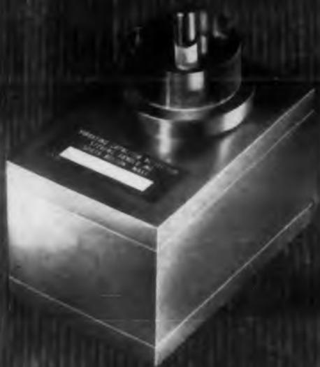
A vibrating-reed type capacitance modulator for use in measuring currents as low as  $10^{-16}$  amperes.
