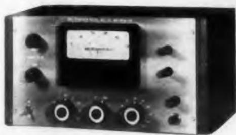
Voltage calibrator model 600 has two ranges, 0 to 5 and 0 to 50 v dc, with available current up to 5 ma. Each is divided into 10 steps with ±1% accuracy of adjustment. Input is 115 v ac, 60 cps.
