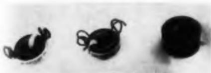
Wound toroidally on molybdenum permalloy powder cores, these high Q coils have inductances from 5 mh to 5 h, accurate to 1%. Open, epoxy encapsulated, or molded, they are 1-5/16 in. in diameter and 11/16 in. high.
