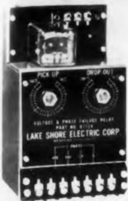
This differential voltage sensing relay protects radar gear, microwave relay systems, and other equipment. Its control range is 70 to 100% of rated voltage for both dropout and pickup with a minimum 1 v differential. Dc ranges are 6 to 49 v and 50 to 250 v; ac ranges are 1 and 3 phase, 3 and 4 wire.
