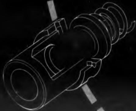
Pilot section of this pressure relief valve has poppet ball (red) and seat of LINDE Sapphire. Valve was designed and manufactured by Whittaker Controls Division of Telecomputing Corporation
