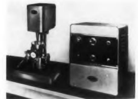
Model 2-335 ultrasonic impact grinder cuts slices, drills, and trepans regular and irregular shapes. It handles semiconductors, ceramics, ferrites, carbides, metals, jewels, and other hard or brittle materials. Its magnetostrictive transducer permits a 100% duty cycle.
