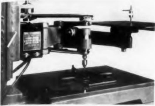
Unskilled operators can drill 100 holes a minute with the model D-2 printed circuit engraver. Various holes can be drilled without changing tools. For two dimensional work, this pantograph has an air cylinder attachment and a single micrometer adjustment for height.
