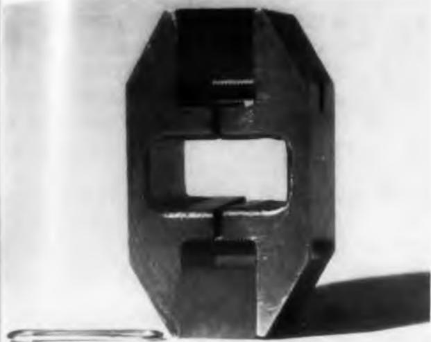
Fig. 4. Pole-piece design, showing detail of special silicon steel extrusions.
