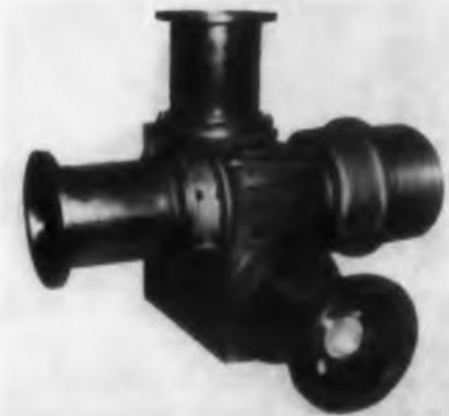
Type 1038 coaxial switch has a 0 to 450 mc frequency range and a vswr under 1.05. It is designed for 6-1/8 in. coaxial transmission lines and has about the same cw power rating as they do. It comes in motor and manually operated models.
