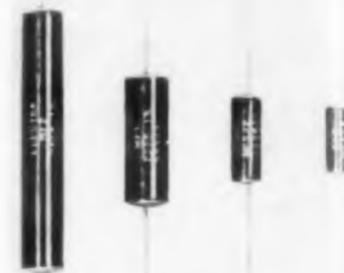
These molded metal film resistors feature low controlled temperature coefficient, low noise level, and long stability under severe humidity conditions. Their precision is comparable to that of wirewound resistors. The units offer good performance, and uniformity of values over wide resistance ranges. They come in five sizes from 1/8 to 2 inches.
