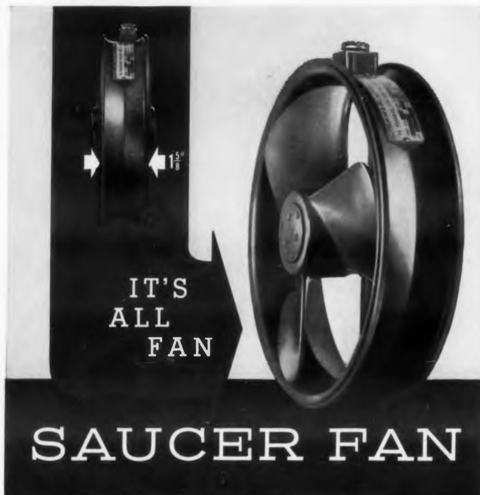
The Saucer Fan represents an entirely new design concept whereby the driving motor is built within the propeller hub limiting its axial length to the minimum measurement required by a highly efficient motor. Ideally suited for tightly packed electronic packages, where space is critical, the Saucer Fan will provide cooling air to the amount of 280 cfm. Power requirement is 115 vac. 50-60 cps, 1 0.
