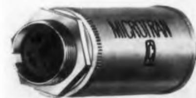
Ruggedly built, this in-line microphone input transformer is designed for insert into cable circuit. It features a shielded core of Mumetal and electrostatic shielding to improve its signal to noise ratio. The unit has a frequency response of 20 cps to 20 kc ±2 db. Supplied with in. shielded microphone cable, it mates with Amphenol 91-PC-100 plugs. Weighs 11 oz; 1-1/8 in. diam., 2-3/8 in. long.
