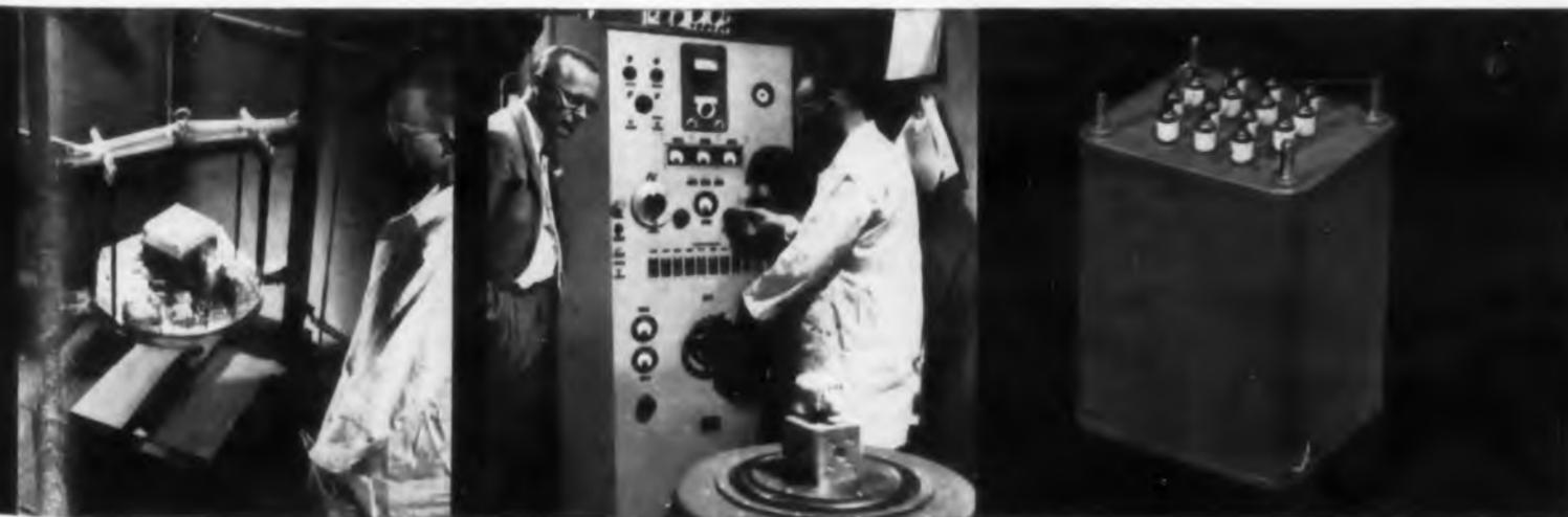
Westinghouse electronic transformers being shock-tested according to specifications of MIL-T-27A with new in-plant qualification testing equipment.
