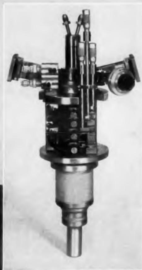
▲ Typical of a family of high-power klystrons under development is this 1-KW CW power output tube (solenoid and cover removed) which tunes over a 1000 mc range at X-band, with 40 db gain. All tubes in this family are of rugged, metal-ceramic construction to meet performance standards of military specifications, and employ an extremely long-life, single-knob tuner. Other designs include high-power tubes for L, S and X bands.
