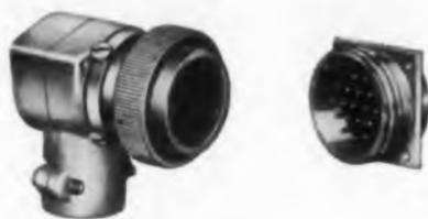
Standard K and RK...in straight and angle 90° plugs, wall mounting receptacles. Conduit and clamp entry types. 1 to 82 contacts in 213 different insert arrangements. 10-, 15-, 30-, 40-, 60-, 80-, 115-, and 200-amp. silver-plated brass contacts. High quality phenolic, melamine, and formica insulators. Cadmium-plated aluminum alloy shells. Flashover voltages: 1100 to 5000v 60cps ac rms.
