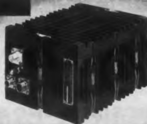
Weighing only 12 pounds , Crosley Command Receivers direct destruction of off-course missiles, control drone recovery.
