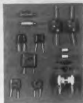
Fig. 2. Discriminator Micro-Module (right) contains the same number of components shown at the left.
