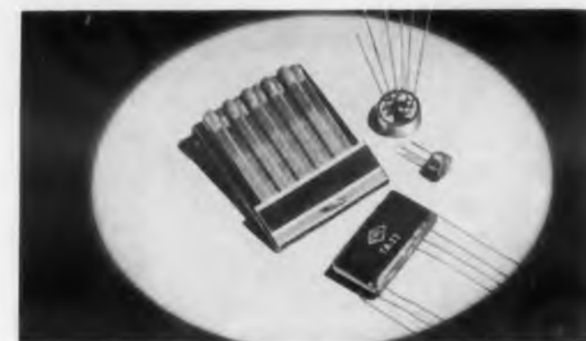
Fig. 23. Centralab's four-stage transistor amplifier, below, compared to wafer-type assembly of the same circuit, top. Single stage amplifier made by layering techniques is at the right.
