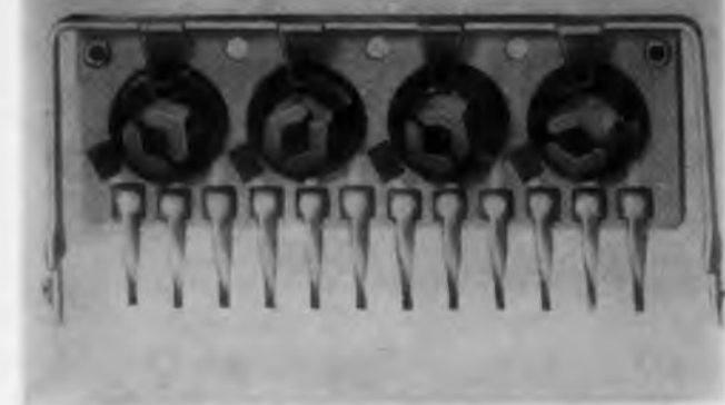
Fig. 21. Miniature variable resistors. This Centralab plate is 2-1/4 in. long. Capacitors and fixed resistors may be screened on the other side.
