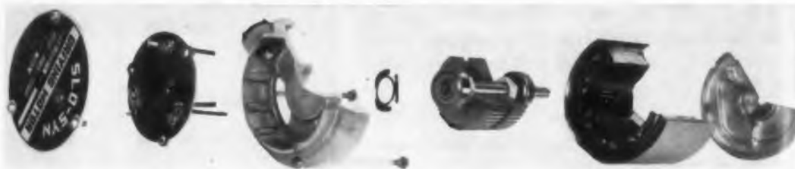
Fig. 1. This exploded view shows the various parts of the synchronous motor. No lubrication of the bearings is required for the life of the motor since the shaft is mounted on two prelubricated ball bearings.
