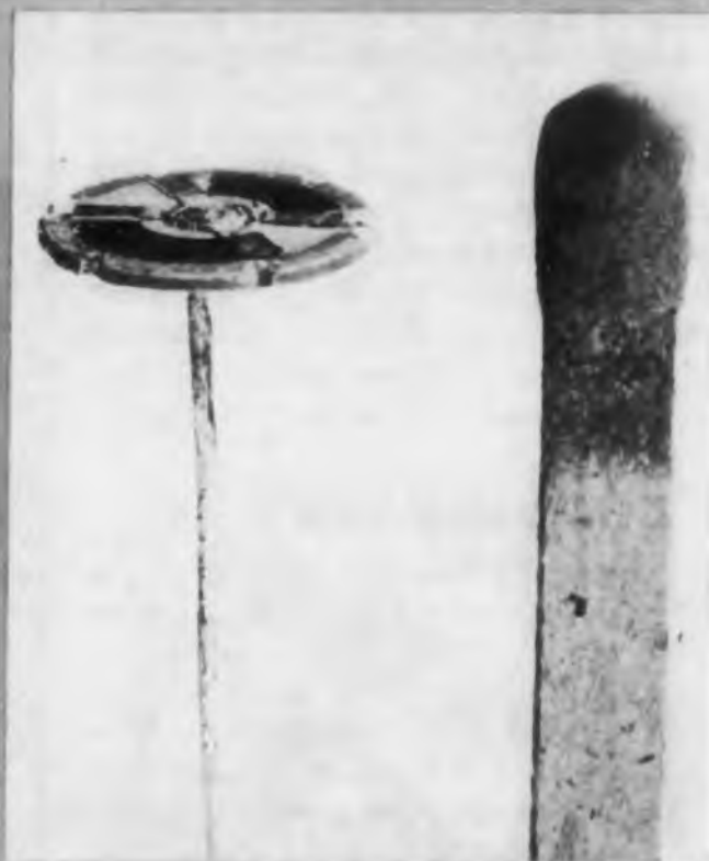
Fig. 18. Passive elements of a multivibrator circuit made by vacuum deposition techniques.
