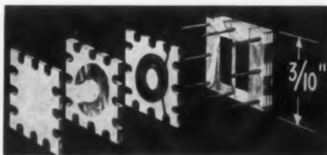
Fig. 10. Possible method of mounting a toroid on a micro-module wafer.
