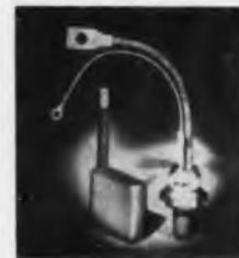
There are 8 models in the C50 group of silicon controlled rectifiers, with average forward current ratings up to 70 amp max ac, and 110 amp max dc. Peak reverse voltage ratings range from 25 to 400 v. Typical gate current is 15 ma at 1.5 v; maximum gate voltage is 3.0 v. Depending on the use, typical turn-on time is 1.0 to 4.5  $\mu$ sec; typical turn-off time is 15 to 25  $\mu$ sec.
