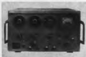
A decade-pulse generator, the GO 1005 can be used for determining transmission characteristics and transient response of amplifiers and networks, or for testing frequency and amplitude limits of electronic counters. It provides positive or negative, single or double rectangular pulses of up to 100 v amplitude at prf from 10 cps to 1 mc. Signal delay and pulse duration ranges are 250  $\mu$ sec to 100 msec.
