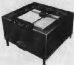
This 30 x 30-in. X-Y plotter is accurate to 0.05% of full scale and repeats exactly from any direction. No servo mechanisms are used in the solid-state plotter. Input can be from IBM cards, punched paper tape, or keyboard. Slewing speed is up to 20 in. per sec. Printing head contains 12 symbols, any of which can be selected at will; other print sectors can be added to plot digital or symbol information.
