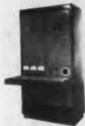
A tool for determining the response characteristics of control, structural, and servo systems, as well as electrical networks, the model OF-3 transfer function analyzer uses a cross-spectral density technique. It operates with driving signals that are random or complex periodic, obtains the causal relationship between two signals, and gives the output as Nyquist or Bode plots. It is applicable to vibration, acoustic, servo, human response and related fields.
