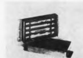
This summary network is in effect a distributed constant delay line and is designed to withstand 100-g shock. It has a total delay time of 1.6  $\mu$ sec  $\pm$ 0.026 and a tap delay of 0.8  $\mu$ sec  $\pm$ 0.013. Impedance is 600 ohms  $\pm$ 10% and operational temperatures are from -65 to +165 F.
