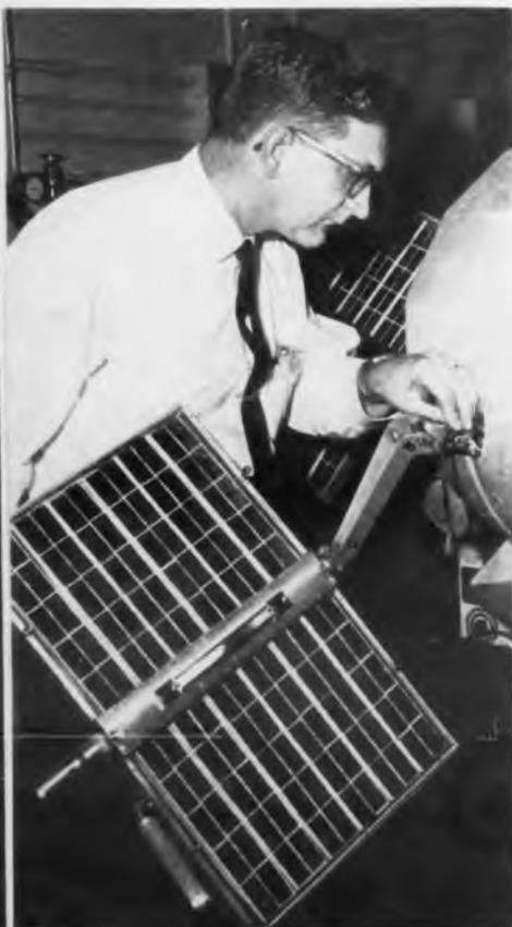
**Fig. 7.** Wires connecting one of the four solar cell "paddles" to the interior of Pioneer V are checked before launching. Each paddle carries 600 Hoffman Electronic Corp. solar cells on each side. White stripes between cells are painted on the assembly to maintain proper temperature.
