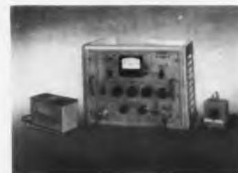
This coil tester measures the number of turns on coils with 0.1% accuracy. It measures number of turns on coils without a core and on coils wound on open ferromagnetic cores protruding from the coil. It detects short-circuited turns equal to one turn of number 25 AWG copper wire and checks for the correct amount of short-circuited layers used for time delay on relays.
