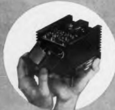
All solid state — zener diode reference; transistor amplifiers and regulator
