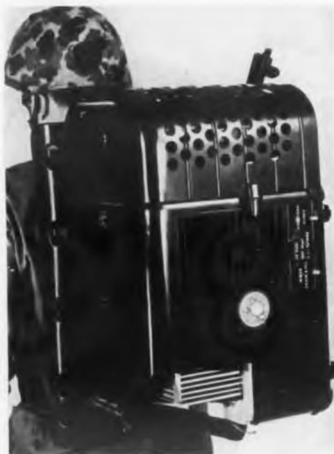
**Fig. 8.** Producing 200 w at 24-v output, the 30-lb fuel-cell power pack can take the place of a 55-lb engine-generator or 80 lb of secondary batteries. Built by GE for the Marine Corps and the Army Signal Corps, the unit contains 30 ion-membrane fuel cells consuming oxygen from the air and hydrogen produced by decomposition of metal hydride. The metal hydride is contained in reusable, hermetically sealed canisters (at top of unit); a canister weighs 6 lb and provides 14 hrs operation.
