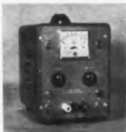
Model L3501 power supply is a portable, transistorized unit which measures 6 x 8 x 8 in. Rating is 0 to 35 v at 0 to 1 amp dc. Regulation is 2 mv per 10% line input change and 5 mv from no load to full load. Ripple is held to 250  $\mu$ v rms. Parts and workmanship are guaranteed for 2 yr for 24 hr continuous duty, without derating.
