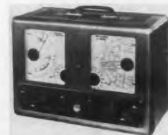
The model 6016 sweep generator has a frequency range of 4 to 250 mc, with continuous tuning. Frequency modulation is 50 cps. Frequency rise is adjustable in 6 steps, 1 to 30 mc. The built-in quartz crystal oscillator has a frequency of 5.5 mc. The 33-lb unit is 17 x 13 x 9 in., and operates from 110/220 v, 40 to 60 cps, 55 w.
