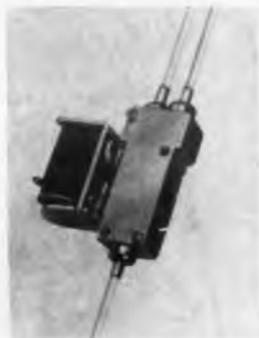
Series RB coaxial relays have a crosstalk rating of 40 db min, 0 to 470 mc; vswr is less than 1.2, 0 to 1,000 mc. Antenna transfer rating is 150 w max. Series includes units of 1-w and 2-w ratings, for ambient temperatures of 25 C, 80 C, and 125 C. Coil voltages are 6, 12, 24/26.5, 48, and 115 v. The 3-oz unit has maximum dimensions of 2-1/8 x 1-7/8 x 45/64 in.
