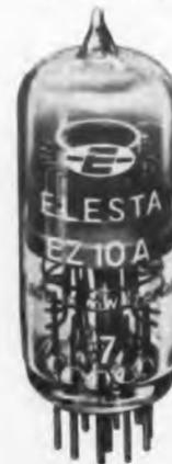
**A** RECENT Swiss development is an electronic decade counter tube capable of counting rates ranging from 200,000 to 1,000,000 pps. Manufactured by Elesta A. G., Bad Ragaz (SG), Switzerland, the tube features a non-symmetrical cathode arrangement. Further, the tube is said to be very small in size, with low current consumption and no tube heating problems.
