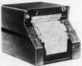
The Model 1108 Visicorder, with many automatic features and the convenience of pushbutton controls, is ideal for intermediate uses requiring up to 24 channels of data.
