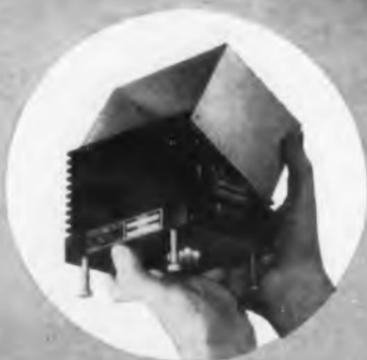
One piece finned aluminum extrusion, achieving high heat dissipation. Most units need no external heat sink to 55° C ambient.
