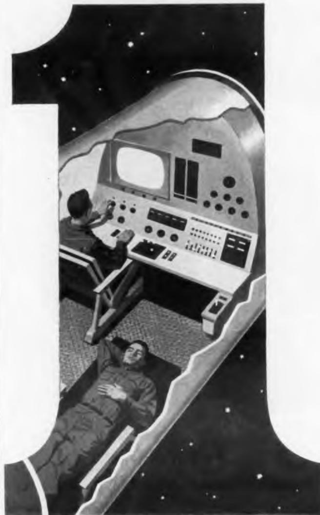
This is the FIRST Space Cabin Simulator used by the Air Force School of Space Medicine to successfully confine 2 men for a 30 day period in a simulated space condition. The creation of this device was the result of the combined efforts of Honeywell's Manned Systems Engineering Section and is one of the many examples of Honeywell's unique capabilities in the fields of environmental control and space technology.
