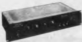
The model N-804 timer measures preset and elapsed time with a 60-cycle controlled time base. Maximum time storage is 10,000 sec. Time readout is by four glow transfer tubes. Time resolution is to the nearest second on times longer than 1,000 sec. The unit may be used with any electronically gated scaler as well as with scalers which are stopped and started with mechanical contact closures.
