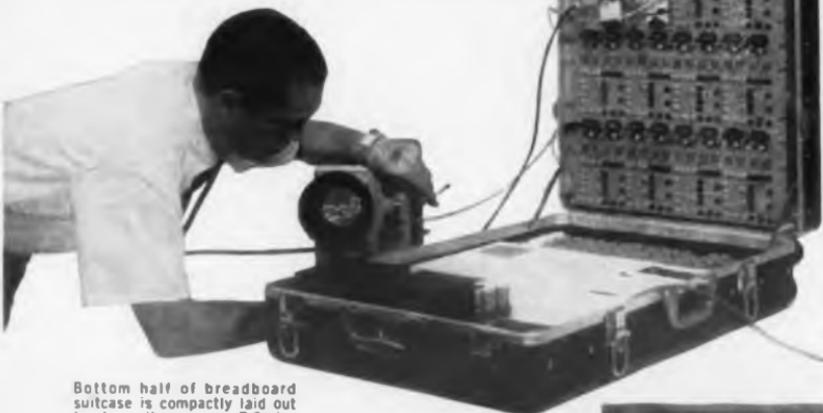
Bottom half of breadboard suitcase is compactly laid out to store all necessary T-Series circuit modules, circuit cards, patch cords, and compatible power supplies.
