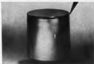
Small, solid state, direct-coupled DC amplifier weighs only six ounces. Less than five cubic inches in volume, this rugged, hermetically sealed instrument is available with solder, plug-in, coax or combination header arrangements and a variety of mountings. DC gain is 200 to 1000  $\pm 0.75\%$ . Input capability is 5 millivolts differential at maximum gain; output capability is  $\pm 5$  volts into not less than 20K (single-ended).
