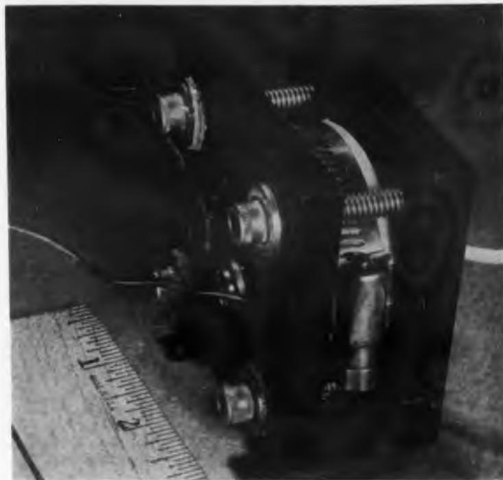
**Fig. 9.** Experimental model of a lightweight regenerative fuel cell under development by Electro-Optical Systems, Inc.
