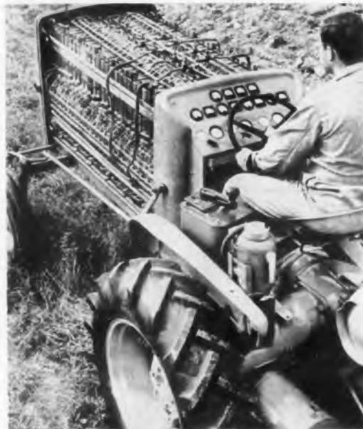
**Fig. 6.** A dramatic example of a fuel-cell application is Allis-Chalmers Research Div.'s tractor demonstration. A total of 1,008 fuel cells, 112 units of nine cells each, are arranged in four banks which can be connected in various series-parallel groups. A mixture of gases is fed through a tubing system under pressure and produces 15-kw output during reaction in an electrolyte. Sufficient output is obtained to drive the 5,270-lb tractor and provide 3,000-lb drawbar pull.
