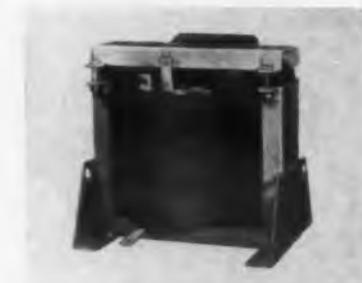
Magnetic amplifiers in 7 sizes, from 75 hp to 400 hp, in the Mega-Power 1310 series are recommended for uses requiring controlled dc power for variable-speed dc motor drives. The static devices are said to offer more compactness and reliability, longer life and less maintenance than conventional motor-generator power supplies.
