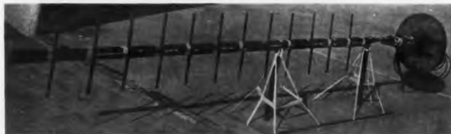
Fig. 3. Experimental end-fire radiator consisting of dipoles which are individually fed.
