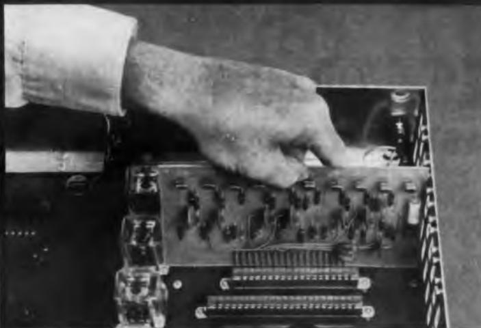
**4** **"NO-NEEDLESS-NINES" LOGIC** in Series 30 results from a new concept in transistor logic which eliminates unnecessary, time-consuming cycling of stepping switches through their 9's and 0's positions. This increases accuracy, speed, reliability and usefulness, particularly in systems applications.
