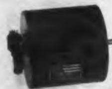
This photo transducer incrementally converts shaft angle to digital measurement information. Maximum speed varies from 15,000 rpm at 128 counts per revolution to 1,250 rpm at 2,048 counts. It provides sampling rates up to 45,000 counts per sec. Output is 12 v at 1 ma; maximum operating temperature is 55 C. The 19-oz unit is 4.68 in. long over-all, with OD from 2.75 to 3.5 in.
