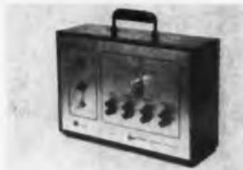
Model 401 is a completely transistorized dc absolute voltage-current source. It has voltage accuracy of 0.0075% and an absolute current accuracy of 0.025%. Stability for voltage outputs is 0.003%; for current outputs it is 0.005%. All outputs are short-circuit-proof.
