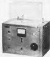
New materials testing AC HYPOT® meets ASTM dielectric strength test requirements. Features automatic rate of test voltage rise, transparent test cage that is safety interlocked and complete line of plug-in materials testing fixtures. Write for new bulletin... "HYPOT® Insulation Tester"
