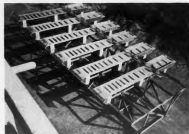
Fig. 4. Linear Yagis array of end-fire elements. Vertical dimension is within 0.3 wavelength of the lowest frequency.
