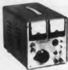
The model 4025 power supply delivers 0 to 150 v ac or 0 to 200 v dc at 4 and 3 amp respectively. The unit has transformer isolation from line voltage, an output impedance of 15 ohms, a recovery time of 30 msec for half-current step changes, and dual 3-1/2-in. meters. It weighs 35 lb and measures 8 in. wide, 9 in. high and 12 in. deep.
