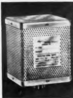
The model TR-30-100, a transistorized, voltage-regulated dc variable power supply, provides 0 to 25 v dc from input of 105 to 125 v, 50 to 60 cps. Output current is 0 to 100 ma; regulation is 0.5%, line and load. Ripple is 0.1% or 25 mv max. The supply plugs into an octal socket. Weight is 2 lb 2 oz; dimensions are 3-1/4 x 3-3/8 x 4-1/4-in. high.
