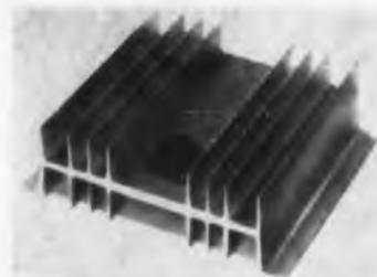
Designed for transistors and diodes where 200-w or more dissipation is needed, the 4AL series heat radiators also function as a chassis. With very low thermal resistance and high radiation capability, efficiency approaches that of an infinite heat sink. Width is 4-1/2 in., length up to 12 ft in 1/2 in. increments. Height is 1.03 in.
