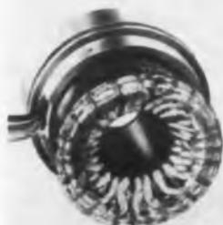
Designed for both low-impedance transistor and medium-impedance cathode-ray tube applications, the series Y58 is available with deflection angles of 52, 70, and 90 deg and fits all 1-1/2-in. neck diameter cathode-ray tubes including 70 deg flat types. The stator type of core permits small effective flux area in relation to inside diameter. Impedances from 0.1 mh to 60 mh may be obtained.
