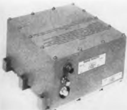
**Transistorized** vehicle pulse-beacon transponder, designed by ACF Electronics Div., provides VERLORT radar with pulsed-signals for tracking. Superheterodyne-type receiver used has sensitivity of  $-70$  dbm, stability of  $+3$  mc between 0 and 70 C, and an image rejection greater than 45 dbm.
