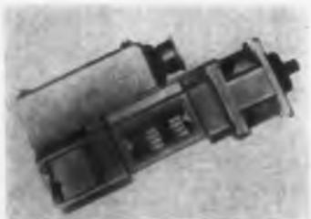
Weighing 4.7 lb with radio noise filter, the model 2030 dc motor produces 0.33 hp at 14,000 rpm, continuous duty, and 0.62 hp at 8,750 rpm, intermittent duty. The 26-v dc unit is 7.48 in. long by 2.44 in. wide. An integral clutch-brake provides fast stopping and irreversibility in power-off condition, and holds 3 in.-lb torque with the motor de-energized. The square-frame motor is rated to 260 F, altitude to 150,000 ft.
