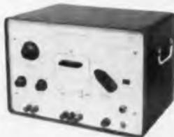
Covering the frequency range of .001 to 10 cycles per second, waveforms are programmed by shaped cams. In addition to the selected function, a square wave at the same frequency is also produced. Function derived can modulate a 60 cycle or other frequency carrier to yield a suppressed-carrier waveform useful in servo testing.
