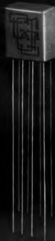
This hermetically sealed relay—no bigger than a postage stamp—is a precise component of unusual flexibility, capable of long-life operation under a wide variety of contact loads.
