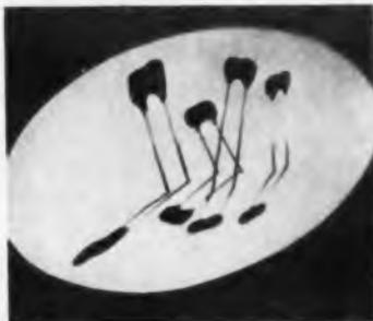
Types CD15, CD19, CD20 and CD30 dipped-silver mica capacitors cover the capacitance range from 1 to 40,000 pf. Standard ratings are 500, 300 and 100 wvdc. Capacitance tolerances are from  $\pm 10\%$  to  $\pm 1/2\%$ . The line meets MIL-C-5B (proposed) specifications. Models for operation up to 2,500 wvdc at 10,000 pf are also available.
