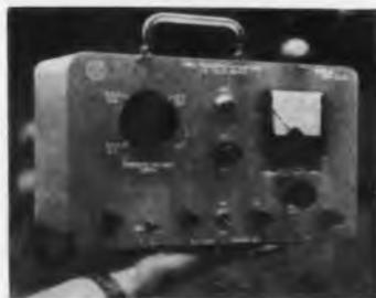
Two dc power supplies are combined in an 8-1/4-lb package. One supply delivers 2, 6 and 12 v dc, selectable; the other 1 to 30 v dc, variable. Outputs may be used separately or simultaneously. Power sources may be 115 v ac, 50 to 2,000 cps or aircraft or marine ac/dc, 20 to 35 v. Transistor circuitry is used throughout.
