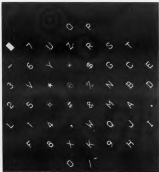
Glass aperture plate used in the Datascope character generator contains 64 characters. The center of each character is lined up with the optical centerline to an associated photocell.
