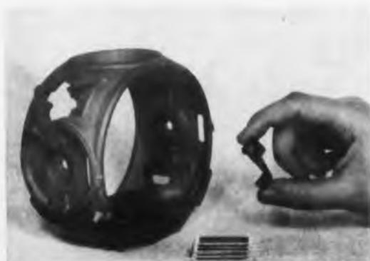
A gyroscope component cast in 17-4-PH steel is shown in comparison to an ordinary sized investment casting.
