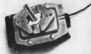
Model EB-3 electric thermostat is designed for domestic electric oven applications. It is a double-pole, snap-action, single-circuit unit rated for 25 amp at 250 v ac. The hydraulically operated control incorporates the firm's diastat.
