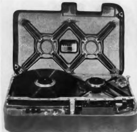
Fig. 3. Flangeless reeling system in this airborne recorder cuts size, increases tape capacity, and improves environmental immunity.
