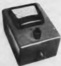
These rf power meters, of the absorption type, operate in the range of 100 kc to 200 mc. Power is measured in 2 to 6 ranges from 1.5 w full scale to 1,500 w full scale, at an accuracy of  $\pm 5\%$ . A resistive voltage divider is used. Meter calibration may be checked against dc or 60 cps.
