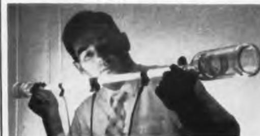
Continuously operating IR maser tube is inspected by a Bell Telephone Laboratories scientist, Donald Herriott. Tube contains helium-neon mixture at low pressure, pumped by rf discharge. Light emanating from tube is the normal neon glow and does not indicate the extremely directional IR beam that exits from the ends of the tube.
