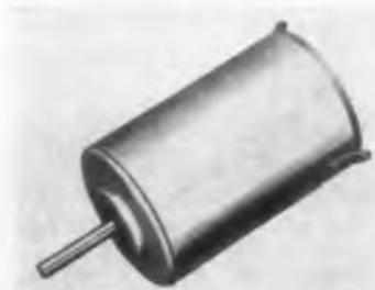
A 1-in. diam, battery-powered dc motor, the HYQM operates from 4.5 to 30 v dc. Governed versions are made, with speeds from 1,500 to 5,000 rpm; the ungoverned motor has a torque of 0.5 oz-in. at 10,700 rpm. Efficiency is 57%; stall torque is 2.3 oz-in. Rotation may be clockwise or counter-clockwise. Motors are rated to 200 F.
