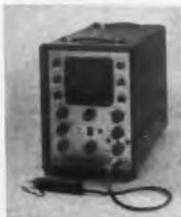
Designed for laboratory use, the GM 5603 oscilloscope has differential vertical input, bandwidth dc to 15 mc. Sensitivity ranges from 50 mv per cm to 5 v per cm, accurate to  $\pm 3\%$ . Time base is 40  $\mu$ sec per cm to 1 sec per cm, in 21 steps, accurate to  $\pm 3\%$ . Magnifications of 2x and 5x are provided. The 13-cm flat-faced cathode-ray tube has an accelerating voltage of 10 kv.
