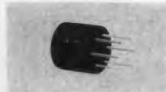
This pulse transformer operates in a blocking oscillator circuit and includes the use of a high-quality ceramic ferrite cup core. Its rugged encapsulated construction enables its use in salt atmosphere marine applications.
