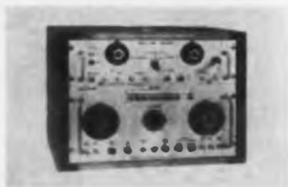
The model SP 160 test set, for determining vswr and attenuation values of rf components or circuits, operates over a frequency range of 200 to 475 mc. In conjunction with a dual-trace oscilloscope, it provides instantaneous readings of vswr or attenuation for the device under test. The generator section has a response that is flat within 5% over its maximum sweep width, an output of more than 0.75 v into 50 ohms, and is equipped with a variable frequency marker.
