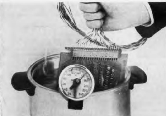
**7** **"NO POTS AT ALL" STABILITY** of the NLS V44 DVM is checked by the "boil in oil" test at 158°F. This feature eliminates all trimming of decade and amplifier circuits.
