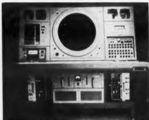
**Control panel** (lower right hand side of display tube) of Tasker Corp.'s PAR Display Console contains controls for both FPN-16, and PAR-1 radar. Vacant spaces in upper right hand section will contain speakers used in pilot-to-controller voice communication. Empty slots on each side of horizontal shelf are for head-phone plug-in jacks.
