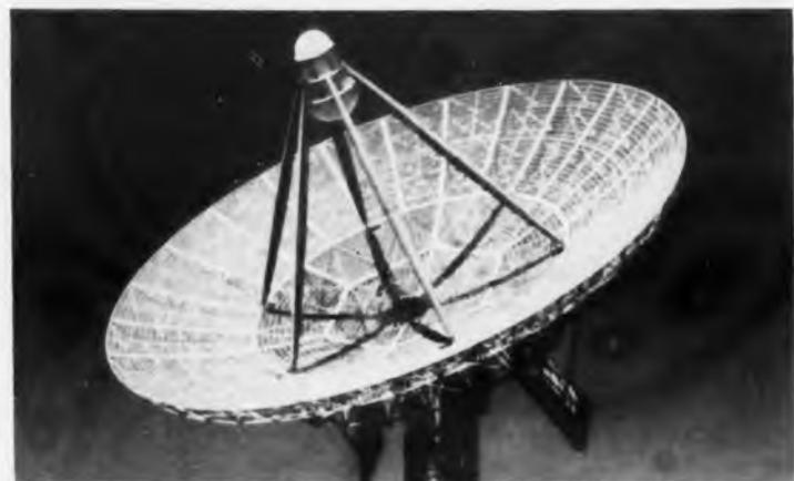
**Sixty-ft dish** for receiving telemetered rf data is part of the automatic-tracking subsystem with 1,500-nautical-mile range. Dish has 7.6-deg conical scan and scan frequency of 10 cps. It can track and slew to 10 deg per sec and accelerate to 5 deg per sec. Crystal-controlled receiver used, which incorporates phase-lock detection system, has 7-db noise figure and gain of  $118.5 \pm 3$  db.
