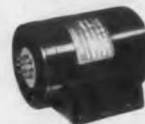
Where output on only one axis is required, and unlimited rotation is not required, the model 1G01 dc integrating rate gyro will replace a free gyro. Potentiometer output indicates displacement within 5% of actual position when displaced at a rate of 10 deg per sec over a range of  $+60$  deg,  $-40$  deg. Weight is 18 oz. The unit will withstand temperatures from  $-65$  F to 186 F, unlimited altitude, shock of 20 g and acceleration of 40 g on any axis.
