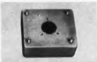
This series of lumped constant delay lines consists of m-derived LC networks. Each section is designed to give linear phase shift beyond 70% of the cut-off frequency. Attenuation is less than 1 db per  $\mu$ sec of delay. Specifications for model DL-2265 are: impedance, 500 ohms  $\pm 5\%$ ; delay time, 1  $\mu$ sec  $\pm 5\%$ ; rise time 0.08  $\mu$ sec; attenuation, 1 db max.
