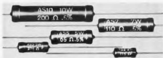
New Thermacoat resistors expand circuit design limits significantly by carrying full power even at 125°C ambients. These resistors meet MIL Characteristic V (MIL-R-26C) with an allowable 350°C hot spot, well above the 250-275° customary for resistors of this type.
