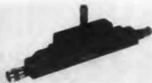
This modified version of the model AU-10 can withstand 100 w of cw power for 24 hours with no change in performance characteristics. Insertion loss is zero. The device provides up to 60 db of attenuation in the 300 mc to 5 Gc range.
