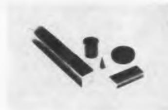
This absorbing plastic, called Microloss, can be used from -70 C to +150 C without deterioration. It may be easily worked into medium power attenuators, mode absorbing rings, etc. It will not support fungus growth. The plastic is available in 12-in. rod lengths, round or rectangular.
