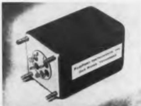
This line of dc-to-dc converters has regulated voltage outputs that range from 700 to 1,500 v and the rated current output is 20  $\mu$ a. Each unit is hermetically sealed. Size is 2-3/8-in. high x 1-1/2-in. sq. They are available with plug-in base or solder connections.
