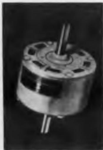
These 2-, 4- and 6-pole shaded pole and 6-pole split capacitor motors are available in ratings from 1/150 hp at 3,000 rpm to 1/3 hp at 1,075 rpm. They can be wound for 115-v, 208-v, or 230-v operation at 50 or 60 cps, and can be engineered for single or double shafts, thermal protectors, special mounting rings, terminals or other features to fit individual motor package needs.
