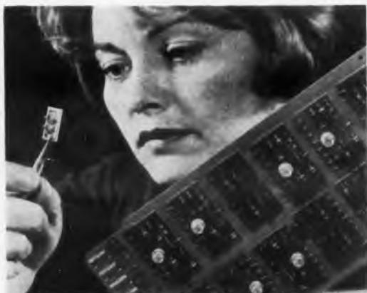
Tiny germanium tunnel diode wafer (upper left) is a part of basic circuitry designed by Radio Corp. of America, Camden, N. J., as the first step toward an ultra-swift electronic computer under the Navy-sponsored Project Lightning. Electronic switching speed is 0.25 nsec. Four of the midget units will perform the same job as the circuit board (center), but 1,000 times faster.
