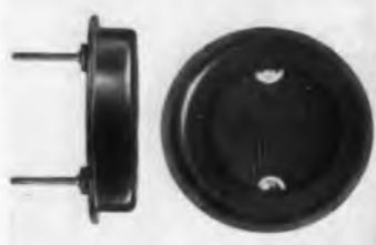
Model CDS-9 cadmium photocell has a resistance of over 1 meg in darkness and has a broad response to visible light. At 1 to 50 ft-c it will permit direct control of a relay requiring as much as 10 ma for operation. Power dissipation is  $1/2$  w continuous, 2 w for 1 min. It is non-polar and may be used for ac or dc, max voltage is 500 v dc or 350 v ac rms.
