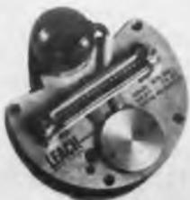
With a diameter of 3-5/8 in. and a length of 3-1/8 in., the model 362 tape recorder will record in 7 or 14 channels on 75 ft of tape. It withstands: vibration of 15 g, 10 to 2,000 cps; shock of 2,000 g for 3 msec on any axis; acceleration of 400 g continuously. The 26-oz unit has a temperature range from -50 to 180 F. Tape speed may be 3-3/4, 7-1/2, 15, or 30 in. per sec; wow and flutter are less than 1%. Power requirement is 24 v dc at 1-amp start and less than 500-ma run.
