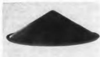
These conical, fiber glass covers, called Para-Dome, are designed to withstand a wind force of 50 lb per sq ft. Signal attenuation between 2,000 and 6,200 mc is less than 0.1 db. Standard models cover reflectors of 4, 6, 8 and 10 ft.
