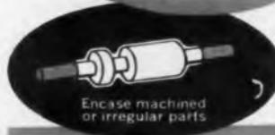
PF expands tubing mechanically to a much larger diameter. In use, tubing is positioned and heated to gel point. On cooling, it recovers its original diameter, shrinking to form a tight fit over the part it encloses.
