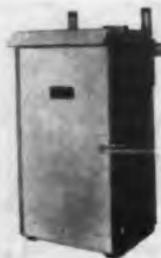
The model 600 pole-mounted air dryer will deliver 600 standard cu ft of dry air per day at pressures from 0 to 15 psig. The fully automatic unit, encased in an aluminum cabinet, operates within an ambient temperature range of -40 F to 120 F. Compression, cooling, and desiccation will reduce the relative humidity of hot air from 100% to less than 2% at 70 F.
