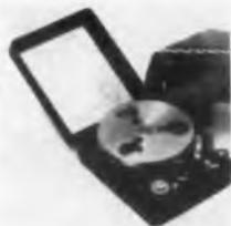
Model PS-303M magnetic tape recorder measures 2 x 4 x 5 in. and weighs 31 oz including 7 oz of tape. It will record dynamic data from 100 to 5,000 cps. It requires 3/4 w of power, supplied by standard mercury cells. Frequency response is flat within  $\pm 3$  db from 100 to 5,000 cps and signal-to-noise ratio is better than 30 db. It will record for 1 hr at 1-7/8-ips speed.
