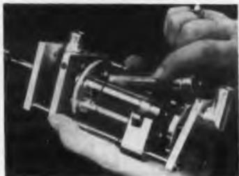
These step-type turret attenuators permit quick change of db combinations. The removal of 3 set screws allows pad retainer ring to move forward for easy replacement, removal, or rearrangement of pads. Turrets are available in any combination of values from 0.1 db through 60 db, in 0.1-db increments.
