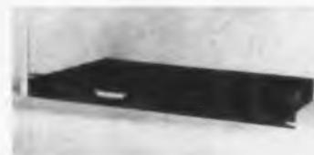
A rack-mounted dc power supply, the 3210-R is 1-3/4-in. high. Output voltage is continuously adjustable from 0 to 32 v; current, from 0.1 amp to 1.25 amp. An automatic limiter maintains load current at the preset level. Ripple is less than 1 mv rms; regulation is better than  $\pm 0.1\%$ , or 5 mv, for load or line change. Input is 105 to 125 v, 400 cps. Depth is 10 in.
