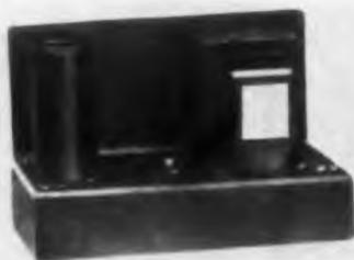
A regulated power supply module, the model P-30-1 has an input of 115 v rms  $\pm 10\%$ , 1 phase, 55 to 400 cps. Output may be 12 to 20 v at 0 to 1 amp, or 26 to 30 v at 0 to 1 amp, or 10 to 33 v at 0 to 0.75 amp. Load regulation is  $\pm 0.05\%$ , zero to full load; line regulation is  $\pm 0.05\%$  for 105 to 125 v line. Ripple is 3 mv peak-to-peak max, and recovery time is 50  $\mu$ sec. As many as 10 units may be connected in series. The unit weighs 4-1/2 lb and measures 8 x 5 x 3-1/4 in.
