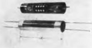
A mechanical filter designed for mobile radio equipment, the F455YA-120 has a 455-ke center frequency and a passband of 12 ke to match a  $\pm 5$ -ke transmitter deviation. Another filter, the F455YA-320, with a 455-ke center frequency and a 32-ke passband, is suited for wide-band mobile equipment applications.
