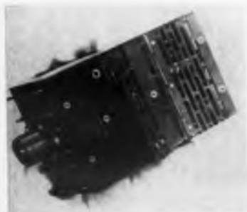
Model 90-156-0 solid-state inverter weighs 3.7 lb and occupies less than 65 cu in. of space. It operates on an input of nominal 28 v dc with an output of 115 v, 400 cps, sine wave, single phase, 100 va. Output frequency is factory adjusted to 400 cps  $\pm 0.5\%$ ; stability is  $\pm 0.25\%$  from  $-60$  to  $+71$  C. Distortion of the sine-wave output is less than 4% under all operating conditions.
