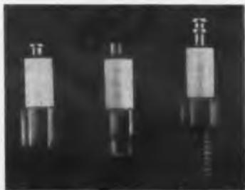
The bodies of these stand-off insulators are made of Teflon; turrets are machined from brass rod. The units are unaffected by humidity, mechanical shock and vibration, and are designed for ambient temperatures from  $-110$  F to 500 F, pressure altitudes from 0 to 80,000 ft.
