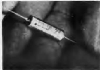
These subminiature Teflon capacitors, developed for missile guidance systems, have temperature coefficients from 0 to 120 ppm per deg C. Tolerances to 0.1% are available. These units have the self-healing characteristics of metallized film capacitors.
