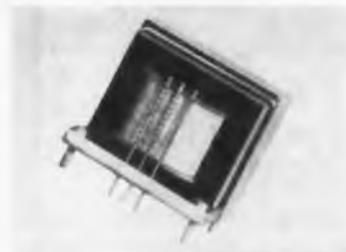
Series C custom designed transformers have a can size only slightly larger than the core itself. Extended-pin terminal design eliminates internal flex leads and exposes magnet wire and pin-solder connections for continuous inspection.
