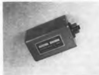
Thermostatically controlled oven, model 1206, has internal temperature stability of  $\pm 0.5 \text{ C}$  at 70 C over an ambient range from 0 to 50 C. It is for housing crystals, filters and other circuitry requiring temperature stabilization. Specifications are: power supply, 24 v dc; external dimensions, 2-in. sq x 3-1/2 in.; weight, 7 oz.
