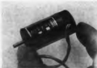
A permanent-magnet dc motor, model PM-1 is suitable for military and commercial uses. With efficiencies to 54% through high-flux utilization, the motor requires very low current at full load. Weight is less than 2 oz; length is 2 in., OD 7/8 in. Motor operates from -55 to +100 C, under vibration, shock and acceleration satisfying military specifications. Voltage range is 3 to 30 v dc.
