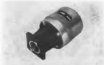
Explosionproof magnetic tachometer pickup model 2040 produces high-amplitude, low-modulation sine wave signals proportional to speed. Standard frequencies are 60 or 120 impulses per revolution, adaptable to a range of 1 to 240 impulses per revolution. Speed range is 75 to 10,000 rpm; output is more than 1 v rms at 100 rpm. Weight is 2-1/2 lb.
