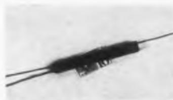
Encased in a 13 32-in. diam tube, these distributed constant delay lines have an impedance of 500 ohms. Delay times are 0.05 to 1.0  $\mu$ sec, with rise times from 50 to 120 nsec. Operating temperature is from -55 to +125 C.
