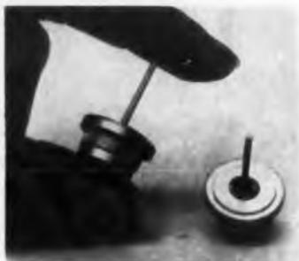
Low cost of the MR322 diffused-junction silicon rectifier enables wide application. Rated at 18 amp, unit operates at case temperatures from -65 to +175 C. Welded case of 5/8-in. OD is designed for press-fit mounting.
