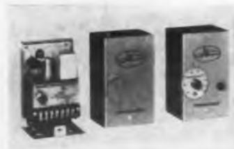
Series 7000 electronic temperature controls are available in ranges from  $-300$  to  $+2,000$  F. Standard range is 0 to 800 F. A special plug-in "anticipator" actuates the relay by anticipating, on a proportional basis, the actual set-point, either high or low. The control circuit is encapsulated in epoxy.
