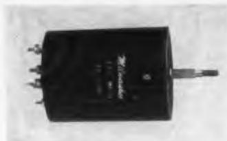
Enclosed, dustproof power rheostat is readily adaptable to any linkage for either manual or automatic operation. Design allows operation at full power rating with as little as 25% of the winding in use. The unit is available with standard or tapered windings in ratings of 100, 200 and 300 w. Center tap is optional.
