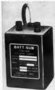
Constant voltage supply, model BS(TC)-2 can substitute for dry and wet cells for use with precision laboratory potentiometers such as the L&N types K2 and K3 and the Rubicon types B and S. Voltage stability is better than 0.01 per cent for 10 per cent variations in 117 v line. Over 15 C to 35 C temperature range, stability is 0.001 per cent per deg C.
