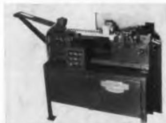
This machine soft-solders the ends of caps to fuse links at the rate of 3,000 fuses per hour. After soldering by induction heating, fuses are sized to uniform length and tested for continuity. A circuit is provided to feed all fuses on the belt after shut-off, so that no unsoldered fuses will leave the machine.
