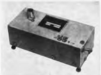
Accurate, stable cw signal for tracking of missiles or vehicles is provided by the TT-1001 Mod 7 uhf telemetering transmitter. Frequency is 225 to 245 mc. Accuracy and stability are better than 0.01%; power output is 260 mw. Silicon transistors are used throughout. Weight is 17 oz with battery, 6.5 oz without. Battery life is 1 hour min.
