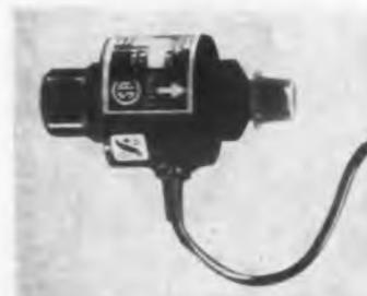
Service to 200 psi is provided by solenoid valve for use in fluid control. Available in standard ac and dc voltages, the valve operates in any position with a maximum rate of 1,000 cycles per min at 100 psi. Temperature range is  $-65$  to  $+350$  F. The 5-oz valve measures 2-5/8 in. long with a diameter of 1-3/8 in. Inlet connection is 1/2 in., outlet 1/8 in.
