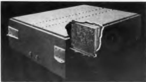
Assembly frame will hold 8 to 10 boards. A central duct in the computer will allow free air flow through the assembly frame slots and over the flat circuit surfaces, carrying away heat.
