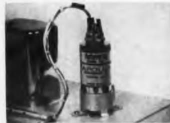
An electro-optical system is used to perform the modulation in the "Autoverter" microvolt modulator. A power source capable of 200 v dc delivering 200 ma is the only requirement to drive the unit. Two 5-v square wave outputs have less than 2- $\mu$ v rms noise level with 2- $\mu$ v zero offset. Weight is less than 3.3 oz.
