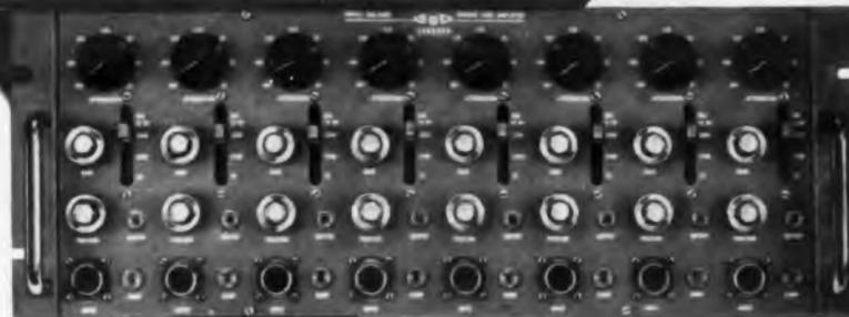
COMPACT 7" HIGH 8-CHANNEL UNITS ARE COMPLETELY TRANSISTORIZED, HAVE FLOATING INPUT ISOLATED FROM OUTPUT
