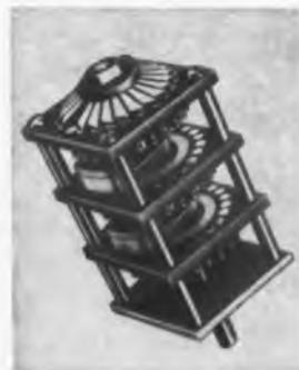
Progressive shorting-type switches have separate collector-ring connection for complete or continuous programming. Switches, which can be ganged, come in a 1-3/4 in. sq for 20 and 24 positions, and in a 2-1/4 in. sq for 24 and 32 positions.
