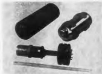
A wide range of crystals is accommodated by the RD-135 mercury thermal switch crystal oven. Useful in low-frequency applications, oven takes crystals up to 1-3/8 in. long. Temperature control is  $\pm 0.005$  C at fixed room ambient, and  $\pm 0.025$  C from 0 to 60 C. Weight is 7 oz, size 5-3/16 by 1-3/4 in. OD. Unit meets military shock and vibration tests.
