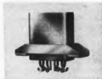
Rated at 10 amp. Designed for space environment, series 200 relay is hermetically sealed and resists moisture and temperature extremes. It withstands shock and acceleration of 50 g, and vibration of 30 g up to 2 kc. Life exceeds 150,000 operations at 10 amp, 26.5 v dc or 115 v ac, at 125 C. The 2.5-oz relay measures 1 x 0.6 x 1.25 in.
