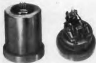
Absolute, gage or differential pressures of corrosive or noncorrosive gases or liquids in the 0 to 5 and 0 to 500 psi full-scale range can be measured by pressure transducer TP-200. Standard performance data includes the ability to withstand shock of 75 g; a static error band, including independent linearity, hysteresis, repeatability, resolution and friction, of  $\pm 2.5\%$  in the 0 to 5 to 0 to 10 psi range and  $\pm 1.5\%$  in the 0 to 15 to 0 to 100 psi range.
