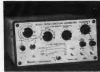
Triple-function type LRG 051 produces these synchronously initiated output waveforms: positive 100-v sawtooth, positive 10-v pulse and positive 10-v pulse delayable within the duration of the sawtooth. Operation can be triggered or gated from an external waveform.
