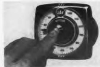
Push-button actuated impulse counter has an automatic reset which counts at a rate up to 500 counts per minute. The start button is integral with the count-setting knob. Four standard counting ranges are available: 1 to 120; 2 to 240; 4 to 480, and 8 to 960.
