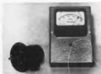
Complete tachometer indicator systems use permanent-magnet, instrument-type, dc generators with precision indicating meters to show speed of motor rotation. Various circuit arrangements are available to provide for expanded or suppressed speed scales and automatic selection of speed scale for either direction of rotation.
