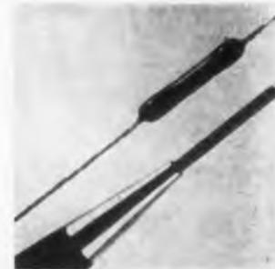
Vitreous-enameled, wirebound 1-w resistors are made in axial-lead configuration. Length is 9/16 in. max, diameter 1/8 in. max. The resistor shows stability under constant full load, low noise, long life and good overload capability. Resistance range is 1 to 6,000 ohms, tolerance  $\pm 5\%$ .
