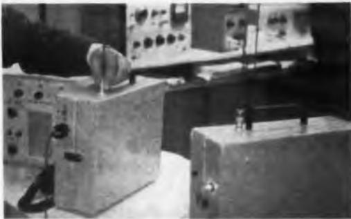
**Test model of RACEP** random-access, discrete-address communications system consists of encoder-decoder for addressing, left; transmitter, center, and receiver, right. System is said to be capable of supporting up to 700 users on 4 mc.
