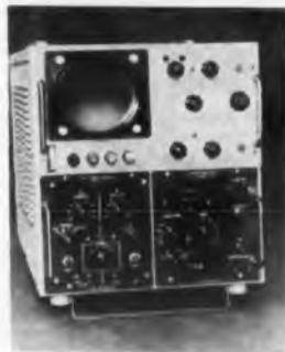
Bandwidth of dc to 70 mc is provided by the LA-270 oscilloscope. Designed to military specifications, unit has 6-cm vertical deflection. Display size is 6 x 10 cm. Single and dual channel plug-in vertical pre-amplifiers and plug-in sweep delays are used. Horizontal sweep circuitry has 24 calibrated ranges with 10X magnifier extending the fastest sweep to 0.01  $\mu$ sec per cm.
