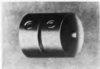
Designed for light duty electromechanical applications, these zero backlash flexible couplings employ torsion spring elements to cushion starting and braking loads. Shaft to shaft misalignment may be up to 5 deg angular and 1/32-in. parallel offset.
