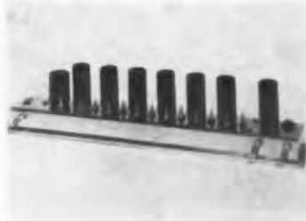
Wide-band IF amplifier model IF301 has a detector and a cathode follower for video output. Typical noise figure at 30 mc is 1.5 db, input vswr less than 2:1. Standard 30 or 60 mc models have 90-db gain, 10-mc bandwidth, and 50-ohm input.
