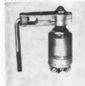
High-temperature, hermetically sealed switch uses a rotary linkage actuator for positive operation regardless of dust or ice conditions. Lever can be adjusted through 360 deg. Rating is 2 amp inductive, 28 v dc and 1 amp inductive, 115 v, 60 or 400 cps. Temperature range is -65 to 600 F.
