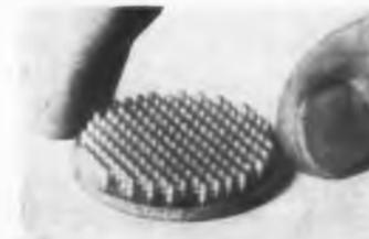
Miniature terminal boards on 0.100 grid patterns, in any shape, are available with glass-filled epoxy, melamine or silicone insulation. The terminals are brass, phosphor bronze or beryllium copper and are silver or silver and gold plated. Terminals measure 0.062-in. OD x 0.026-in. ID; height above board is 0.156 in. and they are bifurcated with slots 0.025-in. wide x 0.068-in. deep.
