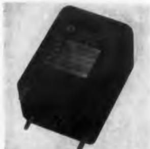
A frequency-to-voltage converter, the IIP Magacycler produces an output voltage or current directly proportional to input frequency or pulse rate. Full scale outputs range to 10 v with accuracy of  $\pm 1/2\%$ . Standard units cover the audio range from 5 cps to 12 kc, with up to 100 kc on request. Internal impedance is low. The converter meets military requirements. Can size is 3-1/8 x 2-5/16 x 2-5/16 in.
