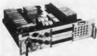
For PAM or PDM standard IRIG and nonstandard inputs, type 3201 operates with pulse repetition frequencies of 75 to 2,700 pps. It has automatic drift and gain correction. Fingertip selection of 10 from up to 99 channels is possible.
