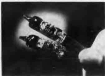
Subminiature frame-grid tubes CK 7994 and CK 7995 are housed in T-3 button envelopes with nominal outside dimensions of 0.375 by 1.25 in. The CK 7994 is a high-frequency, grounded-grid triode, designed for use in wide-band amplifier stages and grounded-grid amplifier applications. With a ratio of 15 ma plate current to 18,000  $\mu$ mhos  $g_m$ , the tube has a plate-to-cathode and heater capacitance of 0.25 pf.
