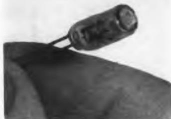
Similar to the human eye in its sensitivity variation with the color temperature of light sources, this cell measures light accurately, whether the light is tungsten or daylight or whether the color temperature is 2,700 or 6,500 K. A footcandle meter incorporating the cell needs no correction filter.
