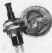
Normally open, spdt push-on, pull-off switch No. 30-16 has a positive detent action. Life expectancy is over 100,000 cycles. Contact rating is 1 amp, 115 v resistive, contact resistance 0.010 ohm. Base and button are molded phenolic.
