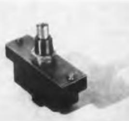
Snap action limit switch is designed to bridge the gap between the very small and larger, enclosed limit switches. Ratings are as follows: ac, 40-amp make, 15-amp break; dc, 2-amp make and break on single throw forms with 0.040-in. gap.
