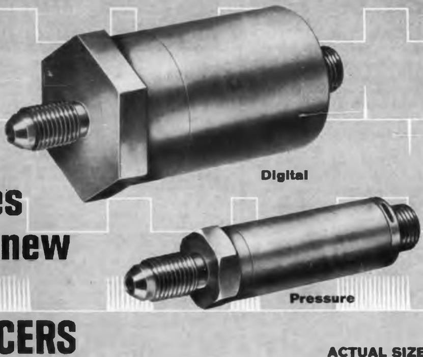
DeJur Digital Transducers are self-contained solid state miniaturized packages designed to measure various parameters (pressure, temperature, flow, acceleration) and supply a digital signal output without the use of auxiliary equipment. The result can be a pulse duration type (PDM) digital signal whose pulse width in time is directly proportional to the amplitude of the input parameter being measured. PPM and PFM outputs also can be made available.
