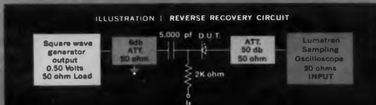
**ELECTRICAL CHARACTERISTICS** Forward currents range from about 1 to 25 mA at one volt while reverse currents range from 15 to 500uA at 50 volts. Peak inverse voltages range from 50 to over 150 volts. The diode capacity is generally less than 1 pf. Frequency response is about 100 mc. The diode operates efficiently within the range from -55°C to +90°C.
