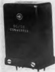
Designed for use with "Nixie" indicator tubes, models VC 12-170 and VC 28-170 have an output of 170 v dc from 12 and 28 v dc respectively. Full load current is 30 ma for each, enough to power 10 "Nixies."
