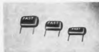
Designed for rapid insertion in printed-circuit boards, series F207 capacitors have right-angle leads. These double-dipped, Mylar film capacitors are available in capacities of 0.01 through 1.0 µf, with ratings of 200, 400 and 600 v dc.
