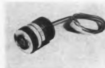
With increments of 15 and 7.5 deg and rates of 200 to 550 steps per sec, these motors work in conjunction with a logic circuit which controls rate, sequence and direction. They may be driven by electromechanical or electronic logic.
