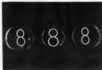
New design of Nixie tubes provides flattened tube face and cutaway anode to permit higher positioning of the cathode numerals. Viewing angle is increased from 90 to 160 deg. Life is 200,000 hr. Type B5092 replaces B5031; type B6091 replaces B6033. A completely new large tube is also offered.
