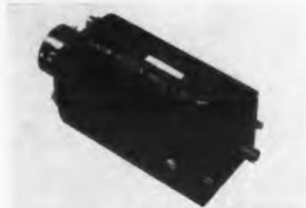
This positive-indexing synchro transmitter has 48 positive detents at 72 deg intervals on the input shaft. The transmitter is electrically zeroed on the 5th detent. The package is 1-17/64 in. sq x 2-1/2 in. long; it weighs 3-1/2 oz.
