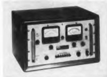
Fm-monitor deviation calibrator, "Monocal 500", provides better than 0.5% deviation accuracy. It combines the functions of five instruments previously needed to determine the peak deviation of an fm signal by the carrier drop-out method. It can be used directly with any fm monitor tuning to 12 mc. Deviation ranges are: 10-, 30-, 100-, and 300-kc peak.
