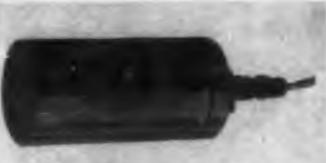
Magnetic anomalies of 0.1 gamma or less are detected and relayed in digital or analog form by this instrument. The continuous output is sufficient to drive telemetry systems or recorders. The unit is 7 in. long x 3 in. in diameter. Power consumption is 0.8 w at 200 ma.
