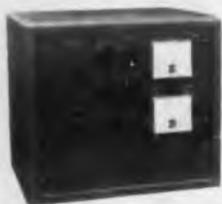
Forward and reverse dc characteristics of diodes and rectifiers are measured by model 1808 diode test set. The forward current supply is metered and adjustable from 50  $\mu$ a to 3 amp. The forward voltage is measured in three ranges of 1, 3, and 10 v full scale. Reverse voltage is metered and adjustable from 0.5 to 2,000 v. Reverse currents from less than 1 na to 3 ma are read directly.
