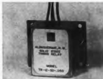
Solid-state timing relay, for pulse or squib applications, can turn on a 50-amp load within 10  $\mu$ sec of the application of a short, low-energy, voltage trigger having an amplitude of  $+17 \pm 11$  v. The relay, model TR-12-50-050, operating from a 12 v dc source, shuts off the load after 50 msec.
