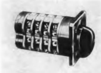
Modular-constructed types C-25 and C-40 are for power switching and motor control. Type C-25 is for 25 hp at 600 v, three-phase; type C-40 is for 40 hp. Each stage has two isolated double-break, silver alloy contacts, up to 24 contacts can be provided.
