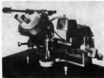
Thermocompression wire bonder model 402 is capable of bonding a wire 0.0002 in. in diameter to a transistor stripe measuring 0.001 x 0.003 in. Developed for making mesa transistors, the bonder can be used in the production of other transistors and diodes. Precision controls allow manual positioning accuracy of 10 to 15 millionths of an inch.
