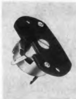
Preset and variable, type INS-110 has a mounting plate to insulate the control. It is for hot-chassis or other potentiometer uses and can be furnished with a molded shaft. Diameter is 3/4 in. Rating is 1-1/4 w at 40 C, derated to no load at 105 C.
