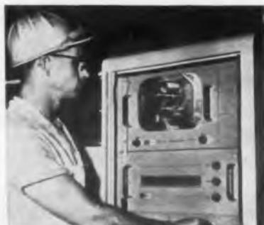
For example: American Potash and Chemical (above) monitors conveyor line and warehousing operations with a KIN TEL TV system.
