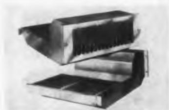
Two-speed blower for electronic racks is designed to provide greater air turbulence over the entire rack interior. Output of the 19-in. unit is 500 cfm. Various rack depths are available. Washable filter can be serviced without removing the blower.
