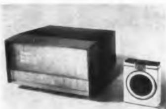
With a conversion rate of 0.5  $\mu$ sec, analog-to-digital converter model 101 has accuracy of  $\pm 0.5\%$ ,  $\pm 1/2$  least significant digit. Input amplitude is 10 v at impedance of 250 ohms. Visual display is 2 binary-coded decimals. Size is 6-1/2 x 3-1/2 x 6-1/4 in.
