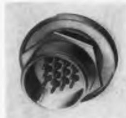
This compression-sealed unit has a normal leakage rate of less than  $10^{-7}$  cc per sec, with rates of  $10^{-9}$  cc per sec available on special order. Bodies and pins are fused with glass, meeting MIL-C-5015 specifications. Various contact arrangements with 12 to 32 pins are available. Unit mates with any standard MS socket.
