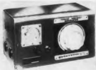
This variable-voltage power supply has an output from 0 to 140 v ac with regulation of  $\pm 6\%$  at 75 w. Maximum no-load output is 142 v rms. Front panel meter reads 0 to 150 v with 1% full scale accuracy. Unit measures 9-3/8 x 4-7/8 x 5-1/2 in.
