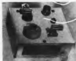
Miniature cavity amplifiers, series 20, are entirely gold-plated and designed for heat sink type mounting and operation. Frequency range covered is 215 to 2,325 mc. All units can be used as building blocks stacked side by side on 4 surfaces.
