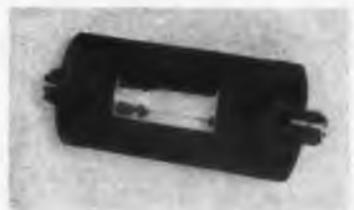
Broad-band ferrite coaxial isolator C992-100-409 operates from 2 to 4 Gc. Bandwidth isolation is 15 db, insertion loss 1 db, vswr less than 1.25:1. The 2-lb isolator is 6.16 in. long. Type N female coaxial connectors are standard, with other types optional.
