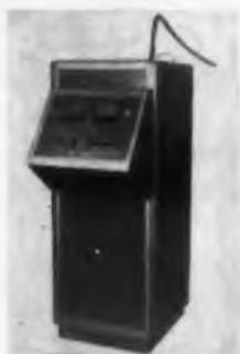
Rated at 100 kv, 10 ma, continuous duty. Model 5492 power supply has a highly regulated output, automatic rate of voltage rise and is short-circuit proof. Provisions are made for remote control operation and remote metering. Plug-in shielded cable is used for connections.
