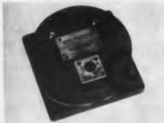
Resolution is 0.01% of full scale. The AA series angular accelerometers for sensing roll, pitch and yaw cover from 0.5 to 500 radians per sec<sup>2</sup> in five models. They can be used with carrier amplifiers or 400-cps power systems and are suitable for missile instrumentation and control.
