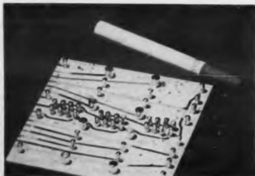
**Beryllium oxide board** 3-in. square by 0.06-in. thick was used for the thermal link between the modules and the heat sink which would be clamped on one edge. Kovar studs were weld points for the module leads of nickel-plated copper.
