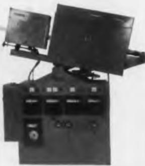
Diffusion furnace used in semiconductor manufacturing, developed by BTU Engineering Corporation, Waltham, Mass. The Stepless Control designed around the General Electric SCR has no moving parts, does not deteriorate with age. It is also fail safe. In the absence of a signal it shuts off the power.
