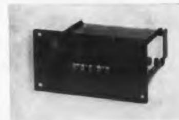
Differential pulse counter F 160 has separate coils for addition and subtraction. Simultaneous add and subtract commands are accepted without error. Count rate is 25 per sec max. Front plate size of the five-digit counter is 2 x 3-3/4 in.
