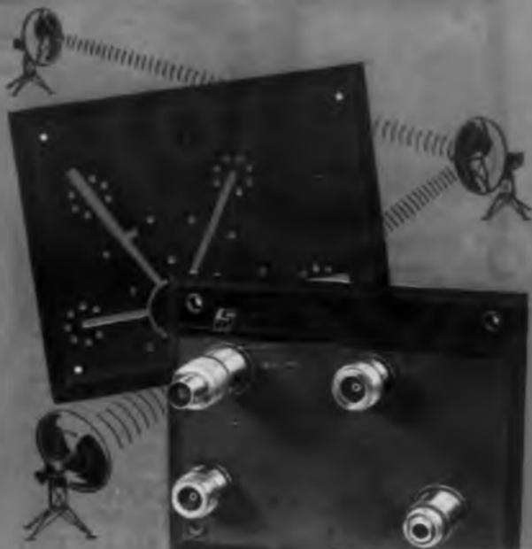
Impedance-matched Greomar RF adapters combining small size, and low VSWR provide reliable, efficient transitions from strip transmission line components to coaxial cable. Typical is the Sanders Associates TRI-PLATE® hybrid mixer shown above.
