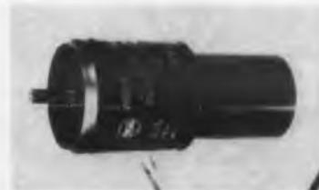
Designed for missile use, this 6-pole, 400-cps, size 15 servo motor offers the following characteristics: theoretical acceleration at stall, 22,700 radians per sec<sup>2</sup>; minimum power output, 1.151 w; input power at stall, 6.1 w; motor dampening, 130 dyne-cm per sec.
