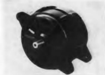
Semiconductor voltage regulation, holding the output to  $\pm 2\%$  from 1,000 to 12,000 rpm, is provided by these alternators. Two types are offered: 15 v dc, 1,000 w; 100 v dc, 1,500 w. Construction features radially oriented ceramic magnets in the rotor.
