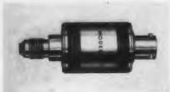
High-range absolute pressure transducer 737 meets government specs in miniature size. Ranges from 0 to 4,000 up to 0 to 10,000 psi are made, with resolution to 0.2%, resistances 1 K to 10 K  $\pm 5\%$ .
