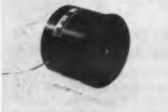
Delivers 140 cfm of air against a static pressure of 5 in. of water at 25,000 ft. Sea level output is 77 cfm against 5 in. of water. No pressure-sensing or speed-regulating switches are needed in the system. Motor is wound for 200 v ac, 400 cps, three phase.
