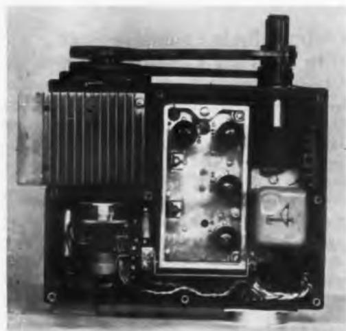
**Interior of camera.** Left to right: aperture and focus controls, 10-mc video preamp strip, and vidicon tube enclosed within the thermoelectric coolers.
