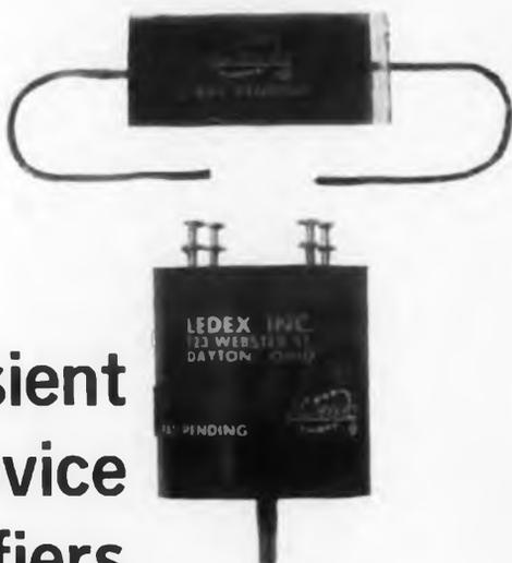
**H**IGH-VOLTAGE transients, appearing across power supplies when an inductive load is suddenly turned off, can be effectively reduced by a newly developed gas-tube device. Conventional means to avoid rectifier burnout include the use of relatively expensive, high piv diodes or Zener devices.
