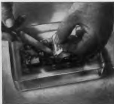
LTV-602 is easy to work with and easy to repair. To repair parts embedded in LTV, merely cut out and remove section of material, repair or replace defective part, pour fresh LTV into opening and cure. Pot life, with catalyst added, is approximately 8 hours and may be extended with refrigeration. When desirable, LTV may also be cured at room temperature.
