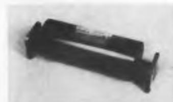
Broad-band ferrite load isolators in five models cover spans between 2.60 and 12.4 Gc. Insertion loss of the type 101 units is 1 db max, isolation 20 to 40 db min. They are designed for use with medium-power equipment.
