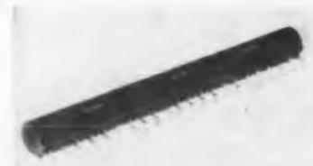
**Lug-type resistor networks** are made in lengths to 6 in., with up to 13 resistors. Values can be matched to 0.005%; individual tolerances are 0.01%. Values range from 1 ohm to 2 meg, with ratings to 3 w and 1 kv.
