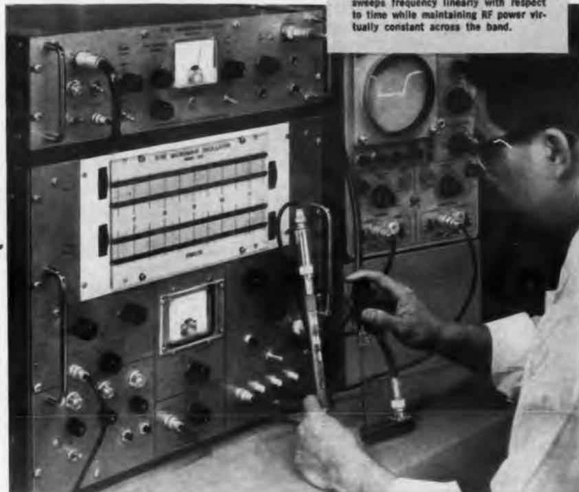
Testing insertion characteristics of X-band filter with Alfred Sweep Generator which consists of Alfred Microwave Oscillator and Alfred Microwave Leveler. This combination electronically sweeps frequency linearly with respect to time while maintaining RF power virtually constant across the band.
