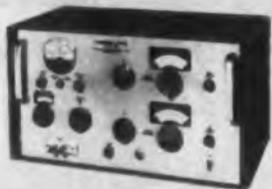
Designed for 400 to 20,000 cps operation, this inductance bridge is basically a calibrated variable frequency oscillator coupled to a modified Maxwell bridge. The bridge, model 63B, provides direct-reading calibration of both the inductance and resistance dials, with a resolution of 0.01%. Inductance range is  $0.02 \mu\text{h}$  to 1h; resistance range, 0.002 ohm to 110 K. Accuracy is about 0.25%.
