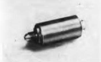
Miniature, low-pressure transducer, model L-96, has less than 1% error at vibration levels exceeding 35 g. Available in 0 to 10 to 0 to 350 psi absolute or gage pressure ranges. Performance is said to be unaffected by temperature variations. The unit weighs 4 oz and measures 1 in. in diameter and 2 in. long.
