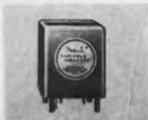
For low audio range. Miniature saturable-core reactor model EL-215 operates at 1 w from 30 to 450 cps min, and 250 to 3,750 cps max. Used to determine frequencies in filter and oscillator circuits, it is effective as a low-frequency sweeping device. The potted unit operates in temperatures from  $-55$  to  $+85$  C.
