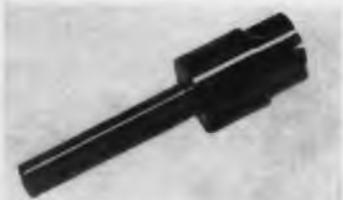
Available in 1/8, 3/16, and 1/4 in. shaft sizes, these precision shaft extensions have male and female ends in the same or any combination of these sizes. Length of extension is 1-5/8 in. Diameters are concentric to 0.0005 in.
