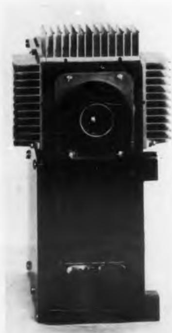
**Thermoelectrically cooled** television camera (with front cover removed). At top are the heat-radiating fins of the cooling elements, which enclose the vidicon. Motors and pulleys at the bottom control the focus and aperture of the lens.
