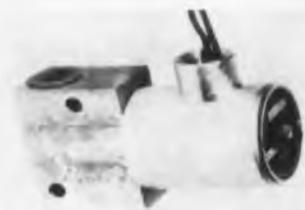
For up to 3,000-psi oil pressure, two-way solenoid valves are available in normally open and normally closed types. Both are pilot operated poppet valves in cartridge form and can adapt to any type of manifold or sub-plate. The poppet and plunger are the only moving parts.
