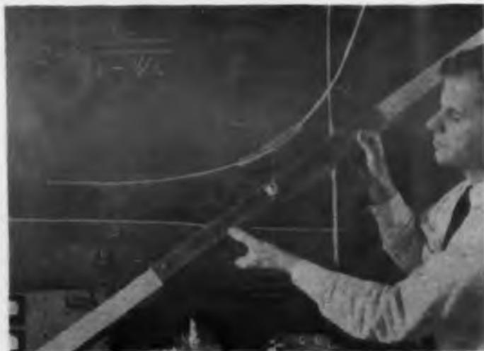
Fig. 1. Half-wave dipole parant designed for 108-mc signal. Stripline section at center connects internal pickup loop to the coax connector. Square aluminum pipe is used for outer element of the antenna.
