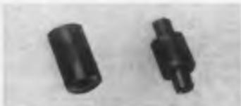
Allow 5-deg misalignment. Solid, split-hub, and combination miniature bellows couplings transmit 200 oz-in. max torque. The phosphor bronze units have zero backlash, permit 5-deg max misalignment, and 3,000 rpm max speed. Surface is palladium flash-plated.
