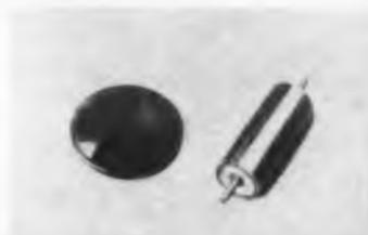
Coaxial ceramic seals for traveling-wave tubes consist of dense alumina insulator sealed to a monel inner conductor and surrounded by a nickel outer conductor. Metallization process results in good rf match characteristics.
