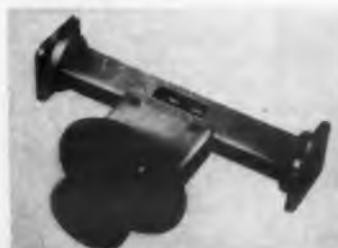
For field equipment. Type 170 series of panel-mounting attenuators is made for operation over full waveguide bandwidth, or with direct-reading dials for narrow-band use. Frequency range of type X170 is 8.5 to 10.5 Gc, with accuracy  $\pm 2$  db from 0 to 50 db. Insertion loss is 0.75 db max, vswr 1.15:1 max. Average power handling capability is 1 w, peak lower 1 kw.
