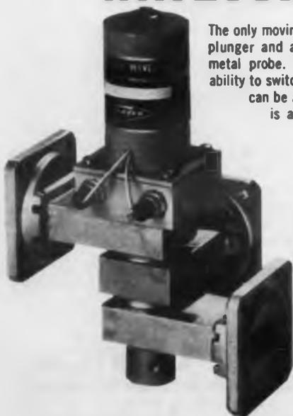
The only moving parts of the "Transprobe" are solenoid plunger and a light weight, dielectrically supported metal probe. Result... greater flexibility, longer life, ability to switch under full waveguide power. The design can be applied to any waveguide size. Unit shown is a single-pole-double-throw, X-band switch.
