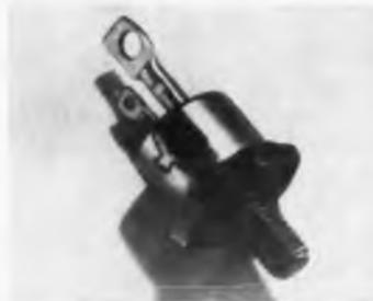
Rated at 25 amp at 100 C, diffused silicon controlled rectifiers of the TI-150 series are housed in stud package. Rated breakover voltages, both forward and reverse, are 50, 100, 200, 300, and 400 v respectively for the TI-150, 151, 152, 153, and 154.
