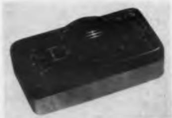
Range is 35 to -142 db; response is from 40 to 8,000 cps. Model 450 sound meter measures 2 x 3 x 6 in., weighs 2 lb and operates from a 22.5-v battery. It meets ASA Standard A, B and C weightings. The amplifier is stabilized against voltage and temperature changes.
