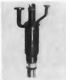
A 3-mw pulse amplifier traveling-wave tube, the VA-126 is rated at 5 kw average power. Frequency range is 5.4 to 5.9 Gc. Efficiency is 30%; gain is 35 db. The liquid-cooled unit is self-centering in its electromagnet for ease in mounting.
