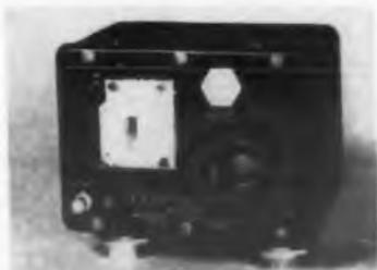
Self contained, battery operated, X-band cw crystal video receiver, model R115, employs video chopping. It is designed for direct connection to an antenna and provides a dc output proportional to the X-band signal input. Nominal sensitivity is -45 dbm.
