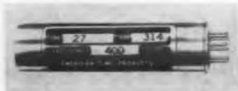
For 360 to 1,300 cps with accuracies of 0.002%. Type 27 frequency standard measures 11/16 in. in diameter and 2-15/16 in. long. It weighs 1-3/4 oz, requires 20 to 30 v dc at 5 ma and operates over a temperature range of -65 to +125 C. Vibration conditions of MIL-E-5272B Procedure II are met.
