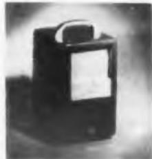
Five-ampere current recorder has better than 2% over-all accuracy, and a frequency response of 25 to 500 cps. Safe working voltage is 750 v rms, input resistance is 0.02 ohm. At standard chart speed of 1 in. per hr. paper supply lasts 31 days.
