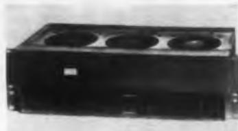
Designed to cool digital modules, particularly the firm's S-PAC series, the model CU-30 cooling unit utilizes three axial-flow fan units mounted in parallel within the chassis. It has a removable dust filter. The airduct may be adjusted to draw air from either the front or rear of the cabinet. Unit measures 19 x 5 x 8 in.
