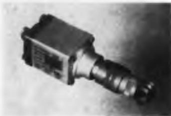
For missile applications. Type 4-328 pressure transducer operates from between 0 to 15 and 0 to 99 psia. Output is 50 mv; linearity and hysteresis are less than  $\pm 0.5\%$  of full range output. Thermal zero shift is within 0.005% per deg F. Weight is 5.5 oz.
