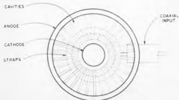
**Inverse magnetron converter** developed by Raytheon. Left to right: cathode, anode-cavity structure, coaxial rf input and cover. Final version of this device may approach 60 per cent efficiency and generate up to 1 kw cw in the 1- to 2-Gc range. Wright Air Development Div. is presently emphasizing development of this type of microwave power converter over other possible inversely operated tubes. The weight of the final version, including magnet, will be approximately 35 lb.
