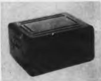
MIL-C-4150E aluminum military cases are available in 11 sizes from 18 x 21 in. to 28-1/4 x 28-1/4 in. The female closure has an environmental gasket seal. Standard equipment includes handles, latches, pressure and humidity valves and shock support cushioning. Cases meet applicable standards for temperature, humidity, fungus, salt-spray, etc.
