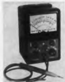
Model 222, available in both kit and wired form, measures ac and dc voltages up to 1,500 v in five ranges, and resistances of 0.2 ohms to 1,000 meg in five ranges. Input impedance is 11 meg on dc, 1 meg on ac. Voltage ranges are 0-3, 15, 75, 300, and 1,500. Response is 30 cps to 3 mc; frequencies up to 250 mc can be read with probe.
