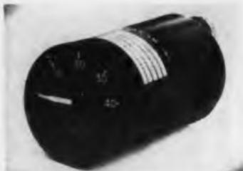
All metallic seals are used in model 8007 low pressure gage. Range of this water pressure gage is 0 to 40 in., accuracy and repeatability are  $\pm 1$  in., operating temperature is from  $-65$  F to  $185$  F and the device meets shock and vibration tests of MIL-E-5272C. Measuring 2 in in diam and 3.9 in. long, the indicator weighs 12 oz.
