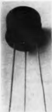
Eight models of series C5 differ by forward breakover voltages which range from 25 v for the C5U to 400 v for the C5D. Units accommodate transient PRVs up to 500 v. Average forward current rating is 1 amp dc at 82 C case temperature. Max gate current to fire is 200  $\mu$ a at 25 C.
