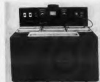
Self-contained printed-circuit console also can be used for small cleaning operations. The entire installation needs only one water, electrical and drain connection. With tanks at normal cabinet height, a typical unit occupies 6 x 4 ft of floor space.
