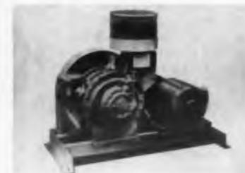
Capacities in excess of 50 cfm and pressure down to  $1 \times 10^{-4}$  mm Hg are claimed for Duo-Seal 1398. Suggested uses of this pump include electron tube evacuation, vacuum distillation and most other industrial and laboratory uses.
