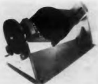
Available in two models, the No. 201 tables feature a large vernier scale on the outer axis providing setting accuracies to 0.05 deg throughout the 360 deg range. Model 201A incorporates a handwheel with a friction drive, and model 201B utilizes a servo-type worm gear drive.
