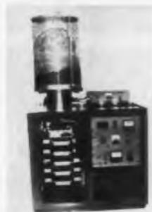
Achieves clean vacuum to  $5 \times 10^{-9}$  mm Hg in 4 hr. or less. The "Boostivac" system operates from a single electrical connection and requires no plumbing or liquid nitrogen cold traps. In operation, the equipment is said to minimize the pressure rises which normally occur when other materials are evaporated during bell jar operation.
