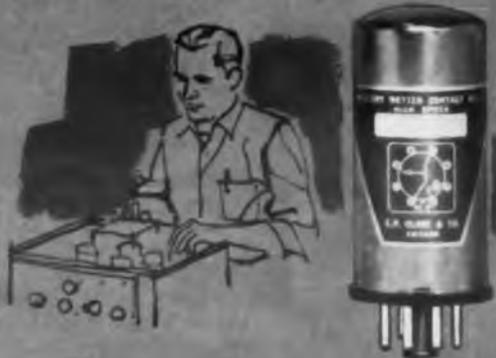
CLARE HGS switch capsules are available in single switch units, surrounded by a coil, mounted in high-melting point wax and encased in cylindrical steel containers provided with plug-in base. A smaller type (HGSS) is designed for use where space is limited. HG relays are available with one, two, three, or four capsules, surrounded by a single coil. Also with permanent magnets (HGP) for single-side stable, bi-stable or chopper operation.
