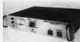
Accepts inputs of any parameter which can be reduced to a dc voltage and compares this unknown voltage to two, externally provided high and low limit references. Input impedance is 10 meg; input grid current is less than  $10^{-11}$  amp; and operating differential is 1 mv max. Sensitivity in the nulling mode is  $250 \mu\text{v}$  per meter-scale division.
