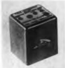
Operating at unlimited altitudes, this low-level subcarrier oscillator is designated type 1274A. Differential floating input allows operation at ground potential, at dc levels to  $\pm 50$  v from ground, or it can be left floating. Input impedance is larger than 90 K and input power for full deviation is less than 1.12 mw. Total volume is 4.5 cu in.
