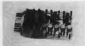
Decade counting unit is solid-state plug-in type. The DCU-100 counts at speeds of dc to over 200 kc, with less than 3 sec double pulse resolution. Units require less than 10 ma at 6 v for operation. The epoxy glass board, etched circuit has standard 0.157 in. spaced connection tabs and measures 3-3/4 x 2-1/16 x 1/2 in.
