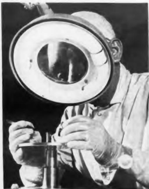
A tiny accelerometer, expected to be a key to increasing Polaris range from 1,200 to 2,500 miles, is assembled in a sterile laboratory at Sperry Gyroscope Co., Great Neck, L. I., N. Y. The company is producing sub-miniature prototype models of the new MIT-designed devices for a smaller, lighter and more accurate missile-guidance system. The accelerometers can sense and measure changes in the velocity of the missiles in flight.
