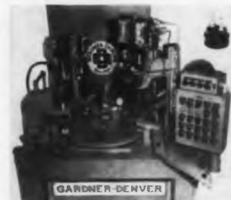
Assembles stop lamp switch contacts at the rate of 1,200 pieces per hr. Controls are completely electrical and interlocked with an air motor driven index table. The silver contact points are automatically fed and driven. These special machines are designed and built to the specifications of the individual purchaser.
