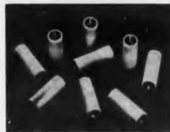
Ceramic utilized is 90-97% pure alumina. Bonding strength of the metallizing techniques used is 15-20,000 psi. Ceramic tubes can be metallized in sizes varying down to 0.080 in. ID. Ends of the tubes, which have a maximum length of approximately 8 in., can also be metallized where required.
