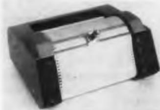
Digital high-speed plotter accommodates any analytical or discontinuous function and presents the data in graph form, for visual interpretation. Plotting is 1/100-in. increments, at speeds of 200 increments per sec, at 0.01 in. resolution. Power supply is self contained.
