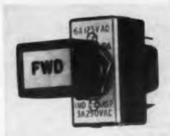
Switch ratings are 3 amp, 250 v ac and 6 amp, 125 v ac. Units are available in normally open or closed contact arrangements and feature one-hole mounting, shallow panel depth and 90 deg "snap-on-cap" orientation. Rating for removable incandescent lamps are 14 v, 0.08 amp; for integral incandescent lamps, 28 v, 0.04 amp.
