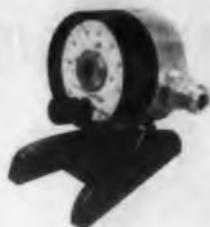
Frequency range of 0 to 3,000 mc is offered by model RT-1, variable attenuator. The accuracy of the device is  $\pm 2$  db over the entire range. Max standing-wave ratios are 1.2, input and 1.4, output. Models come in 50-, 60-, and 75-ohm impedances, with a power handling capacity of 0.5 w.
