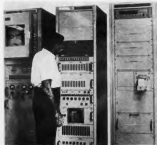
**Pulse-code-modulation** equipment is checked out at Bell Laboratories' Hillside, N. J., test site. The unit is one of three to be used in American Telephone & Telegraph Co. satellite.
