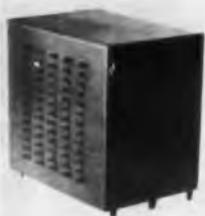
Type CTC-168 Q-Line has an 8-mc bandwidth for an overall delay of 6.3  $\mu$ sec, at an impedance level of 200 ohms. Rise time is 0.08  $\mu$ sec with a resulting delay-to-rise time ratio of 80:1. The unit has 63 taps at 0.1  $\mu$ sec intervals. Housed in a 5 x 5 x 4-in. steel case, the unit is designed to meet environmental requirements of MIL-STD-202B.
