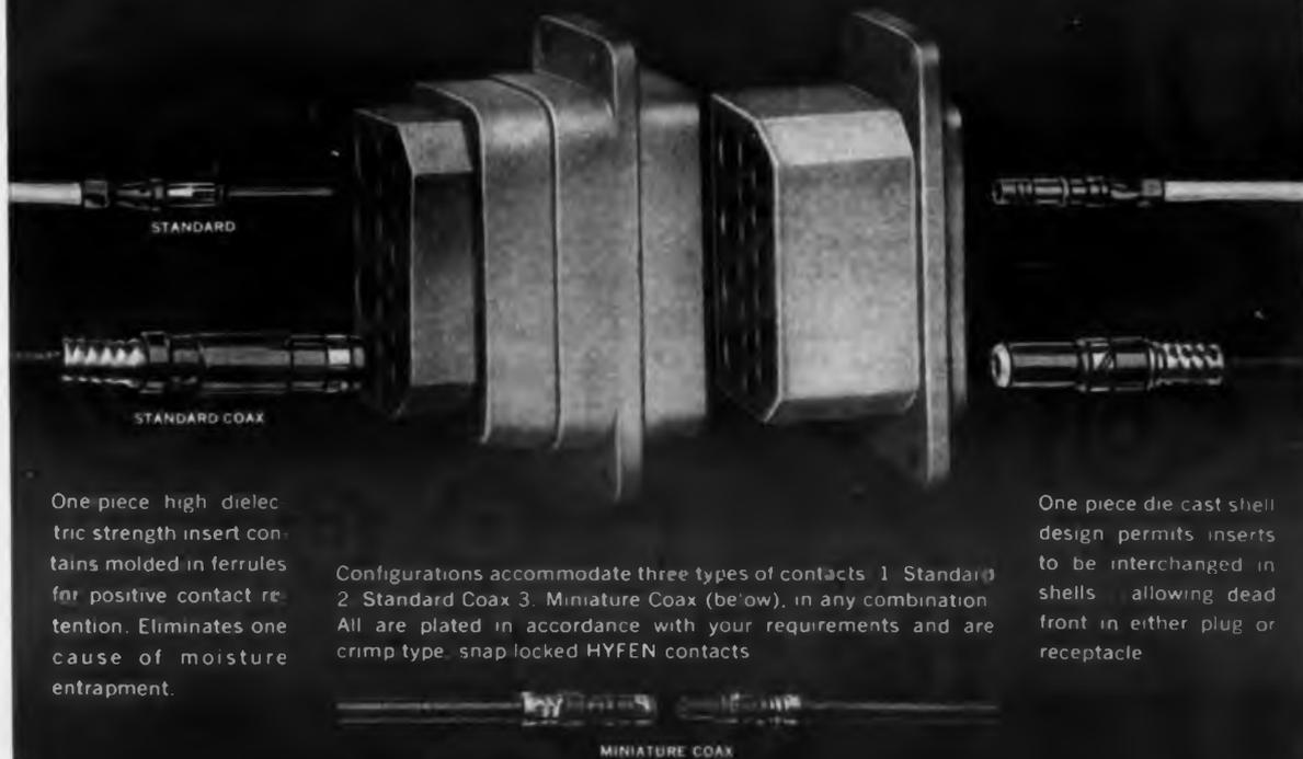
One piece high dielectric strength insert contains molded in ferrules for positive contact retention. Eliminates one cause of moisture entrapment.
