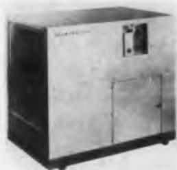
Removes moisture up to 36 gal daily. Model D20 uses 2 hp hermetic refrigerating cycle. Operating range is 50 to 110 F, with relative humidities down to 40%. Equipment includes electric humidistat, magnetic starter, freeze-stat, 12-ft, 3-wire lead, and pail compartment with 5-gal pail. Unit requires 208 or 230 v, 60 cps, or 200 or 230 v, 50 cps single-phase.
