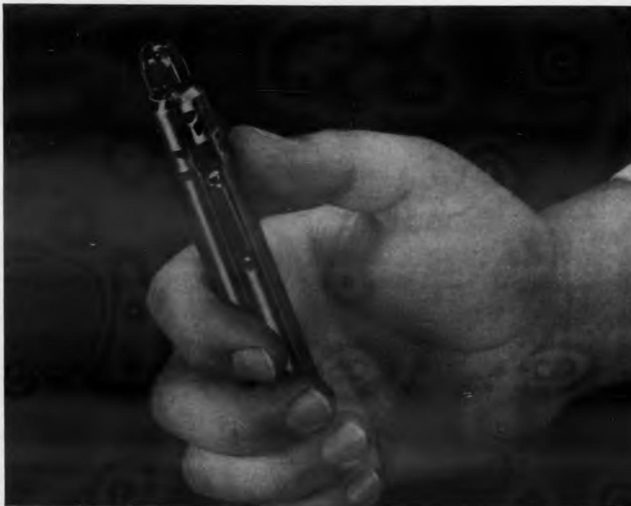
**PERSONAL RADIATION MONITOR**, developed at Oak Ridge National Laboratory, warns of radiation levels by flashing a neon lamp and sounding a tone in a hearing aid earphone. The transistorized circuit operates 24 hours a day for 30 days at a time, from power by a single Mallory TR-133R mercury battery.
