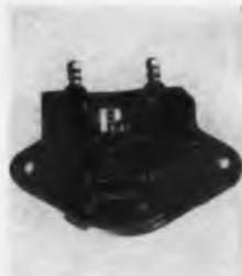
Designed as a plate-coupling or blocking oscillator transformer, this 10-kv pulse transformer is for pulse widths up to 1  $\mu$ sec. Maximum voltage rating is 400 v with interwinding insulation capable of withstanding 10 kv, max. Rise times of less than 0.04  $\mu$ sec are typical. The transformer meets all the specifications of MIL-T-2103A, grade 5, class T, life X.
