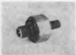
Piezoelectric accelerometer weighs 4.5 g. Model AK106 features a natural frequency of 60 kc and operates over a range of  $\pm 10,000$  g. Encased in a stainless steel case, the unit operates at temperatures between  $-65$  and  $+250$  F.
