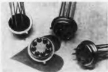
Up to 13 separate leads can be accommodated in a closure conforming to the basic TO-5 transistor configuration. Leads may be grounded or ungrounded, depending on design requirements. Measuring no more than 0.300 in. in body diam, and 0.100 in. high, the header can be supplied with electrically isolated flat forms or "islands" with a common body. Multiple lead configurations in TO-18 and TO-46 packages can also be furnished.
