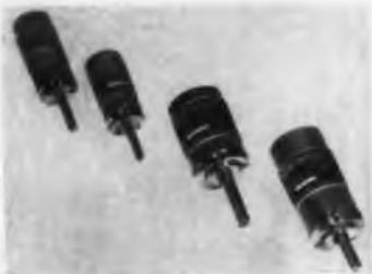
Subminiature mechanical units incorporate a post construction design. Sizes 5 and 8 include stainless steel servo mounting plates, hardened and ground shafts and phosphor bronze traveling nuts. Designed for 0 to 10 turns and 0 to 40 turns, units conform to MIL-E-5272C. Repeatability is within 3 min of arc. Torque ratings on sizes 5 and 8 are 50 and 160 oz-in., respectively.
