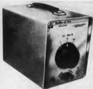
Accuracy is  $\pm 0.05\%$ . Model DFVS-101 has outputs of 1, 10, and 100 v ac rms to load impedances of 10 K, 100 K and 1 megohm respectively. Frequency is 400 cps (with others available on special order) and harmonic distortion is less than 0.1% total. The 12-1/2-lb unit requires 117 v ac, 60 cps.
