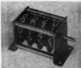
Model 3522 has large digits and is reversible. Drums and pinions are molded nylon in this 1-11/16 x 2 x 3-8/16 in. unit. The 0.420 in. high digits, on 1-7/16 in. diam drums, are either hot stamped or silk screened. The unit comes with either oilite or ball bearings.
