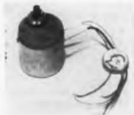
Model R-17-10-1 utilizes two capacitive pick offs per channel arranged in a balanced bridge circuit. An interwinding capacitance toroidal transformer converts bridge unbalance to a low output impedance audio frequency output. The instrument measures approximately 1.66 in. in diam and 1.80 in. in length.
