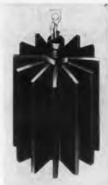
For stud-mounted transistors, rectifiers and diodes. Constructed of aluminum, the model HS 8040 is available for stud-mounted semiconductors with 8-32 to 1/4-in. pipe thread. The dull black anodized unit meets applicable MIL specs. The equipment is said to feature a very low contact resistance and has a surface area of 20 sq. in. per in. of length.
