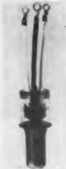
Miniature high vacuum type 581 delivers 13 kw pulse power output in pulse modulator service. Maximum anode voltage is 20 kv; peak plate current, 1.2 amp; and grid bias is 300 v. The tube is 2.75 in. long and 1.13 in. in diam.
