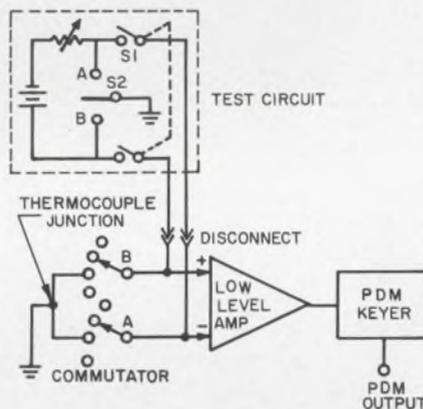
The constant-current source consists of a battery and adjustable resistor. It is connected across the pulse-duration-modulated (PDM) output of the commutator in proper polarity. As each thermocouple loop is sampled by the commutator, the voltage across the loop is proportional to its resistance and the voltage read-out signal is a measure of this resistance.
