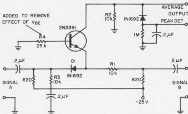
1. Phase shift between two signals A and B applied to the base and the emitter of a transistor results in an output at the collector.
