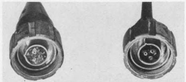
3. To remove cured urethane and reclaim expensive brass connector parts from this power connector (left, both photos), Uresolve was used to remove Products Research Corp. 1538 cable encapsulant. Neoprene cable jacket is unaffected (right, both photos).
