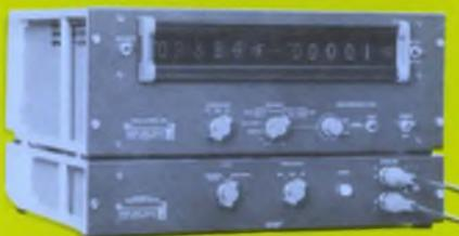
General Radio Type 1680 Bridge automatically measures capacitance and loss simultaneously, generates coded digital output data, and displays measured values in about one-half second. The basic accuracy is  $\pm 0.1\%$  and the range is from 0.01 pF to 1000  $\mu$ F.
