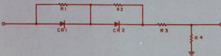
3. Diode limiting of the output amplitude can take many forms. Network shown was chosen for this case.
