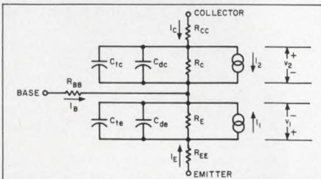
This pnp equivalent circuit can be used for a npn simply by changing the polarity of  $v_1$  and  $v_2$ , the emitter-base and collector-base voltages, respectively.
