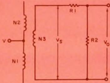
5. Number of secondary turns is determined by the values of R1, R2, and the desired output voltage, V<sub>0</sub>.
