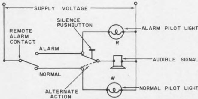
Audible and visual alarm signal will persist until the silence switch is operated and the alarm condition is removed.
