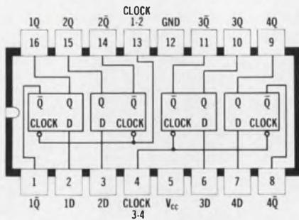
This specialized circuit was designed for readout tube applications. When used with the SN7490 decade counter and the SN7441 decoder/driver, the SN7475 will enable you to realize substantial savings in overall system costs.
