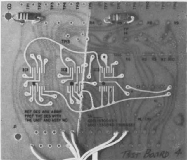
4. Urethane is stripped from this glass-epoxy PC board with a Uresolve gel. The board, the epoxy printing and even the resistor color code are unaffected.
