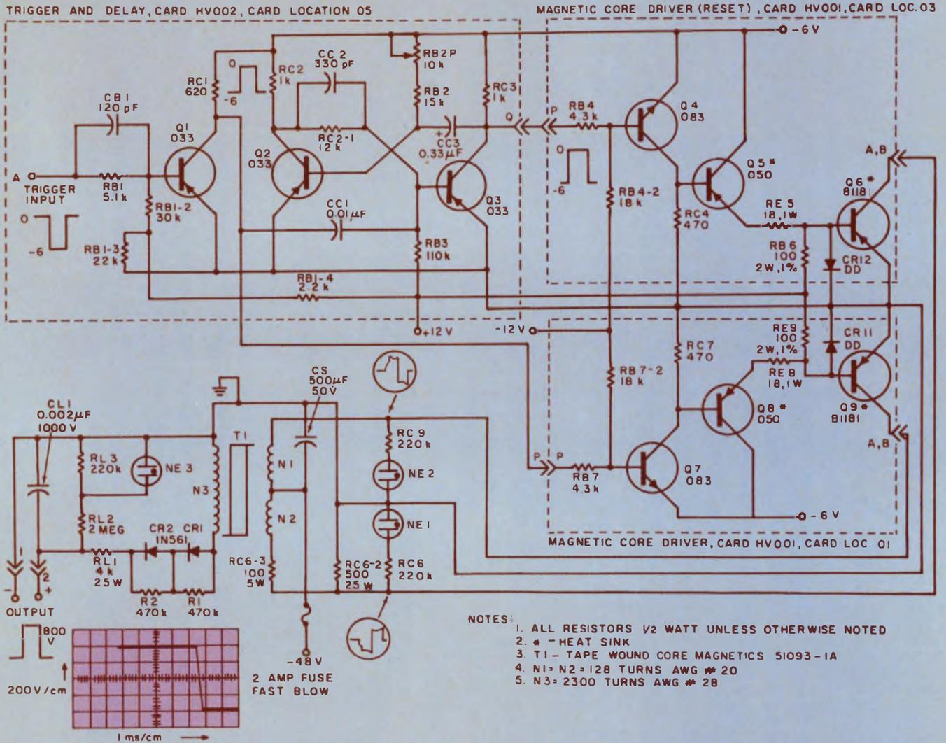
6. 800-volt pulse generator produces accurate clean pulses (see facsimile of the scope photo near the output terminals) of 5 ms duration at 40% duty cycle.
