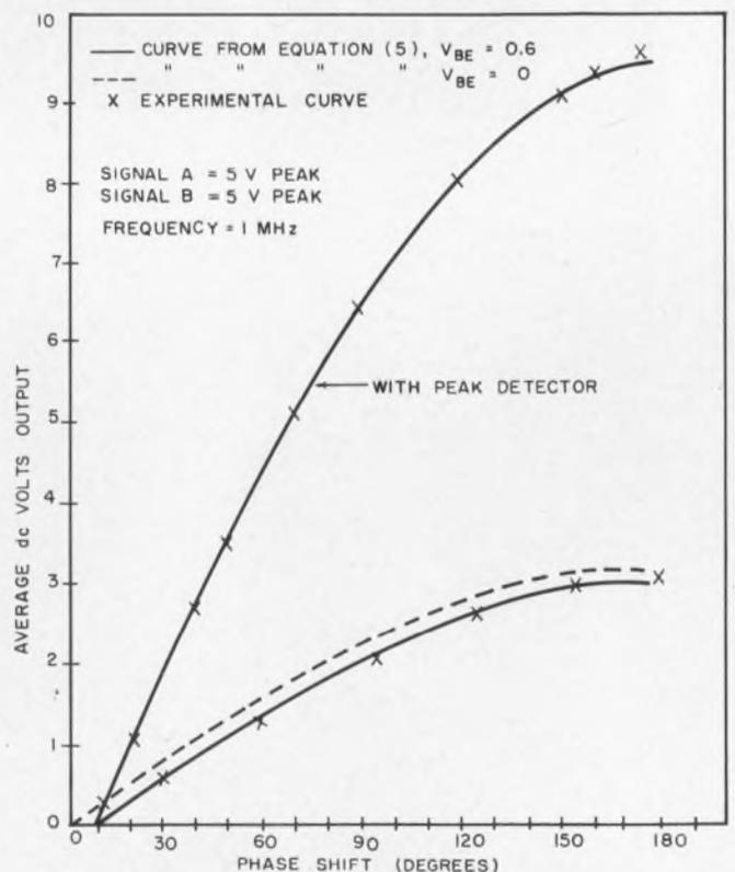
3. Phase shift vs average voltage output shows good agreement between calculated and experimental curves. Value of  $V_{BE}$  shifts the curve by a fixed amount.
