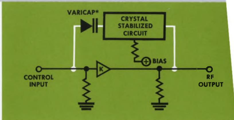
Figure 1 — Simplified Damon VCXO Schematic Diagram
