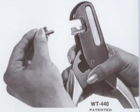
Snap-in dies now make it practical for a single tool to install different sizes of connectors. This light weight, aluminum hand tool features the Shure-Stake technique. Qualified operators can't make a faulty crimp — the tool will **not** release the connector until the compression stroke is properly completed.
