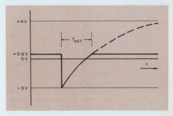
2. The voltage at the base of transistor T1 is pulled to -3 V on application of a trigger pulse, and then rises as  $C_T$  is charged through  $R_T$ . When the voltage on C<sub>T</sub> reaches +0.6 V, the base voltage is sufficient to turn on Q1 and conclude the pulse output.
