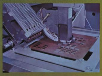
Model 3099 is designed for use with DIP automatic insertion equipment.
