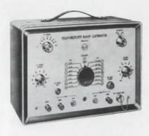
The RCA WR-69A Television/FM Sweep Generator is designed for lab, service, and production applications for sweep-frequency alignment of color and black and white TV receivers and broadcast FM receivers. It's also used to align VHF tuners, picture-and-sound IF amplifiers, video amplifiers and chrominance circuitry in color TV receivers. AND IT'S ONLY \$295.00.\*
