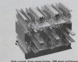
High current, three phase bridge. 1400 amps continuous.
