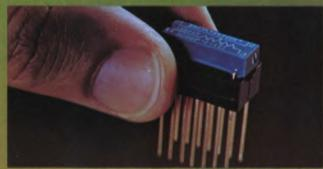
Model 3099 in standard 14 pin DIP socket.
