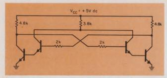
7. A radiation-resistant IC flip-flop (with triggering logic omitted) uses a pseudo-Darlington arrangement to overcome radiation-degraded  $h_{\rm FE}$ . Proper operation of this circuit has been verified after the  $h_{\rm FE}$  of the transistors was lowered to two by radiation,
