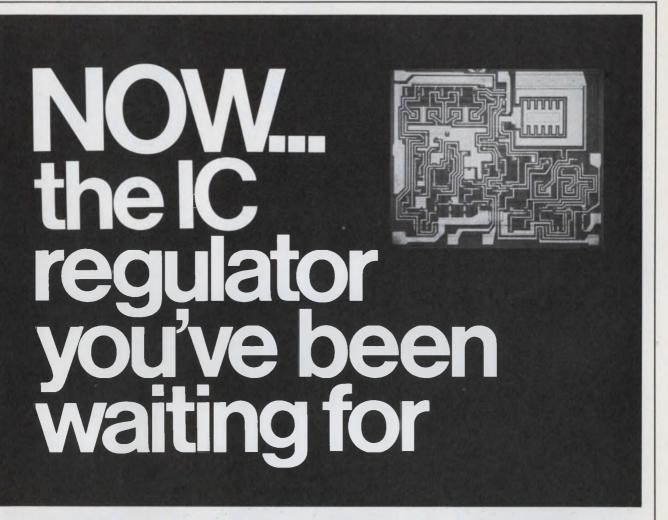
The TVR-2000 – Highest efficiency ... independent, programmable foldback ... 8-40V input range ... output to 200mA ... internal temperature compensated reference.
