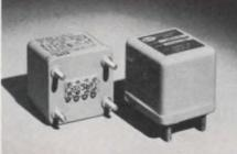
Series 900-064 has been accepted as a standard for many military and aerospace applications where high quality, reliability and cost are requirements. Features: hermetically sealed; fixed or adjustable time delays 0.1 to 60 sec,; solid state or relay output; vibration to 2000 Hz; shock, 50g.
