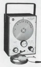
The RCA WA-504A Transistorized Sine/Square Wave Audio Signal Generator covers a frequency range from 20 Hz to 200,000 Hz with exceptional frequency stability. For use in audio, hi-fi and general electronics applications, as well as in electronics training, demonstrations and lab work. ONLY \$95.00\*
