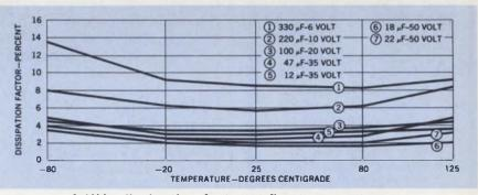
1 KHz dissipation factor at five temperatures
