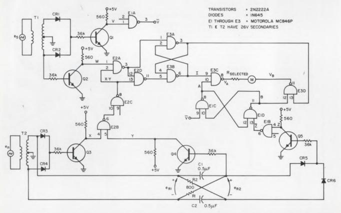
1. Phase shift between two sinewaves is read out directly on the microammeter, M, which can be calibrated to
