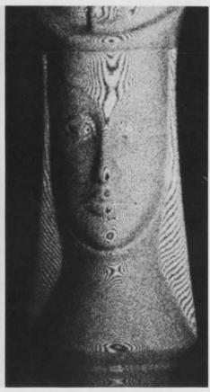
4. Contour mapping, done at Aerojet-General by changing the refractive index of surrounding liquid or gas. At left, the hologram of a chess queen immersed in liquid. At center, the same queen, observed through the first
