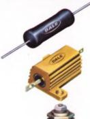
**TYPE RS** Axial-lead, silicone-coated wirewound. Meets MIL-R-26D. Proven failure rate of .006%/1,000 hours backed by 32,000,000 unit test hours (full rated power, 60% confidence, 25° C, failure rate  $\Delta$  R 1%).
