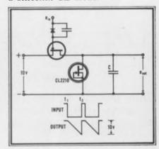
The FET switch is initially closed with C charged to +10v. At  $t_1$  a -10v opens the FET switch. C discharges linearly, due to the constant current characteristic of the CL diode. At  $t_2$  the switch is closed; C is again charged. Sweep time is determined by the values of C and the CL diode. Flyback time depends on C and the FET switch  $R_{ON}$ . FET switches are available with  $R_{ON}$  as low as 5 ohms!
