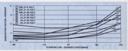
120 Hz dissipation factor at five temperatures
