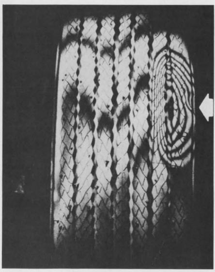
2. A separation at the tread edge of an  $8.25 \times 14$ , two-ply tubeless tire is clearly revealed by real-time holographic interferometry unit built by G. C. Optronics. The tire was inflated to 30 psi and stressed by natural tire creep. The separation is between the tread and the outer-ply.
