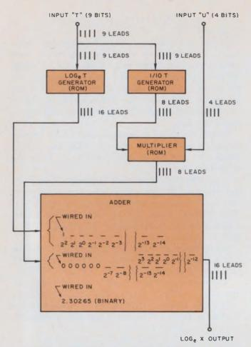
2. A log, X generator, again exclusively MOS, provides log, to  $\pm 2^{-12}$  accuracy. The variable X is inserted as the equivalent function X = 10T + U. This generator uses 9600 bits of memory, against 64,000 bits for a simple table look-up scheme.
