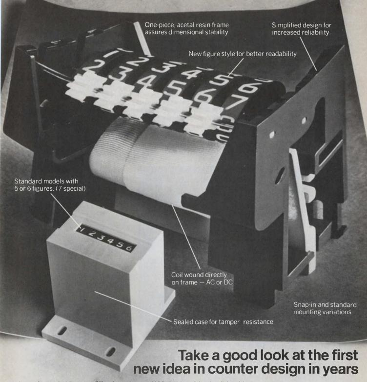
It's the Series 7437 counter. The first of a new MOD 7400 line coming to you from Veeder-Root. What's so new about it? *Total Engineering*. From a multi-purpose frame to a new figure style, pretested for highest readability. The dimensionally stable, acetal resin frame in one piece. All working parts affix to it. From the coil, which is wound directly on the frame, to the verge clapper and wheel shaft which seat in molded receptacles.
