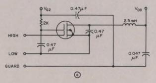
2. Capacitances of dual-gate MOS transistors are measured with these test circuits. Input capaci-
