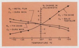
5. The RC network determines the temperature stability, with a secondary and opposing effect from the base-emitter temperature coefficient of the transistor. The variation of output pulsewidth was less than 2 per cent over the range  $-55^{\circ}$  to  $+100^{\circ}$ C when a dura-mica capacitor and tin-oxide resistor were used in the network ( $R_T = 47$ K,  $C_T = 0.001 \ \mu\text{F}$ , output pulsewidth  $= 35 \ \mu\text{s}$ ).
