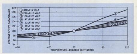
1 KHz capacitance change at four temperatures
