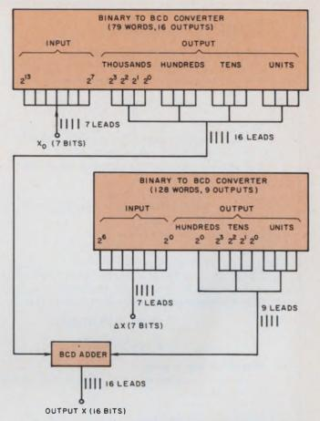
4. An optimized binary-to-BCD converter needs only 2416 bits of memory to cover the decimal range 0 to 9999. This represents a 98% reduction in memory from an equivalence as simple as  $x=x_{\circ}+\Delta x$ .
