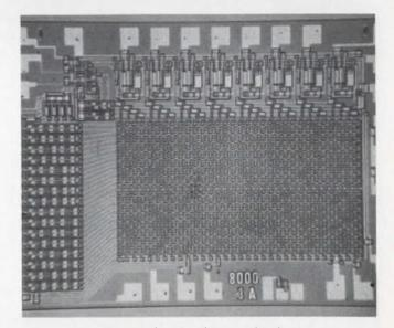
The Philco PM1024 is a typical read-only memory containing 1250 transistors on a 70 by 100-mil chip. Its output of 128 words of 8 bits or 256 words of 4 bits is compatible with either MOS or bipolar circuitry. Cycle times are as low as one microsecond.
