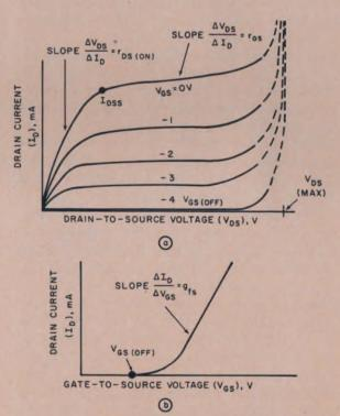
2. Typical MOS transistor curves that can be displayed with reasonable accuracy on a curve tracer include the family of drain-current vs drain-voltage curves (a), and the drain-current vs gate-voltage curve (b).
