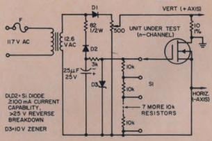
1. Special adapter circuit makes it possible to use a standard X-Y oscilloscope for displaying the output characteristics of MOS transistors.
