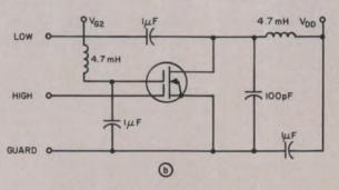
tance is measured with the circuit of (a), and reverse transfer capacitance with that of (b).
