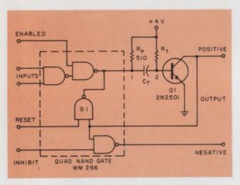
4. The quad NAND gate gives added flexibility. Two sources of input pulses can trigger the one-shot, but only when "enabled." Both positive and negative outputs are available, with an "inhibit" on the negative output. The monostable timing can be "reset" at any time by means of G1.
