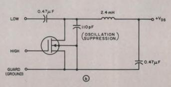
measured with these test circuits. A 1-MHz capacitance bridge is used for the measurements.
