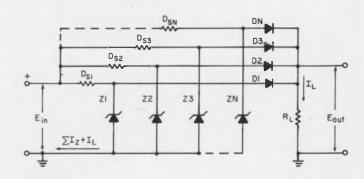
Parallel connection of zener diodes provides a means for drawing high load-current from a dc regulator.
