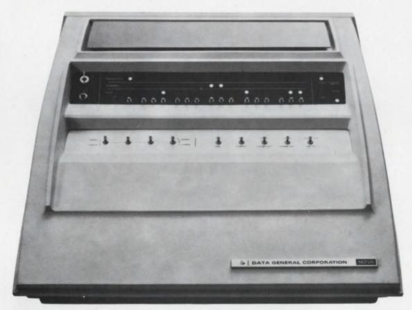
Data General Corporation built a revolutionary computer with Fairchild MSI circuits. The building block approach allowed them to design and build the whole system in six months. And put it in either a desk top console (shown above) or a 51/4-inch high standard 19-inch rack mount package. The central processor fits on two 15-inch by 15-inch plug-in circuit boards.
