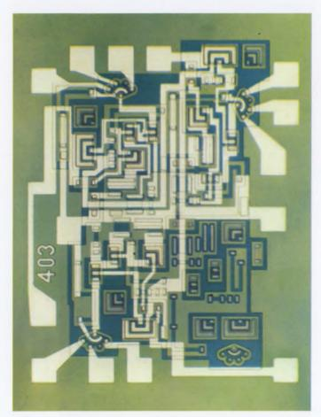
Logic Layout of SF-80, SF-90 dual "D" flip-flop.
