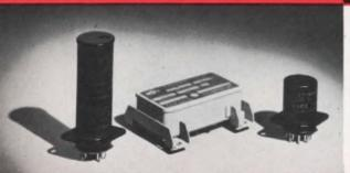
G-V is the largest source and offers the widest variety. Several types are hermetically sealed and still adjustable. All meet requirements of Mil-R-19648. Available in a wide variety including: subminiature, miniature, octal and missile types. Features: delay time, 0.1 sec. to 3 min.; heater voltages to 230 V; ambient operating temp., —55°C to +125°C; vibration to 2000 Hz; shock to 50g.
