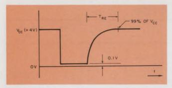
3. The recovery time of the circuit  $(T_{\rm RE})$  is the time required for the voltage at point 1 (Fig. 1) to reach 99 per cent of  $V_{\rm CC}.$  If the circuit is retriggered after only  $T_{\rm RE}$  seconds, the error caused in the output period will be less than 0.7 per cent.
