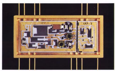
Hybrid construction of high-speed clock driver makes it compatible in size with integrated circuits.
