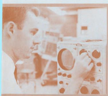
Author Carlson views the family of drain-current vs drain-voltage curves for an MOS unit under test.
