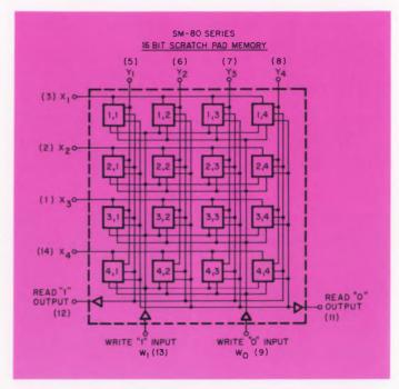
Fig. 1. Logic layout of SM-80 16-bit scratchpad memory.
