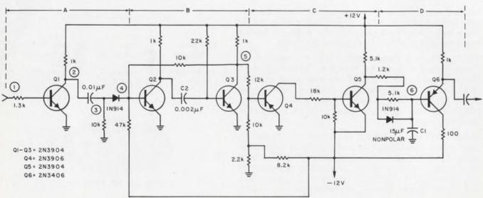
1. Triggered sawtooth generator circuit develops a sawtooth output that has the same frequency as the input but a constant amplitude. The sawtooth has excellent linearity over the range of 300 Hz to about 10 kHz.
