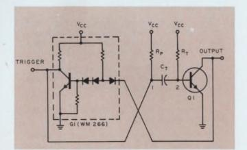
1. The basic monostable circuit uses four discrete components and a NAND gate, with the output pulse duration controlled by the values of  $R_{\scriptscriptstyle T}$  and  $C_{\scriptscriptstyle T}$ . If a duramica capacitor and a tin-oxide resistor are used, the temperature coefficient can be as low as 0.027 % / °C.
