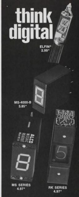
Think ELFIN® — the new single plane, segmented neon readout indicator that provides brighter displays and wider viewing. Only 0.41" dia. ELFIN® displays 0-9, + and -, some alpha symbols and decimal.
