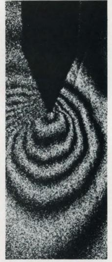
7. Holographic tests of metal toughness conducted by T. D. Dudderar of Bell Telephone Laboratories, show 12 microinch strain contours.
