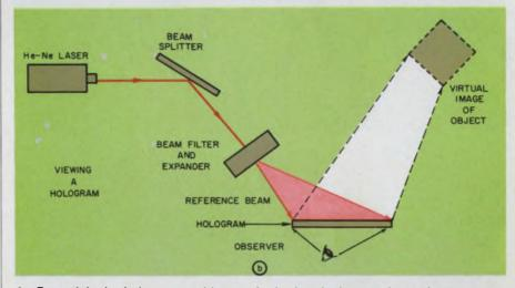
1. Essentials in hologram-making and viewing include a laser for coherent light; a beam splitter for obtaining one beam (the reference) to illuminate the hologram plate and another beam to illuminate the object; expanders to spread the beams; and a stable mount for the hologram plate. The finished hologram is a diffraction grating through which 3-D reconstruction of the object can be seen.
