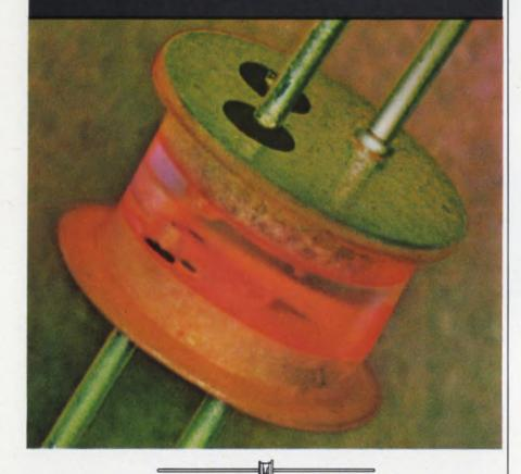
This new photodiode coupled pair offers the designer 5 ns rise and fall times together with over 3,000 volts isolation between input and output. The IR emitter and companion detector are optically coupled through clear epoxy—as seen here. The unit is then encased in opaque epoxy for
