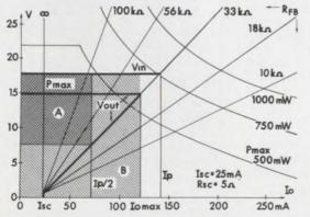
Peak power prediction for typical output characteristics. Programmable foldback permits maximum power dissipation ("A" above) only  $\frac{1}{3}$  that resulting from conventional current limiting ("B" above) or optionally, 3x greater output current with the same power dissipation.
