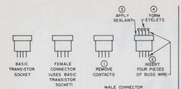
1. Two inexpensive transistor sockets can be quickly converted into a versatile mini-connector.
