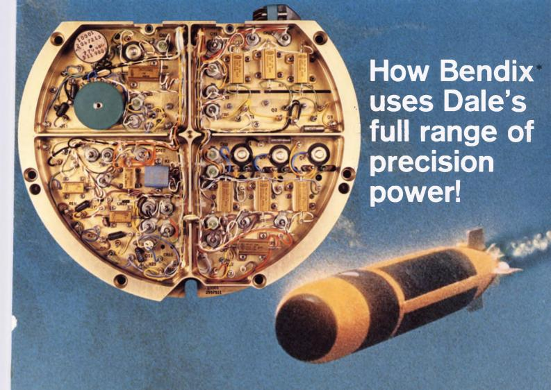
Electrodynamics Division selects Dale Wirewound Resistors for guidance system of Mark 46 submarine hunting torpedo.
