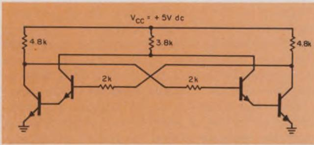
7. A radiation-resistant IC flip-flop (with triggering logic omitted) uses a pseudo-Darlington arrangement to overcome radiation-degraded  $h_{FE}$ . Proper operation of this circuit has been verified after the  $h_{FE}$  of the transistors was lowered to two by radiation.
