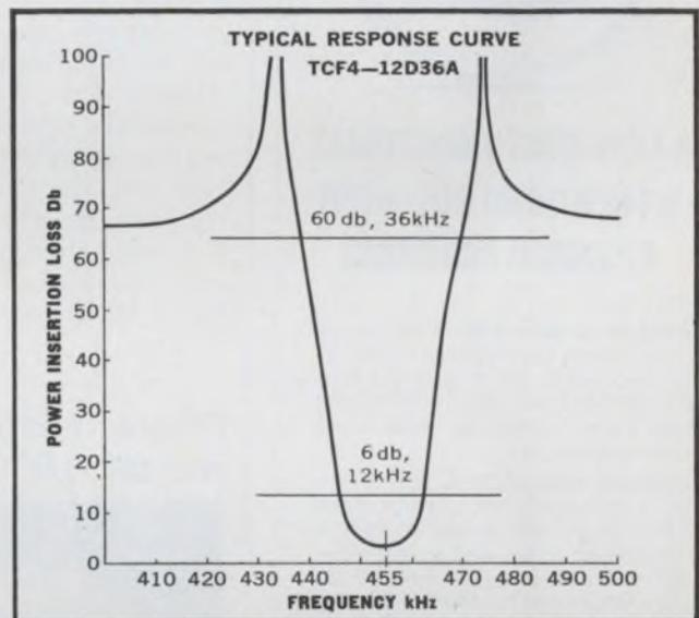
TCF — a hybrid combination of a tuned transformer and ceramic resonators . . . in less than 0.6 cu. in.!
