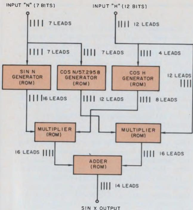
1. A  $\sin x$  generator, built completely of MOS read-only memories, provides the sine function to 14 binary-place (4 decimal-place) accuracy for inputs to within 0.01 degree. The generator uses only 2648 bits of memory, a vast reduction from the 144,000 bits required by an equivalent simple look-up table memory.
