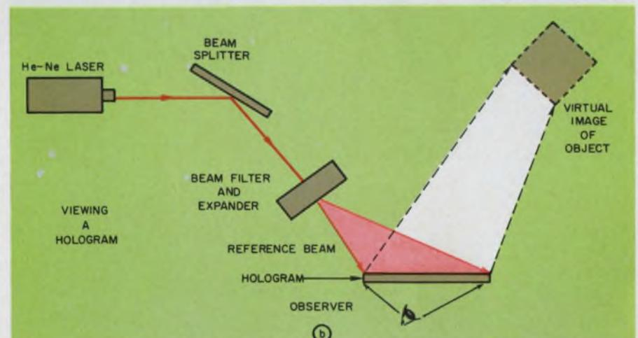
1. Essentials in hologram-making and viewing include a laser for coherent light; a beam splitter for obtaining one beam (the reference) to illuminate the hologram plate and another beam to illuminate the object; expanders to spread the beams; and a stable mount for the hologram plate. The finished hologram is a diffraction grating through which 3-D reconstruction of the object can be seen.
