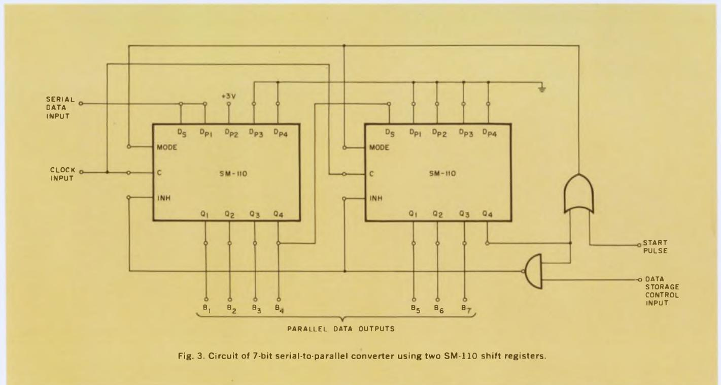
Fig. 3. Circuit of 7-bit serial-to-parallel converter using two SM-110 shift registers.
