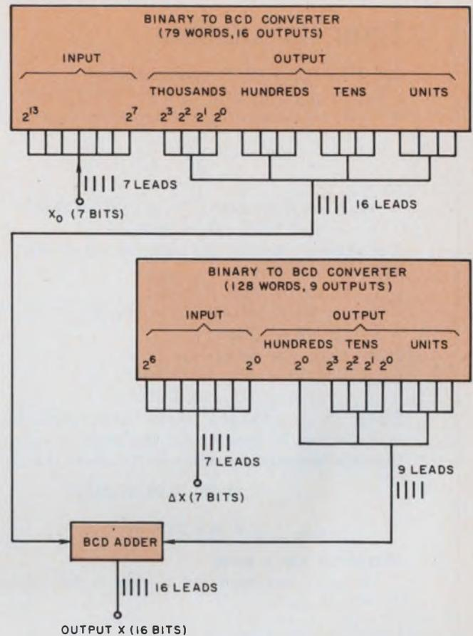
4. An optimized binary-to-BCD converter needs only 2416 bits of memory to cover the decimal range 0 to 9999. This represents a 98% reduction in memory from an equivalence as simple as  $x = x_0 + \Delta x$ .
