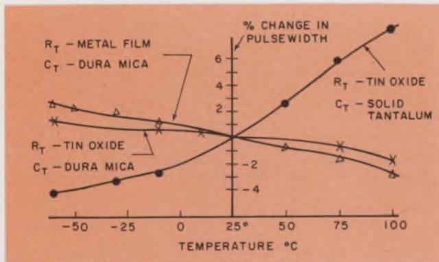
5. The RC network determines the temperature stability, with a secondary and opposing effect from the base-emitter temperature coefficient of the transistor. The variation of output pulsewidth was less than 2 per cent over the range  $-55^{\circ}$  to  $+100^{\circ}\text{C}$  when a dura-mica capacitor and tin-oxide resistor were used in the network ( $R_T = 47\text{K}$ ,  $C_T = 0.001 \mu\text{F}$ , output pulsewidth =  $35 \mu\text{s}$ ).
