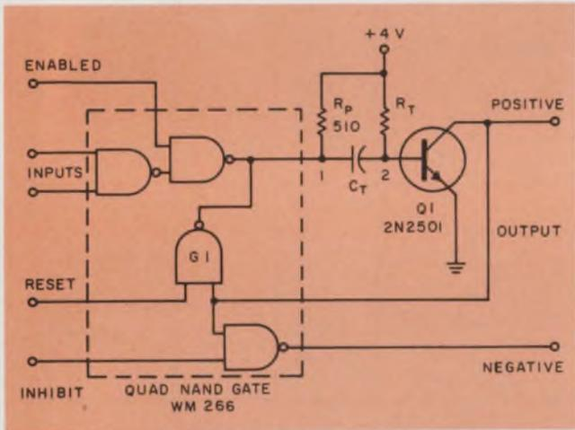
4. The quad NAND gate gives added flexibility. Two sources of input pulses can trigger the one-shot, but only when "enabled." Both positive and negative outputs are available, with an "inhibit" on the negative output. The monostable timing can be "reset" at any time by means of G1.
