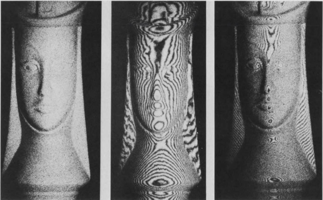
4. Contour mapping, done at Aerojet-General by changing the refractive index of surrounding liquid or gas. At left, the hologram of a chess queen immersed in liquid. At center, the same queen, observed through the first
