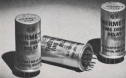
Metal enclosed thermal time delay is dust proof and shatter proof — designed for industrial applications requiring reliable operation and long life. **Features:** temp. compensated; time delays, 2 to 180 sec.; heater voltages, 6.3, 26, and 115V. AC or DC; contacts, SPST, NO or NC.
