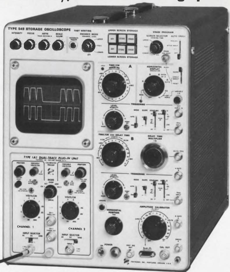
The Type 549 allows up to one hour of continuous visual storage, giving you ample time in most applications to measure and analyze stored waveforms. Stored displays can be erased in less than one-quarter of a second.
