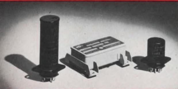
G-V is the largest source and offers the widest variety. Several types are hermetically sealed and still adjustable. All meet requirements of Mil-R-19648. Available in a wide variety including: sub-miniature, miniature, octal and missile types. **Features:** delay time, 0.1 sec. to 3 min.; heater voltages to 230 V; ambient operating temp.,  $-55^{\circ}\text{C}$  to  $+125^{\circ}\text{C}$ ; vibration to 2000 Hz; shock to 50g.
