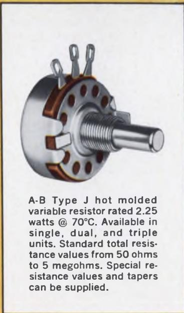
A-B Type J hot molded variable resistor rated 2.25 watts @ 70°C. Available in single, dual, and triple units. Standard total resistance values from 50 ohms to 5 megohms. Special resistance values and tapers can be supplied.
