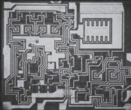
The TVR-2000 – Highest efficiency ... independent, programmable foldback ... 8-40V input range ... output to 200mA ... internal temperature compensated reference.
