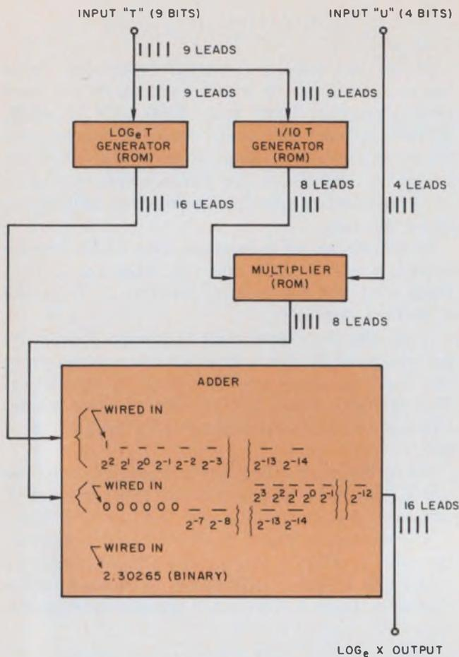
2. A  $\log_e X$  generator, again exclusively MOS, provides  $\log_e$  to  $\pm 2^{-12}$  accuracy. The variable  $X$  is inserted as the equivalent function  $X = 10T + U$ . This generator uses 9600 bits of memory, against 64,000 bits for a simple table look-up scheme.
