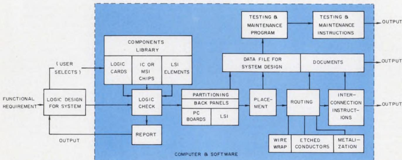
1. Logic system design computer programs throughout the industry are approaching the degree of automation
