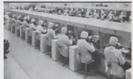
P&B also produces aero-space and military relays which are assembled, tested and sealed in a spacious clean room where all production is under our Intensified Control and Reliability Program.
