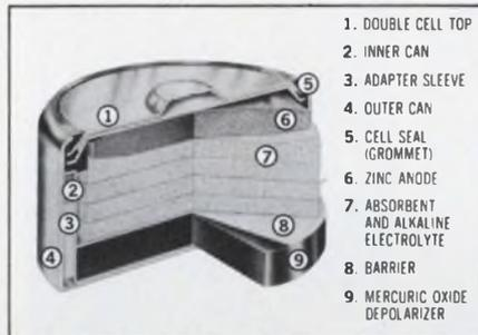
mercury cell has a double steel jacket, and a grommet that can withstand internal pressures up to 300 psi. Potted in epoxy, these cells have performed reliably powering heart pace-makers and other medical-electronic devices actually implanted in the body for years. Ordinary batteries may have no place in the operating room. It's clear that Mallory mercury batteries do.
