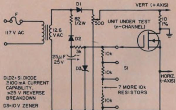
1. Special adapter circuit makes it possible to use a standard X-Y oscilloscope for displaying the output characteristics of MOS transistors.
