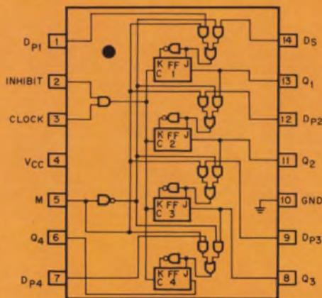
Fig. 1. Logic diagram of SM-110 4-bit shift register.
