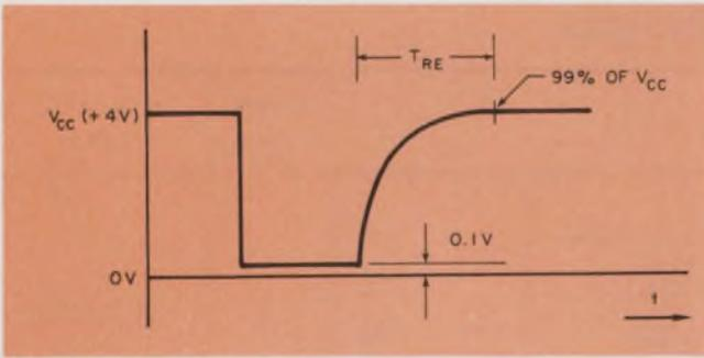
3. The recovery time of the circuit ( $T_{RE}$ ) is the time required for the voltage at point 1 (Fig. 1) to reach 99 per cent of  $V_{CC}$ . If the circuit is retriggered after only  $T_{RE}$  seconds, the error caused in the output period will be less than 0.7 per cent.
