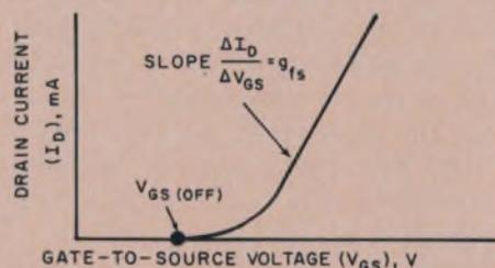
2. Typical MOS transistor curves that can be displayed with reasonable accuracy on a curve tracer include the family of drain-current vs drain-voltage curves (a), and the drain-current vs gate-voltage curve (b).
