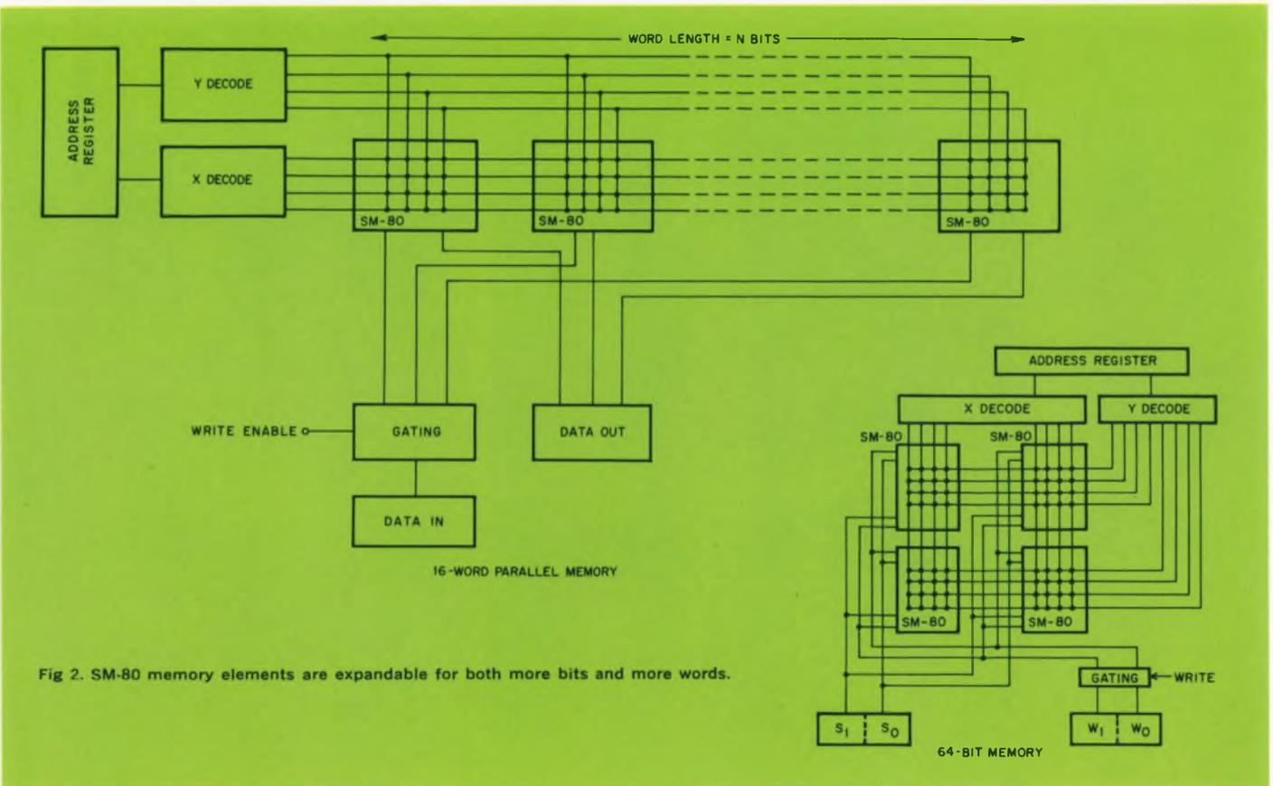
Fig. 2. SM-80 memory elements are expandable for both more bits and more words.
