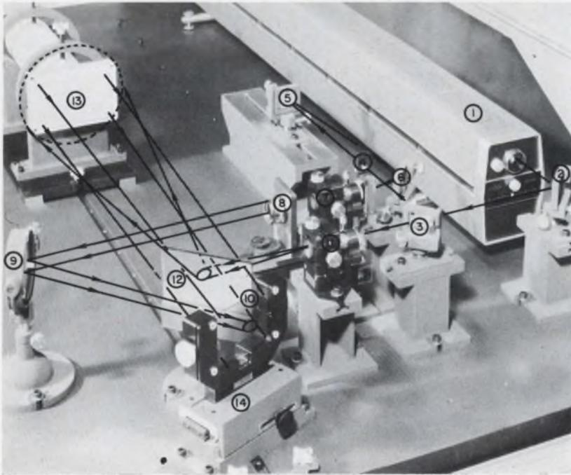
The representative holographic interferometry testing setup, shown here, is made by Optronics, for vibration analysis of rectangular sonar transducers.
