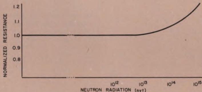
1. Integrated resistors increase in value under radiation, because the p-type material tends to change its behavior toward that of the intrinsic semiconductor. The percentage increase depends on the amount of radiation received and the original impurity concentration.
