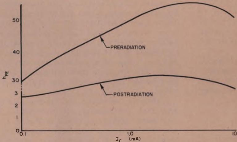
5.  $h_{FE}$  is reduced by fast neutron radiation, and the collector current at which  $h_{FE}$  has its peak value is decreased. The post-radiation curve is the result of a  $10^{15}$  nvt dosage on a silicon npn planar transistor.
