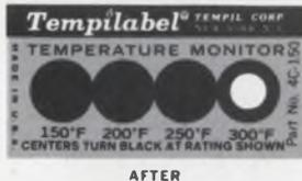
Self-adhesive Tempilabels<sup>®</sup> assure dependable monitoring of attained temperatures. Heat-sensitive indicators, sealed under the little round windows, turn black and provide a permanent record of the temperature history. Tempilabel<sup>®</sup> can be removed easily to document a report.
