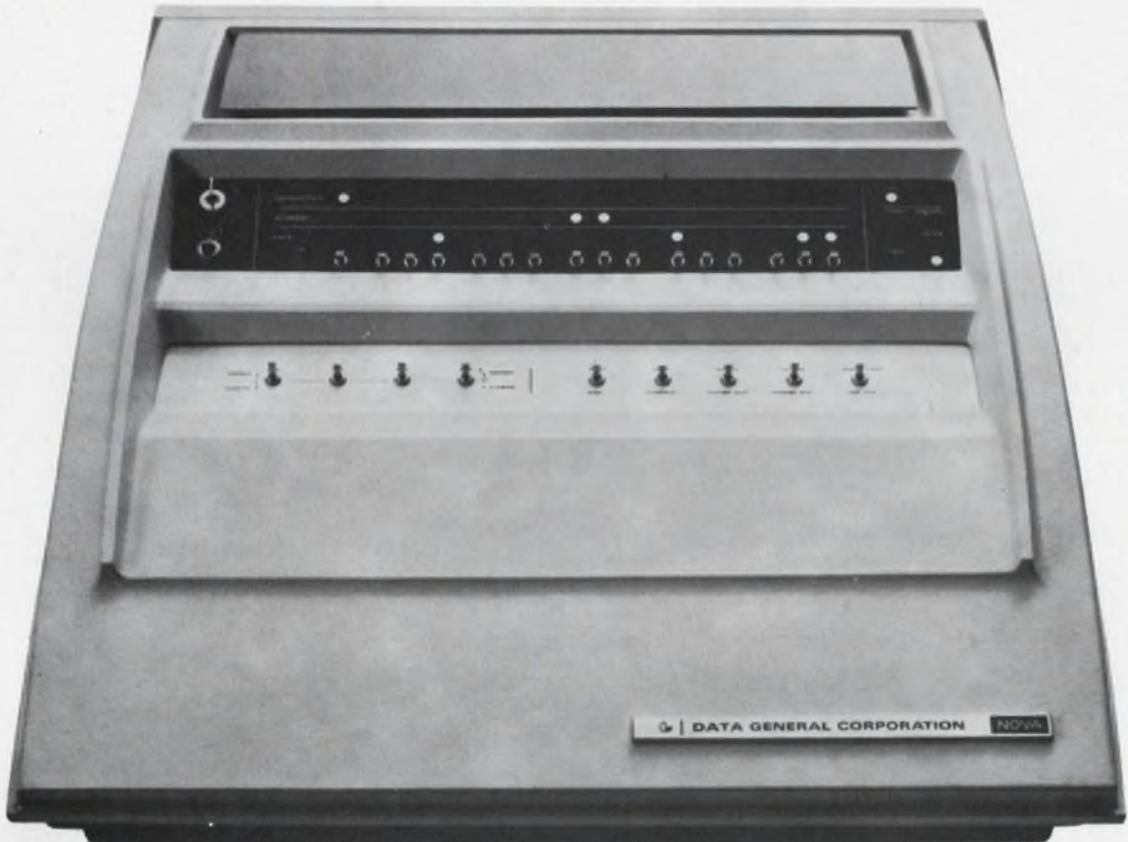
Data General Corporation built a revolutionary computer with Fairchild MSI circuits. The building block approach allowed them to design and build the whole system in six months. And put it in either a desk top console (shown above) or a 5¼-inch high standard 19-inch rack mount package. The central processor fits on two 15-inch by 15-inch plug-in circuit boards.
