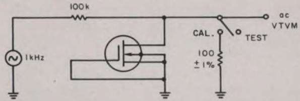
sition, the amplitude of the 1-kHz signal is adjusted until the indicator of the ac vacuum-tube voltmeter points to unity on some convenient scale between 0.1 and 10 mV. The MOS transistor is then inserted into the test socket, the switch is turned to the "Test" position, and the channel resistance is read directly (except for the decimal point) from the voltmeter. The maximum error of the test circuit is 1 per cent when channel resistance  $r_{DS} \leq 1000$  ohms.
