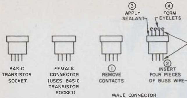
1. Two inexpensive transistor sockets can be quickly converted into a versatile mini-connector.
