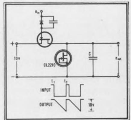
The FET switch is initially closed with C charged to +10v. At  $t_1$  a -10v opens the FET switch. C discharges linearly, due to the constant current characteristic of the CL diode. At  $t_2$  the switch is closed; C is again charged. Sweep time is determined by the values of C and the CL diode. Flyback time depends on C and the FET switch  $R_{ON}$ . FET switches are available with  $R_{ON}$  as low as 5 ohms!
