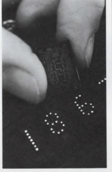
A new solid-state LED numeric display features 5-V logic-level compatibility and a 4-by-7 dot matrix. It also includes a decoderdriver and a memory on the same substrate, plus a red filter, for a cost of only \$10.
