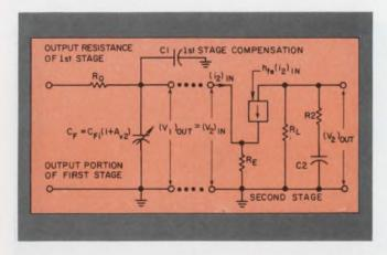
6. Valid ac model of combined first and second stages of the device, with  $C_{\rm Fo}=0$  and with the effect of h-parameters reduced for analytical simplicity. Note that  $C_{\rm Fi}$  is a function of the second-stage gain,  $A_{\rm V2}$ , the impedance of which decreases with an increase in frequency; this variation in  $C_{\rm Fi}$  is compensated by  $C_{\rm 1}$  connected in parallel.
