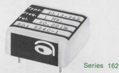
FREQUENCY: 1 Hz to 1 MHz FREQUENCY TOLERANCE: ±0.001% TEMPERATURE RANGE: 0°C. to 60°C. typical SUPPLY VOLTAGE: -20V DC, or +6V DC, or +12V DC OUTPUT VOLTAGE: Compatible with MOS, TTL logic, Sinewave also available.
