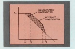
2. Bode plots of both compensation techniques are compared by graphical superposition to illustrate the increased gain for the extended frequency domain. Note the addition of another pole and zero to the Bode plot.
