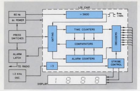
The LSI chip in the clock radio contains timekeeping and alarm circuits that drive the digital readouts. The timing system is controlled by the 60-Hz line. Either the time or alarm-time setting is displayed on command. The cost of the chip is high but will come down in volume production.
