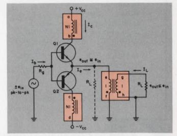
3. The generalized split-load output stage has an N<sub>1</sub>:1 turns ratio between the collector windings and the output windings. In the analysis in the text it is assumed that  $\beta$  is high enough to consider  $I_e = I_c$ .
