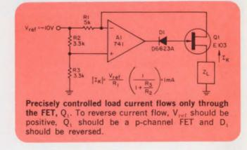
with respect to ground allows the load to be grounded, and active loads can be accommodated as long as the drain-source voltage of  $Q_1$  is maintained greater than its pinchoff voltage.
