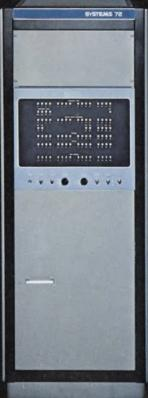
SYSTEMS 810B Word length—16-bit Cycle time—750 nanosec. Maximum core memory—32 SYSTEMS 72 Word length—16-bit Cycle time—880 nanosec. Maximum core memory—65
