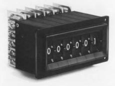
resistance decade, it utilizes a weighted code of 1-2-2-2-2-, using five resistors to achieve nine discrete steps of resistance from (0-9) or multiples thereof. It is a linear progression that yields the desired total resistance.
