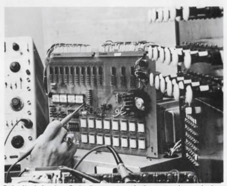
**Entire North American Rockwell organ stop-selection system** is contained on a single printed circuit board. The system contains four MOS/LSI arrays and 550 discrete components.
