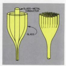
**Fiber electron optics** begin as glasscoated wires (left) that are stacked and drawn into multifiber bundles (right). A new glass-metal conductor makes possible these large-area highresolution arrays. would accept an electron charge and could then be developed with a toner process, like the one used in Xerox machines."
