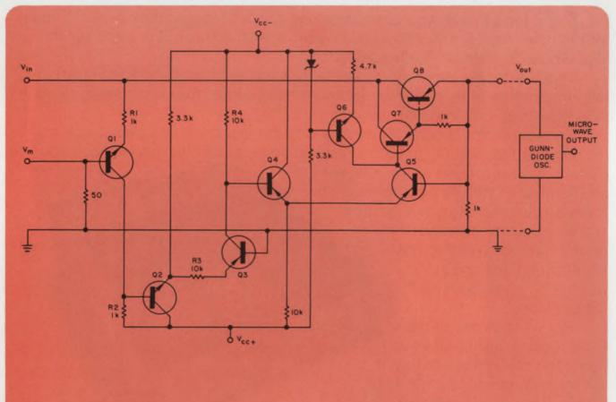
This modulator for X-band Gunn diodes supplies 100 to 300 mA at 7 to 12 V dc. Its output resistance is extremely low, to prevent bias oscillations of the diode. Transistors  $Q_1$ ,  $Q_2$  and  $Q_6$  are ITT
