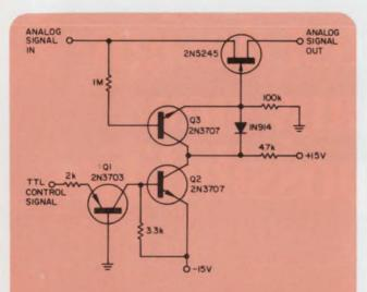
This analog gate can handle large signals because emitter follower  $Q_a$  allows the FET's gate to follow the analog signal input, keeping the channel resistance low over a wide voltage range.
