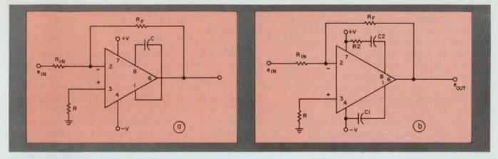
1. The recommended compensation specified by the manufacturer employs a single capacitor that introduces a simple 20-dB roll-off at low frequency and stabilizes the device against temperature variations and parts re-
