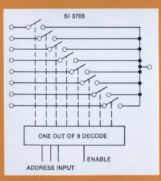
able from Siliconix as are alternate versions with MIL specifications and internal pull-ups for true TTL compatibility. Delivery on schedule.
