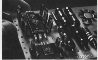
**Power levels of plastic power devices** such as X58's, MS9's, and M386's can be increased up to 80% in natural convection and 500% in forced air when used with PA and PB Dissipators. PA's need only .65 sq. in. to mount; PB's 1.17 sq. in. Staggered finger design gives these light-weight dissipators their high efficiency.
