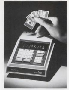
Sharp calculator is mechanized with four MOS/LSI chips and a clock generator. Each chip contains 900 MOS transistor equivalents.
