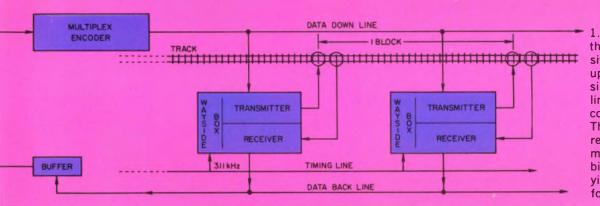
1. Speed commands on the Bay Area Rapid Transit system will be sent to up to 30 wayside boxes simultaneously on a single line with this multiplexed communication system. The comparison of data received with data transmitted in the fail-safe, bit-by-bit comparator yields vehicle location information as well.
