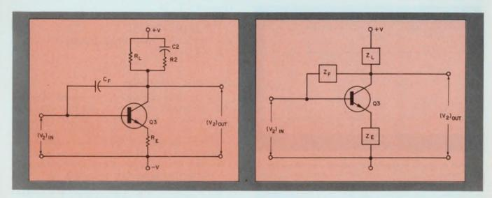
4. The device's second stage is redrawn (a) for analytical simplicity. Internal as well as compensation (external) feedback elements are recognized. The second
