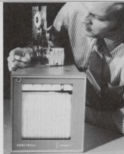
LSI package held by Honeywell engineer replaces the mechanical assembly shown on top of the process recorder case.
