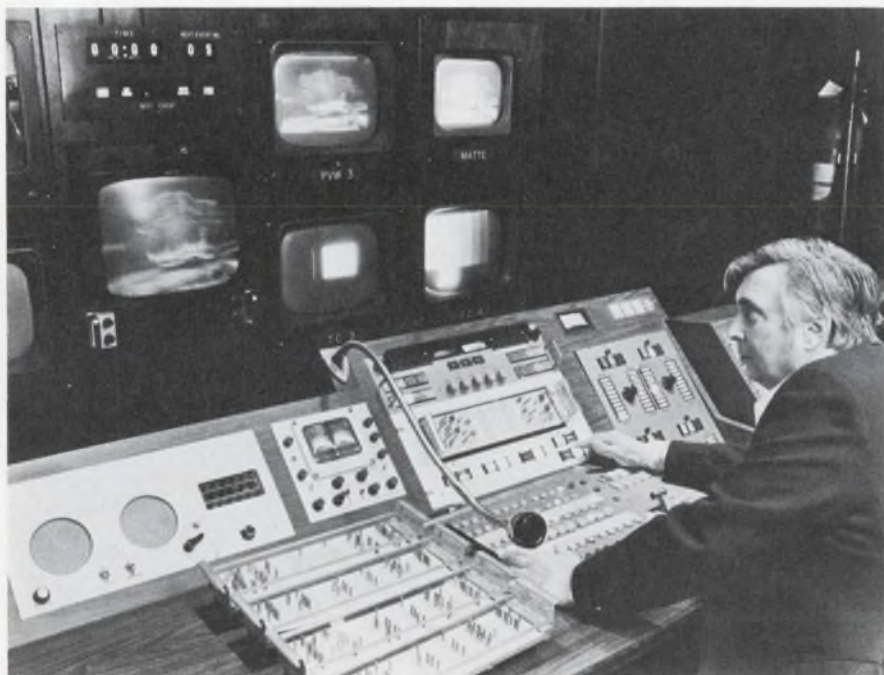
A large number of switching operations must be performed with split-second timing during TV station-breaks. To avoid mistakes, this Chrono-Log Corp. system uses programmed peg boards to control switching.
