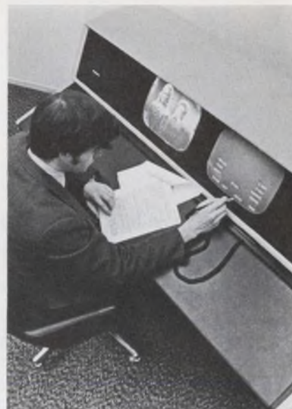
Use of a light pen places edited scenes on a disc pack for storage in this CMX Systems tape editor.
