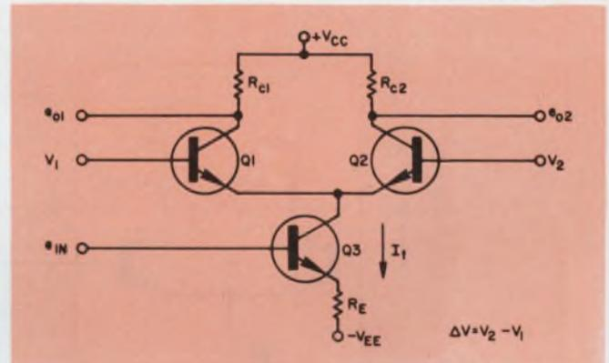
2. In the basic variable-gain amplifier circuit, the input voltage,  $e_{in}$ , is converted to a current by  $Q_3$  and  $R_E$ , and is then divided through  $Q_1$  or  $Q_2$ . The outputs are non-linear functions of  $\Delta V$ .
