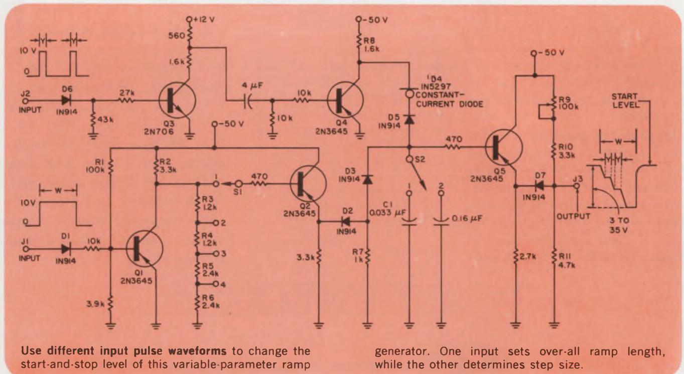
Use different input pulse waveforms to change the start-and-stop level of this variable-parameter ramp
