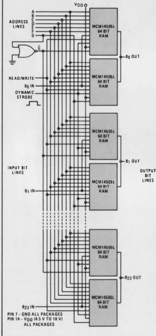
It's simple and practical using Motorola's extremely low power McMOS. The 128-word by 24-bit Static Random Access Memory shown is just one of the many medium speed, micropower organizations possible with the flexible design of the latest addition to this rapidly expanding complementary MOS line, the MCM14505L 64-bit RAM.
