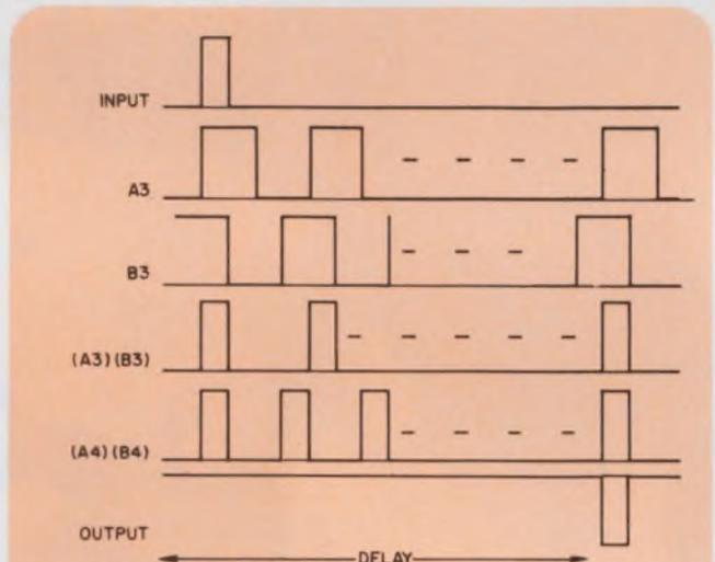
2. A delay between the output of  $A_3$  and its complement,  $B_3$ , is used to create narrow pulses,  $(A_3) \cdot (B_3)$ . Coincidence between  $(A_3) \cdot (B_3)$  and  $(A_4) \cdot (B_4)$  determines circuit timing.
