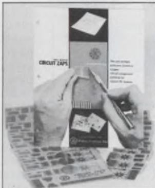
Circuit Zaps® are 1 ounce copper circuit component patterns, pads, and conductor paths, precision-etched on 5 mil (.005") glass epoxy base material, backed by a special pressure-sensitive adhesive. Circuit Zaps® completely eliminate the artwork, photography, photoprinting, touch up, etching, stripping, and other time-consuming steps in PC board development.
