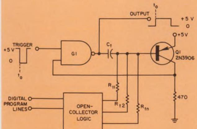
You can digitally control the output pulse width of this hybrid monostable multivibrator. Pulse width, which equals  $0.55 RC$ , is varied through the selection of timing resistance.
