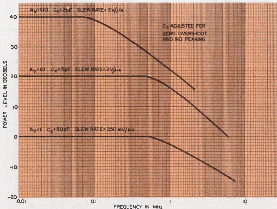
The  $\mu A791$  op amp has a flat response to nearly 1 MHz, for unity voltage gains (lower curve). Responses for higher gains are also shown.
