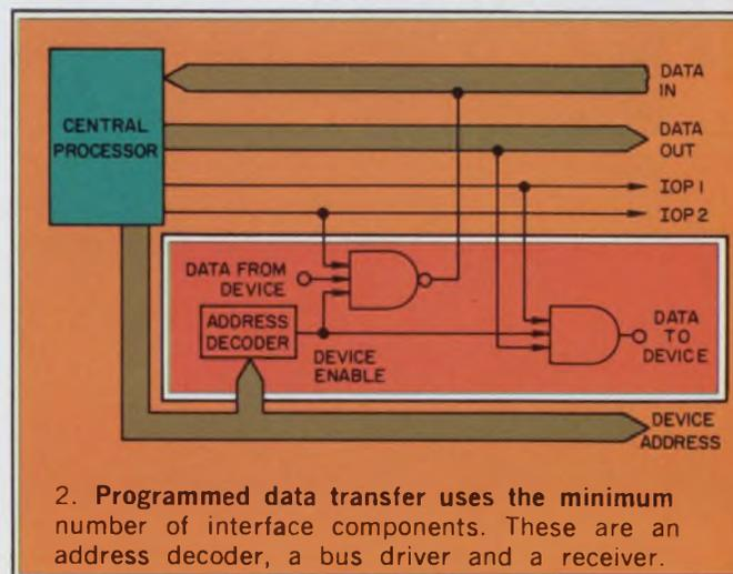
2. Programmed data transfer uses the minimum number of interface components. These are an address decoder, a bus driver and a receiver.
