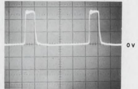
**10-MHz, two-port converter waveforms**
