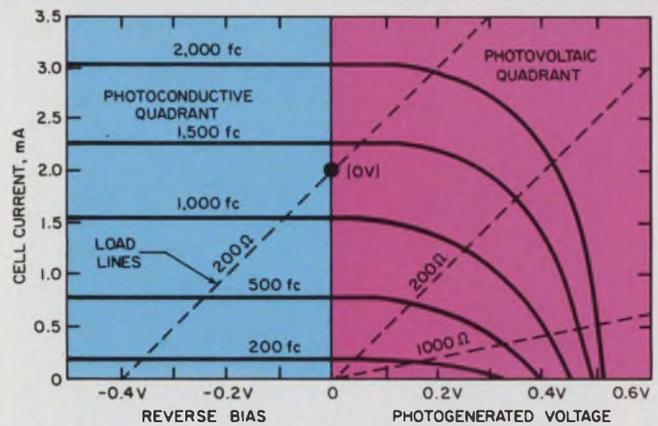
13. The operating characteristics of a photovoltaic cell, by Solar Systems, fabricated for two-quadrant application. With low values of reverse bias and load resistance, it is possible to change the polarity of the output voltage by increasing the illumination from low to high levels.
