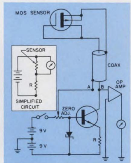
The potentiometer in this Mosimeter radiation-measuring circuit resets the meter to zero after each dose.
