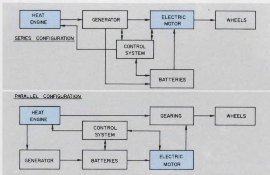
Hybrid electric motors can be designed in either series or parallel configurations. While the series configuration is more flexible and can be produced at a lower cost, the parallel configuration gives lower exhaust emissions by 10% to 20% and is therefore the choice of Aerospace Corp. designers.
