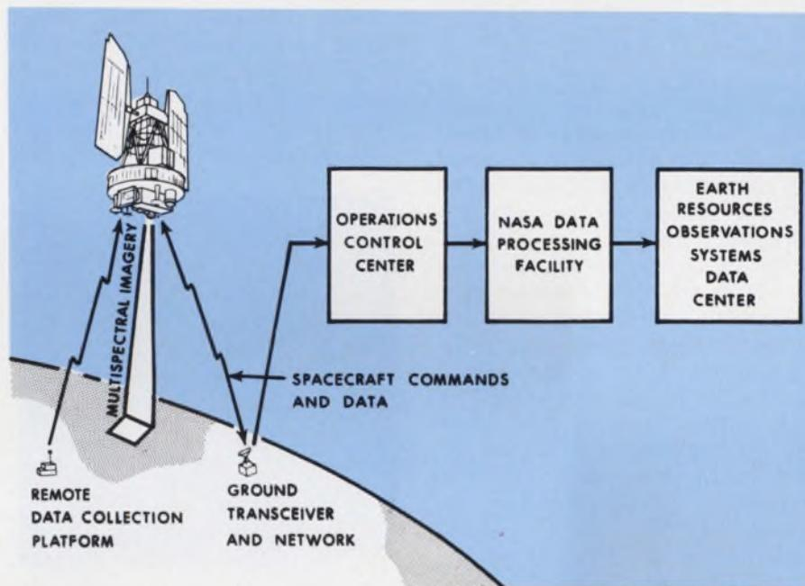
The ERTS satellite will send data it collects plus that from ground-based platforms to Goddard’s ground stations, then to a control facility, to data processing, and on to the data supply center in Sioux Falls, S. D.
