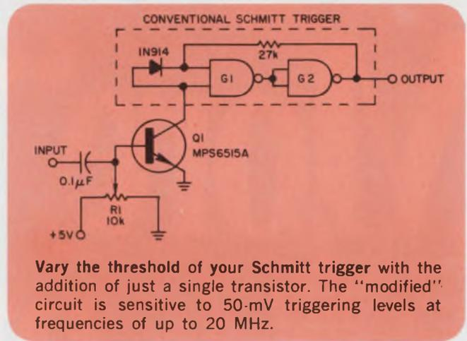
Vary the threshold of your Schmitt trigger with the addition of just a single transistor. The "modified" circuit is sensitive to 50-mV triggering levels at frequencies of up to 20 MHz.
