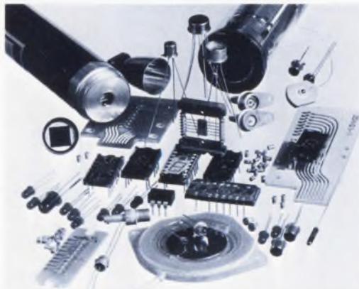
tom arrays or matrices. These complete units can be designed for tape readers, position indicators, pattern and character recognition, shaft encoders and many other special applications. Almost any configuration can be manufactured, and arrays are delivered tested and ready for installation. We can supply sensor arrays only, emitter arrays only, or sensor/emitter combinations. Components can
