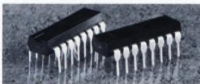
The SN75308 is an array of eight high-current transistors designed for two-dimension memory systems using ferrite cores, plated wire, planar film, diodes, resistors or other memory elements. At 500 mA, collector-emitter saturation voltage is 0.45 V, resulting in low power requirements.
