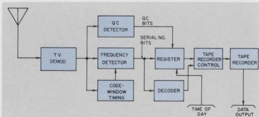
Binary code patterns that identify TV commercials are detected by unmanned monitors tuned to a TV station. The monitor output is recorded on tape. This includes an identification number, the time of day and the presence or absence of test, video, audio or color signals. This data is converted to digital format and stored on tape. Once a day the data is sent via phone to a central processing computer.
