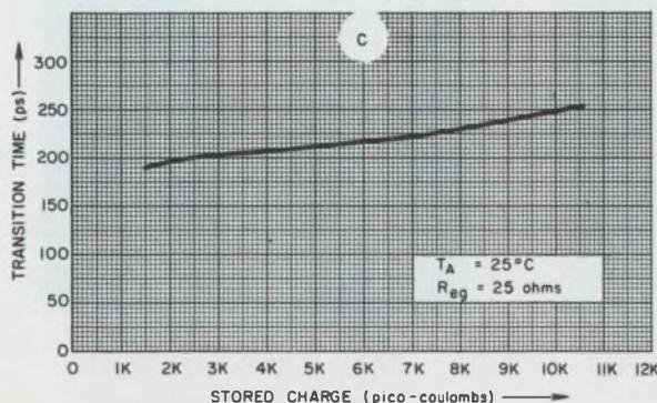
C. Transition time vs stored charge curve for an SV110 pulse snap diode shows the increase in transition time for additional amounts of stored charge. Stored charge is a function of time and  $I_F$ .
