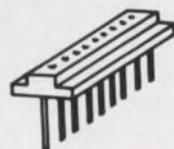
Provides (9) L15E devices on 100 mil centers. Designed primarily for punched tape reader applications.
