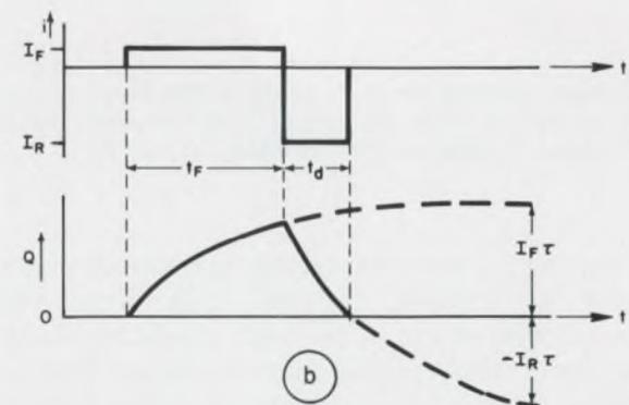
B. Constant current (top) and charge waveforms show that the time,  $t_d$ , to remove the stored charge from a pulse snap diode is dependent on the reverse current,  $I_R$ , through the diode.
