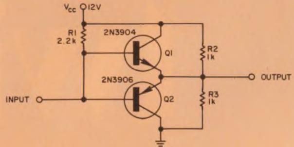
Low-value equal resistors across the output of this complementary emitter driver improve its noise immunity by making it less sensitive to load conditions. Crosstalk is also reduced.
