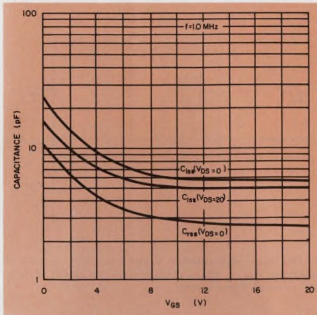
3. Capacitance vs gate-to-source voltage for 2N4091, 4391 and 4856 JFETs.  $C_{rbs}$  is the gate-to-source capacitance;  $C_{iss}$  is the sum of gate-to-source and gate-to-drain capacitances.
