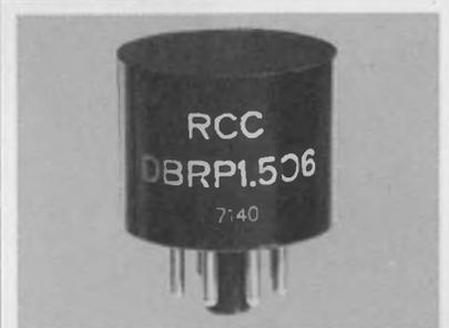
**RCC DBRP1.500 series silicon single phase bridge rectifiers** — Two 1.5 Aav bridge rectifiers in one standard 8 pin octal "plug-in" base. 50-800V., High Rel., Max. Service Appl. 1-99 \$2.95 to \$6.00. Rectifier Components Corp., Freeport, N.Y. (516) 868-0470.
