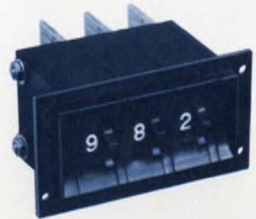
Use these long-life, compact, 10-position thumbwheel switches for data entry, control or programming applications. Decimal and BCD outputs are standard, plus a number of optional coded formats. They're ideal for both matrix and individual outputs.
