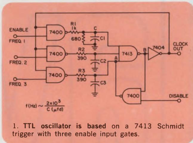
The clock runs until the disable input goes high. If disable goes high when the clock is low (node B high), the positive feedback maintains this state. If disable goes high when the clock is high (node B low), nothing happens until the clock is again low. The system is then latched in the quiescent state. This insures that an integral number of full-width clock pulses is generated, thus eliminating chopped pulses.
