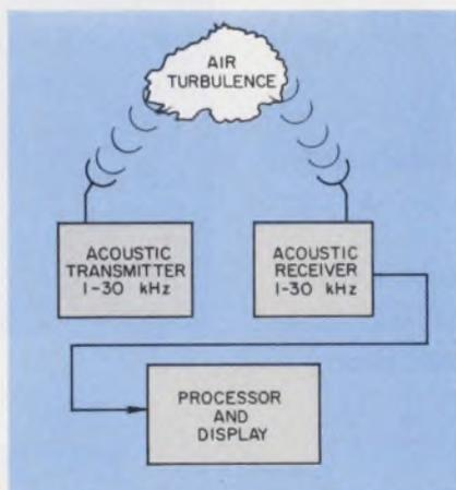
Acoustic radar for detecting aircraft wake turbulence.
