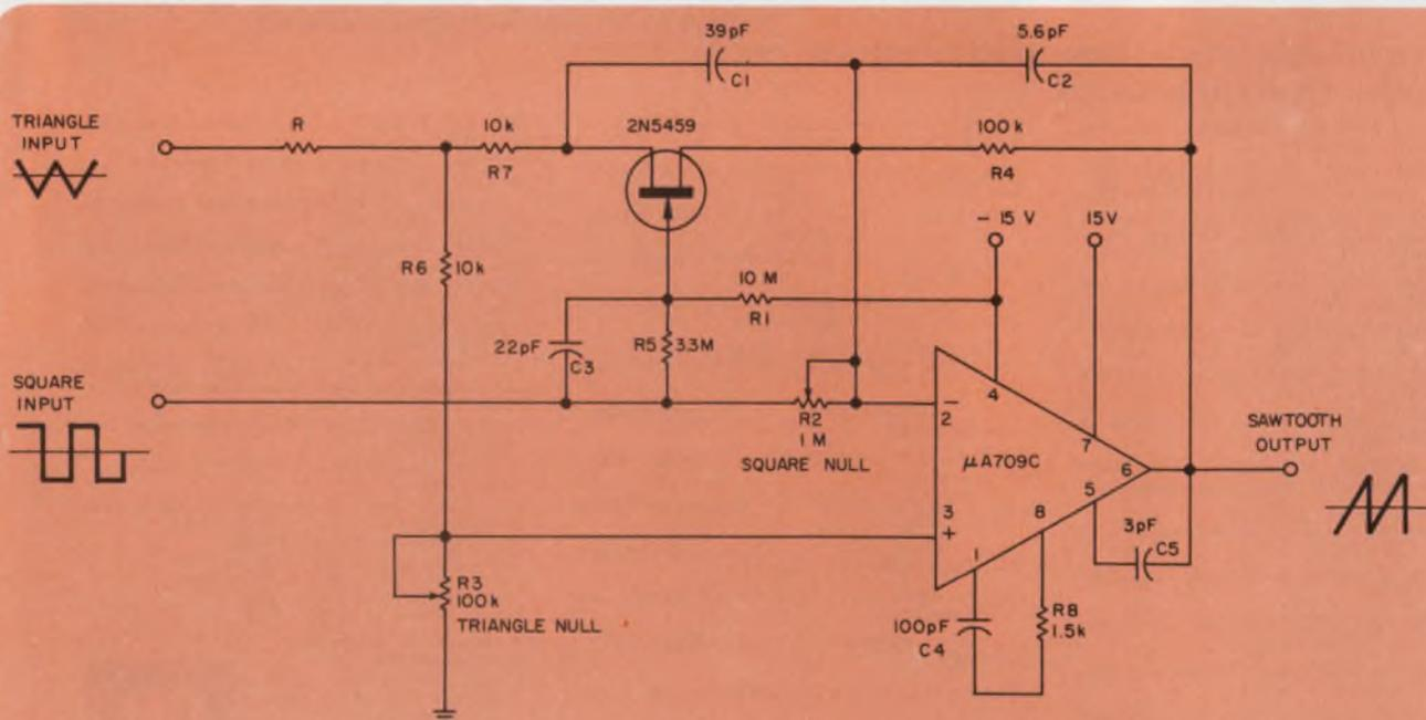
An n-channel JFET chops a triangle input to generate a sawtooth that is synchronous with concurrent
