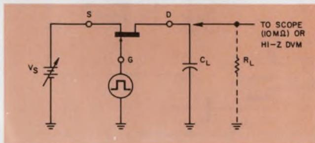
4. Basic circuit for measuring transients by the charge-transfer method.
