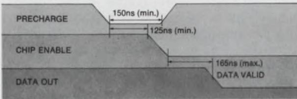
**No Precharge and Chip Enable overlap requirements.** The 3534 requires only that the Precharge pulse stays low for a minimum of 150ns and that at least 125ns delay occur from the start of Precharge to the start of Chip Enable. The Data Out is valid 165ns after the Chip Enable goes low but is independent of Precharge.
