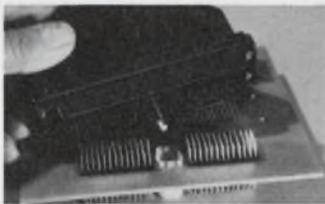
And there's more. The DL *Instamate* contact accommodates #20 through #30 AWG solid or stranded wire. The contact mating life exceeds 10,000 cycles — 20 times the norm. There are contact arrangements with 96 or 156 positions on a .100" grid. Removable con-
