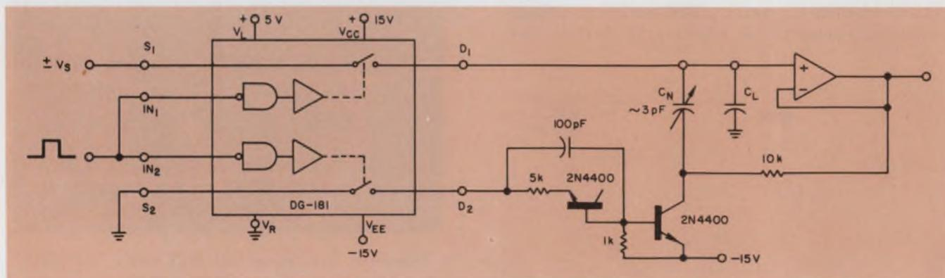
7. This neutralization circuit is almost perfect over a  $\pm 15$ -V signal range. It uses a dual driver and the DG181
