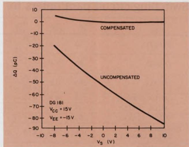
8. Compensation with the circuit in Fig. 7 drastically reduces the change in transferred charge with signal level for the DG181, a 30- $\Omega$  JFET switch.
