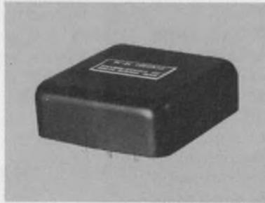
**Isolated dc/dc converters.** Isolation 10 pF and 8 kV dc max. Inputs from 5 to 36 V dc available. Outputs single or dual 8 to 15 V dc 4.5 watts. Noise 5 mv peak (BW 10 M Hz). Regulation 0.05% (Line or Load). Custom Designs no charge. Stevens-Arnold, Boston, Mass. (617) 268-1170.
