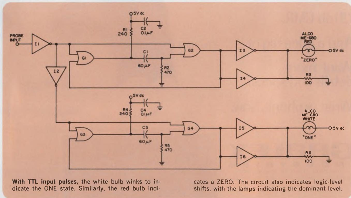
With TTL input pulses, the white bulb winks to indicate the ONE state. Similarly, the red bulb indi-
