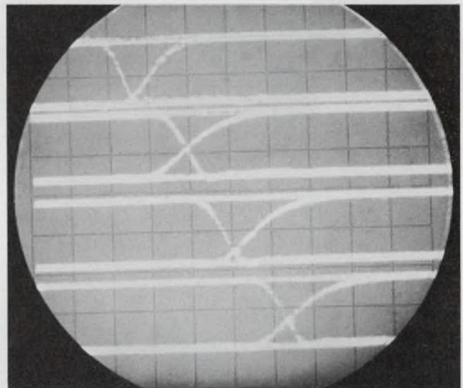
6. Stage-by-stage delays of a four-gate NAND circuit are checked with a pseudorandom generator. The "Xs" depict both positive and negative transition delays. Deflection factors are 10 ns/div. and 2 v/div.
