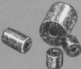
Ceramag<sup>®</sup> ferrite beads provide a simple, inexpensive means of obtaining RF decoupling, shielding and parasitic suppression without sacrificing low frequency power or signal level. Install beads by slipping one (or more) over appropriate conductor(s) for desired effect. Sizes from .020" ID - .038" OD - .050" L. Beads available with leads for PC boards. Send for samples.
