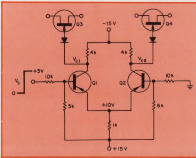
3. JFETs could be used as analog switches, but due to the large pinch off voltages (P-channel), they cannot be driven directly from the comparator outputs. Hence complex and costly drivers would need to be provided.
