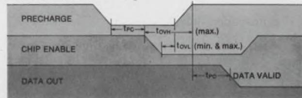
With other 1103's, the Precharge pulse not only must stay low for a precise Precharge interval but its transition from low to high must occur within a time interval which has a *minimum* as well as a *maximum* limit. As a result, the designer must stay within very tight boundaries of these maximum and minimum values. All control circuitry must be extraordinarily precise, and system costs rise sharply.
