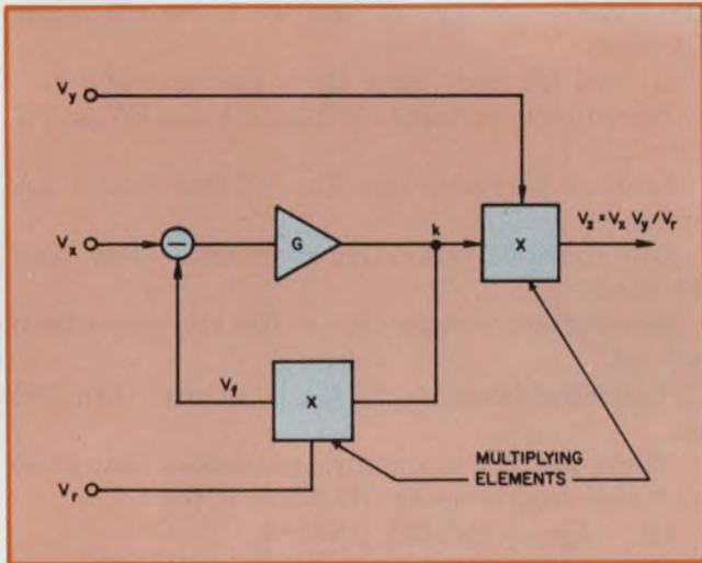
1. Every servo multiplier employs two elements to multiply two signals  $V_x$  and  $V_y$ . The element in the feedback loop normalizes the product with respect to  $V_r$ .
