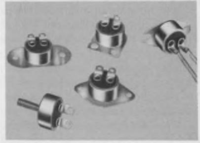
**Precision snap-action thermostats** from Elmwood, widely specified for quick, reliable response; proven industrial and military performance record. Environ. expos. -85° to 550° F; narrow or wide diff.; rated to 15 amps. Prototypes from stock. Wide choice of brackets, terminals. Elmwood Sensors, Inc. (401) 781-6500. TWX 710-381-6413.
