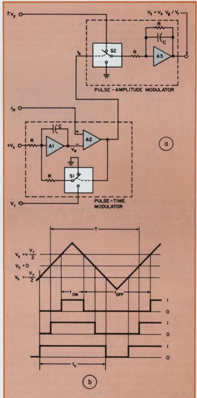
2. Using analog switches as multiplying elements (a), we can build a very accurate pulse-time multiplier. The pulse-width signal,  $t_x$ , is a linear function of one multiplication variable,  $V_x$ , and of the voltage reference  $V_r$ .
