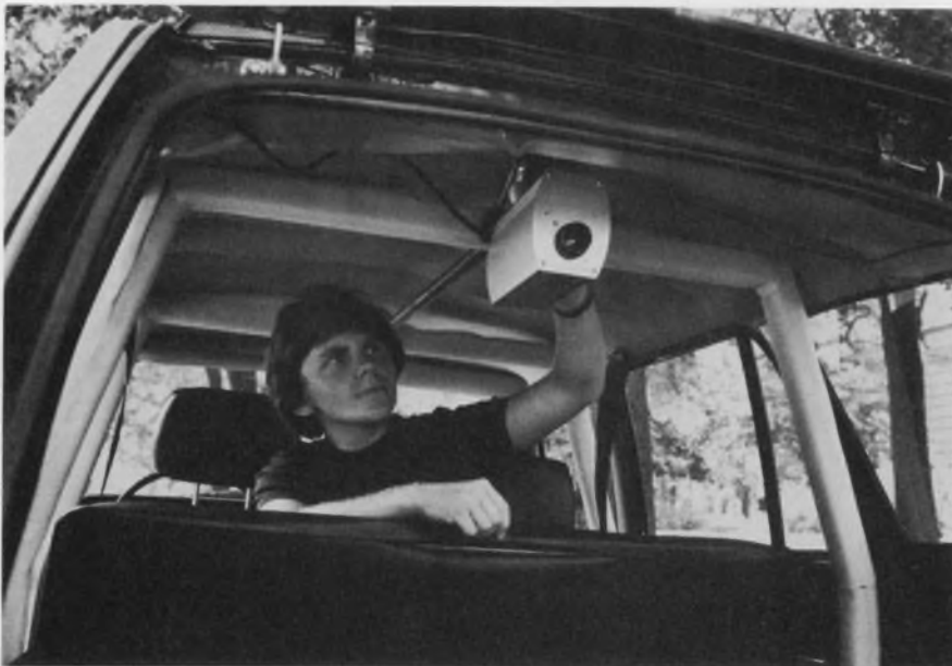
A television camera looks out the rear window in place of a mirror. It covers 90 degrees, operating well in moonlight and in rain.
