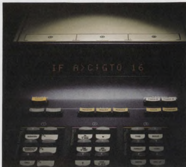
2. A programmable algebraic-language calculator accepts and displays equations almost as you would write them.
