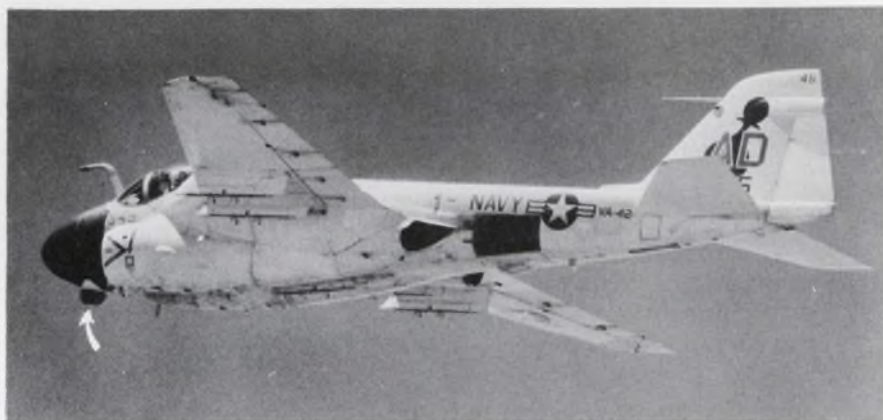
A small bulge had to be built into the A-6E attack plane to accommodate the new infrared-laser sensor system called Tram.
