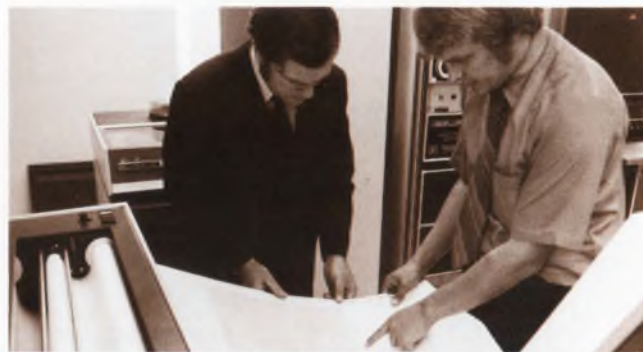
In Motorola's new LocaLogic Design Center, two designers use an X-Y plotter to visualize cell placement.
