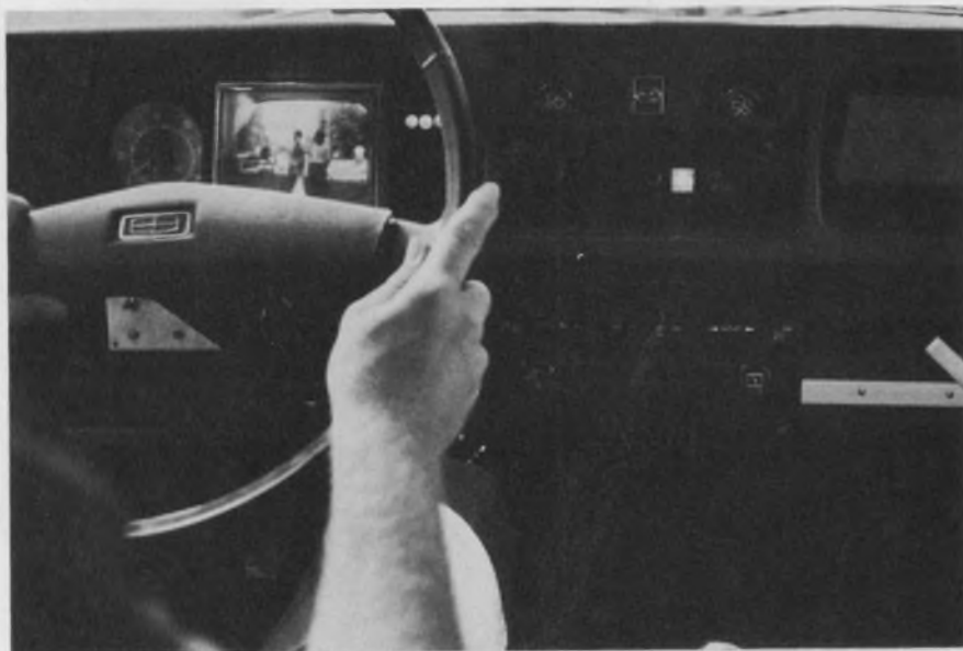
The dashboard instruments (from left to right) are the speedometer, the rear-view TV display and the digital Nixie tube display.
