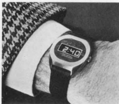
A four-digit dynamic-scattering liquid crystal display gives the time on this Microma Universal watch.
