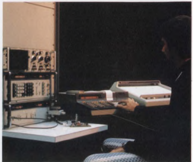
4. Automatic testing, data analysis and logging can be done by coupling a programmable calculator to programmable signal sources and measuring instruments. A programmable frequency sweeper and tracking detector, when added to a calculator, becomes a versatile network analyzer that is simple to program.
