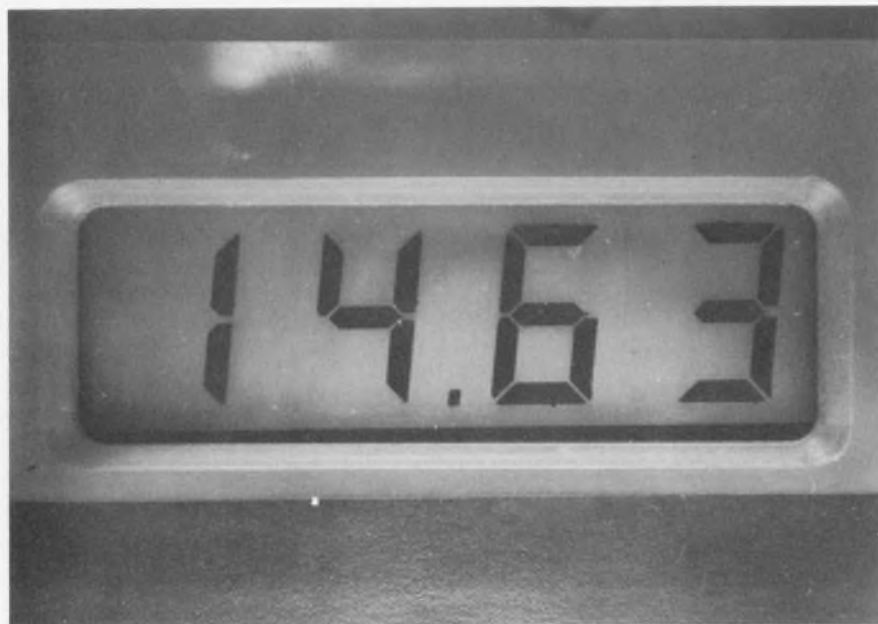
The field-effect, liquid-crystal reflective type display (above) provides better all-angle viewing in diffuse light than does the standard dynamic scattering display. The segments use 7 V from a 60 Hz to 10 kHz source.
