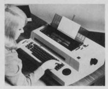
New memory typewriter from IBM can store 50 typewritten pages of information on an internal magnetic tape. Page location is selected by the knob at the right.
