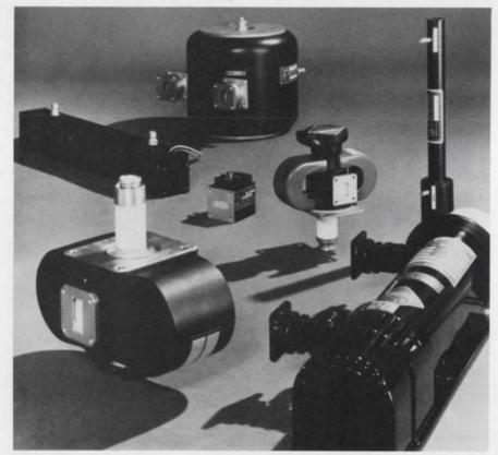
Typical microwave tubes in use today and produced by Litton include (from the top and moving clockwise): Re-entrant beam, distributed emission crossed-field amplifier; pulse magnetron for weather avoidance radar, low-noise, cw traveling wave tube; high-power, coupled cavity TWT; high-power pulse magnetron for military radar applications; high gain, 1-kW TWT. The small cube in the center is a solid-state microwave oscillator.
