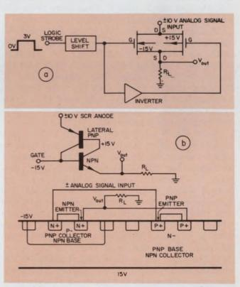
3. No SCR action can occur as long as the  $\pm 15\text{-V}$  supplies are turned on. However, under normal operating conditions, such as the switching of analog signals (a), the circuit can latch up (b). A sufficiently high load resistance,  $R_{\rm L}$ , can avoid destructively high currents.
