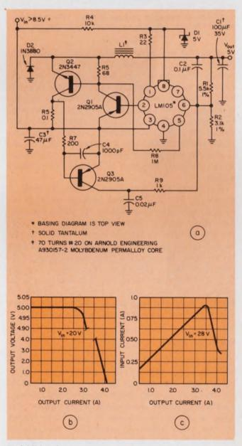
5. Additional components can be added externally to an IC regulator to provide current limiting (a). The achieved characteristics are shown in "b." When the circuit goes into limiting, the input current drops (c).
