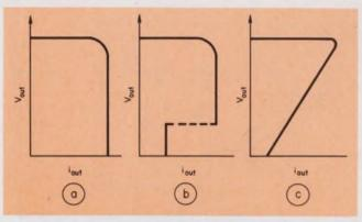
4. Various methods of overload protection can be used. They include current limiting (a), short-circuit shutdown (b) and current foldback (c).
