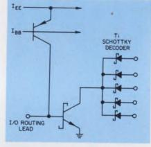
Multiple inputs and outputs are possible with a C<sup>3</sup>L NAND gate. The I/O routing lead connects to the collectors of driving gates.
