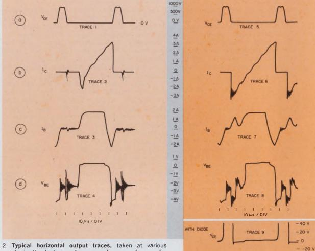
2. Typical horizontal output traces, taken at various points in the test circuit, are used as a reference for circuit modifications to optimize performance.
