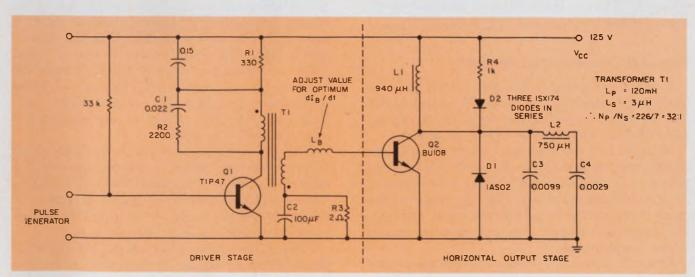
1. A test circuit can simulate the horizontal output stage of most CRT display systems. This can help evaluate the
