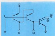
Current-hogging injection-logic NAND gate (left) is 20% smaller than equivalent l<sup>2</sup>L cells. Schematic of cell (right) shows CHL gate with a functionally integrated output transistor.
