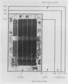
One of the smallest 4-k RAM chips is Intel's 2107B. The memory has 200-ns access.
