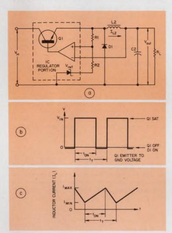
2. Basic elements of a switching regulator consist of a transistor switch, a voltage reference, a comparator and an output filter (a). Regulation is achieved by variation of the relative on/off times of the switch (b). The load current varies as shown in "c."
