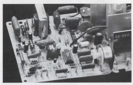
The horizontal oscillator and phase detector of this Sylvania TV-set PLL used for horizontal hold are in the IC (center, front). The oscillator tuning coil shown at the right stabilizes the oscillator frequency.
