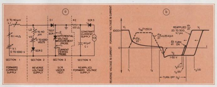
2. Simplified version of a typical SCR test circuit (a) can test for turn-off time as well as many other parameters.
