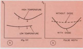
4. Power-dissipation curves of the output transistors are useful in determining safe operating levels for the circuit. Worst-case calculations provide the best guidelines for reliability and stress.
