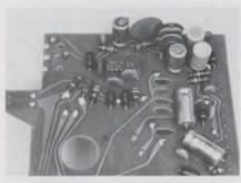
One mass-produced PLL IC is the FM stereo demultiplexer, shown here on a Delco FM auto radio PC board. This IC has a 76-kHz VCO, which is divided into 38-kHz segments for demodulating stereo information.
