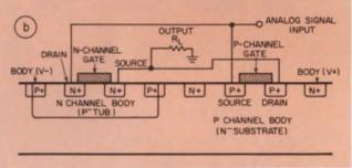
1. A typical CMOS analog switch employs an n and pchannel MOSFET in parallel (a). The gate's cross-section (b) contains three parasitic transistors that are inherent in conventional CMOS processing.
