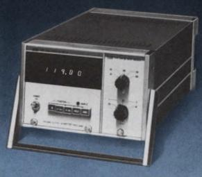
Standard ranges (Multirange Model): 30V/60V/100V/150V/300V, 0.5A/1A/2A/5A/10A (15W to 3,000W) Frequency range: 25 Hz to 1 kHz
