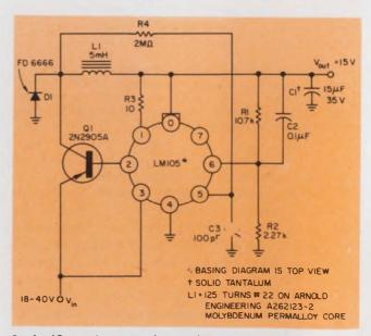
3. An IC regulator can be used as the basis for a switching design. Transistor  $\mathbf{Q}_1$  is added to increase the current-handling capability.
