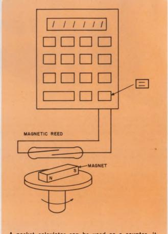
A pocket calculator can be used as a counter. It can count in multiples of any number within its range.
