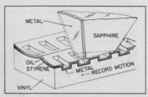
Capacitance pickup detects variations in the width and separation of slots in record groove that contains recorded information.
