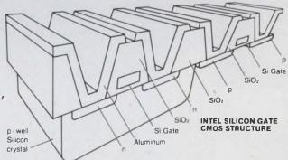
back-up. The 5101 silicon gate CMOS RAM is in full production and in distributor stock, along with our other easy to use n-channel static RAMs.
