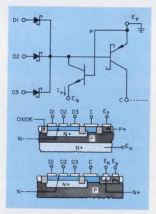
Schottky transistor logic gate (top) uses Schottky diodes and a pnm (m for metal) transistor to get a five-fold improvement in power delay over conventional I<sup>2</sup>L. Practical STL structures can have either vertical (middle) or lateral (bottom) supply injection.
