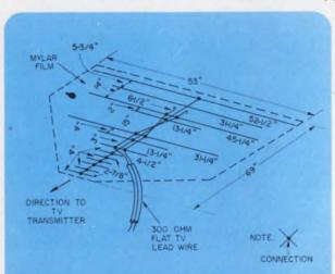
A multi-element TV-antenna array can be easily assembled with adhesive-backed copper tape onto Mylar sheets.
