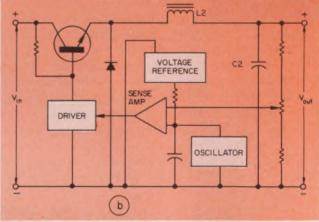
1. Switching regulators can be of the free-running type—in which the transistor operates at constant pulse width and variable frequency (a)—or of the fixed-frequency type, in which the transistor ON time varies (b). Efficiencies exceed those of conventional linear regulators.
