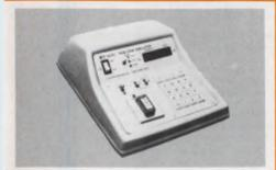
DEVELOPMENT SYSTEM — 65 ns EMULATION CAPABILITY — Allows debugging of software and hardware in microprocessor systems. Plug into any ROM or RAM socket to verify program under actual operating conditions. Display serves as memory map. Programs can be loaded and edited in the 2KX8, 45 ns memory. Choice of ROM or RAM interface · \$1495 ELECTRO-DESIGN, INC., 7364 Convoy Ct. San Diego, CA 92111 (714) 277-2471
