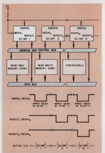
5. **Bus allocation is performed automatically** by SC/MPs. Signals NBREQ. NENIN and NENOUT select which unit has access at any time. SC/MP-1 has the highest priority and SC/MP-N the lowest.
