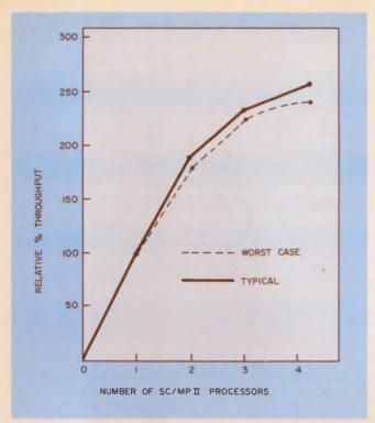
6. **System throughput increases** when three processors share a common bus. But adding a fourth unit doesn't do any good; it will seldom receive access to the bus.
