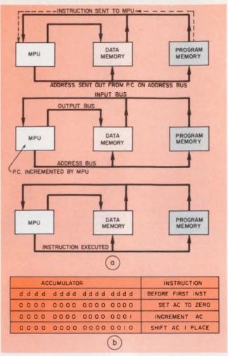
3. The basic instruction cycle for a microprocessor can be broken into three stages (a). All operations on data are performed in the processor's accumulator (b).
