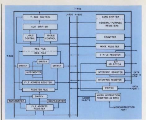
This universal computing element, called Pulce, uses three 16-bit buses to interconnect various specialized registers. Developed in Japan, it's built in an n-channel MOS-on-sapphire substrate, and holds about 20,000 transistors.
