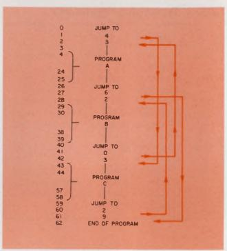
5. Three independent subprograms, A, B and C, can be set to run in any order by a larger supervisory program. All the program must do is initiate each of the smaller programs and wait for that routine to finish.
