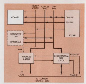
9. With private-bus architecture, you can make each unit in your system into a microprocessor module. The module, which contains its own RAM and ROM, is really a self-contained computer that links up with similar units over a common-bus system.
