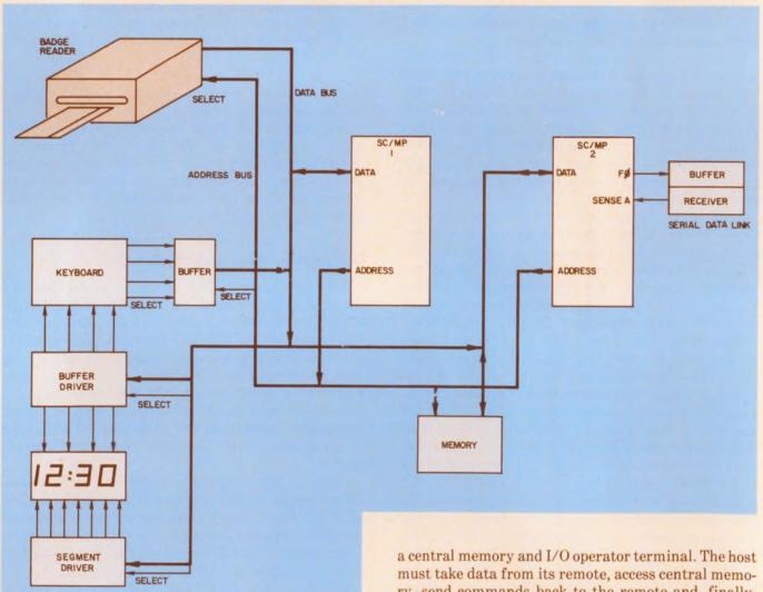
12. Multiprocessing lets you combine three different architectures in one application as in this remote security station. Common-bus is used within the station, which is connected to a central processor via a serial link. A central processor uses private-bus architecture.
