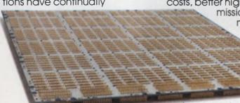
Large scale ECL wire-wrap panel with 660 SIP/DIP patterns.
