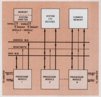
10. Several processors can be connected to the bus in a private-bus scheme. Individual processors are independent of each other, yet have access to memory and system I/O devices.
