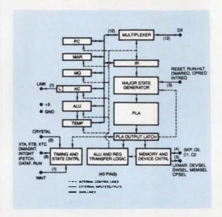
generator and control ROM. All timing and state signals needed by the 6100 are generated by an on-chip clock (only a 4-MHz crystal is required). An internal dividing circuit reduces the clock so that the internal states are 500 ns long.
