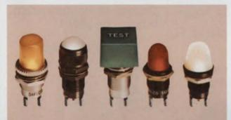
INCANDESCENT OR NEON SUB-MINIATURE INDICATORS—Meet or exceed MIL-L-3661. Mounts in 15/32", 1/2" or 17/32" clearance holes. Incandescent for 1.35-28V; neon has patented built-in current limiting resistor. Choice of cylindrical, faceted, convex, flat, square and round lens shapes, finishes, legends. Stocked by local distributors.
