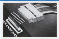
METHODE MASS TERMINATION CONNEC-TORS FOR CABLE-TO-BOARD RIBBON CABLE ON .100" CENTERS. An industry first, "Jaguar 100" connectors eliminate rejections caused by shorts to adjacent conductors, a major cause for rejects when terminating on .050" centers. 1300-200 Series available in straighton and right angle versions. 10 to 28 contact positions (22-26 AWG). Tin plated brass contacts. 94V-0 housings. Methode Electronics , 1700 Hicks, Rolling Meadows, IL. 60008 (312) 392-3500.
