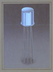
When we first told you about the inherently low inter-contact capacitance and low contact circuit losses of our TO-5 relays, you agreed that they were ideal for RF switching. And you began designing them in immediately. They provided high isolation and low I.L. up through UHF (typical performance 45 db isolation and 0.1 db I.L. at 100 MHz).
