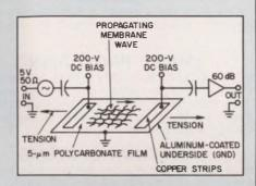
strated to launch 400 to 500-kHz waves with a velocity of 200 meters per second.
