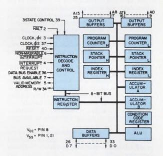
The Read/Write line tells the peripheral devices whether the  $\mu P$  is in the read (HIGH) or write (LOW) state. When the Three-State Control line goes HIGH, it forces the R/W line OFF (high impedance). A Valid Memory Address line tells the memory and peripheral devices that the information on the address bus is a valid address.
