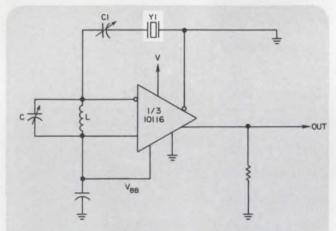
2. **Single-stage oscillators** suffer from frequency shift because the load seen by crystal  $Y_1$  changes.
