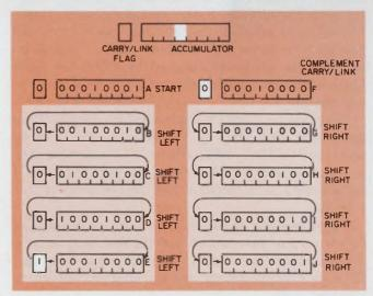
4. To alter the state of accumulator bit 4, the entire contents of the accumulator must be shifted through the carry-link bit of the  $\mu P$ . Once changed, they must be shifted back again to their original position.
