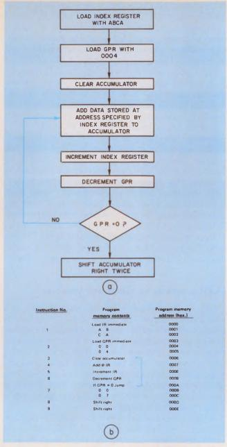
11. Performing the multiple-number averaging using subroutines, this flow chart (a) shows how the processor monitors the value of the general-purpose register. Nine instructions are needed to perform the averaging as well as 15 memory locations (b).
