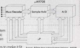
Typical µP Data Acquisition System Utilizing µA9708
