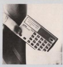
CMOS chips and field-effect liquidcrystal displays combine to cut the power dissipation of two new scientific calculators enough that their batteries needn't be changed more often than once a year. And the units are small enough to fit comfortably inside a wallet or pocket.
