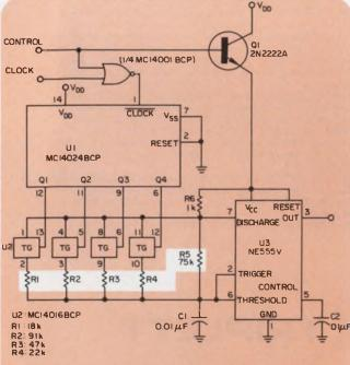
1. The parallel combination of resistors  $\mathbf{R}_1$  through  $\mathbf{R}_5$  determines the output frequency of this pseudorandom tone generator. The frequency is randomized by the count stored in  $\mathbf{U}_1$ .
