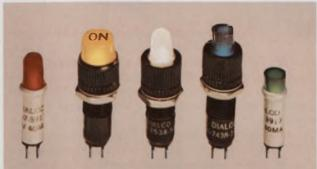
LED, INCANDESCENT OR NEON ULTRA-MINIATURE DATALITES®-Meet or exceed MIL-L-3661. Replaceable plug-in cartridges for 1.35-125V operation. Indicators mount as close as 1/2" centers; available with red, green, amber, blue, white translucent, light yellow or colorless lenses in wide range of lens shapes, legends and finishes. Stocked by local distributors.
