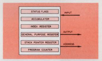
10. **Processors more advanced** than the version modeled in Fig. 2 offer many more registers to the programmer to permit subroutine nesting, on-chip variable or data storage, and special pointers for fast memory access.
