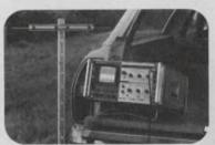
Use the 8554B tuning section to cover the 100 kHz to 1250 MHz range. Maximum resolution is 100 Hz. Measure with  $\pm1\%$  dB accuracy. Its companion HP 8444A Tracking Generator (500 kHz to 1300 MHz) also works with the 8555A tuning section.
