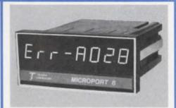
The MICROPORT 8 digital panel display was designed to make interfacing to an 8 bit microprocessor port as simple as possible. The display contains all circuitry required to do its own timing, memory and multiplexing. With proper address decoding for the strobe, the MICROPORT 8 can even be connected to the processor data buss and accessed as a memory location. One year warranty. \$109 (1-4). Jim Eley. Telesis Laboratory, P.O. Box 1843, Chillicothe. Ohio 45601 (614) 773-1414
