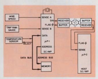
2. A weather station illustrates serial-link architecture in operation. Processors don't have to be hardwired; a modem or radio link can pass data and commands between host and remote units.
