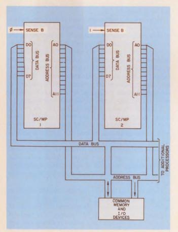
7. Common-bus microprocessors must be separated into their proper starting routines after the system is reset. For SC/MPs, a unique code on the sense inputs gets each unit into its own program.
