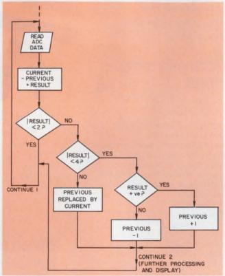
1. **Display jitter is eliminated** when this flow chart is converted into an 8080A microprocessor program. The display is controlled by a small RAM, which is updated only on condition CONTINUE 2.
