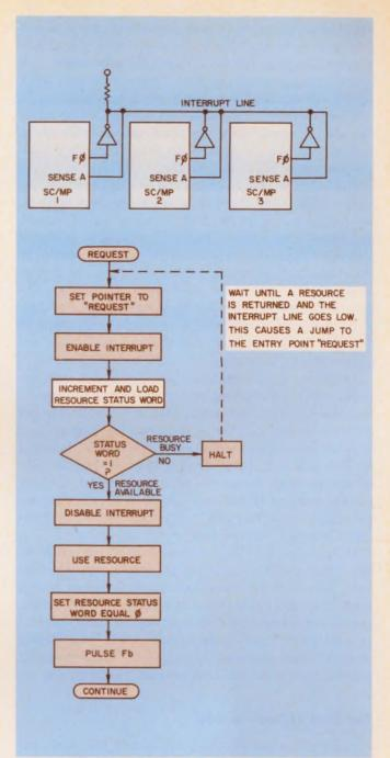
8. It's important to allocate system resources properly, if you want to avoid deadlocks. This flow chart shows how SC/MPs use an ILD instruction to determine if a system resource is available to a processor.
