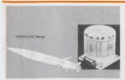
SPRING DRIVEN GYRO FOR MISSILE GUID-ANCE SYSTEMS Rugged, 21/4" diameter, eight-ounce gyro fully qualified to MIL specs and GSA scheduled, contract No. GS-0OS. Solenoid activated, potentiometer on outer gimbal, manual caging, remote electrical uncaging, 100 MS runup time, full rotation, electrical range 357°, resolution 0.25°. Commonality of critical parts ensures low cost and fast delivery. Humphrey, Inc., 9212 Balboa Ave., San Diego, California 92123. Phone (714) 565-6631.
