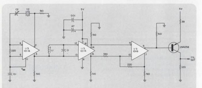
1. A stable harmonic oscillator has three stages: Stage 1 generates the fundamental; Stage 2 is a filter
