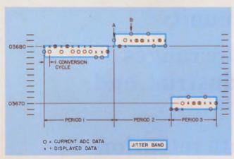
4. **Data eventually settle** in the middle of the jitter band, but not in one conversion cycle. It can take up to three cycles for the data to finally settle.
