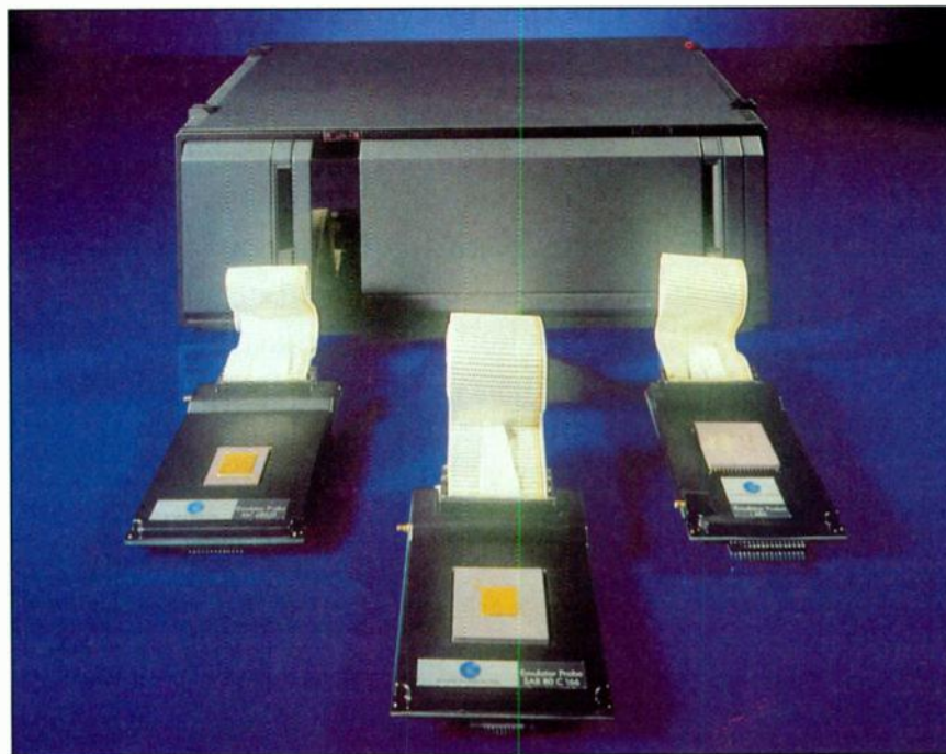
1. THE KONTRON ELEKTRONIK 5SE5 places buffer memory at the probe head thereby reducing signal delays to less than 1 ns.
