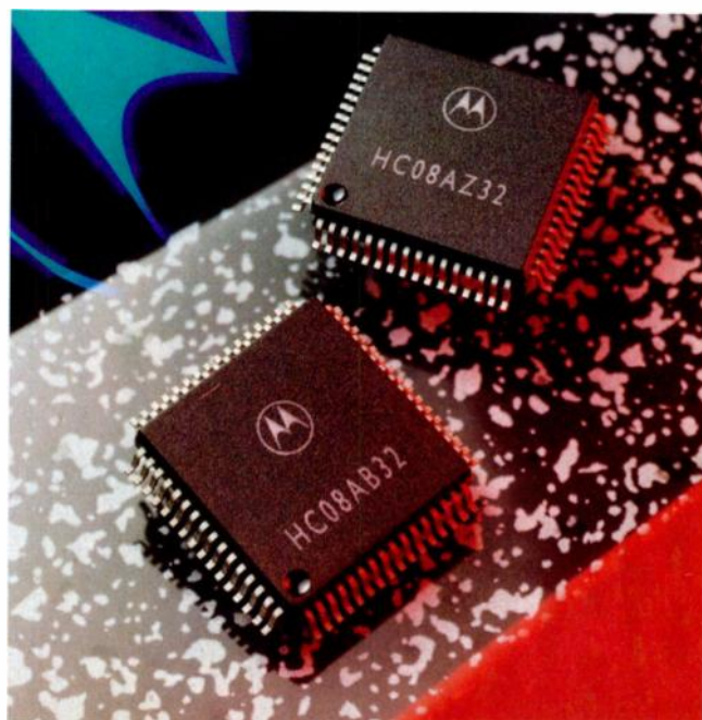
1. FUTURE CAN CONTROLLERS will make use of Motorola's HC08AZ and HC08AB microcontrollers in Swedish Volvo cars. The chips include flash memory.
